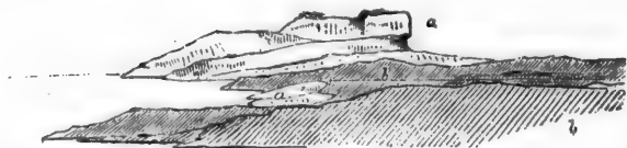
FIG. 7. SKETCH OF OVERLAP OF CRETACEOUS SANDSTONES ON TRIASSIC ARGILLITES. a. Cretaceous sandstones. b. Triassic argillites.
