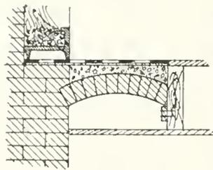
Fig. 1 With Brick Arch
