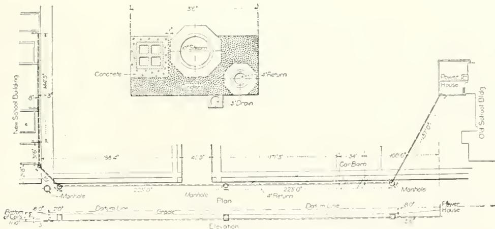
Conduit for Supplying Heat and Electricity to New High School Building
