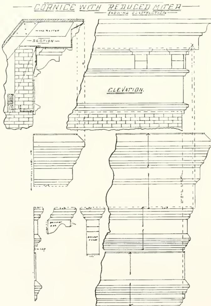
shown in elevation are gotten by the same method as just explained for full projection of section. The stretchout for reduced projection must be taken from reduced profile A of elevation continuing as before explained. The patterns for brackets are gotten by the same method.
