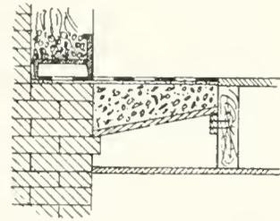
Fig. 2 Without Brick Arch; Section Showing Foundations of Brick Tiling
