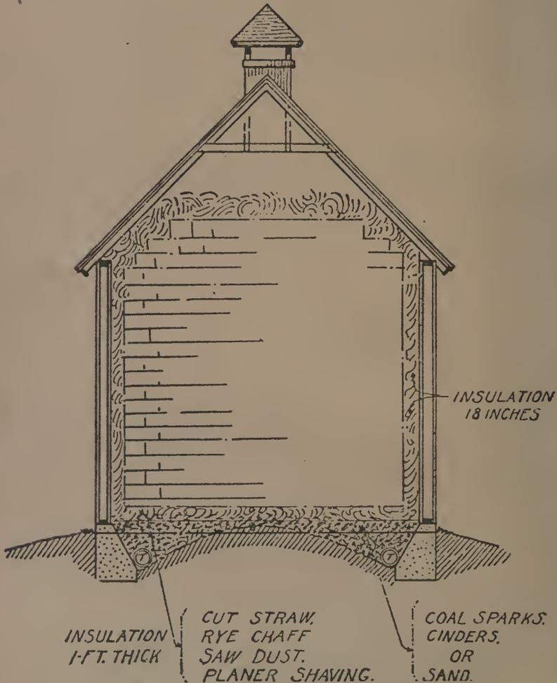
Ice House With Proper Insulation at Base.
