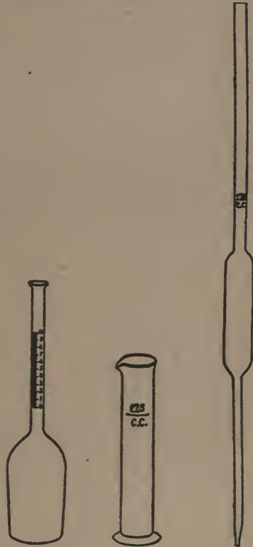
From left to right: Graduated Bottle, Acid Measure and Pipette, used in Babcock Test.
