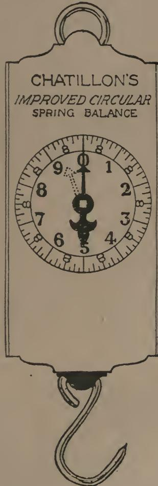
These scales will weigh 30-60 lbs. and have a loose pointer which by means of a thumb screw on the centre may be set anywhere on the dial, thus taking the tare of the milk pail. The price of these is given in test of dairy equipment.
