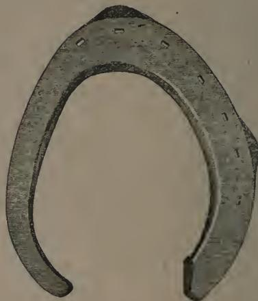
Ground surface of shoe to left. Inner nailer's branch is same in depth as the outer and caulked on to balance foot squarely on the ground.
