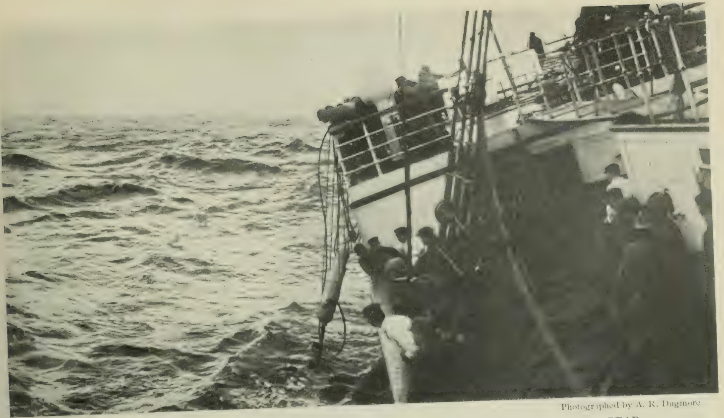
THE LINER WITH BROKEN RUDDER LOWERING BOOM FOR JURY STEERING GEAR
