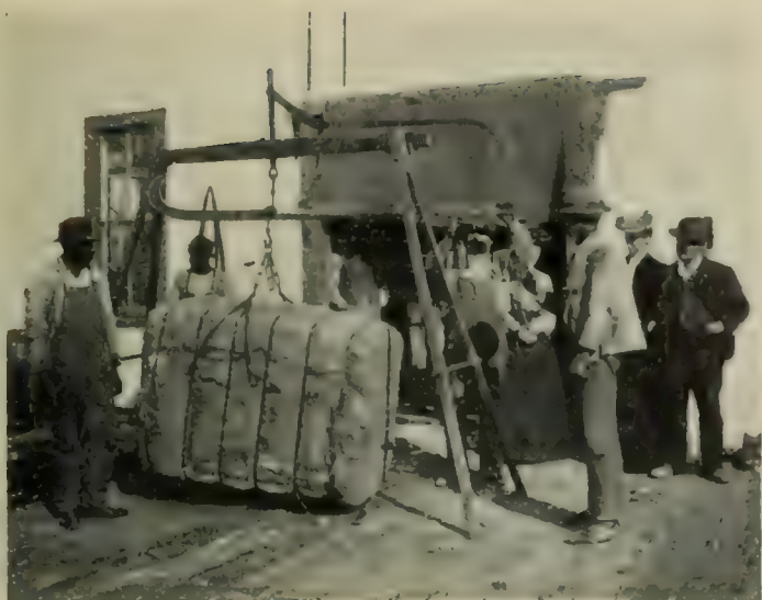
Photographed by George Stark AS SOON AS A BALE IS GINNED IT IS WEIGHED, NUMBERED, AND MARKED WITH THE OWNER'S INITIALS
