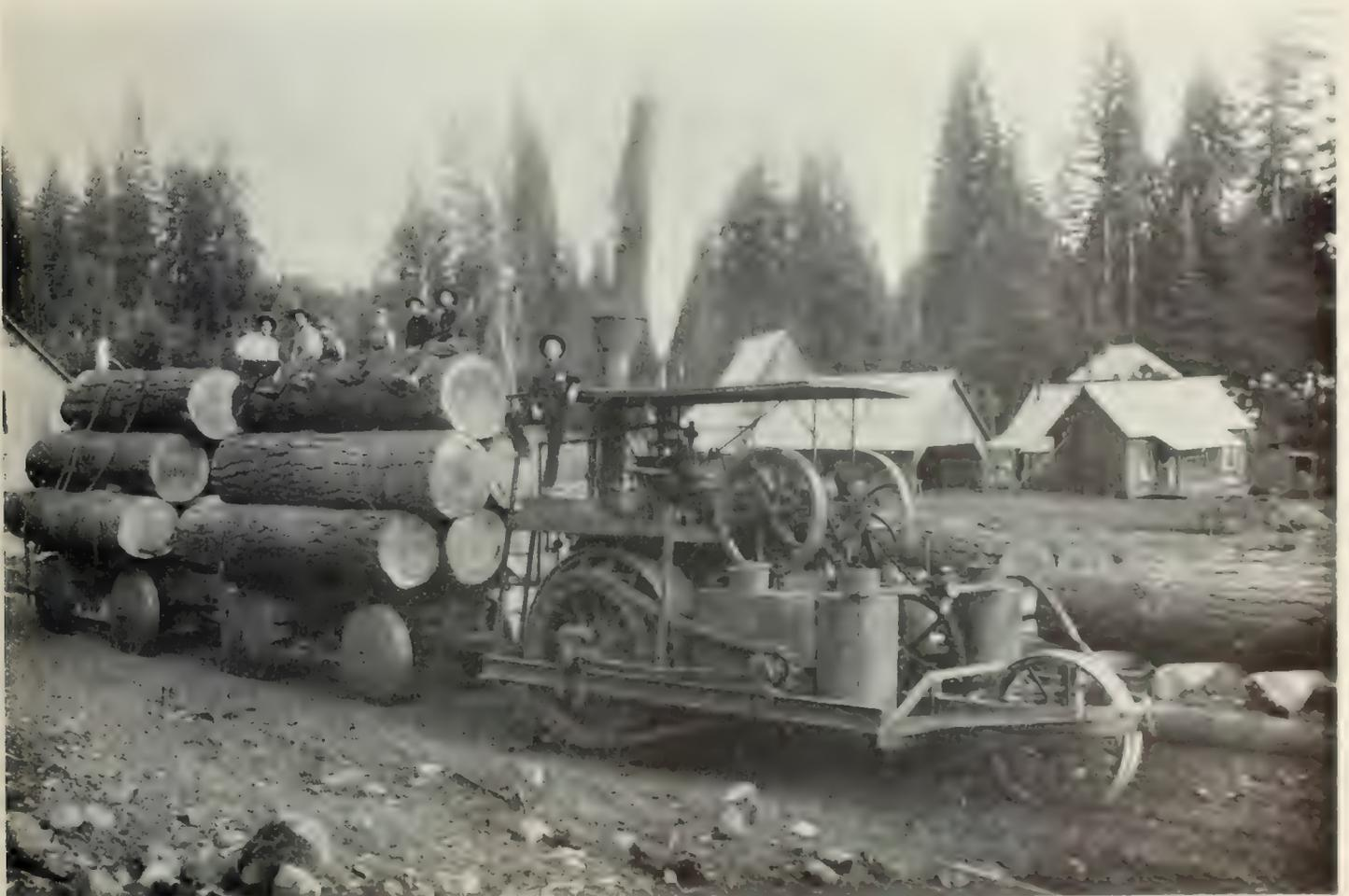
AN AUTOMOBILE ENGINE HAULING 14,000 FEET OF PINE LOGS IN SHASTA COUNTY, CALIFORNIA
