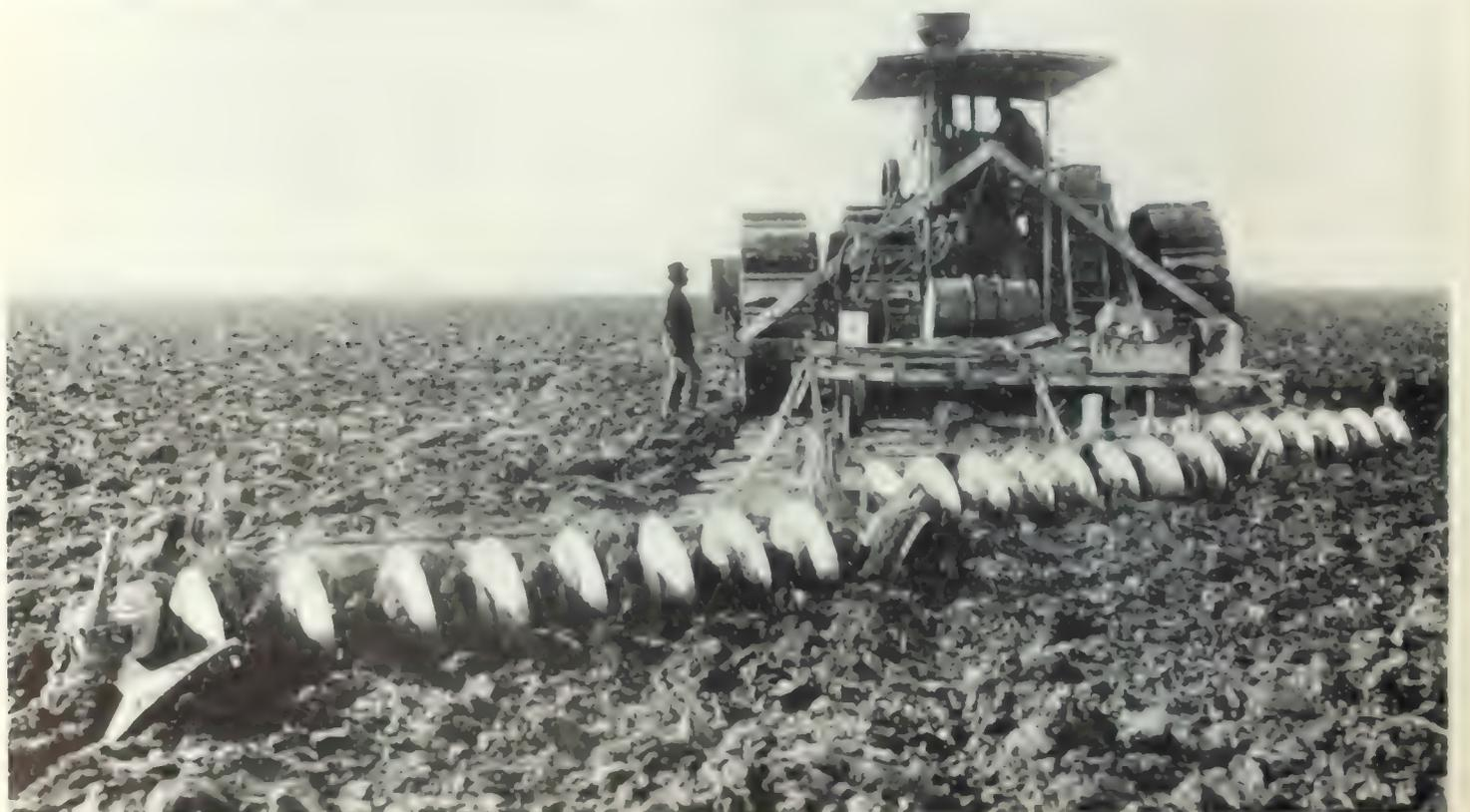
A 6-HORSEPOWER ENGINE PULLING 21 FEET OF DISC HARROW AND AVERAGING SEVENTY ACRES A DAY
