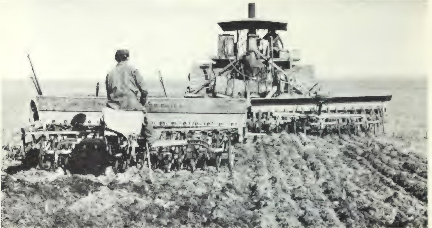
A 60-HORSEPOWER ENGINE PULLING 21 FEET OF PLOWS AND DRILLS, PLOWING SIX INCHES DEEP AND SEEDING AT THE SAME TIME
