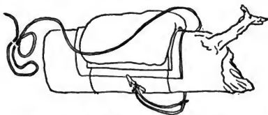
Fig. 304.—The first throw for squaw hitch.
