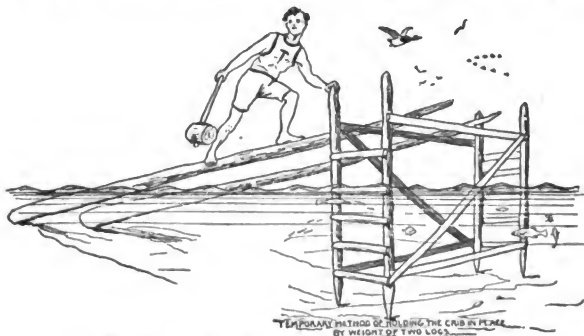
Fig. 163.—The balance logs prevent the crib from upsetting.
