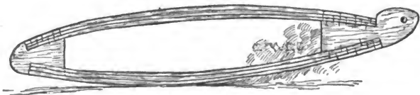
Fig. 483.—A reinforced runner.
