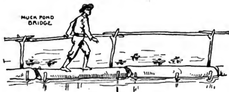
Fig. 162.—A simple and effective bridge for dead water.
