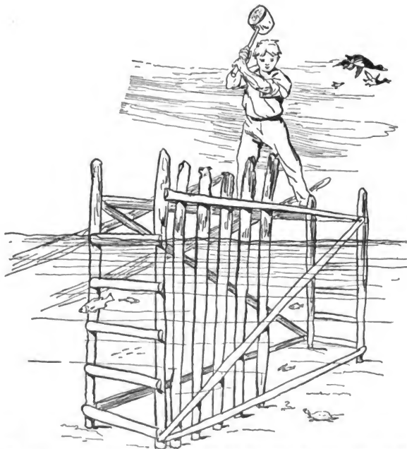
Fig. 164.—Driving the piles for side of crib. Where the winters are severe the front piles should be omitted.
