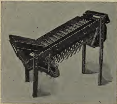
Fig. 29. A potato-sorter (courtesy of Aspinwall Canadian Machinery Company).
