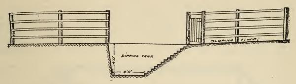
Fig. 48.—Cross section of Dipping Tank and Pens.
