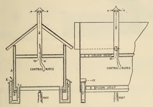
Fig. 57.—The Rutherford System of Ventilation.
