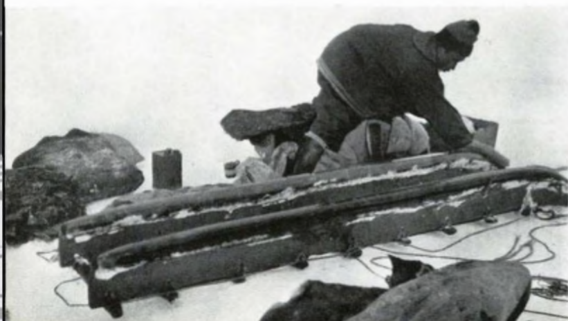
Icing sled runners with a piece of bearskin, Coronation Gulf. Right: The mud shodding is knocked off when spring comes to James Bay. Photos by R. H. G. Bonnycastle and J. W. Anderson.
