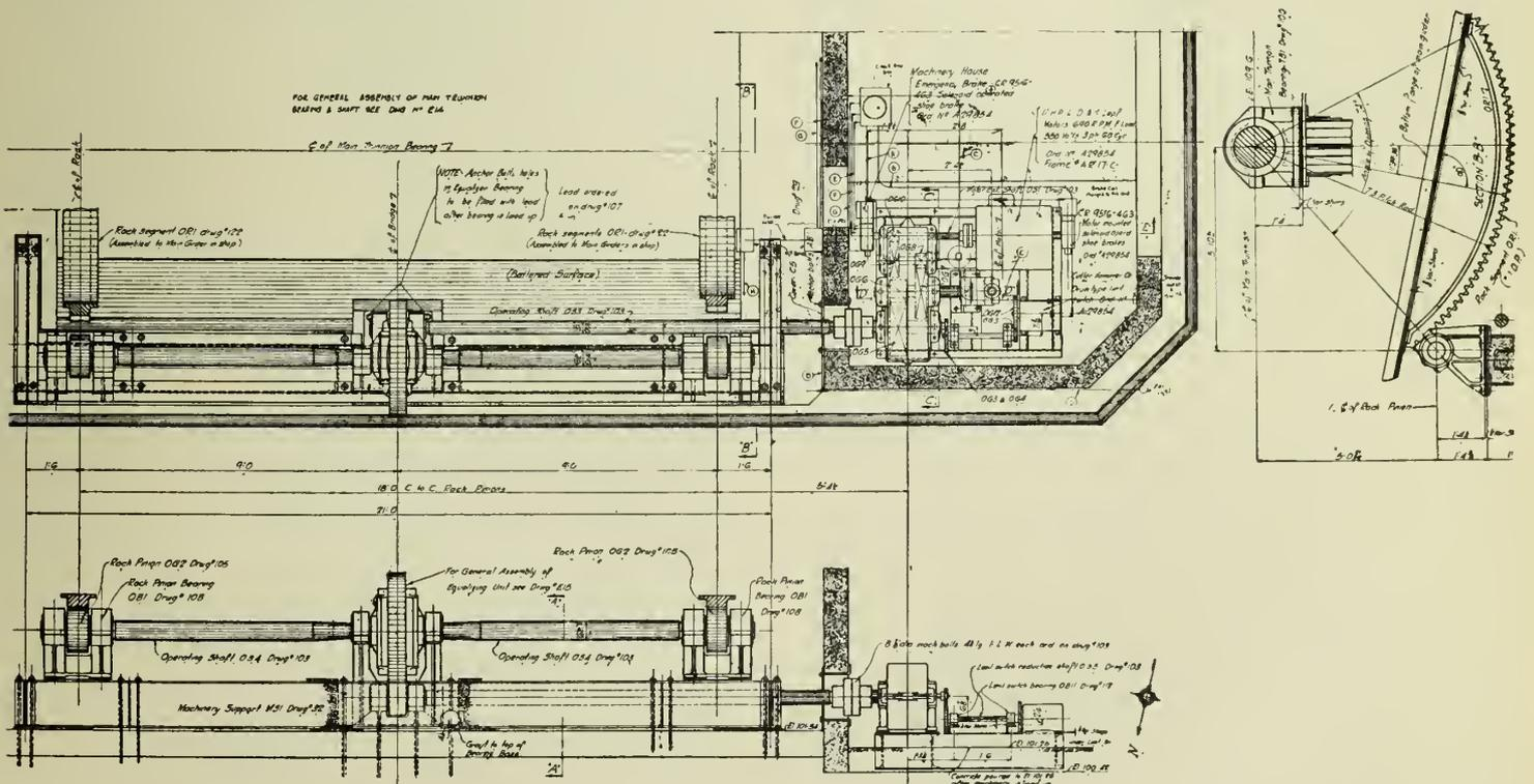
Fig. 9—Operating Machinery at Gaspé.
