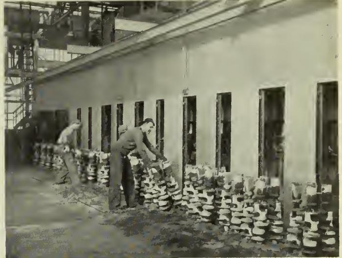
Fig. 4—Assemblies of Crankshafts Before Separation.
