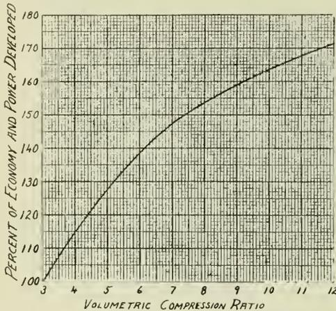
Fig. 6—Effect of Compression Ratio on Operation.
