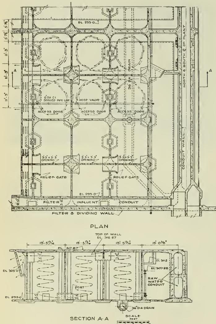
Fig. 12—Mixing Chambers.
