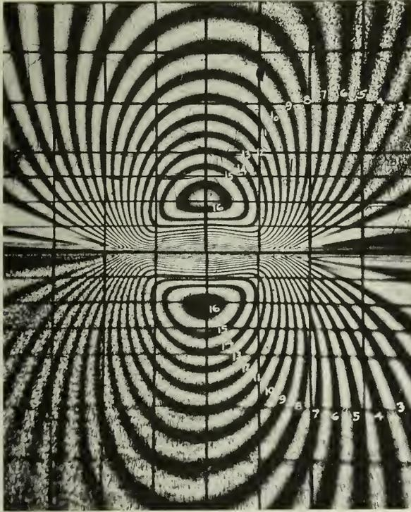
Fig. 9—Stress Distribution in Gear Teeth at Contact Points.
