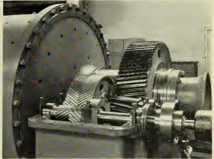
Fig. 7—Drive Gears for a 6-foot by 5-foot Ball Mill.
