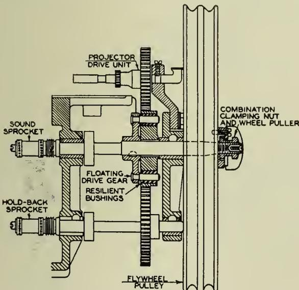
Fig. 8—Cross Section of Film Reproducer Mechanism.
