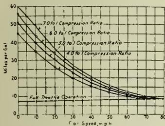
Fig. 10 Effect of Compression Ratio on Operation.
