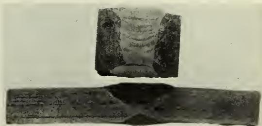
Fig. 1—The effect of Segregation or Lamination in Plate on the Deposited Weld Metal.
