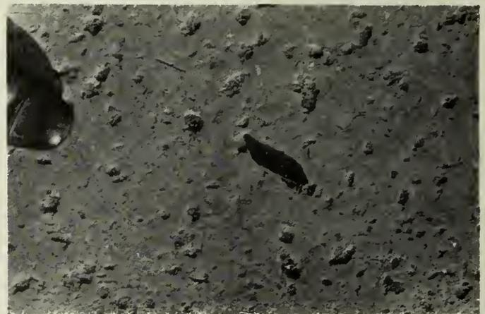
Fig. 7—Fragments of Wood and Bark in Concrete.
