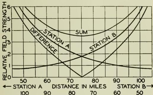
Fig. 4—Field from Two Synchronized Stations of Equal Power.
