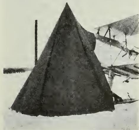
Fig. 3—The Nose Tent. A Wigwam shaped unit supported on the Tip of one Blade of the Airscrew and Laced around the Body of the Aircraft.
