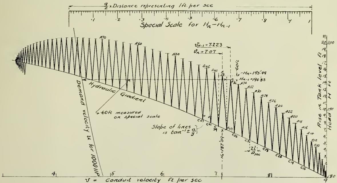
Fig. 11—Simple Surge Tank 12 ft. dia. at the end of 3,400 ft. of 48 in. pipe.
