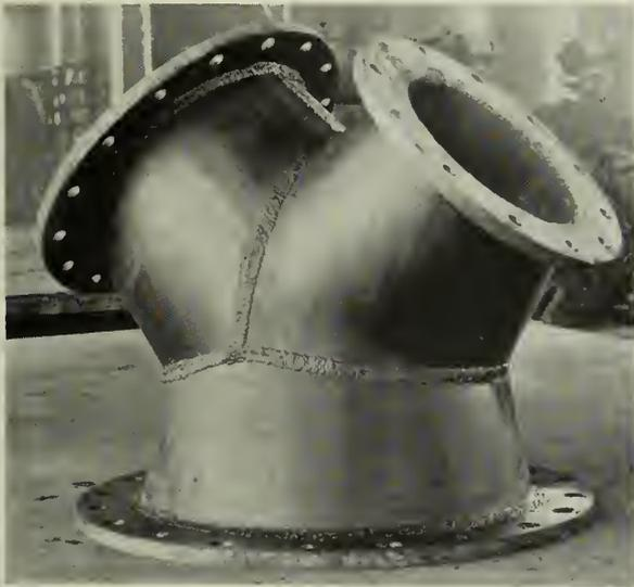
Fig. 10—Welded Pipe Wye, 24 by 16 by 12 inches.
