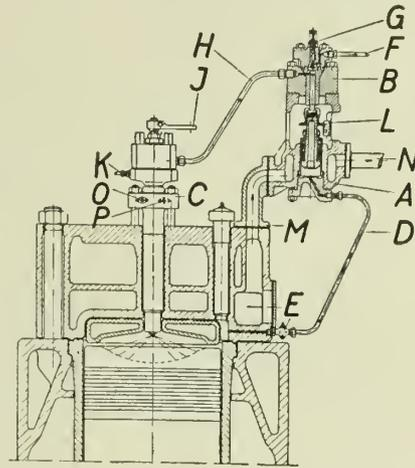
Fig. 2—Section through the Cylinder Head.
