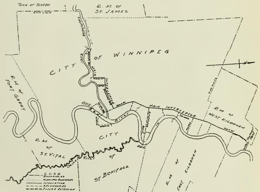
Fig. 3—Proposed Sewerage System for Greater Winnipeg Sanitary District.
