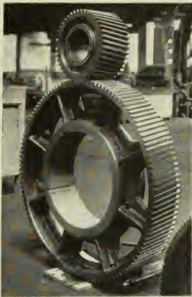
Fig. 4—Single Helical Ring Gear for Suction Roll Drive.
