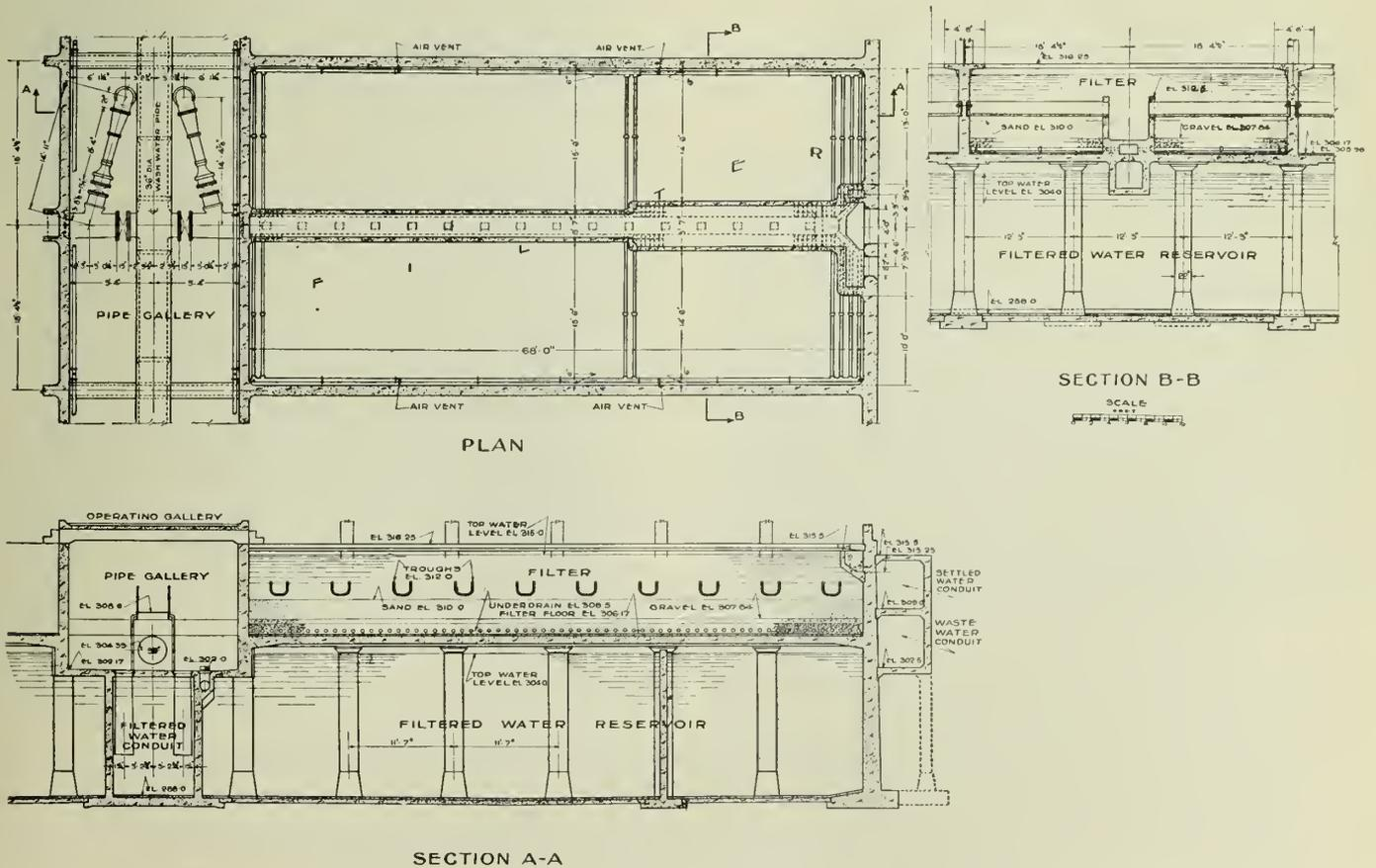
Fig. 10--Typical Filter, Victoria Park Water Purification Plant.
