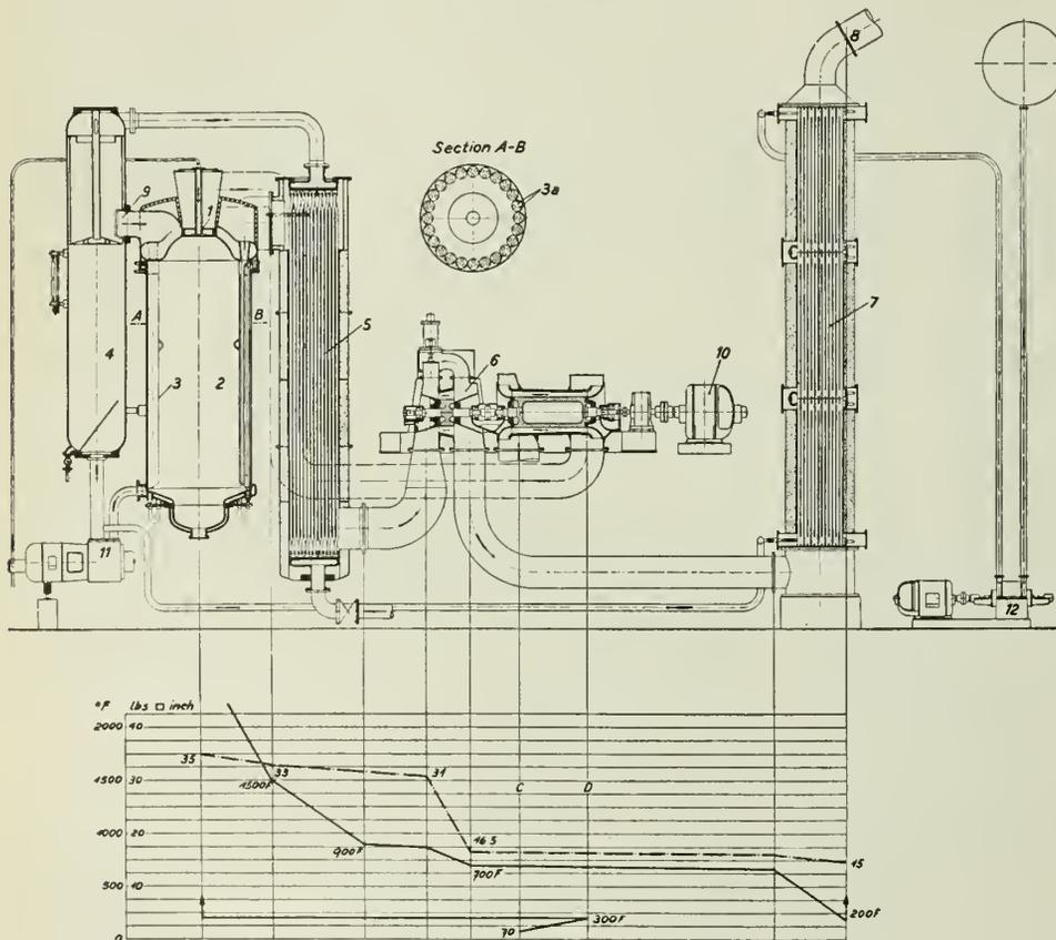
Fig. 1—Diagram of Velox Steam Generator showing Temperatures and Pressures in Various Parts of the Apparatus.
