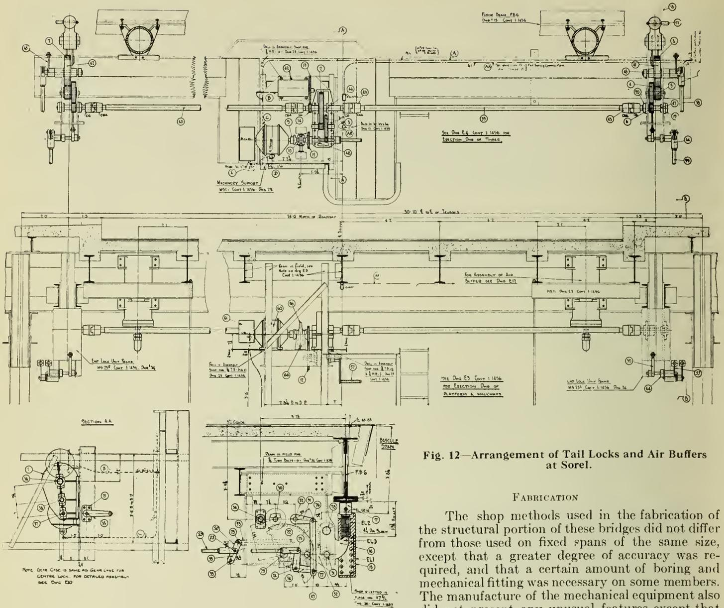
Fig. 12—Arrangement of Tail Locks and Air Buffers at Sorel.
