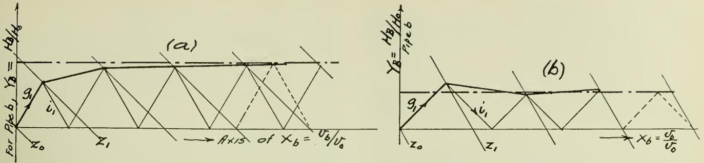
Fig. 20—Water Hammer at Surge Tank for Straight Line Gate Closure.
