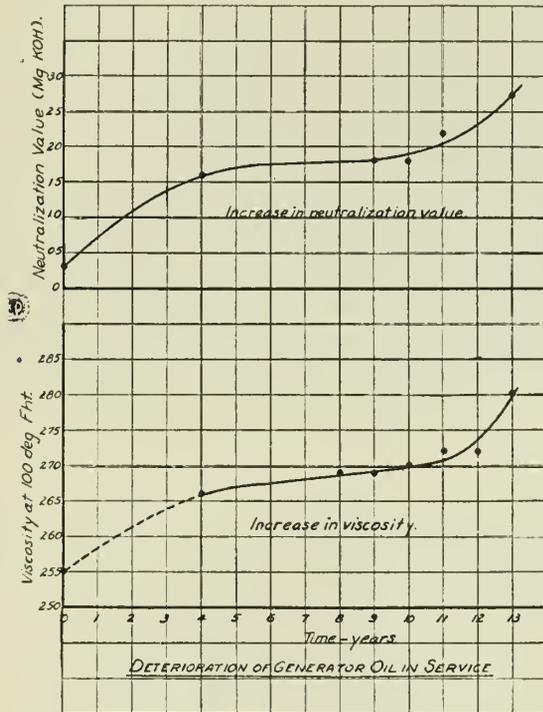
Fig. 4—Deterioration of Oils in Service.
