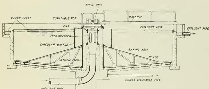
Fig. 4b—Dorr Siphon Feed and Central Drive Clarifier.\*
