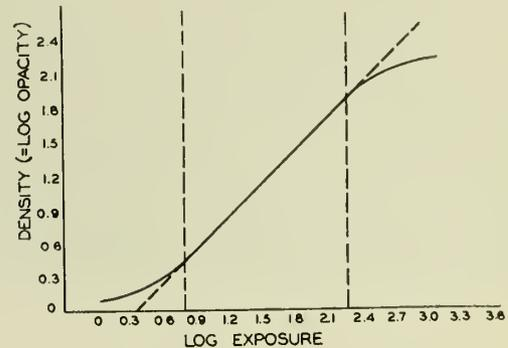
Fig. 13—Exposure-Density Curve for Typical Emulsion.
