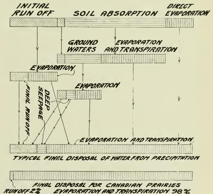
Fig. 2—Final Disposal of Water from Precipitation.
