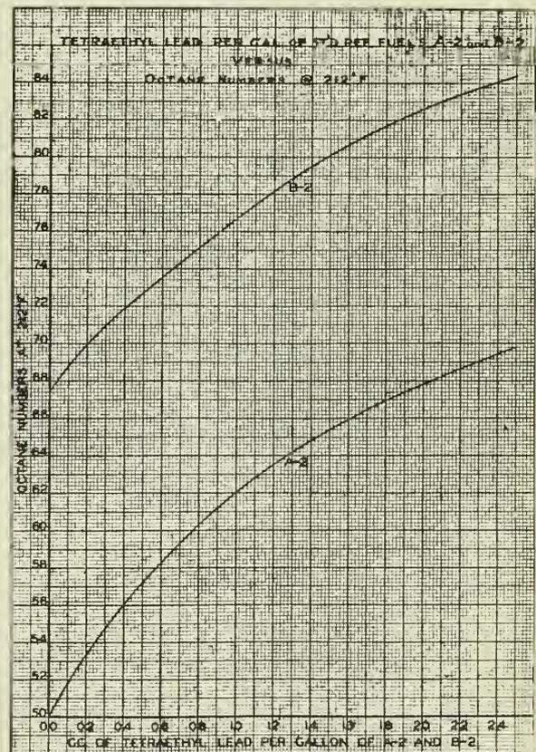
Fig. 15—Reference Fuel Calibration Curves.
