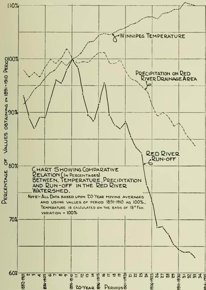
Fig. 5—Relation Between Temperature Precipitation and Run-Off in the Red River Watershed.
