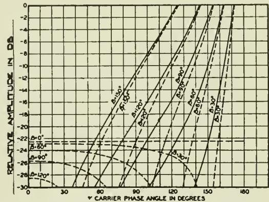
Fig. 5—C.-F. Broadcasting Detection of two Modulated Waves. Second Harmonic Output for Waves of same Amplitude and Frequency Modulated 30 per cent by same Frequency.
