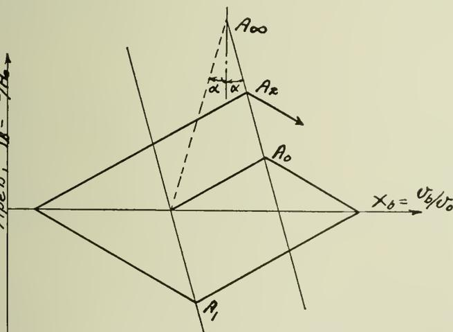
Fig. 21—Water Hammer Effect at Surge Tank due to Gate Swinging Continually, Each Swing Taking  $\frac{2l_b}{a_b}$  sec.
