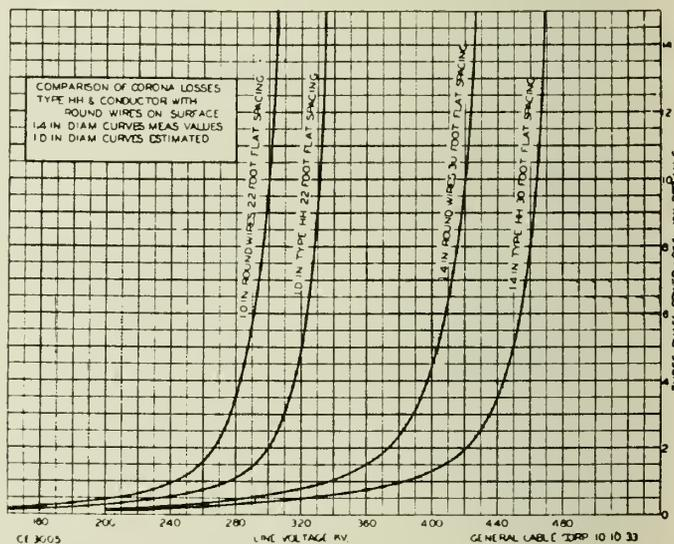
Fig. 4—Comparison of Corona Losses.
