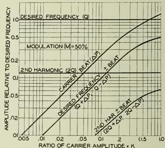
Fig. 2—Detection of two modulated Waves of Frequency-Difference  $\Delta P$ , each modulation 50 per cent in Phase, by Frequency  $Q$ . Curves show relative Amplitude of Audio-Frequency Components in Output of Receiving (Square-Law) Detector.
