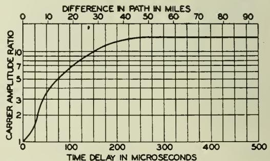
Fig. 7—Detection of two Modulated Waves of same Carrier Frequency, of Relative Phase 180 Degrees modulated by same Programme. Curve shows Time-Delay (or Difference in Lengths of Path to Receivers) versus Carrier Amplitude Ratio at which Distortion is just Perceptible.
