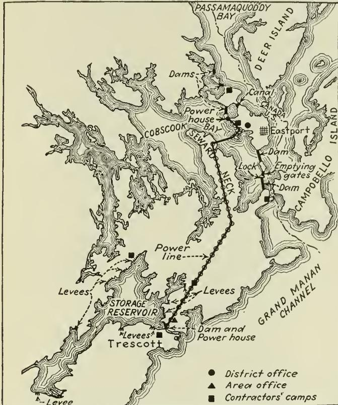
The Tidal Project Originally Designed to Include Passamaquoddy Bay is now confined to the much smaller Cobscook Bay supplemented by a Pumped-Storage Reservoir.
