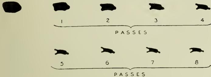
Fig. 5—Steps in Drawing Down Segments.
