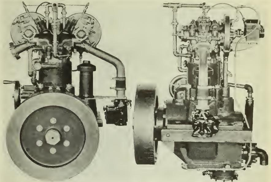
Fig. 12—N.A.C.A. Universal Engine for Testing Fuels.
