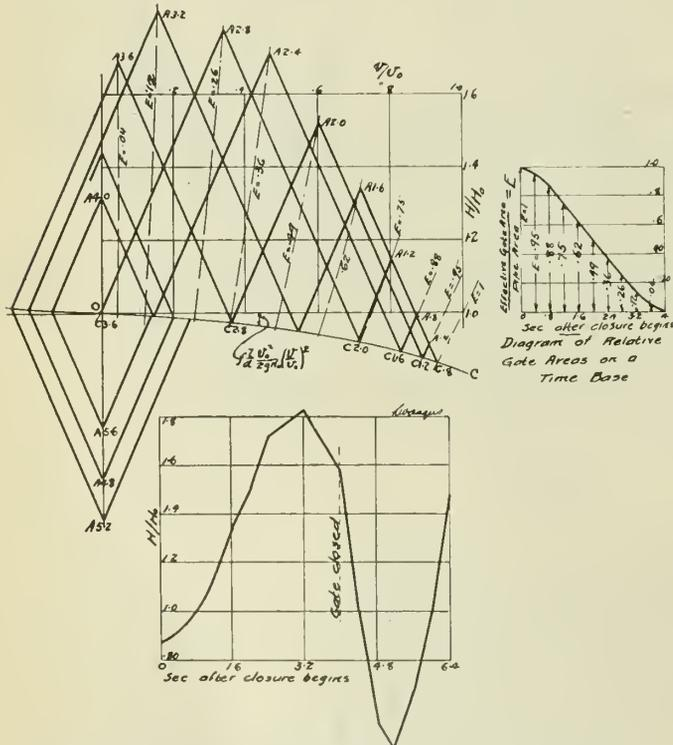
Fig. 13—Gate Closure according to Curve Shown in 4 sec.  $2l/a = 1.6$  sec.  $\rho = 1.125$  Pipe Friction allowed for (see Fig. 6).
