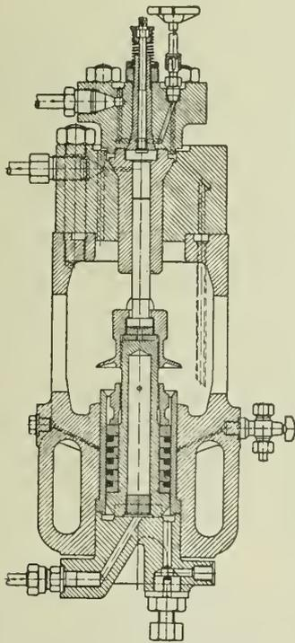
Fig. 1—Section through the Injection Pump—Archaouloff-Krupp Diesel Engine.
