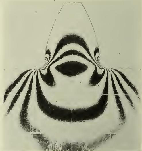
Fig. 7—Stress Concentrations at Fillets.
