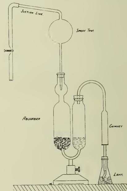
Fig. 2—A.S.T.M. Sulphur Lamp Apparatus.
