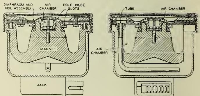
Fig. 12—Cross Section of Microphone.
