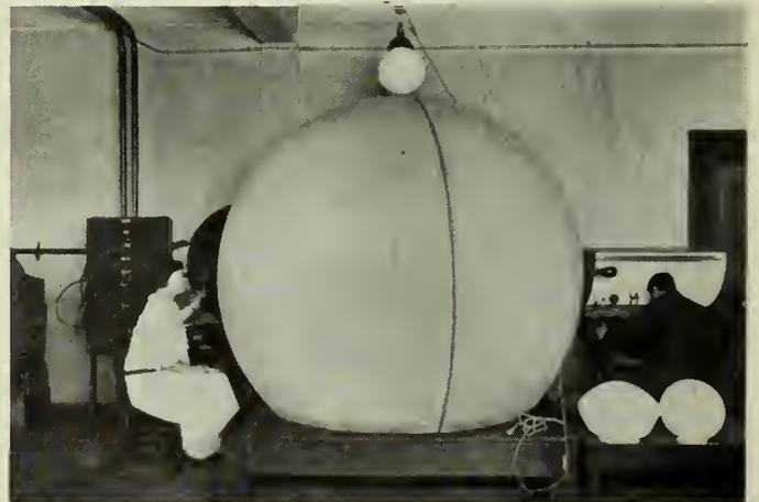
Fig. 8—Integrating Sphere Photometer.
