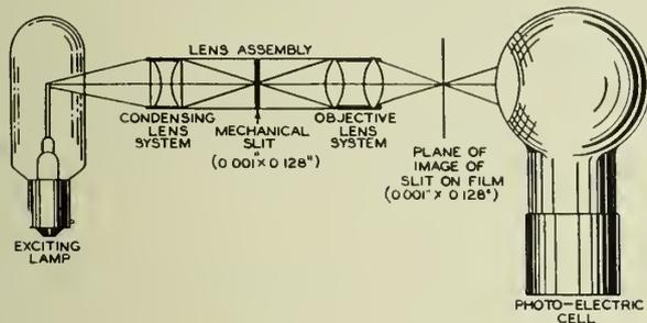
Fig. 4—Reproducer Optical System.
