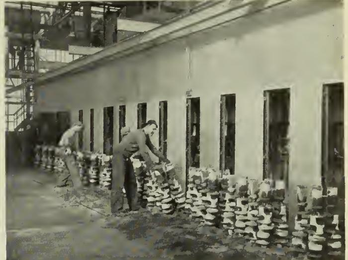
Fig. 4—Assemblies of Crankshafts Before Separation.
