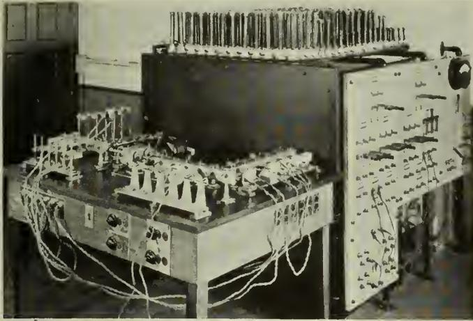
Fig. 2—Machine for Making Endurance Tests on Sockets, Switches, etc.
