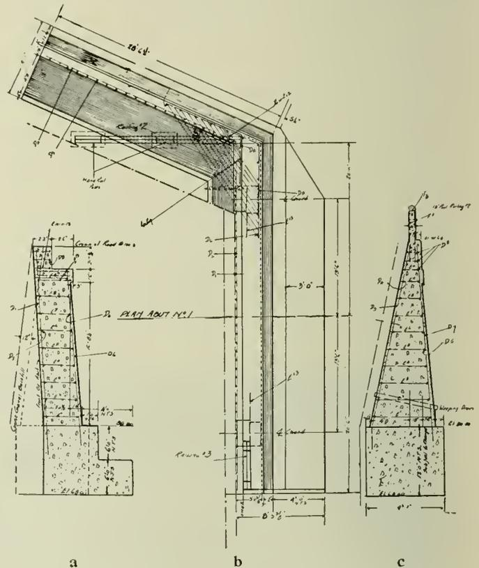
Fig. 4—Detail of Abutment No. 1.
