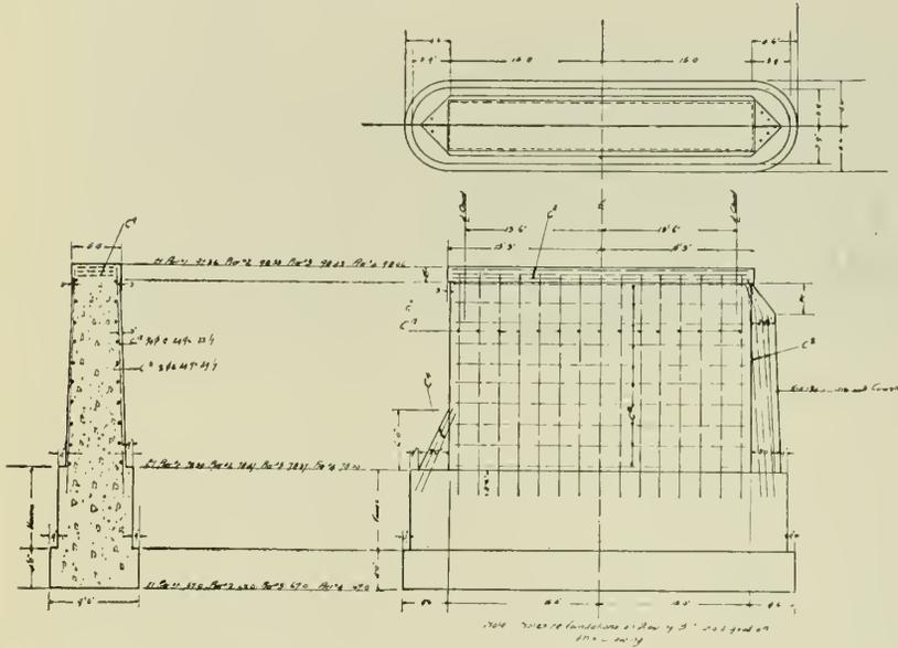
Fig. 3—Detail of Typical Pier.
