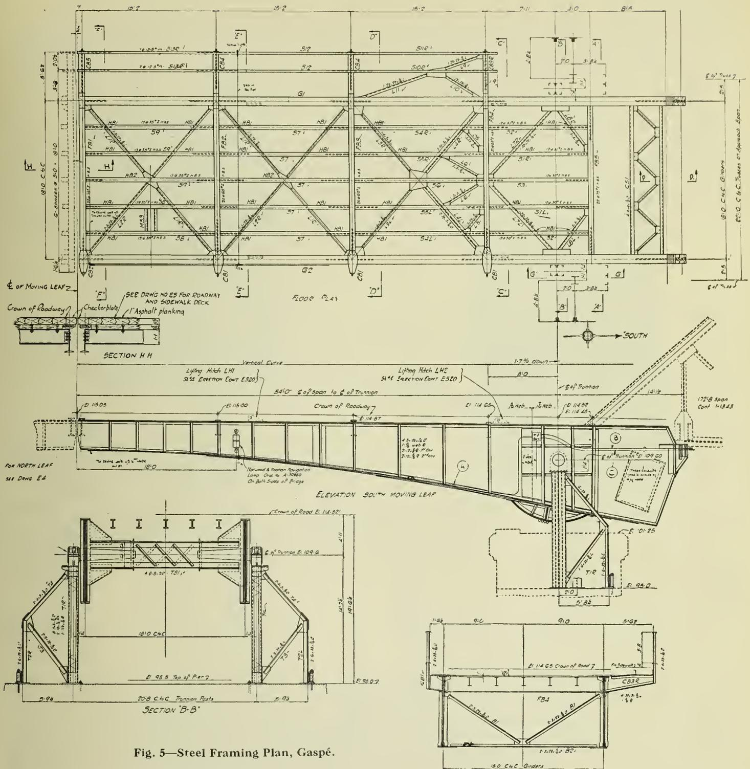
Fig. 5—Steel Framing Plan, Gaspé.
