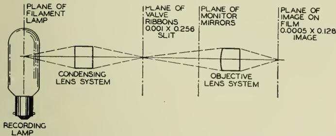
Fig. 3—Recorder Optical System.
