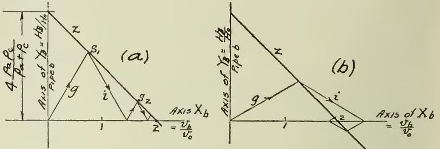
Fig. 19—Water Hammer at Surge Tank for Instantaneous Gate Closure.
