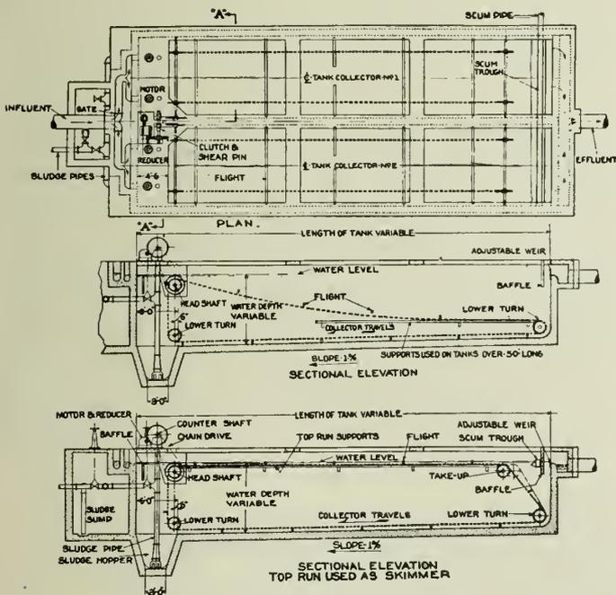
Fig. 5—Arrangement of Link-Belt Straight Line Sludge Collectors.\*
