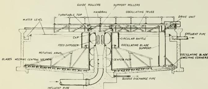
Fig. 4a—Dorr Siphon Feed and Traction Drive Clarifier.\*
