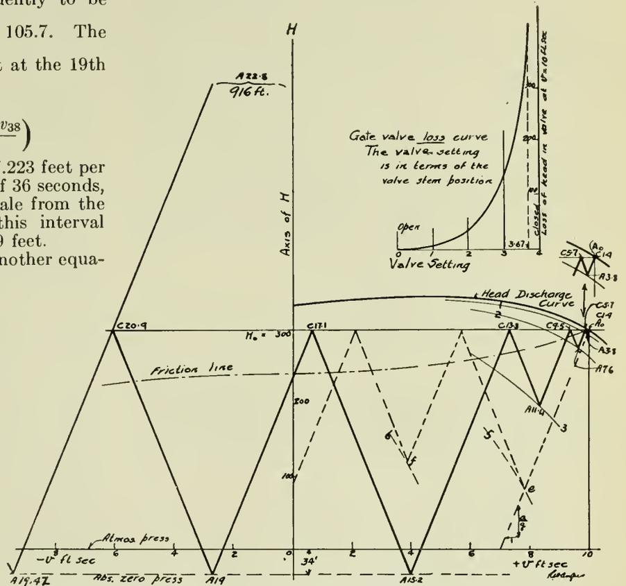
Fig. 12—Discharge Valve Closed with Pump Running up to Speed.
