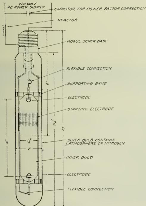
Fig. 2—Schematic Diagram, 400-Watt High Intensity Mercury-Vapour Lamp.
