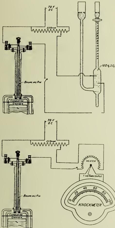
Fig. 14—Apparatus for Measurement of Detonation.
