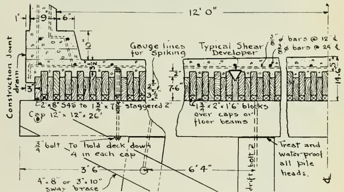
Fig. 5—Timber Substructure and Stringer System Supporting Concrete Deck.
