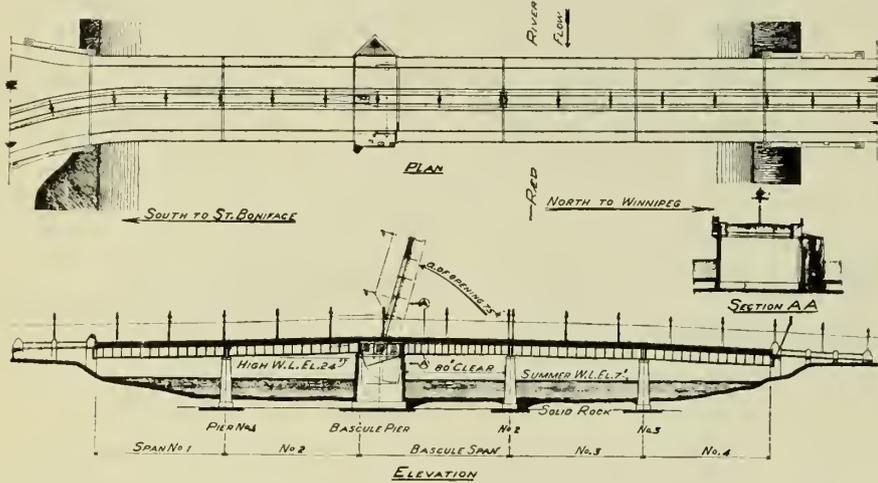
Fig. 1—Plan and Elevation of Norwood Street Bridge.
