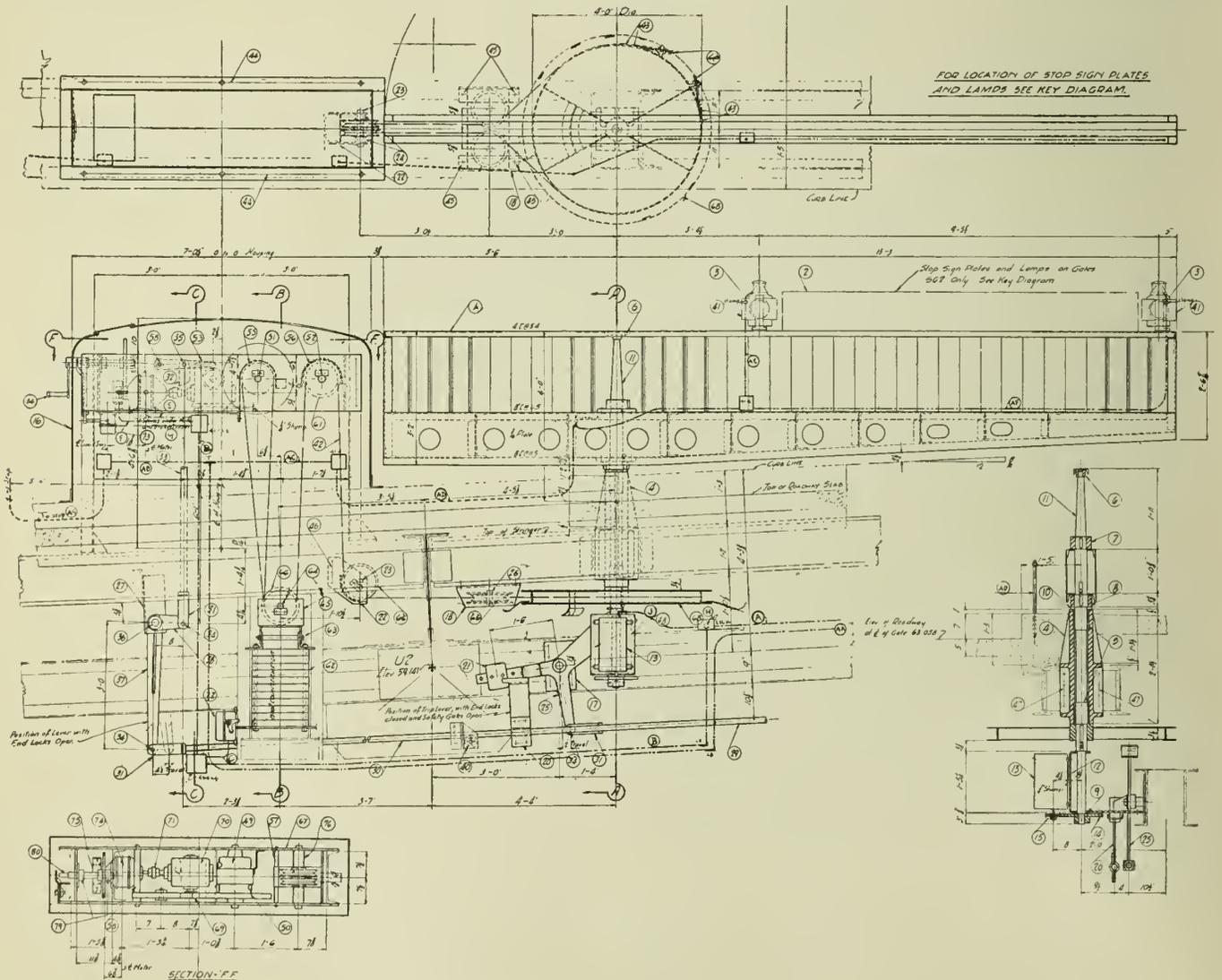
Fig. 14—Arrangement of Highway Gates at Sorel.
