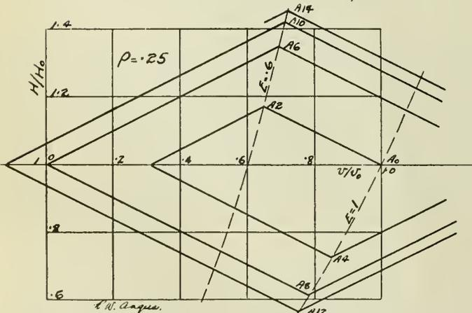
Fig. 10—Resonance Effect due to Continual Swinging of Gate between part and full opening, each Swing taking  $2l/a$  sec.
