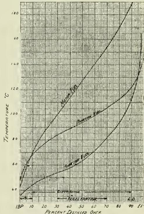
Fig. 5—Distillation Curves.
