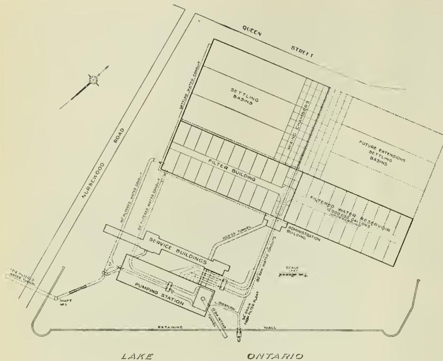
Fig. 9—Layout, Victoria Park Water Purification Plant.
