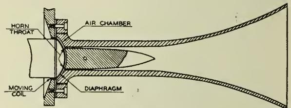
Fig. 11—Cross Section of High Frequency Unit.
