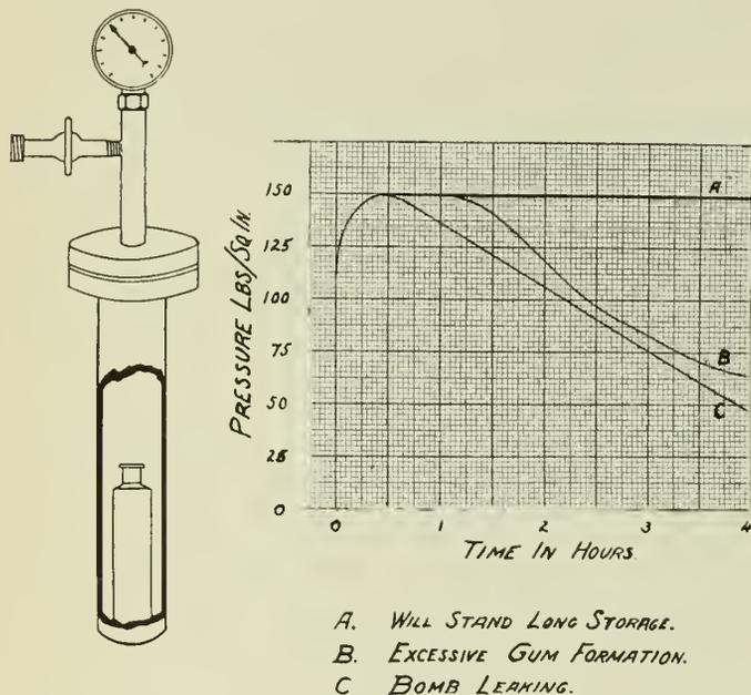
Fig. 1—Oxygen Bomb for Accelerated Ageing Test.
