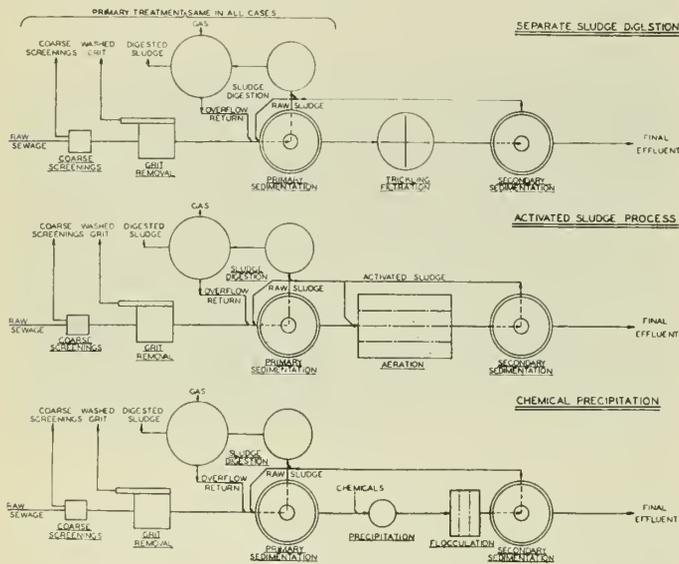
Fig. 7—Typical Sewage Treatment Flow Sheets.
