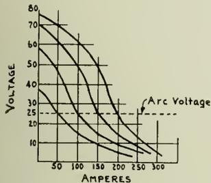
Intercept on Y axis = Open Circuit Voltage.
