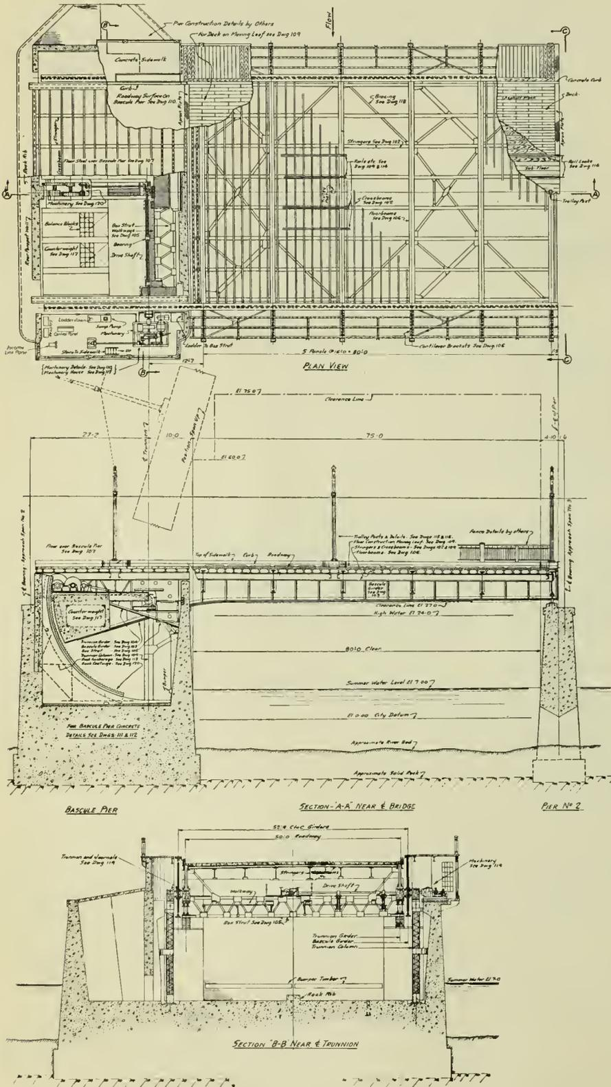
Fig. 4—Steel Framing Plan, Norwood.
