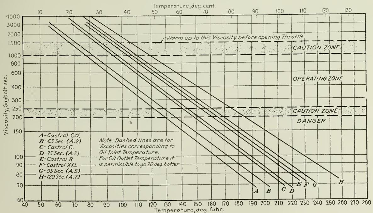
Fig. 6.—Viscosity and temperature for various oils.
