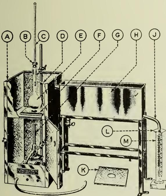
Fig. 4—A.S.T.M. Distillation Apparatus.
