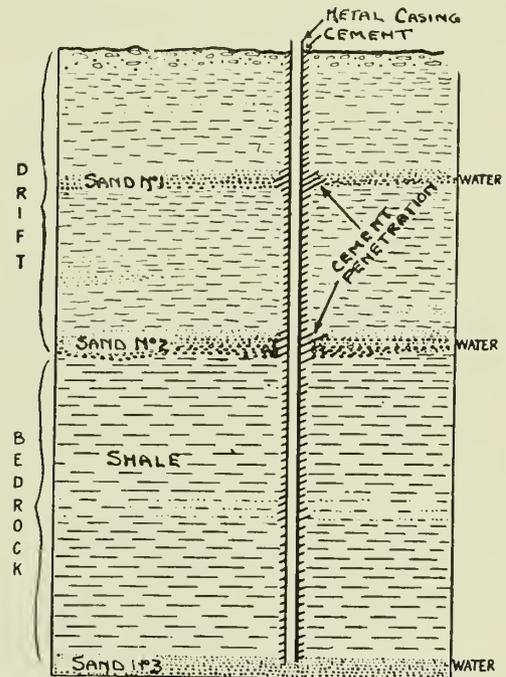
Fig. 2—Section of Drilled Well Showing Cement Protection.
