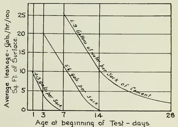
Fig. 5—Permeability of Concrete.
