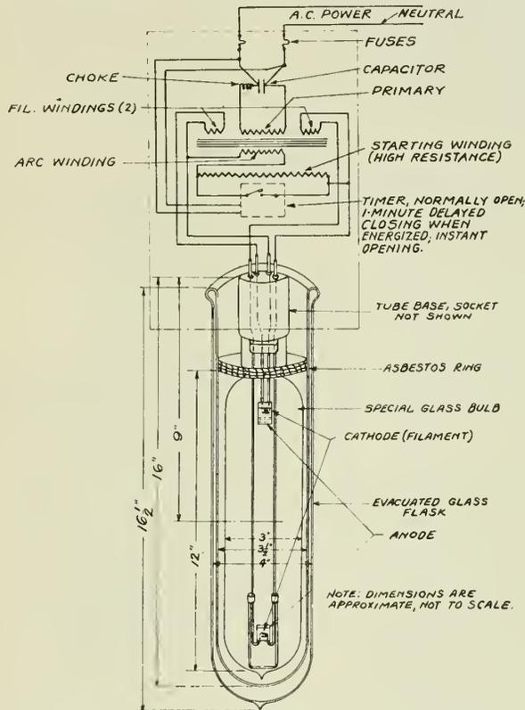
Fig. 1—Schematic Diagram, 10,000 Lumen A.C. Sodium Lamp
