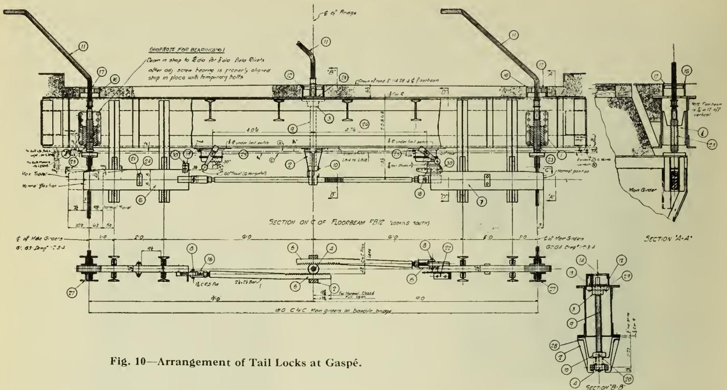
Fig. 10—Arrangement of Tail Locks at Gaspé.
