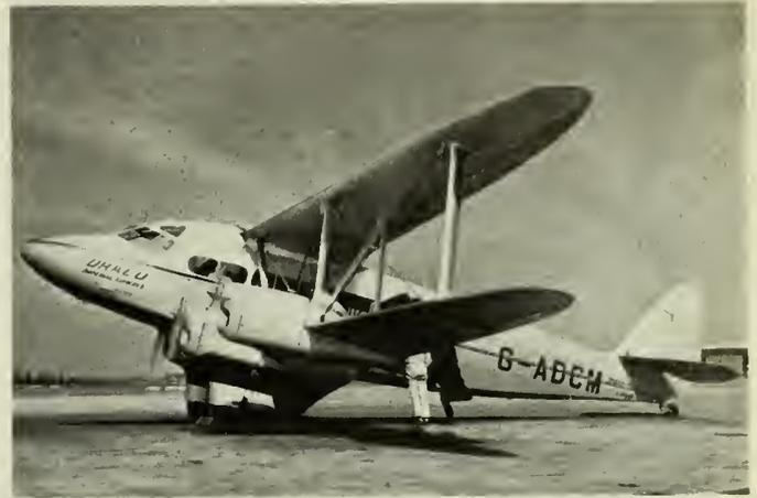
Fig. 5—D.R. Draco used by British and Australian Services. Four 205-h.p. motors. Pay-load 2,480 pounds. Max. Speed 170 m.p.h.
