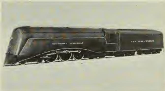
Fig. 9—New York Central Hudson Type Streamlined Steam Locomotive.
