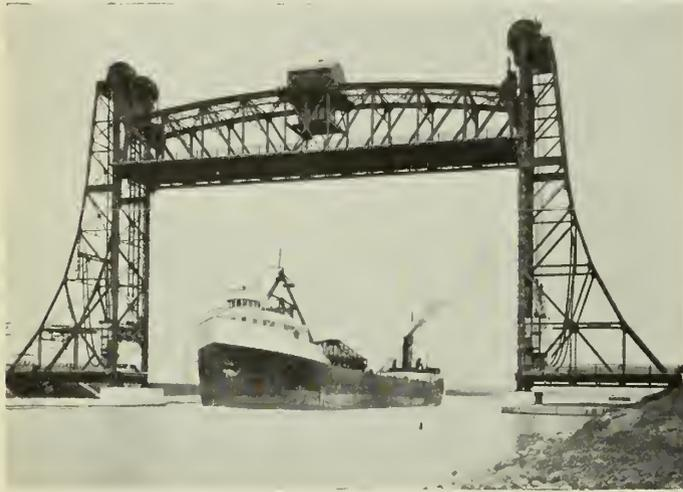
Fig. 6—A Type of Self-Unloading Lake Freighter.
