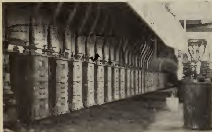
Fig. 6—Completed mould mounted on pouring reel
