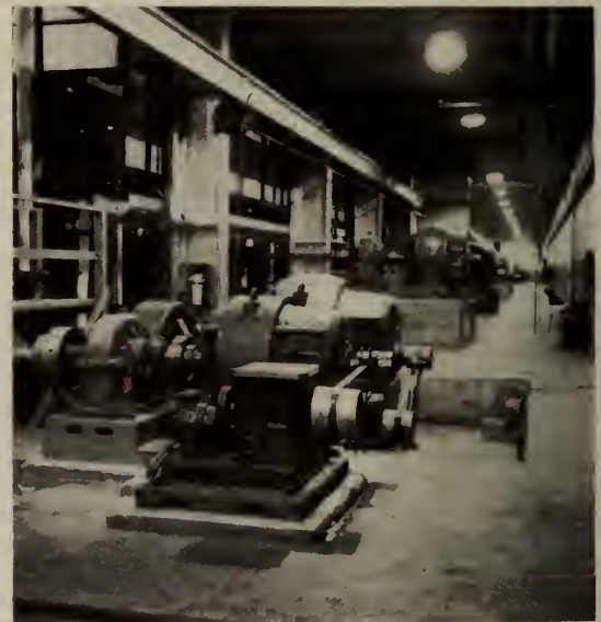
Fig. 11—Paper Machine Drive Motors
