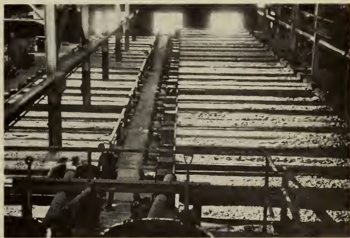
Fig. 6—Flotation cells in concentrator
