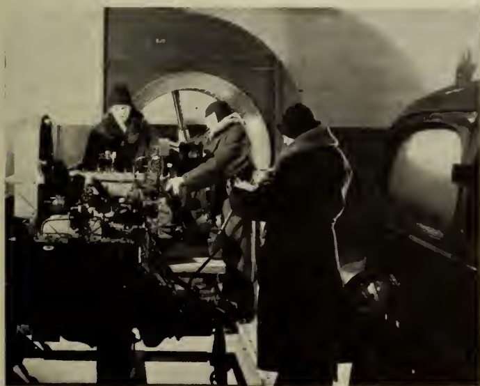
Fig. 2—Starting Tests in a Cold Room
