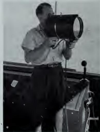
Fig. 1—Light gun used for controlling airport traffic
