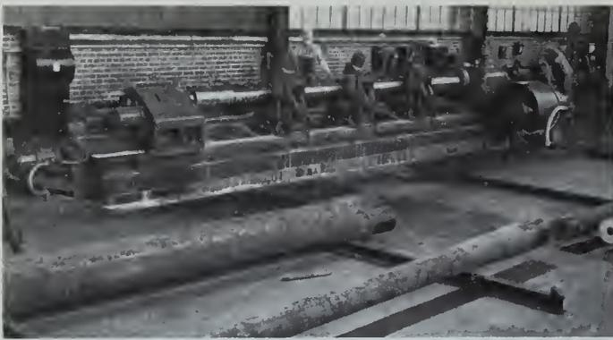
Close up of lathe rough turning gun.
