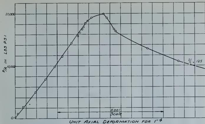
Fig. 18—Average load—axial deformation curve for one-inch round mild steel column.
