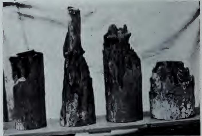
Fig. 4—At left, one of the spruce pile heads uncovered in one of the test holes. At centre, two badly decayed spruce pile heads from the west and south walls. At right, decayed cedar pile head from under the wall of the old building.
