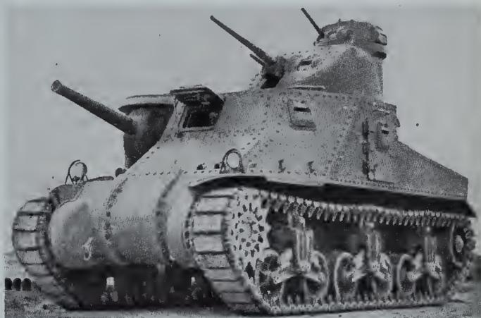
The medium tank M3 mounts a 75mm cannon, a 37mm gun, and two machine guns
