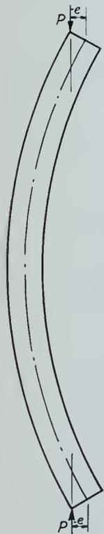
Fig. 23—Loading of flat-ended column after buckling.
