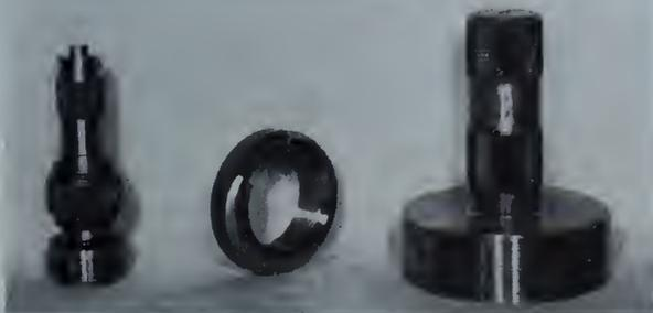
Fig. 3—Male and female screw gauges
