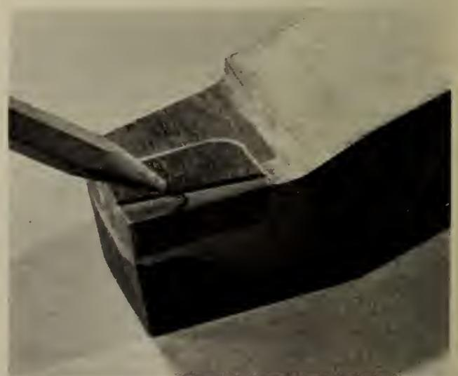
Fig. 2—The ground-in step is the most widely used type of chip breaker.
