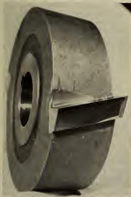
Figs. 1 and 2—Close view of special malleable iron cutters, showing carbide tips which are silver-soldered in place.
