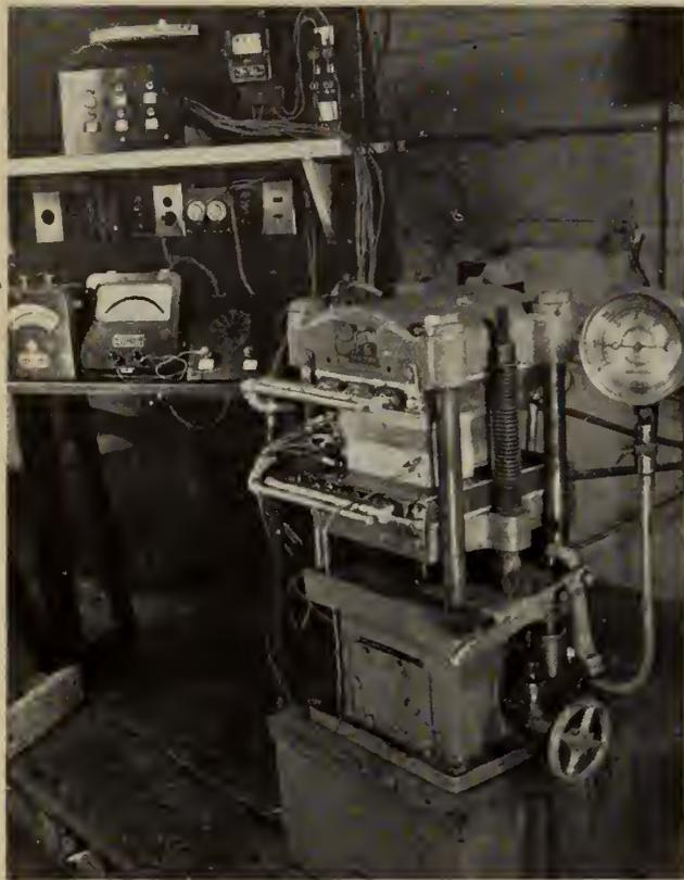
**Fig. 2—Shows multi-ply laminated wood being assembled by the new process in the laboratory. A laboratory hydraulic press with 14 by 14 in. platens is shown, and the arrangement of glue lines in parallel is noted.**
