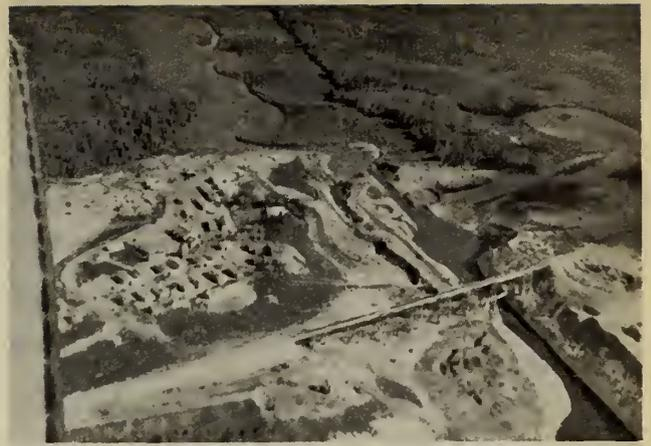
Fig. 8—Aerial view of a portion of the Jackfish river valley showing the C.N.R. bridge, the new channel and the relatively small stream bed of the original Jackfish river.
