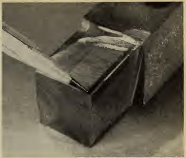
Fig. 3—Ground-in groove type of chip breaker.
