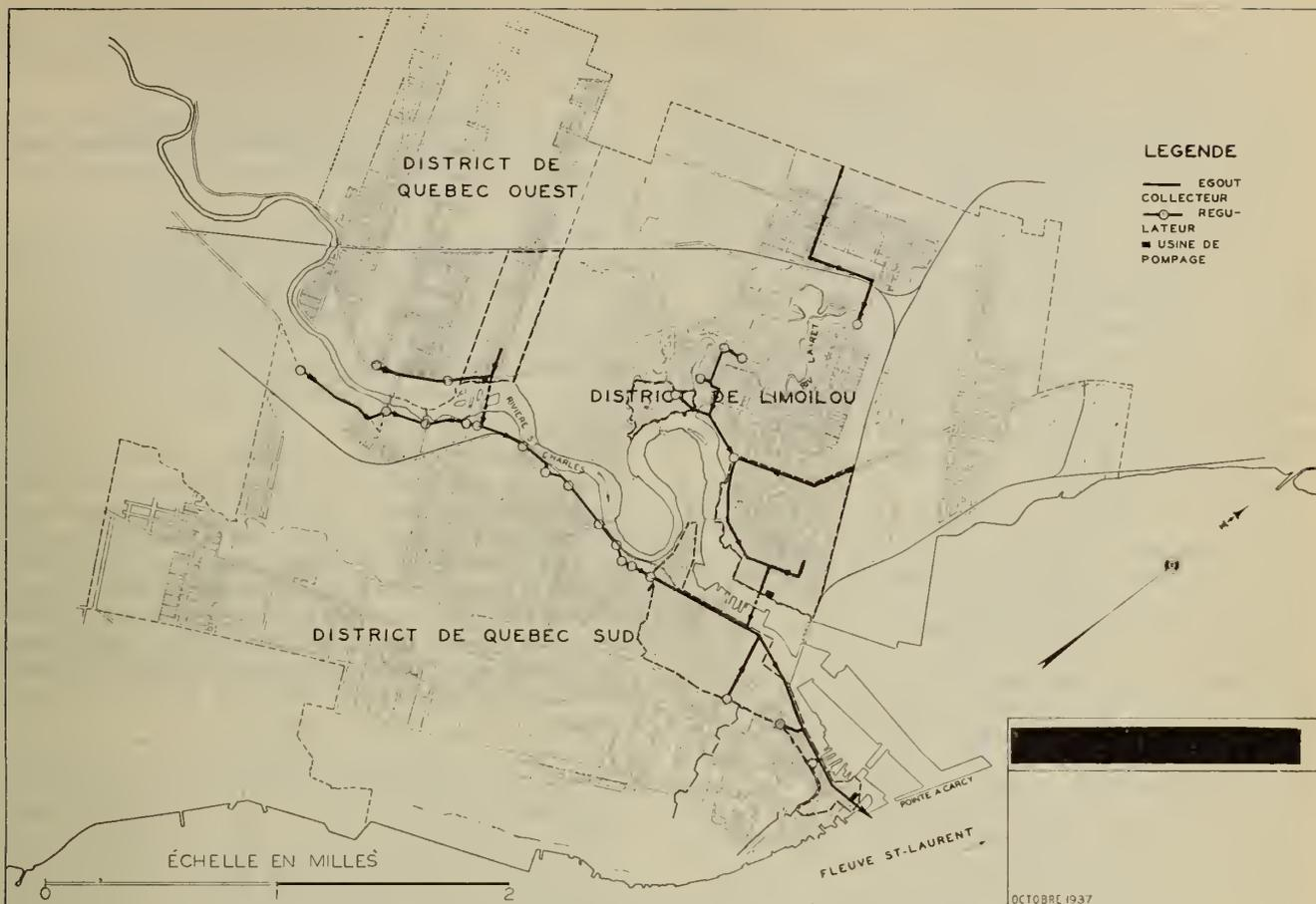
Fig. 3—Plan of city showing proposed intercepting sewers.
