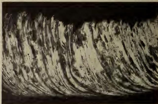
Fig. 2—Photomicrograph of a continuous flow type chip.
