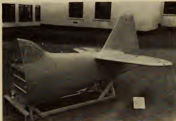
Fig. 5—Moulded plywood rear fuselage for Harvard trainer.
