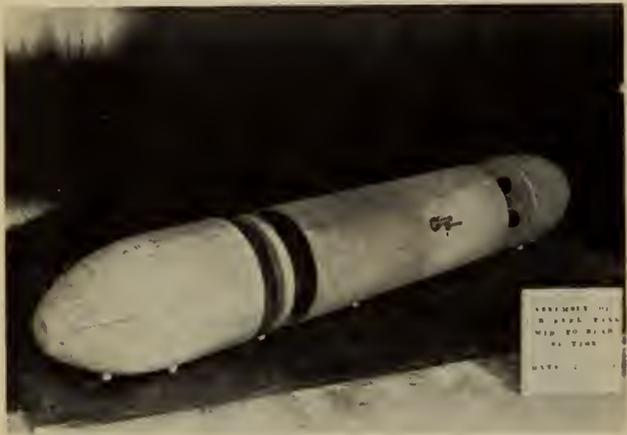
Fig. 13—Assembly of plywood fuel tank.
