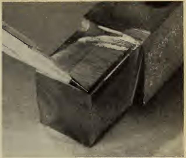
Fig. 3—Ground-in groove type of chip breaker.
