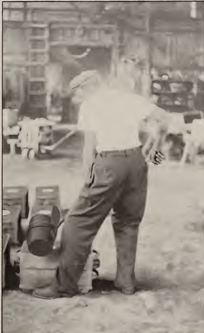
The Wrong Way of Pouring Hot Metal
