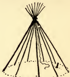
2 nd Set up & bind other six poles
