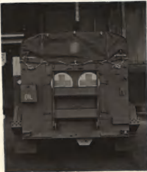
REAR VIEW (STEPS FOLD DOWN FOR LOADING)
