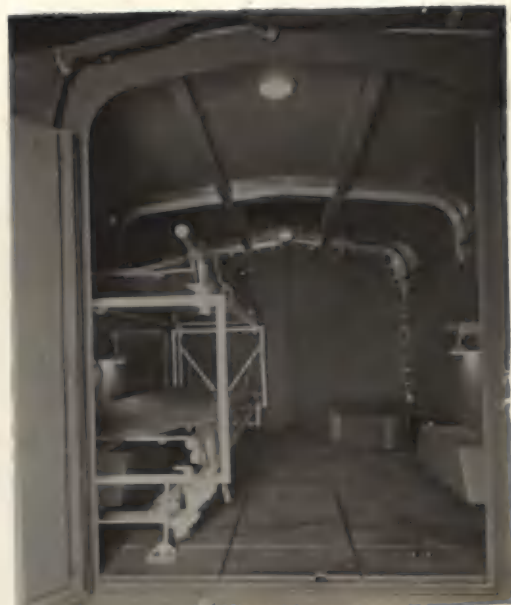
REAR INTERIOR VIEW (DOUBLE BED STRUCTURE MECHANISM SHOWN ON L.H. SIDE - SPECIAL INSTALLATION MADE ON R.H. SIDE MAKING DOUBLE BED MECHANISM OPERABLE)
