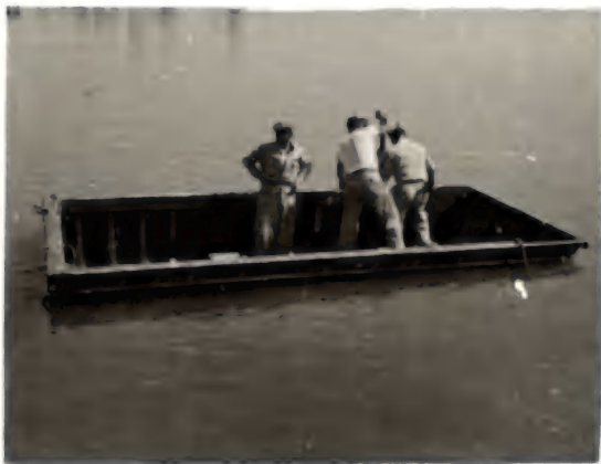
PONTON LOADED WITH 12000# OF PIG LEAD PLUS 3 MEN .
