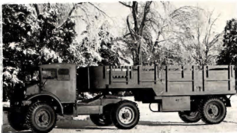
Semi-trailer body - Code 10-G-1, for British Ministry of Supply. Capacity- 6 long tons (13,400 lbs.)
