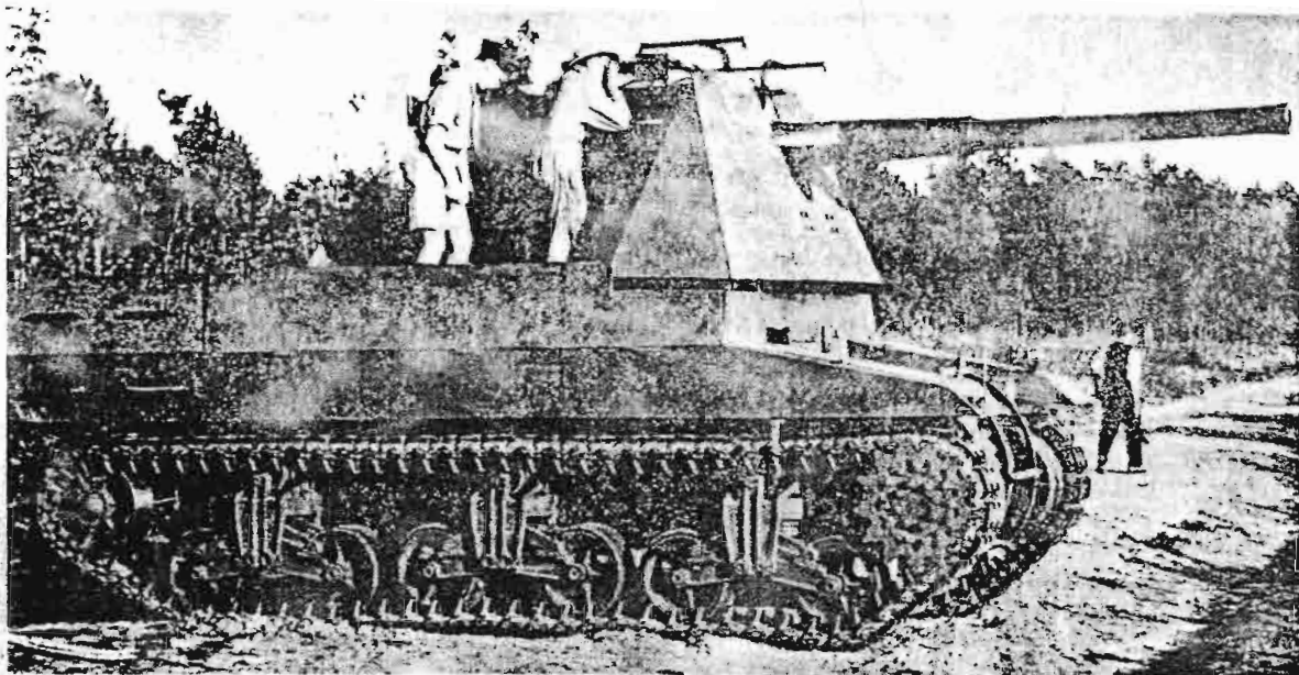
Above and below. The Ram converted experimentally as a SP AA mount for the 3.7-in gun. This project was abandoned at an early stage, 1943. (Canadian Official)
