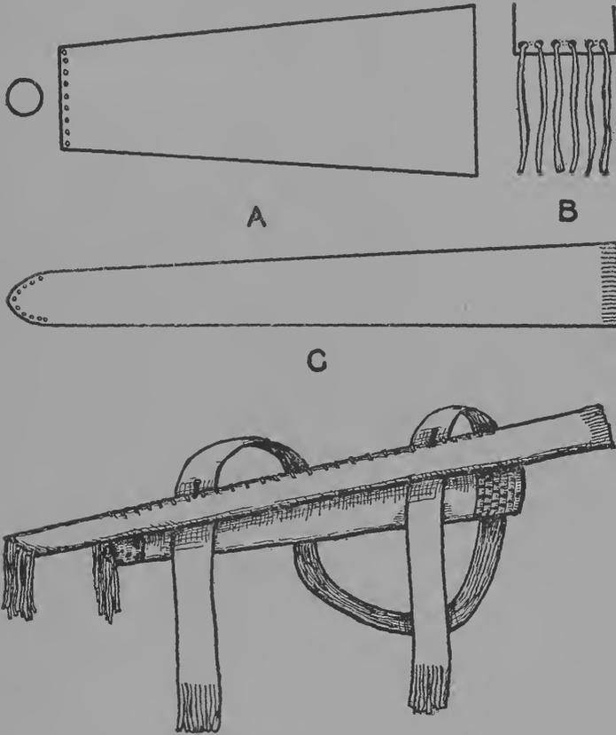
Fig. 92. (A) Quiver Pattern (B) Method of Making Fringe (C) Bow Case Pattern (D) Case and Quiver Complete
