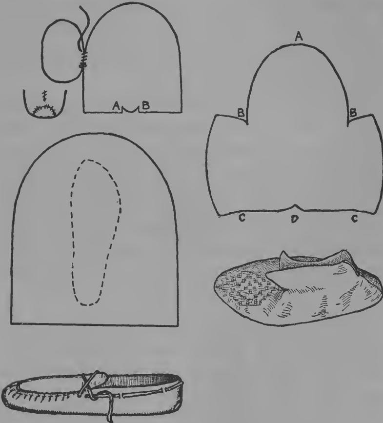
Fig. 49. Woodland Pattern. Fig. 50. Method of Stitching Sole to Tongue
