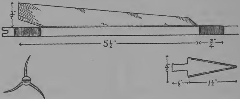
Fig. 88. Method of Feathering Arrow Fig. 89. End View of Arrow
