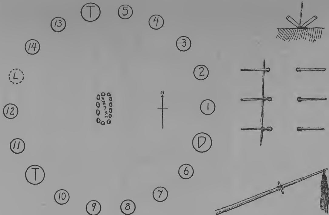
Fig. 71. How the Poles are Put in Place. TTD, Tripod and Door Poles
