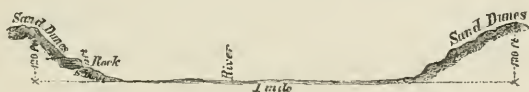
Transverse Section of the Valley of the Qu'appelle at the height of land.
