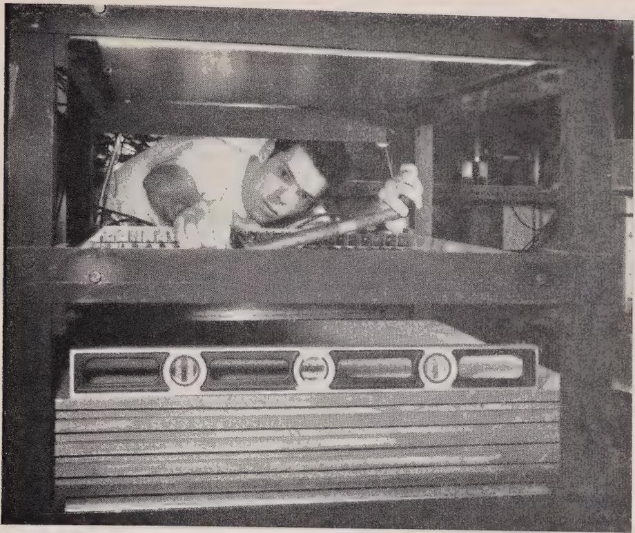
Changing a Geiger-Mueller tube in a "counter-tray". This equipment forms part of a "counter telescope" which monitors cosmic radiation at Resolute Bay, N.W.T.
