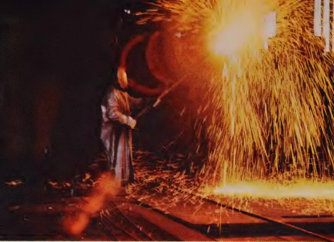
A skilled steelmaker uses an oxygen torch to strip the scale off a forging.
