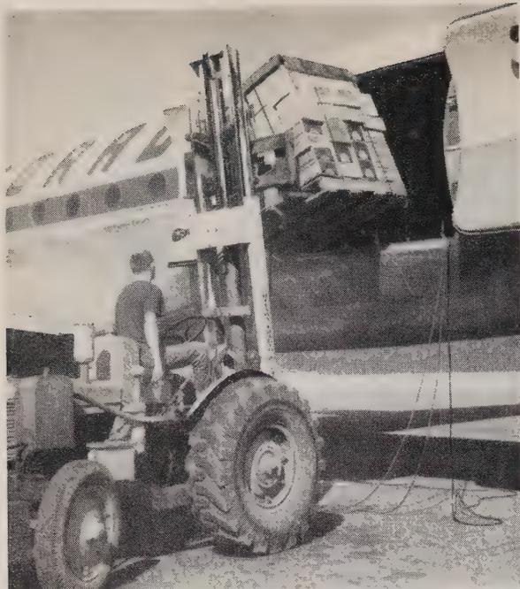
"Palletizing", or the strapping of loads of freight to pallets which are then fork-lifted into aircraft, has vastly speeded operations at both ends of the flight.
