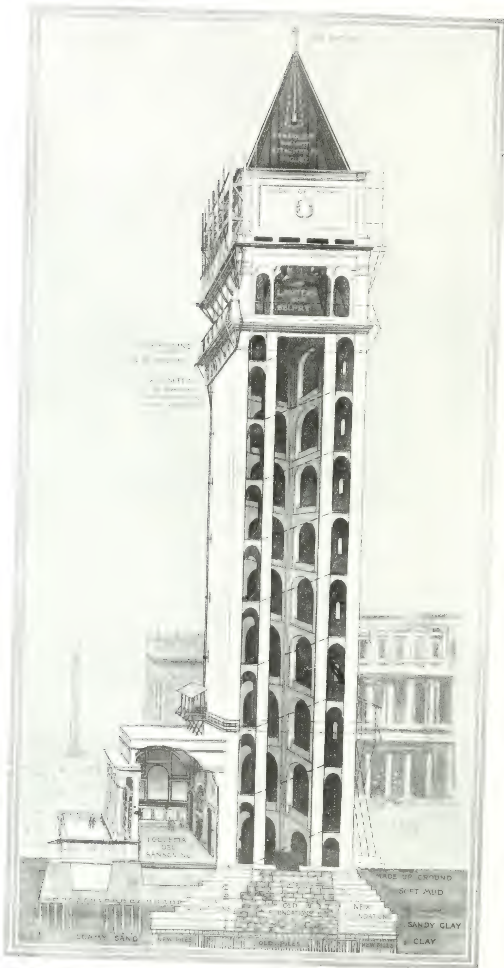
Sectional View of the New Campanile, Venice, which is Now in the Final Stages of Completion. This Illustration Gives an Accurate Idea of the Substructural Work Carried Out to Increase the Size of the Old Foundation, Which Was Found to be of Insufficient Width.
