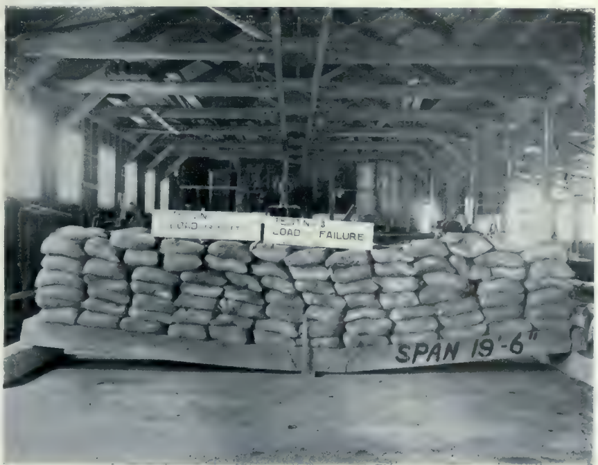
SIEGWART BEAM LOAD TEST. TYPICAL BEAMS FOR ALL DIFFERENT SPANS HAVE BEEN TESTED IN THIS MANNER TO CHECK CALCULATIONS.
