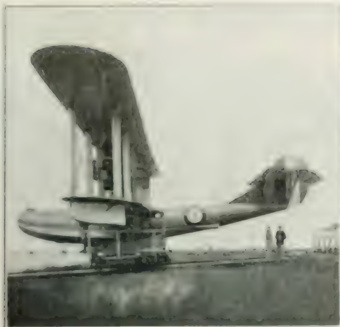
"Phoenix Cork" Flying Boat, two Rolls-Royce Eagle Engines The English Electric Co.
