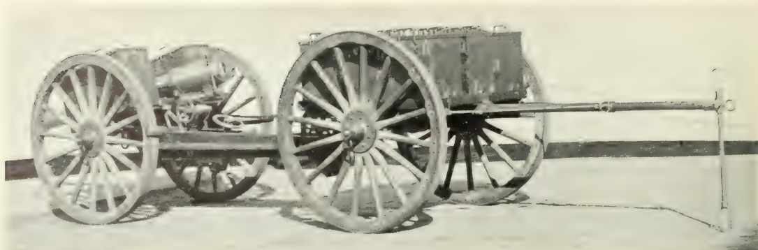
A 3-INCH FIELD MOUNT AND LIMBER
