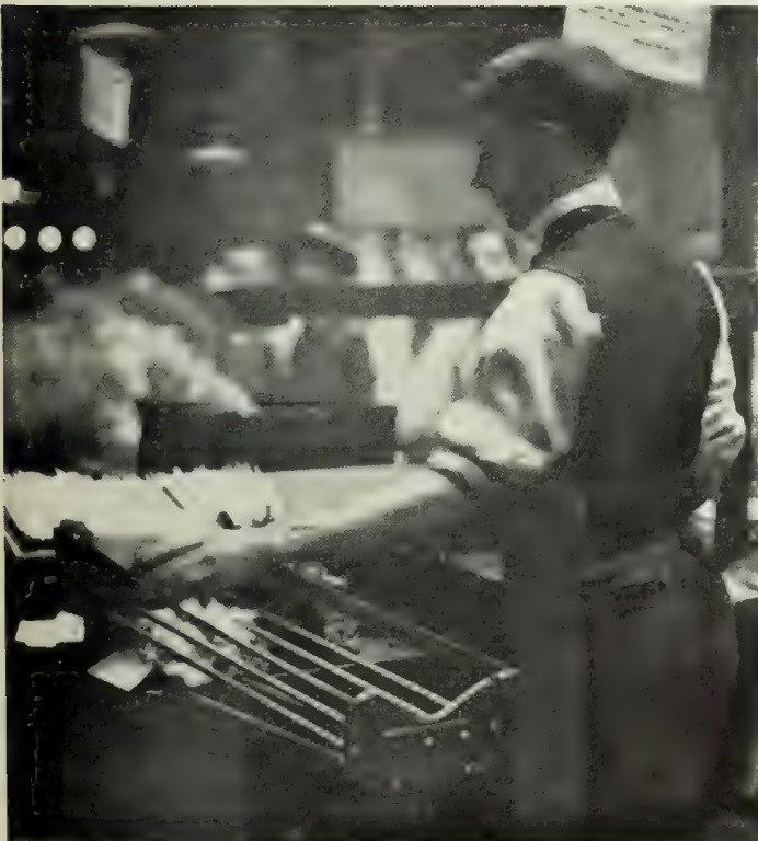
THE MACHINE AT WORK WHICH CANCELS THE STAMPS ON LETTERS
