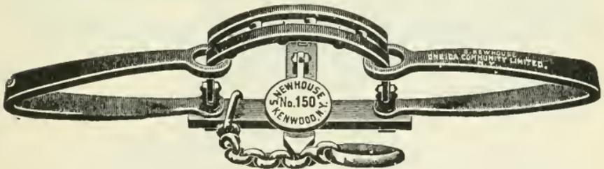
Spread of Jaws, 9 inches. This trap is identical with No. 5 excepting that the jaws are offset, making a space five-eighths inch between them. This allows the springs to come up higher when the bear's foot is in the trap, and thus secure a better grip. Also there is less chance of breaking the bones of the foot. Weight,  $11\frac{1}{4}$  pounds each.
