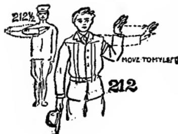
Fig. 212. Move to my left! Surveyors' signal which, reversed, would mean, move to my right. That this signal may be seen further, a surveyor sometimes holds a handkerchief in his hand and sometimes his hat in one hand and his handkerchief in the other.
