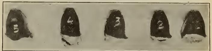
Figure No. 5.—Fractured Teeth of a Series of Pinions Tested by Repeated Compact.
