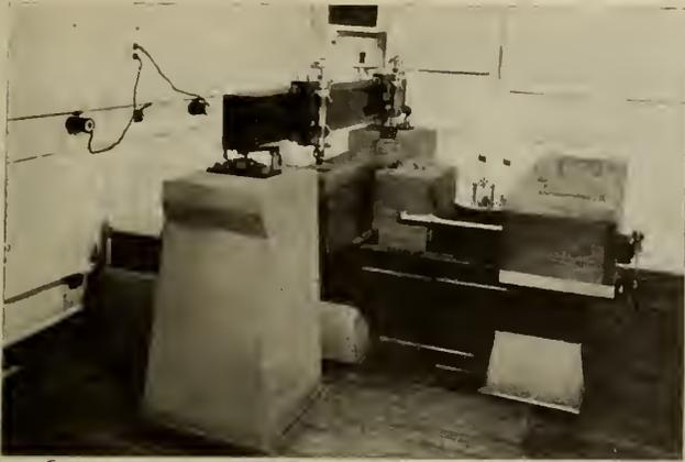
Figure No. 3.—Length Comparator, Physical Testing Laboratory.
