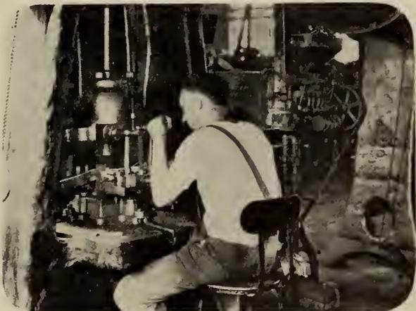
Figure No. 4.—Type of Machine Used in Hot Pressing Method.
