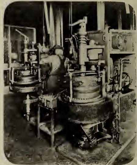
Figure No. 5.—Rough Grinding with Double Head Grinder.
