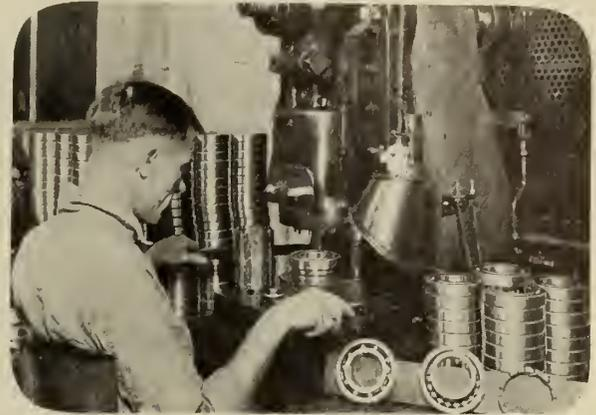
Figure No. 22.—Assembly of Bearings.
