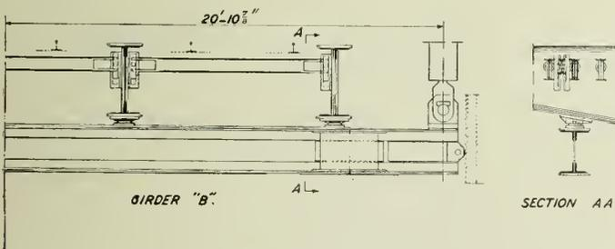
Fig. 12—Details at Apron Girder B.
