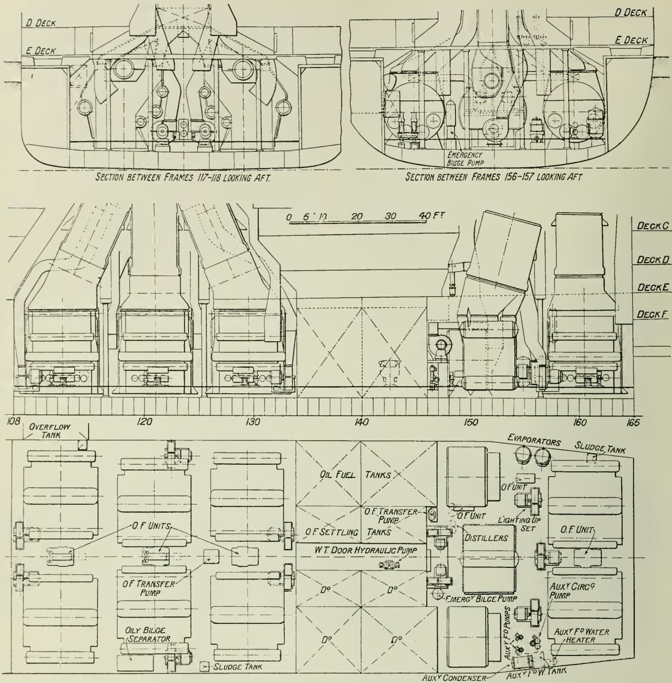
Fig. 3—Plan of Boiler Rooms.
