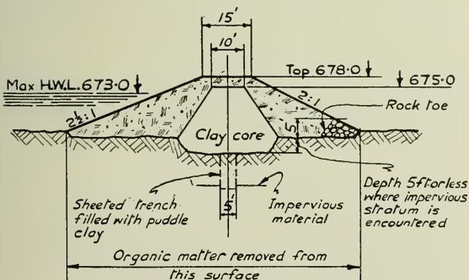
Fig. 9—Auxiliary Earth Fill Dam.
