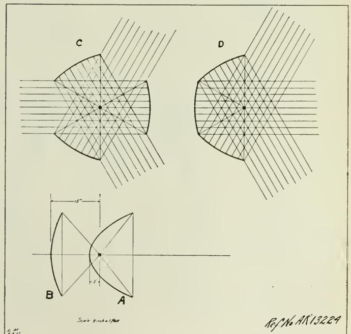
Fig. 9—Diagram of Parabolic Reflector Systems.
