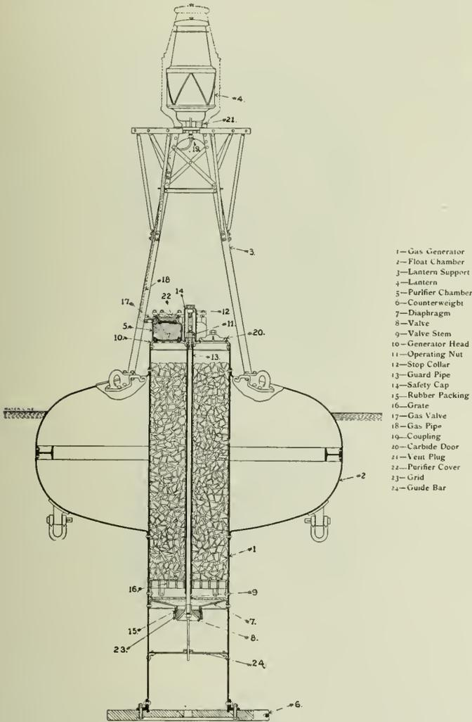
Fig. 2—Diagram of Gas Buoy.
