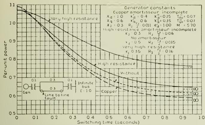
Fig. 25—Power that can be carried through the first Swing with a Line-to-Line Fault by a Water-Wheel Generator with and without Amortisseur Windings.
