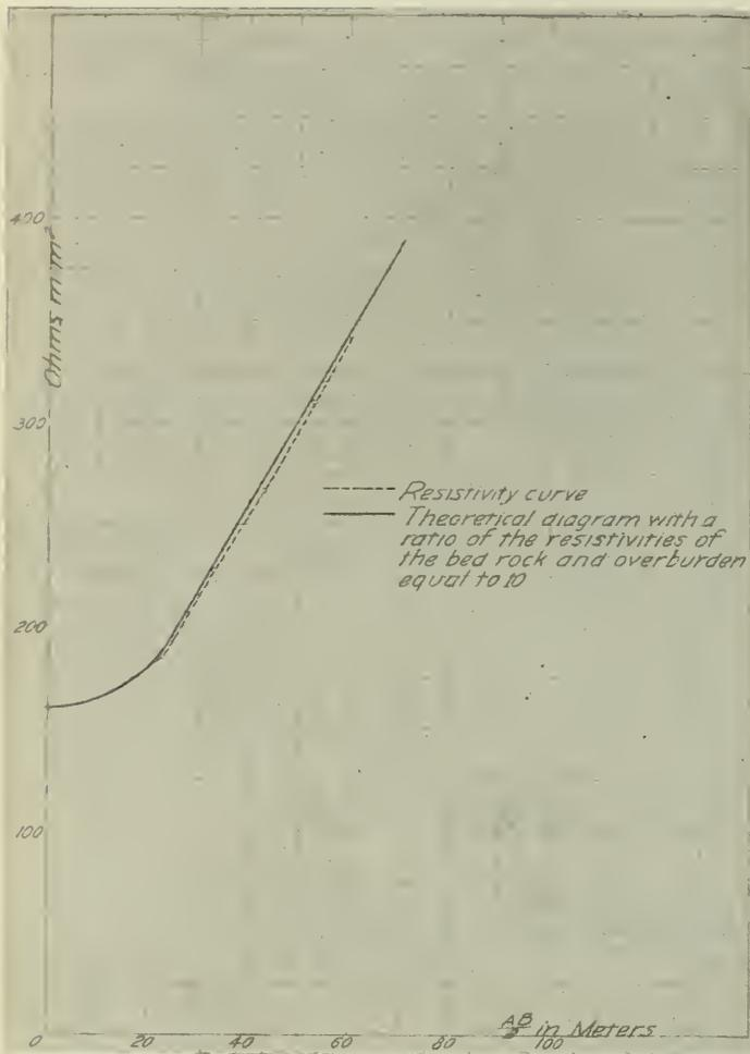
Fig. 4—Resistivity Curve at Electrical Station 18 (Fig. 3) Showing the Variations of this Parameter with Distance between Primary Electrodes.
