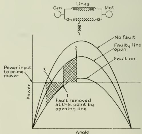
Fig. 14—Stability with Fault Removed from the System.
