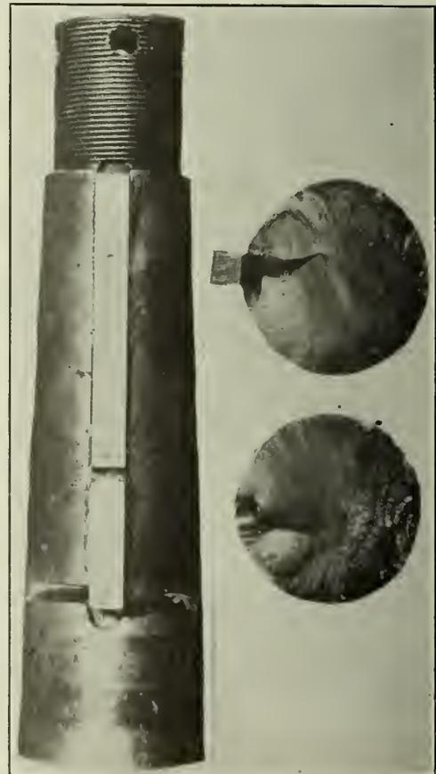
Fig. 1—Axle Fractured at End of Keyway.
