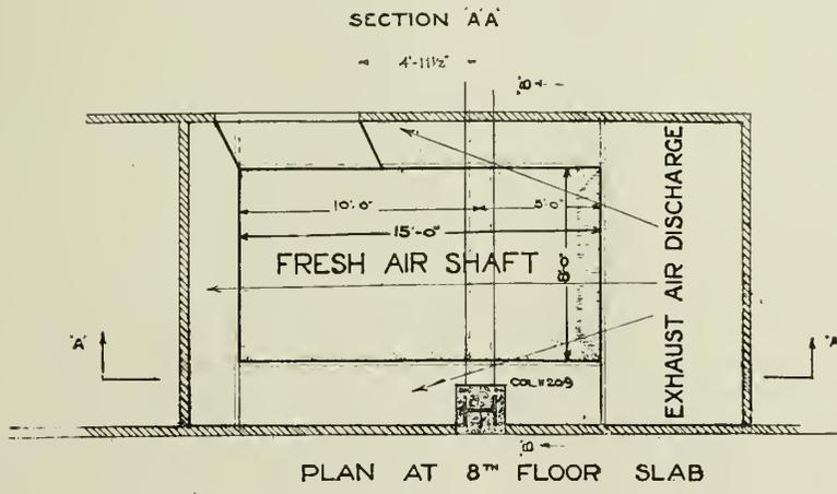
Fig. 7—Section and Plan of Heat Interchanger. Top of Airshaft.
