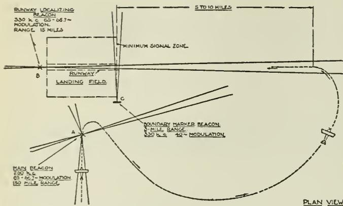
Fig. 1—General Arrangement for the Low Power Runway Localizing Beacon.
