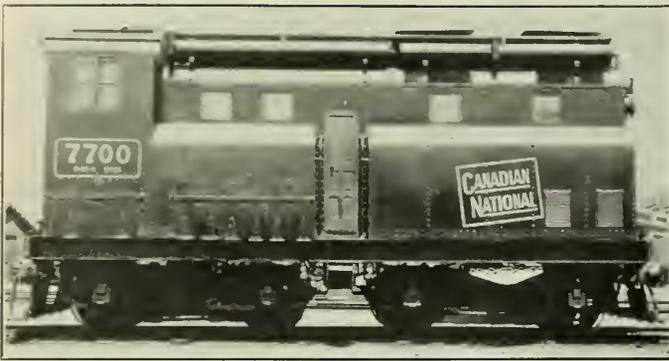
Fig. 7—450 h.p. Six-Cylinder Switching Locomotive.
