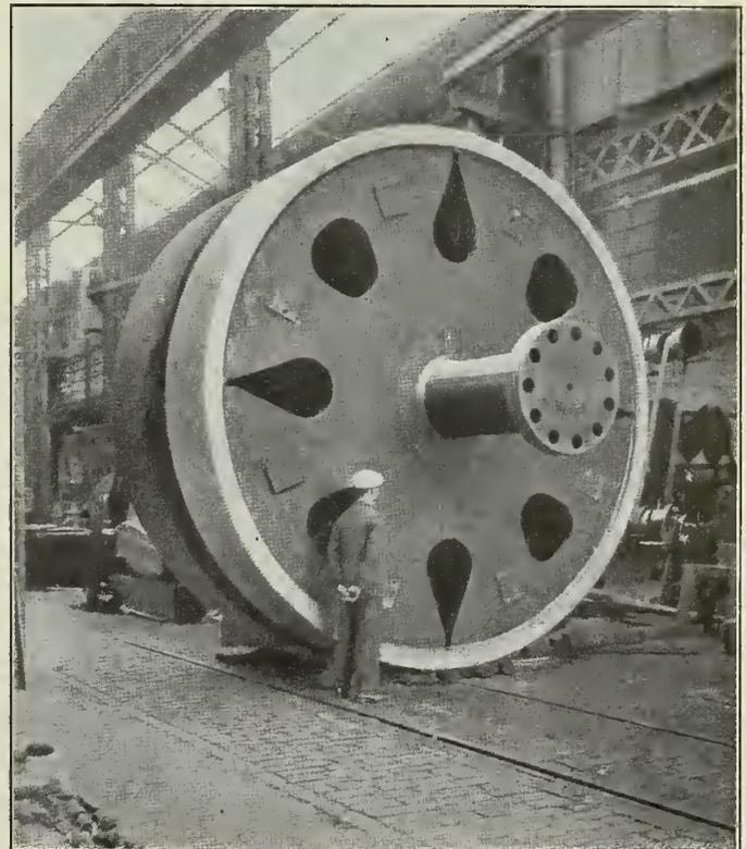
Fig. 4—Main Gear Wheel for Inboard Shaft.
