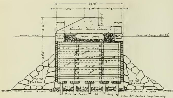
Fig. 3—Typical Section—Concrete Breakwater.
