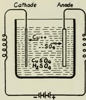
Fig. 1—Simple Electrolytic Cell.
