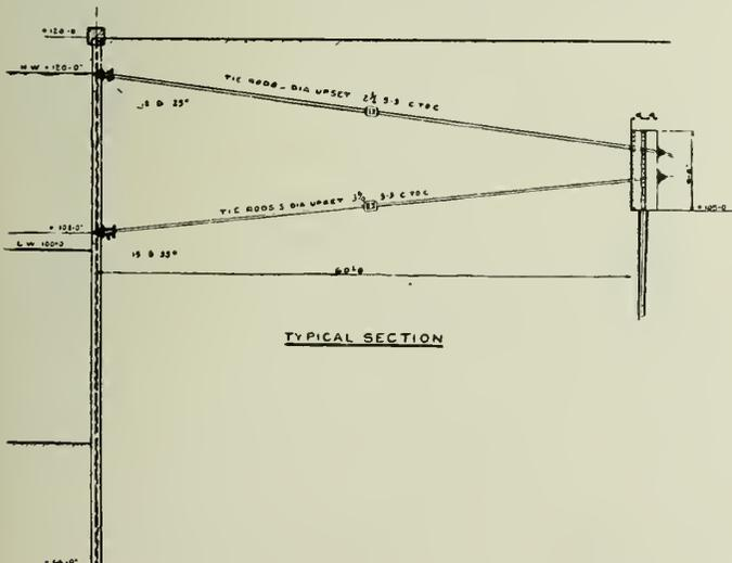
Fig. 4—Arrangement of the Anchor Rods and Walings.
