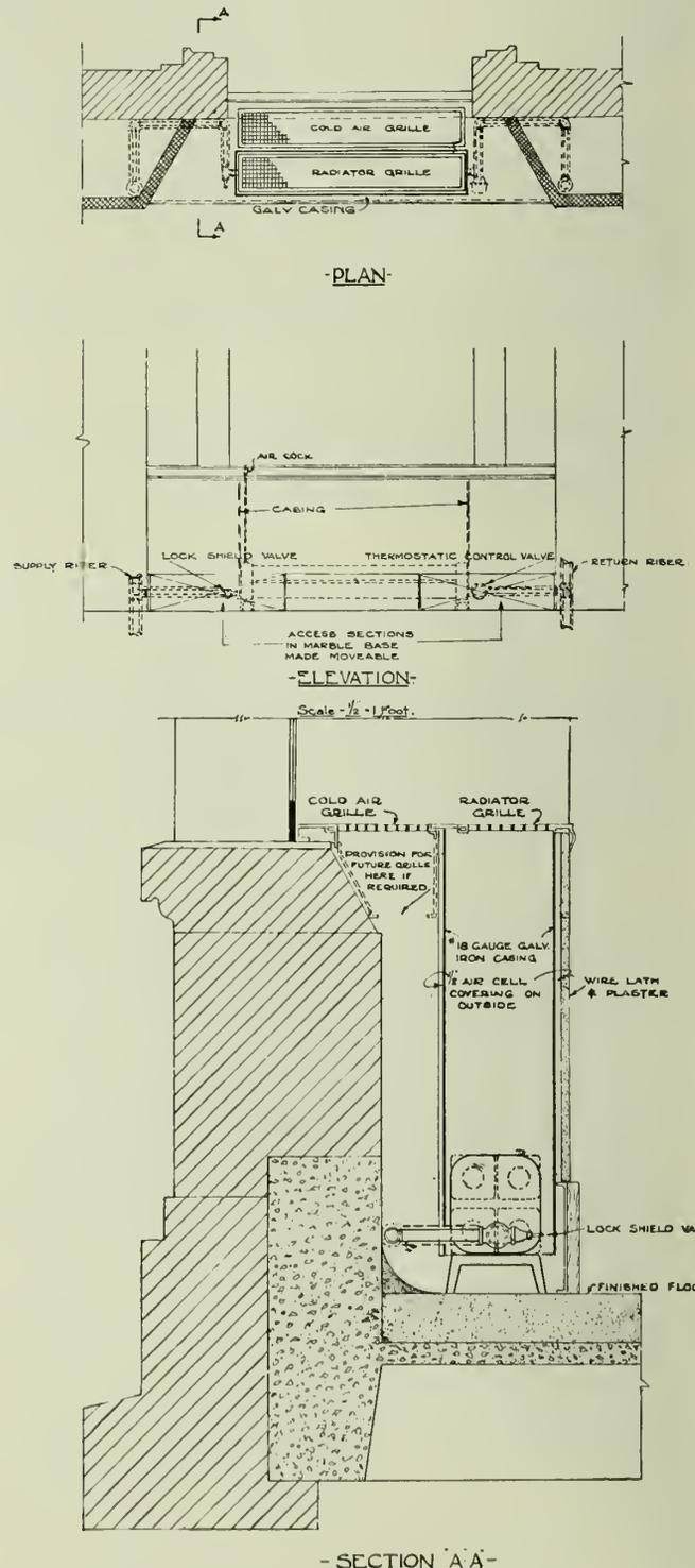
Fig. 2—Typical Details of Concealed Radiators.
