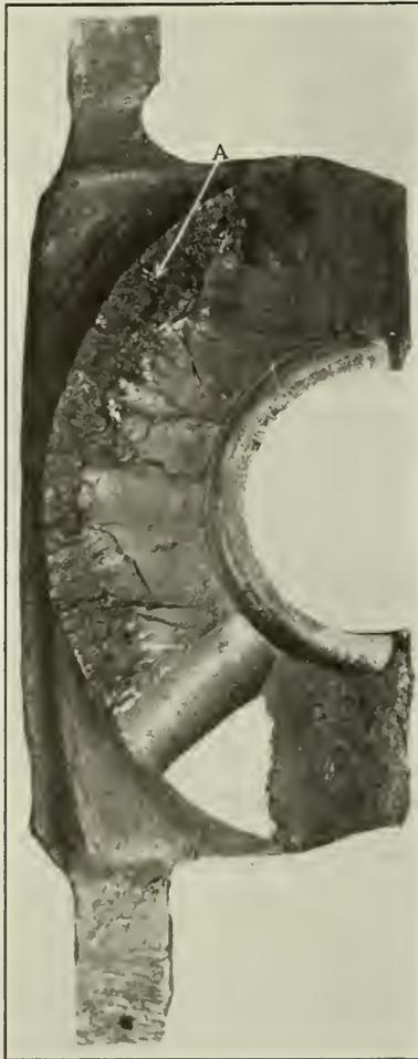
Fig. 10—Failure due to Flaws in Casting.
