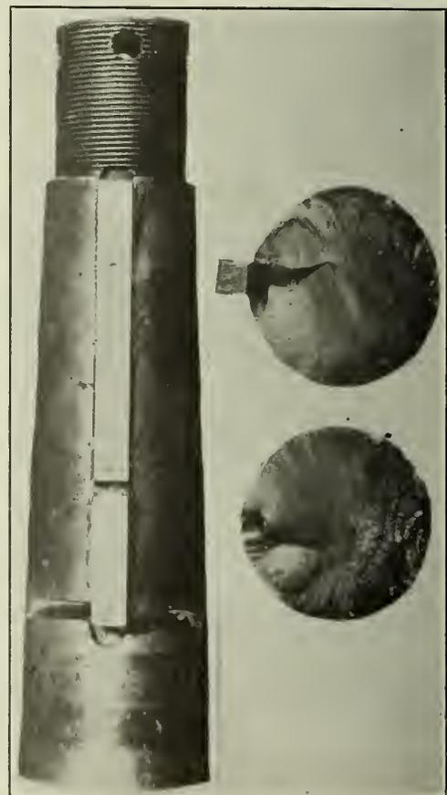
Fig. 1—Axle Fractured at End of Keyway.
