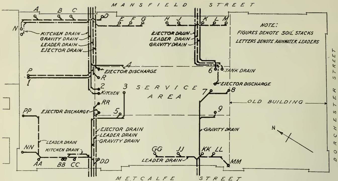
Fig. 1—First Basement Plan.
