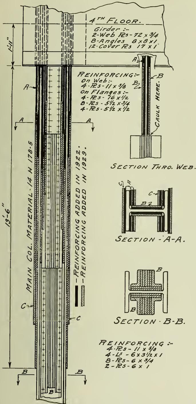
Fig. 8—Reinforcing of Column No. 33.
