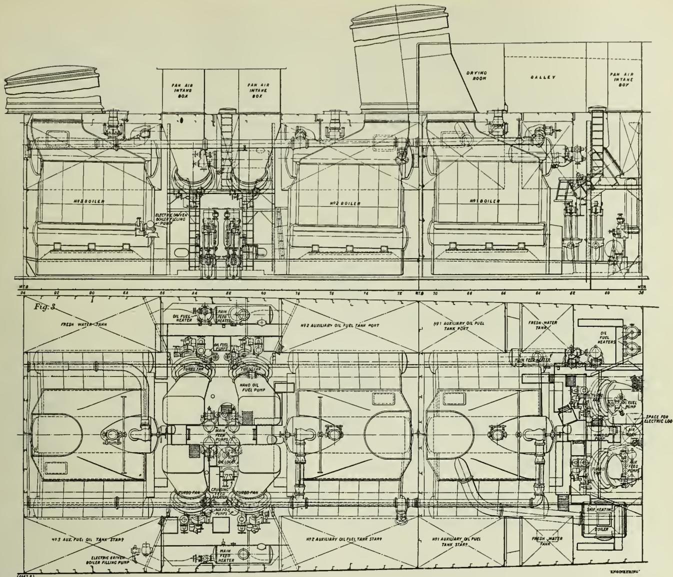
Figs. 2 and 3—Arrangement of Machinery in Boiler Rooms.
