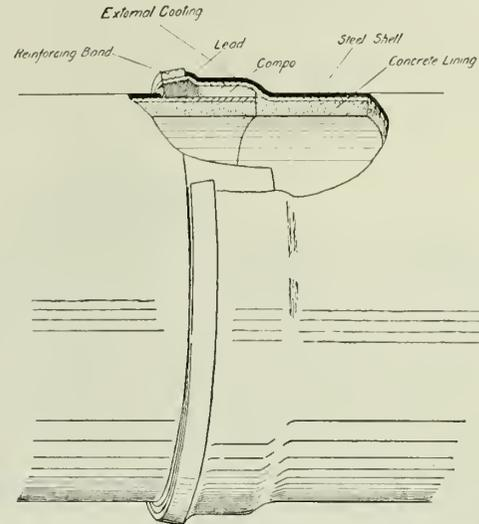
Fig. 5—Section Through Hume Pipe Joint.
