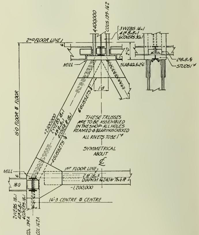
Fig. 12—Truss Carrying Columns 139 and 162.
