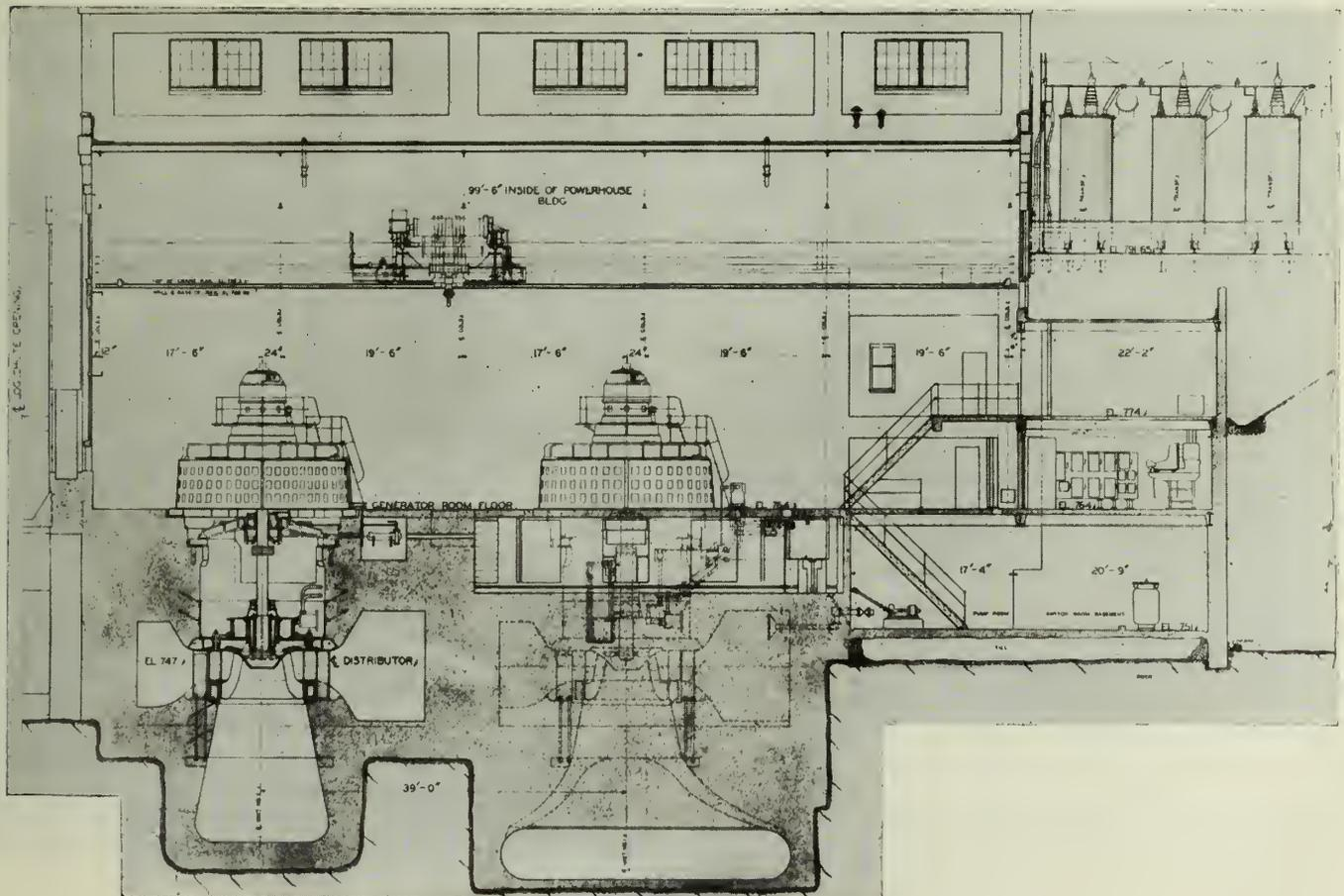
Fig. 4—Longitudinal Section through Generator Room and Switch Room.
