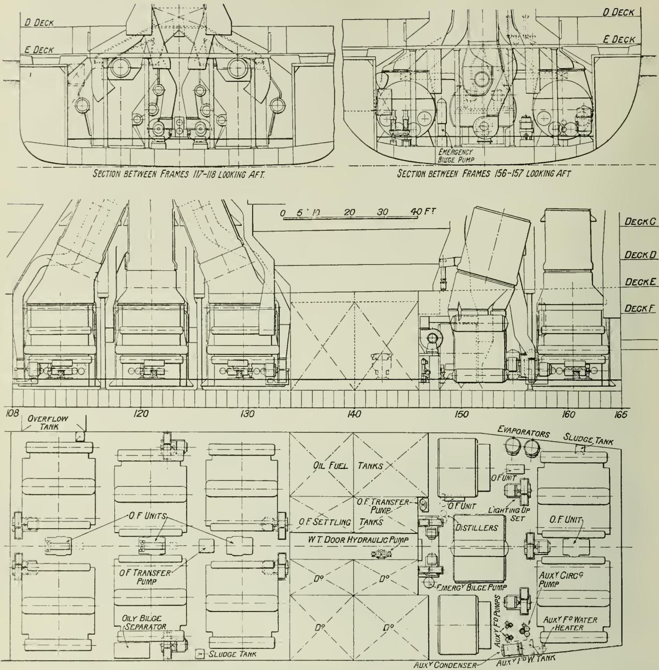
Fig. 3—Plan of Boiler Rooms.
