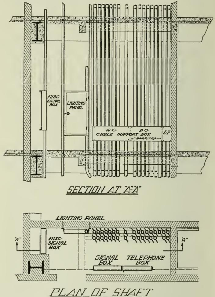
Fig. 7—Details of Typical Electric Riser Shaft.
