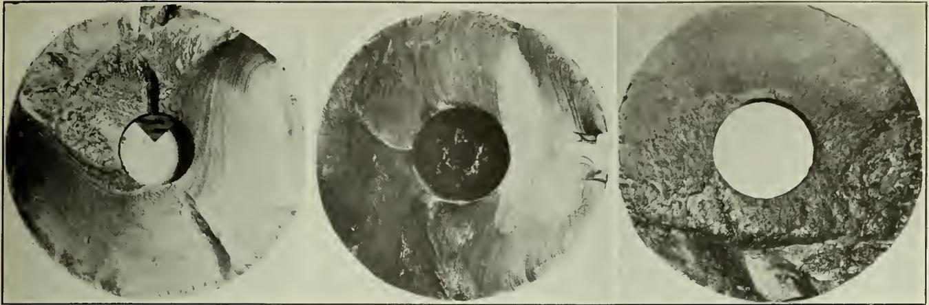
Fig. 2—Section Carbon Steel Axle that Failed in Service.
