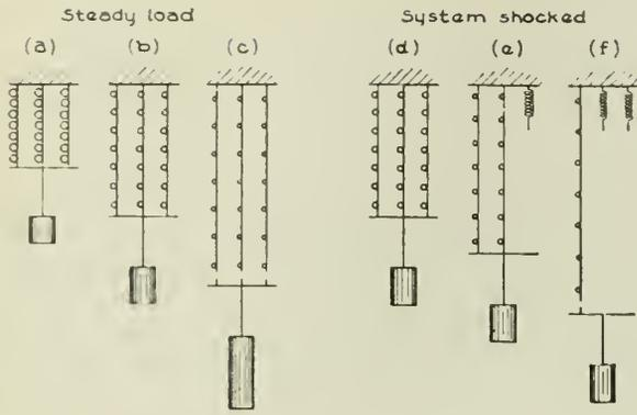
Fig. 1—Analogies of Steady State and Transient Stability.
