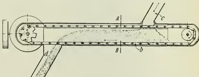
Fig. 9—Diagrammatic Section of Standard Redler Conveyor.
