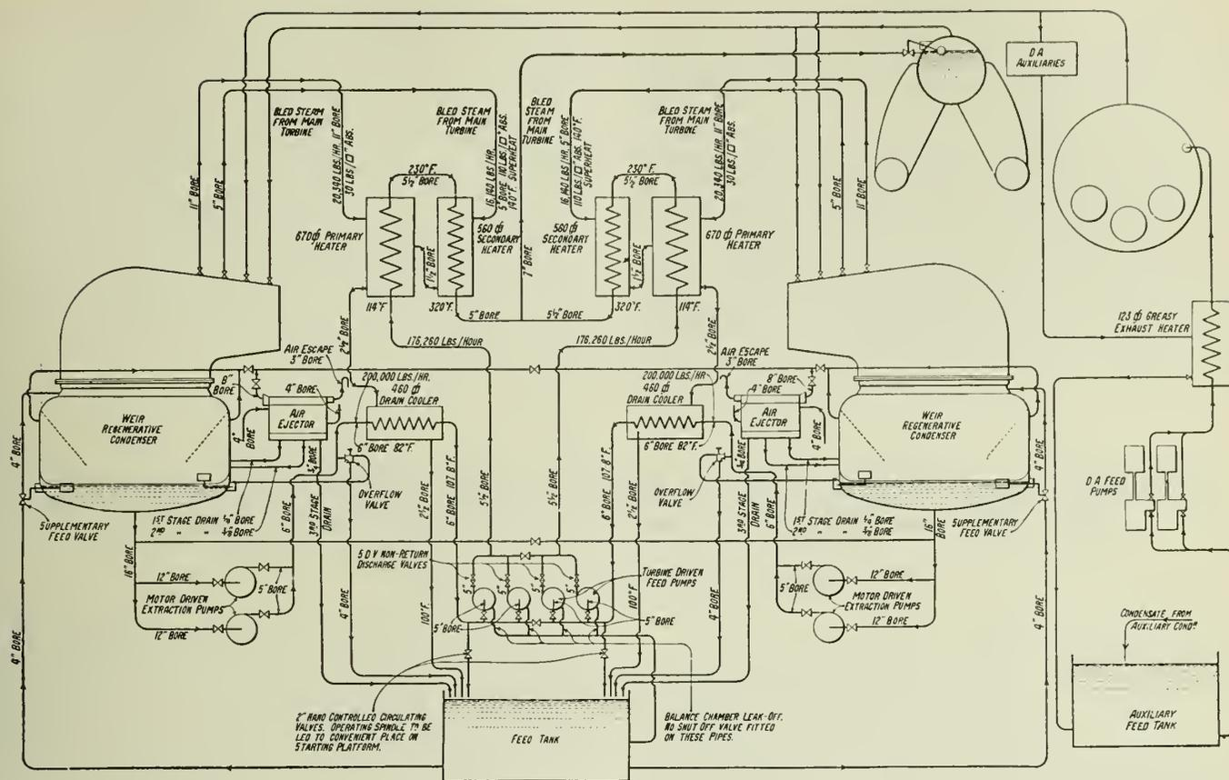
Fig. 6—Diagrammatic Layout of Closed Feed System for Forward Engine Room.
