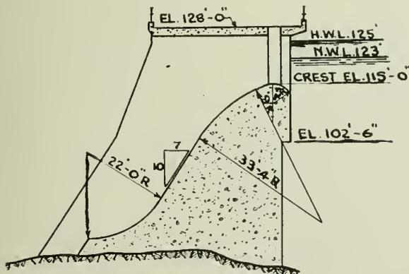
Fig. 9—Section Through Ice Sluice.
