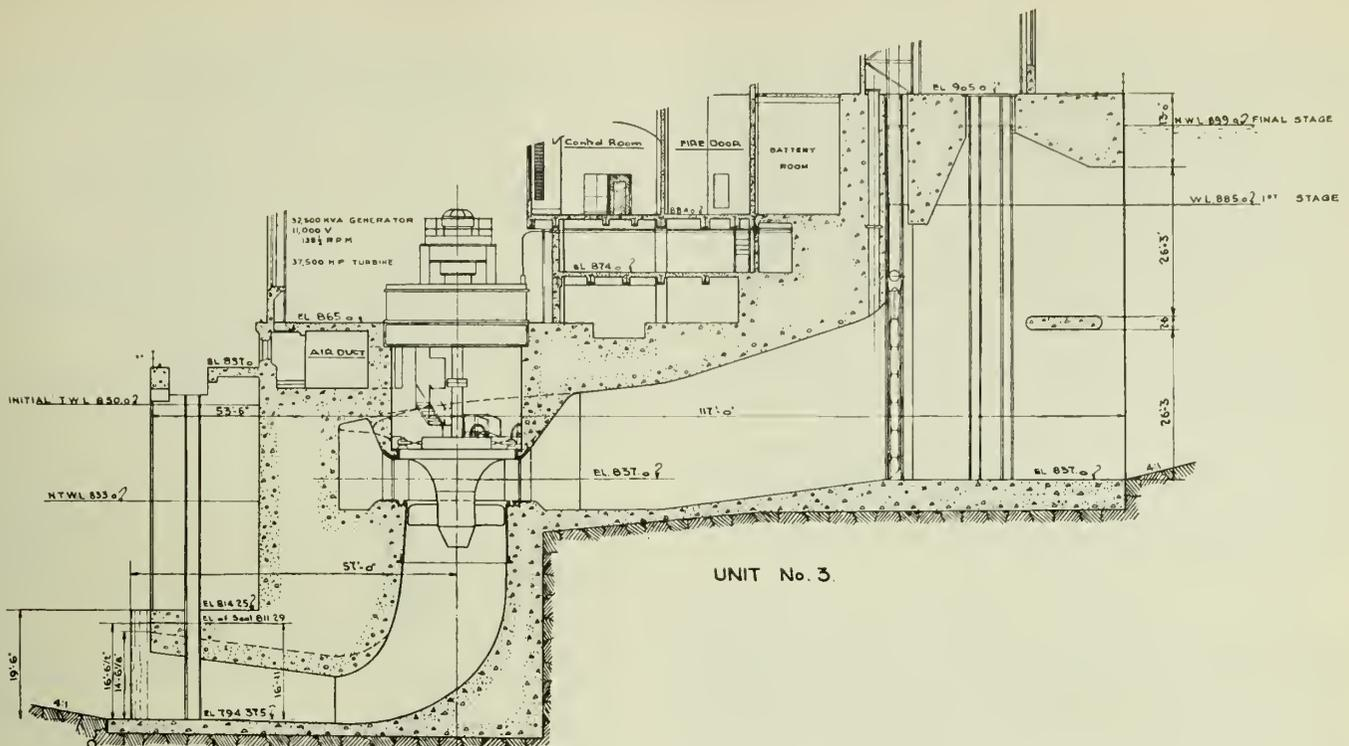
Fig. 8a—Cross Section through Power House Showing No. 3 Unit Turbine Setting.
