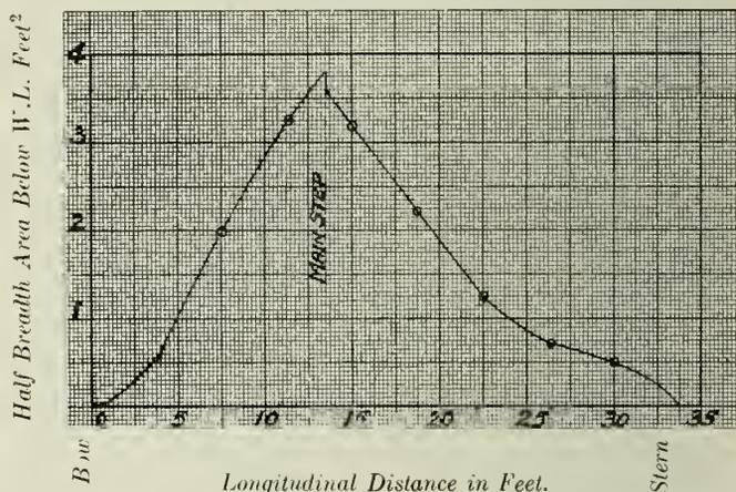
Fig. 4—Buoyancy to L.W.L.
