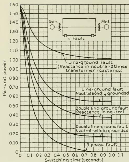
Fig. 22—Power-Switching Time Curves for various Kinds of Faults and the effect of Neutral Reactance.
