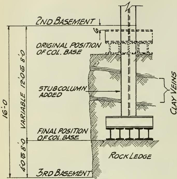
Fig. 5—Downward Extension of Column.
