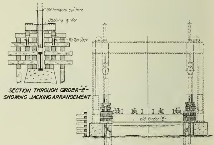
Fig. 19—Temporary Arrangement for Operating Landing Gantry E.
