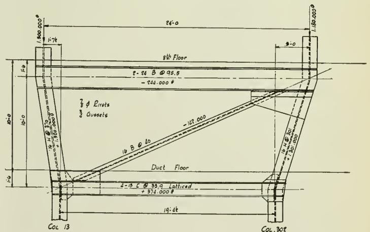
Fig. 10—Details of Sloping Columns Nos. 13 and 302.
