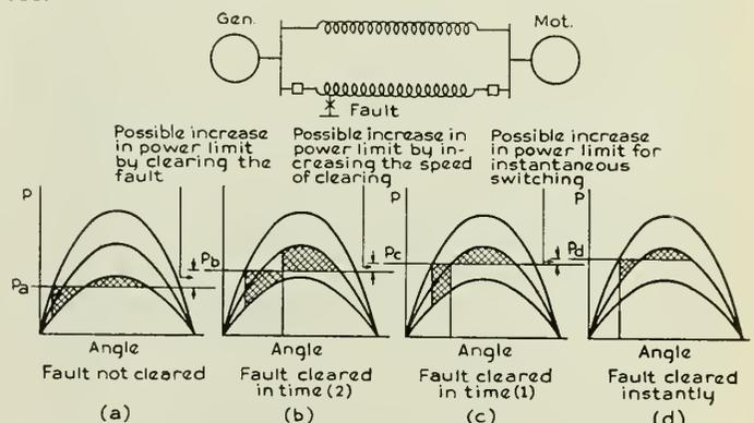
Fig. 16—Variation in Power Limit with Switching Time.
