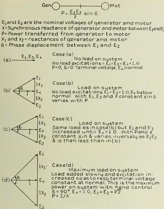
Fig. 7—Successive Steps in Loading a System Comprising an Identical Generator and Motor on the Same Bus.
