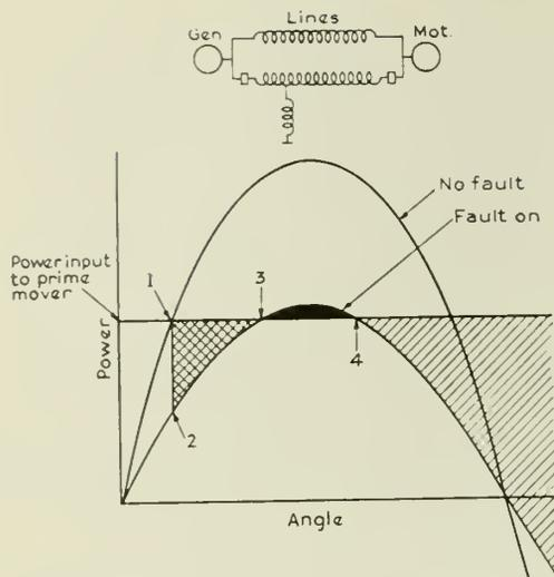
Fig. 13—Instability with Fault Remaining on the System.
