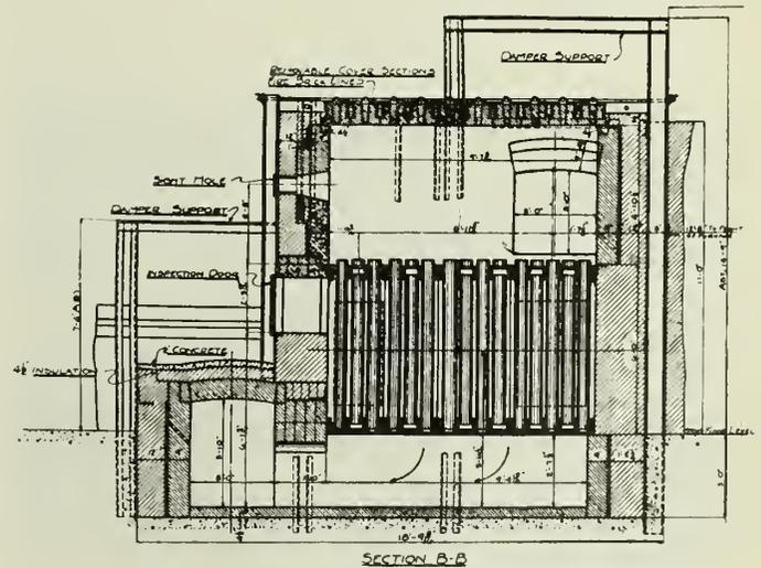
Fig. 5—Section Through Regenerator.
