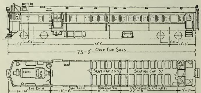
Fig. 3—Plan and Elevation of 300 h.p. Six-Cylinder Car.
