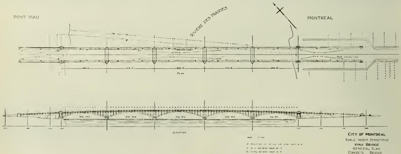
Fig. 3—Plan and Elevation of Bridge.
