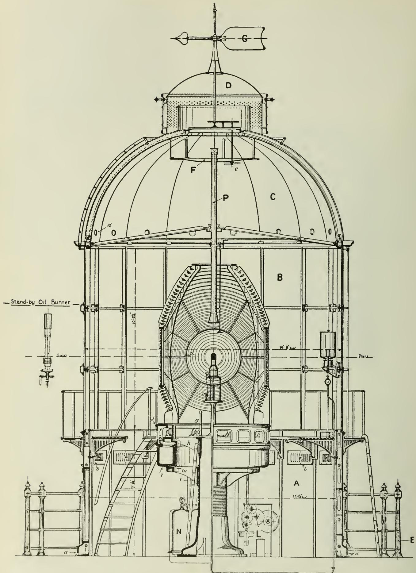
Fig. 10—General Arrangement of Lighthouse Lantern.
