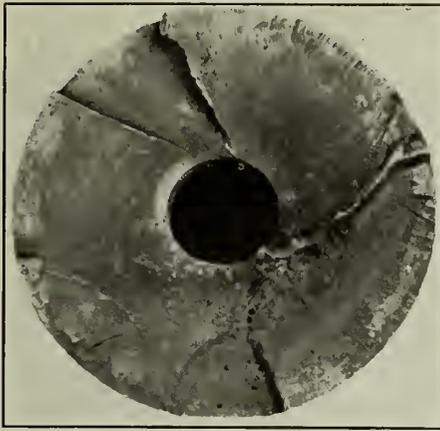
Fig. 7—Failure in Carbon Steel Axle.
