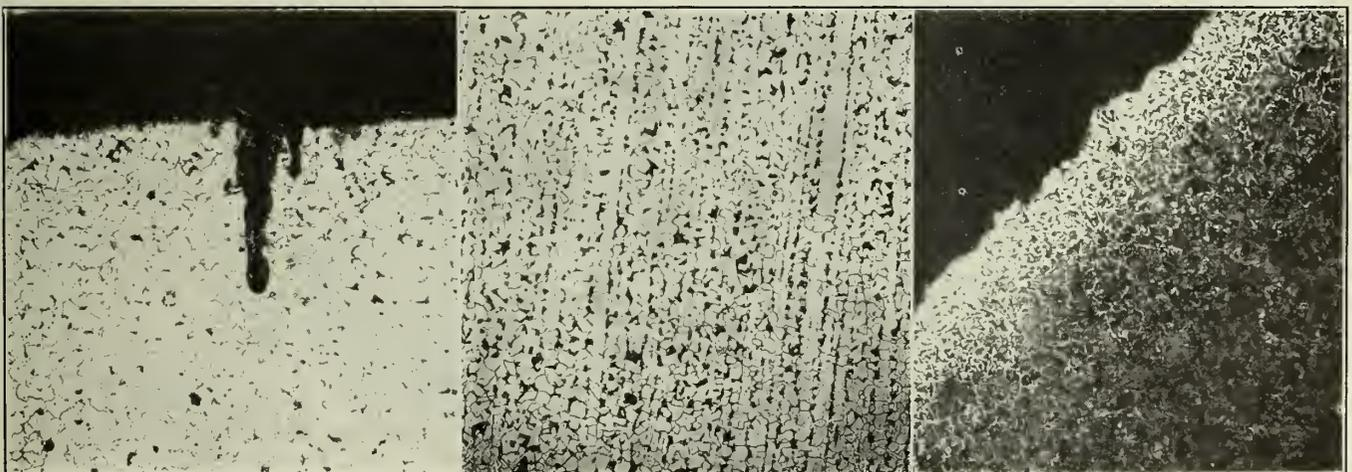
Fig. 13—Corrosion Crack in Boiler Plate.
