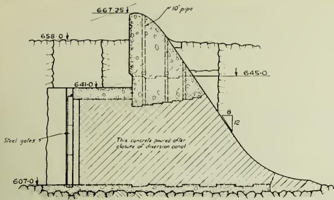
Fig. 4—Section through Sluiceways at Outlet of Diversion Channel.
