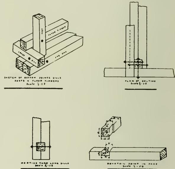
Fig. 2—Cribwork Connections.
