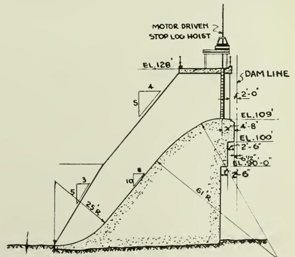
Fig. 10—Section Through Spillway.
