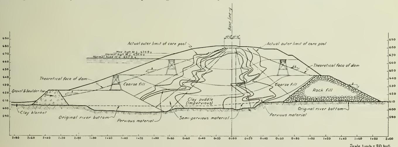
Fig. 5—Typical Section of Main Dam.
