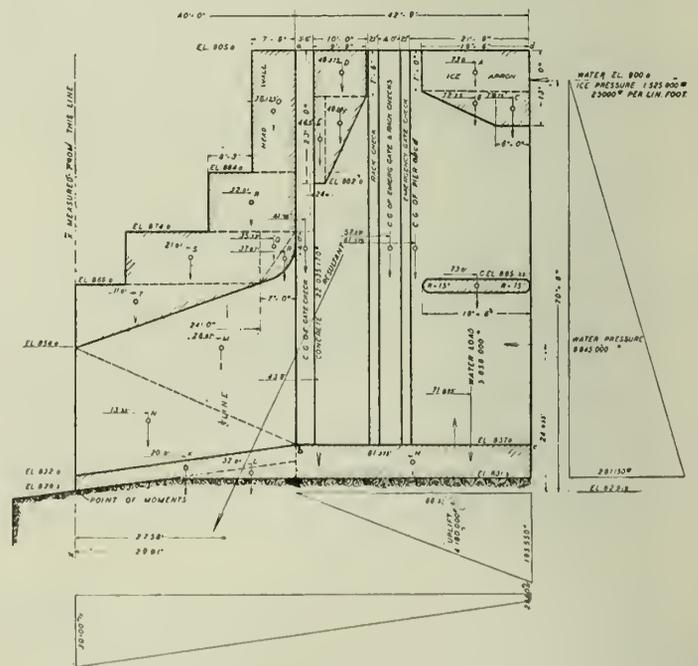
Fig. 4—Power House Stability Diagram.
