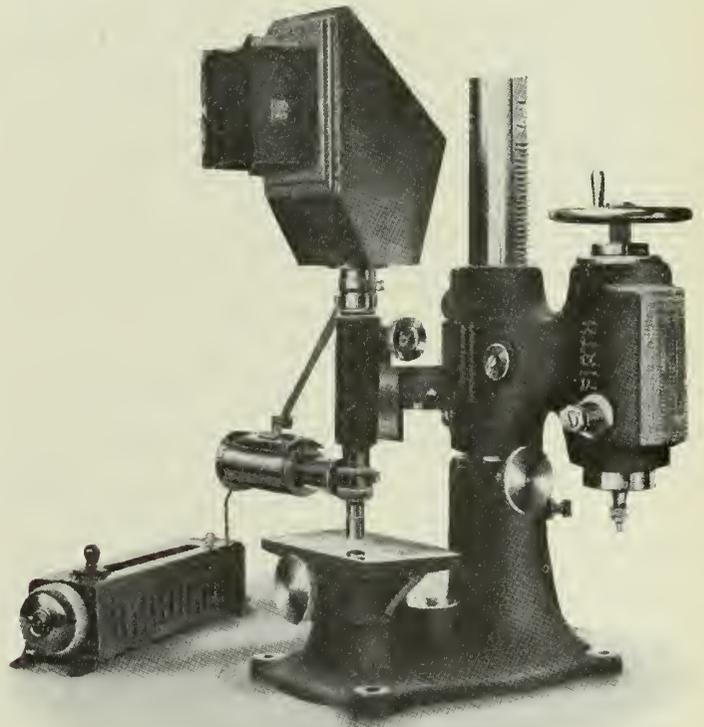
Fig. 12—The Firth Hardometer.
