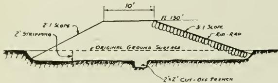
Fig. 11—Typical Section Through Earth Fill Dam.
