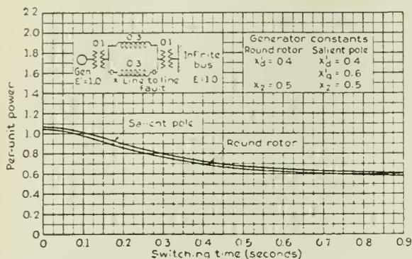
Fig. 27—Switching Time Curve Comparison of Salient Pole and Round Rotor Synchronous Machine Calculations.
