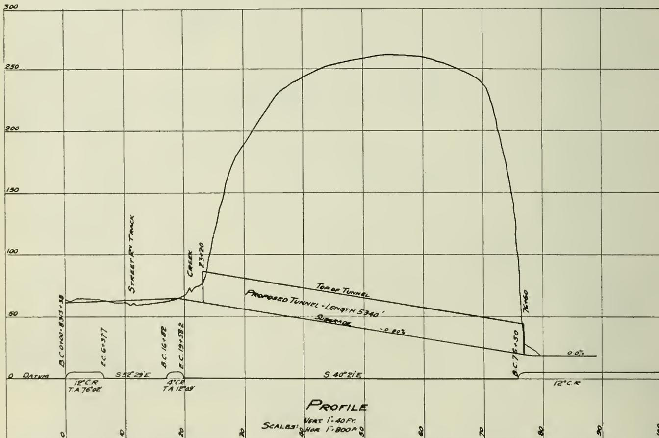
Fig. 3—Profile of Tunnel.
