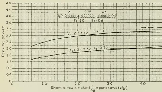
Fig. 5—Short Circuit Ratio,  $\frac{1}{x_d}$  approximately.
