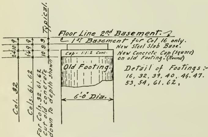
Fig. 6—Reinforcement of Footings in Original Building.
