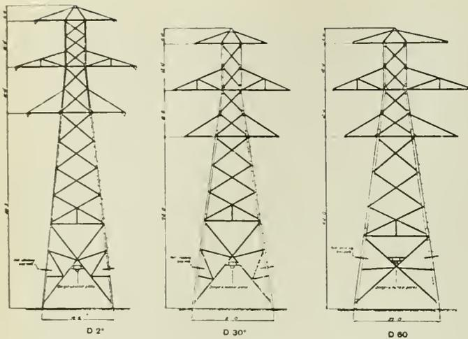
Fig. 5—Types of Double-Circuit Towers.
