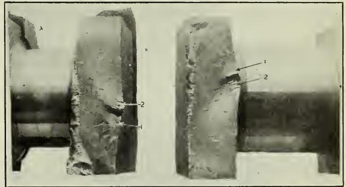
Fig. 8—Fractured Ends of Crank Shaft.
