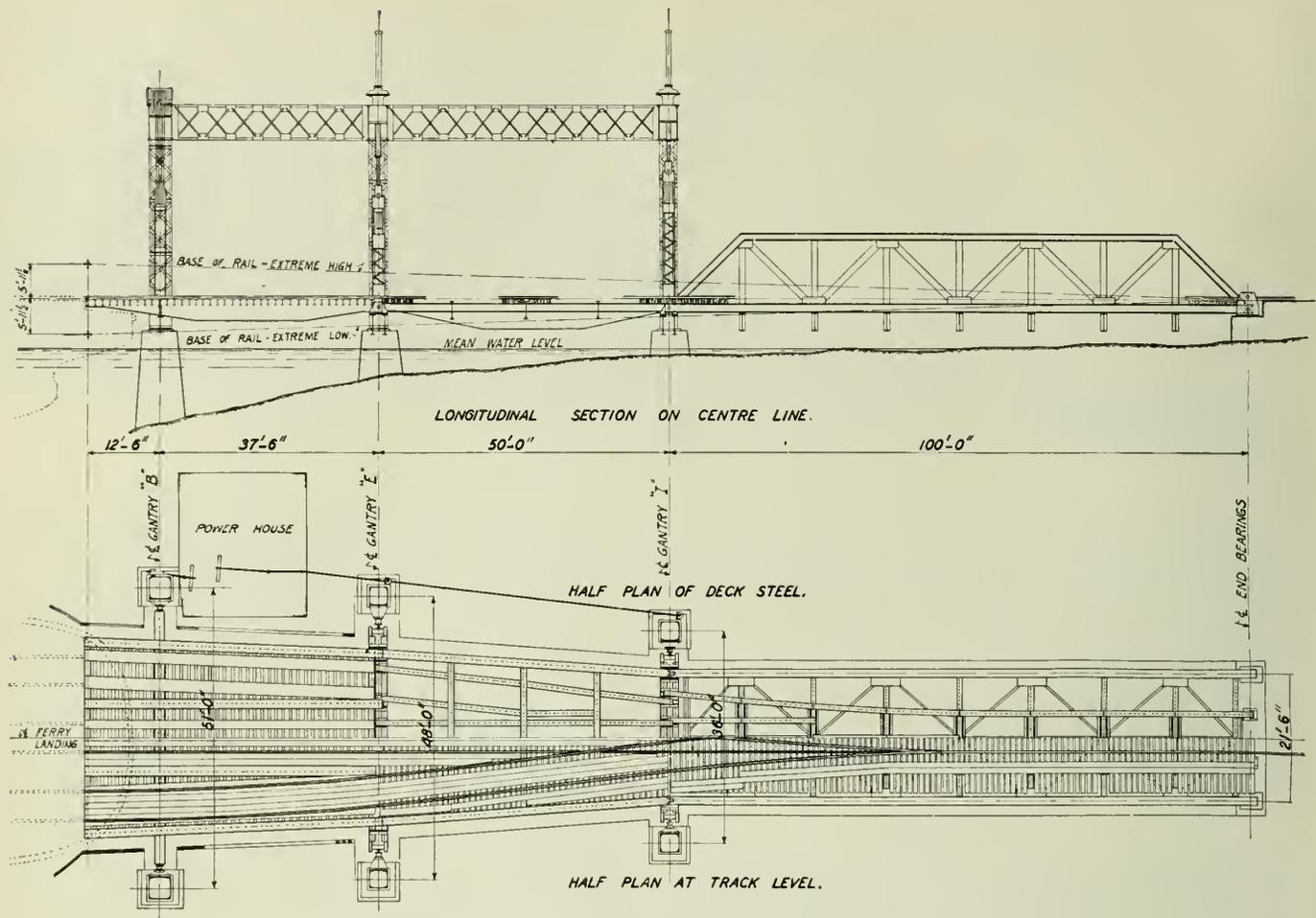
Fig. 5—Plan and Longitudinal Section through Ferry Landing.
