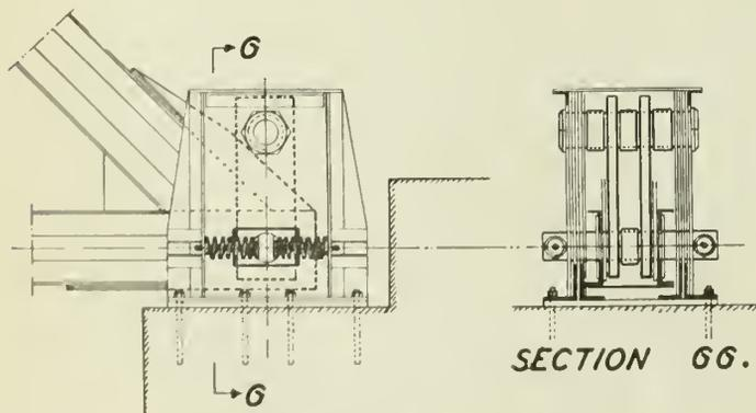
Fig. 8—Truss Span—Shoe and Buffer.
