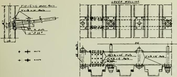
Fig. 3—Typical Section of Steel Wall.
