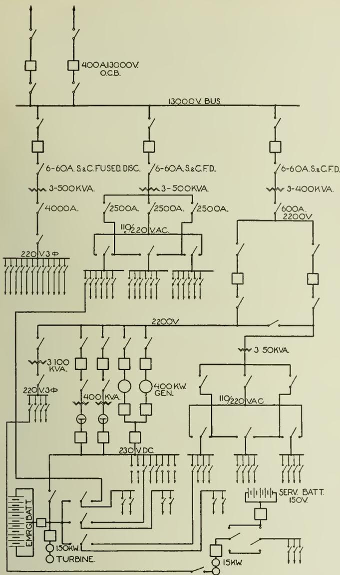
Fig. 8—Single Line Feeder Diagram.
