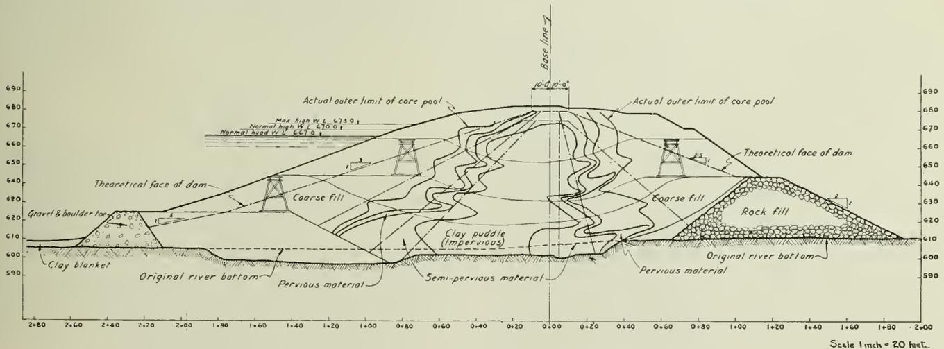
Fig. 5—Typical Section of Main Dam.
