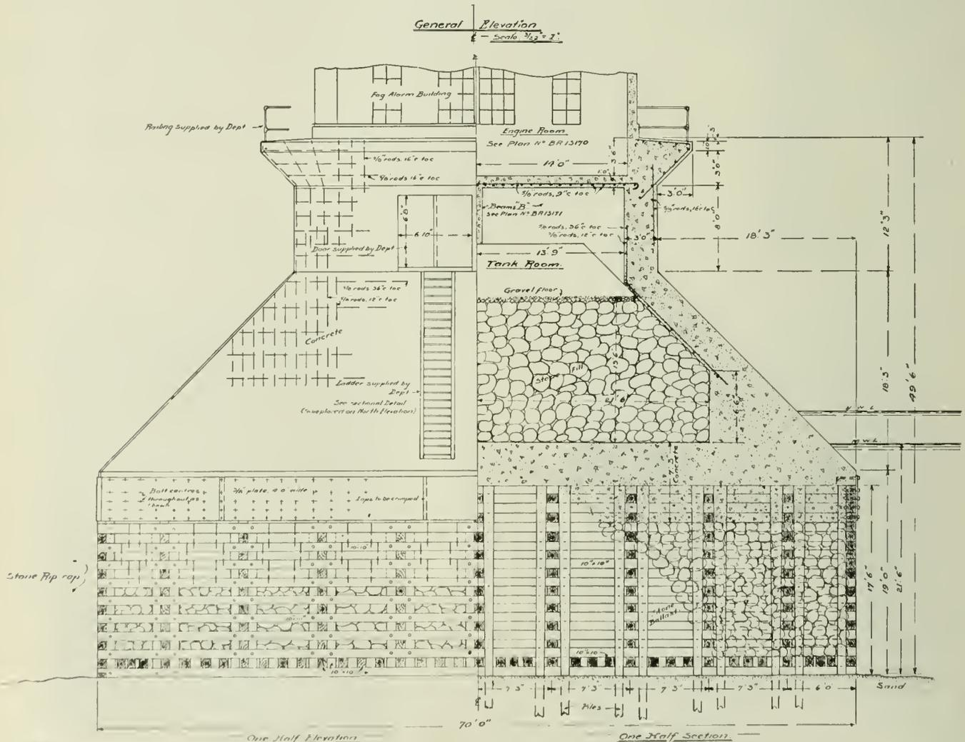
Fig. 6—Elevation and Section, Southeast Shoal Lightstation.
