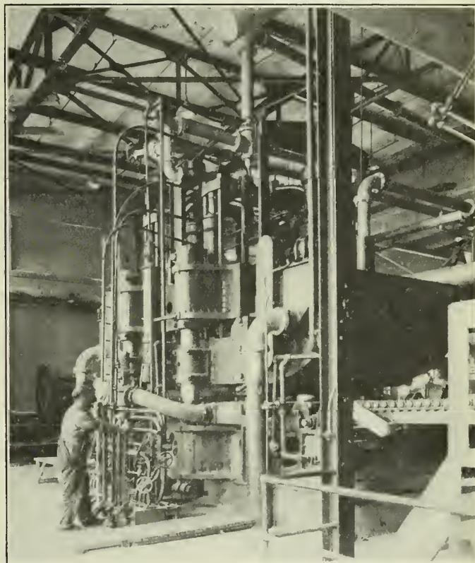
Fig. 3—Forming Machine showing Arrangement of Platens and Hydraulic Press.
