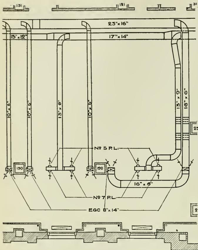
Fig. 5—Part Plan of Typical Floor. Upper Zones.
