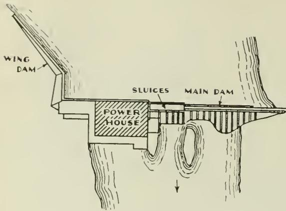
Fig. 6—Plan of Island Falls Power Dam.
