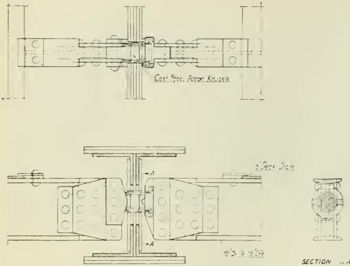
Fig. 14—Connection of Deck Beams to Apron Girders.
