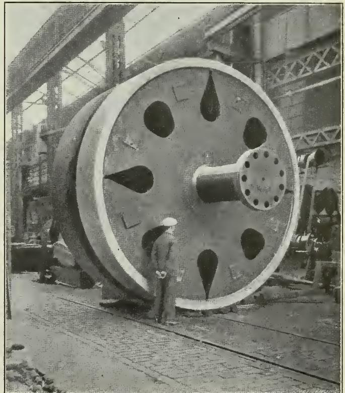
Fig. 4—Main Gear Wheel for Inboard Shaft.
