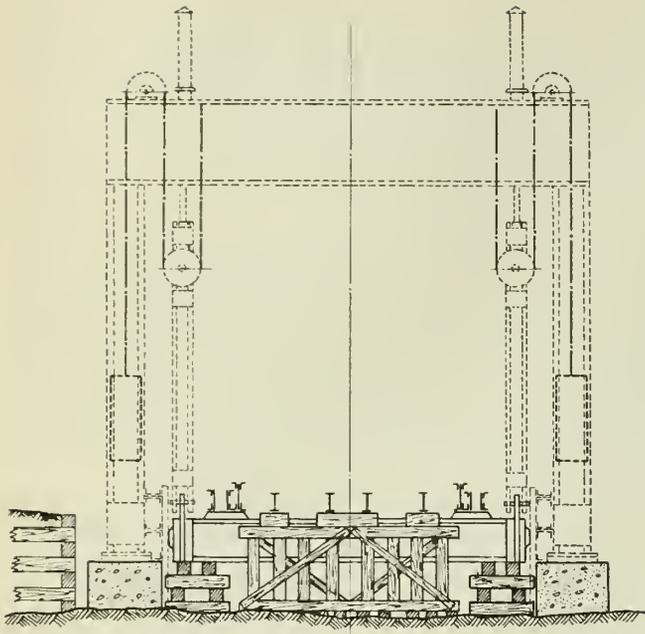
Fig. 17—Temporary Blocking under Girder *I* and Stringers of Truss Spans.
