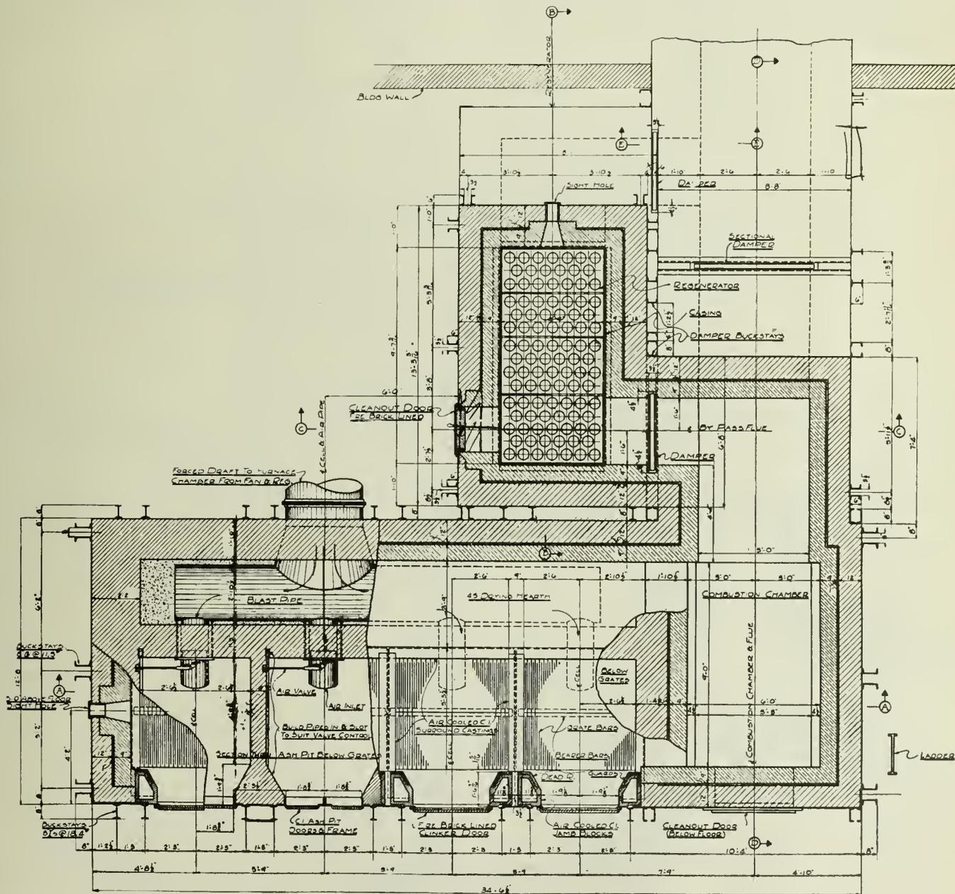
Fig. 2—Plan of Furnaces, Combustion Chamber, Flue and Regenerator.
