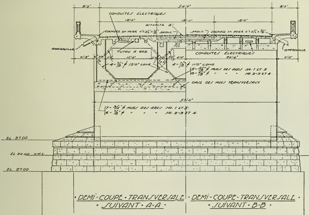
Fig. 4—Plan and Elevation of Pier.
