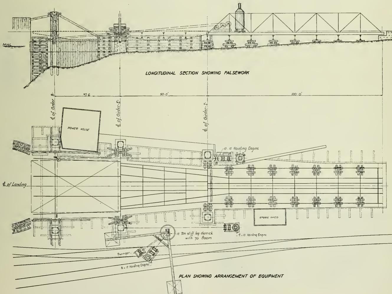
Fig. 16—Plan showing Arrangement of Erection Equipment and Falsework.
