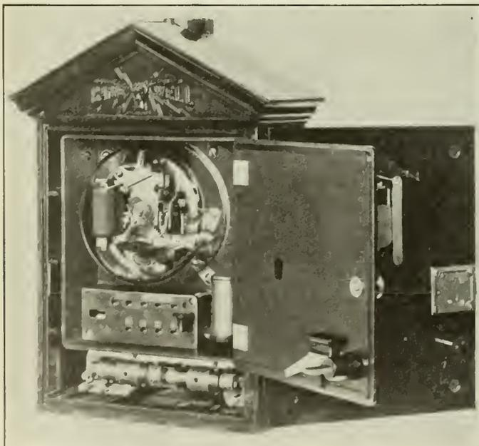
Fig. 8—Positive Non-Interfering Successive Alarm.
