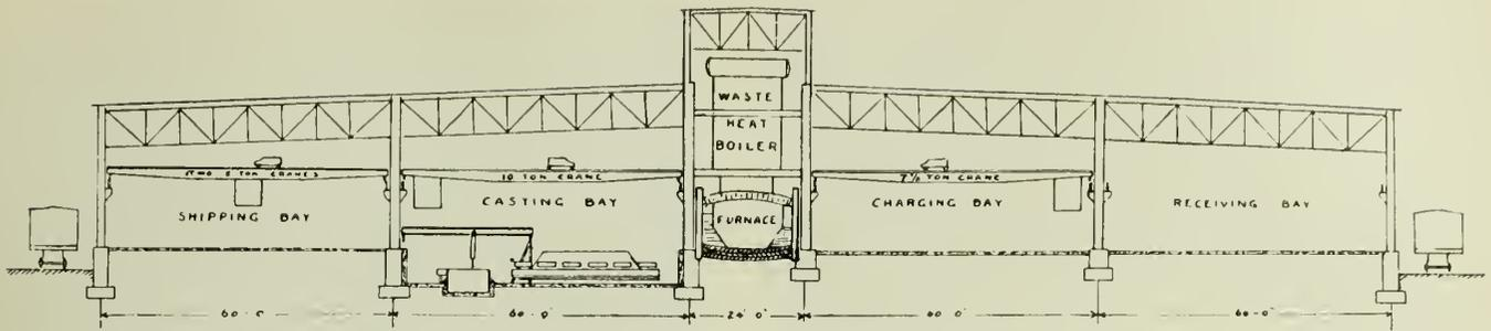
Fig. 3—Cross Section of Refinery.
