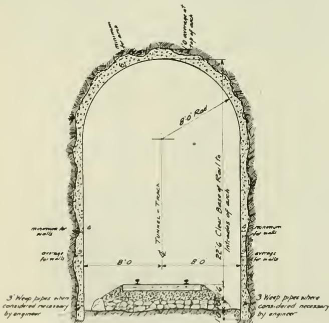
Fig. 7A—Typical Section of Interior Where Rock is Self-Supporting.
