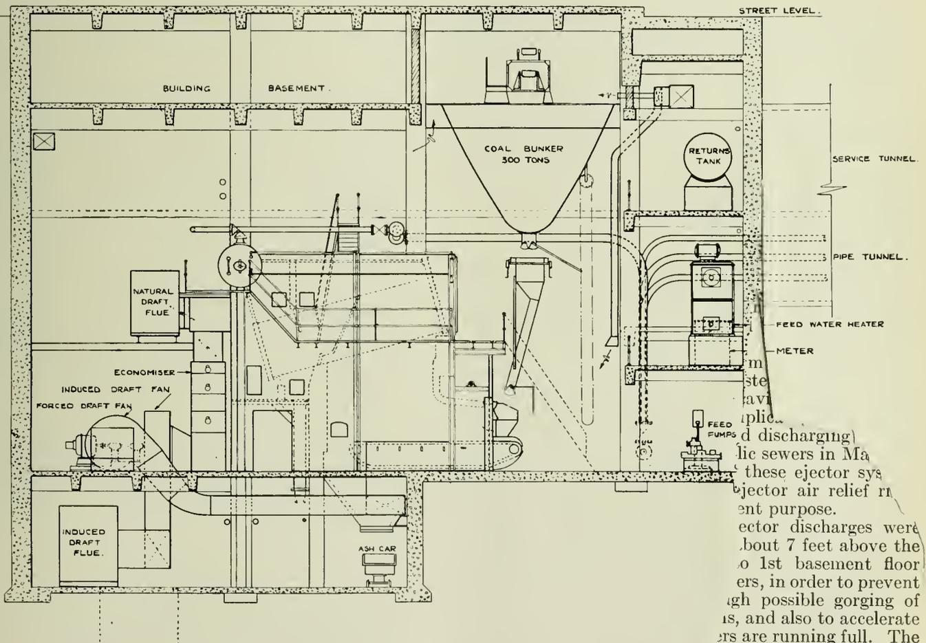
Fig. 2—Cross Section of Steam Station.
