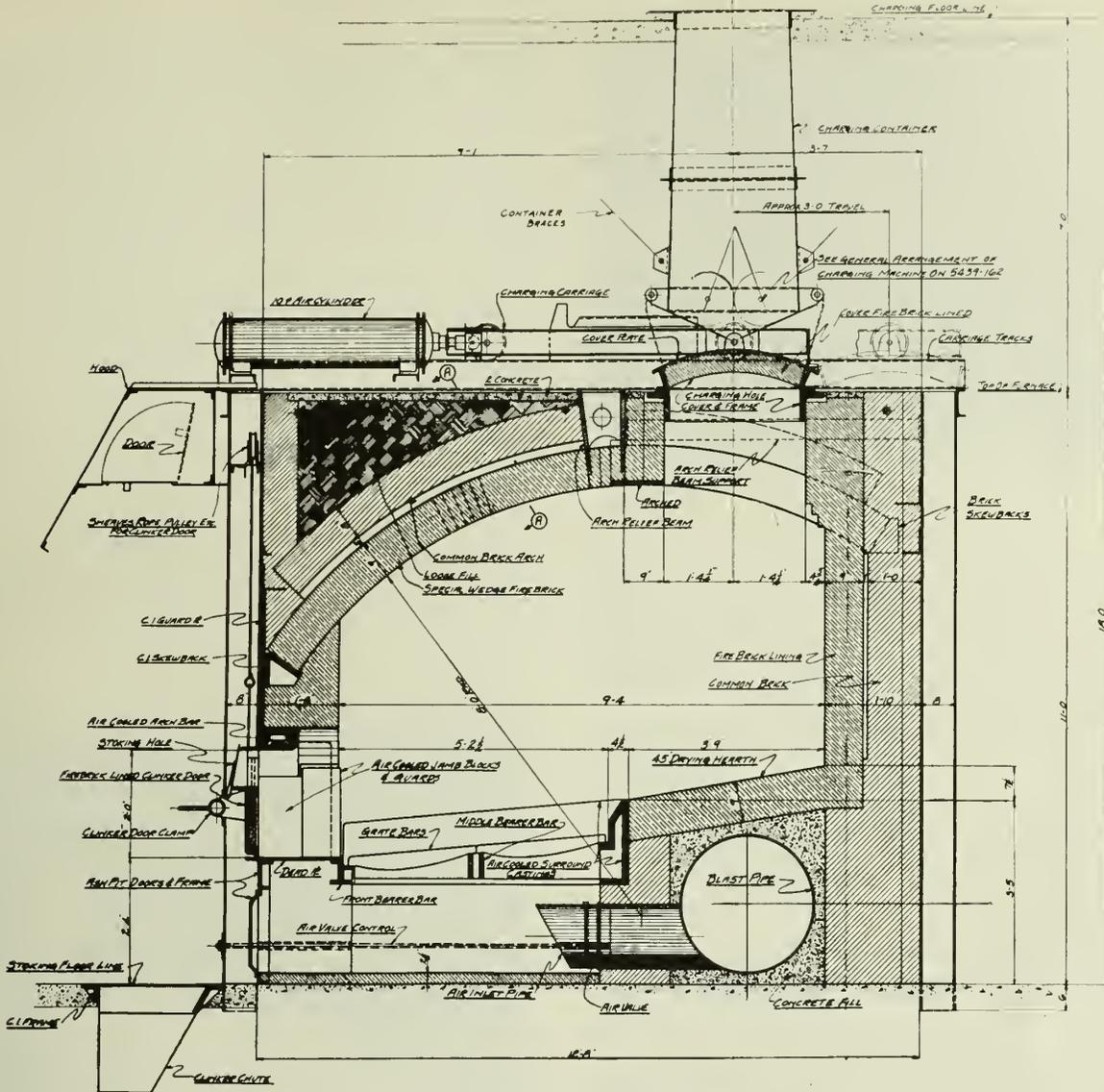
Fig. 4—Section Through Furnace.
