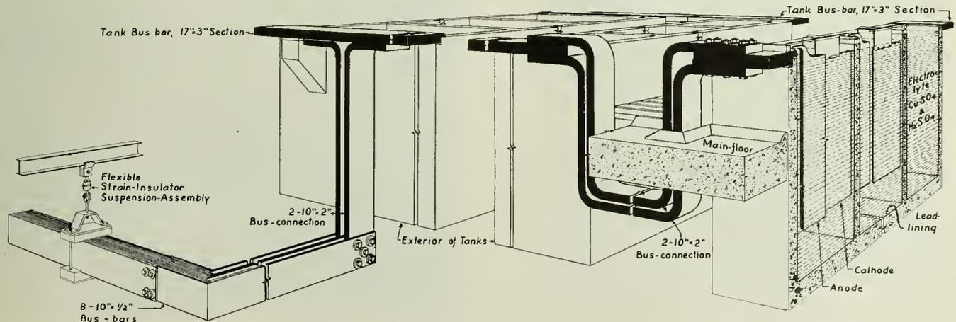
Fig. 4—Section Through Electrolytic Tanks.
