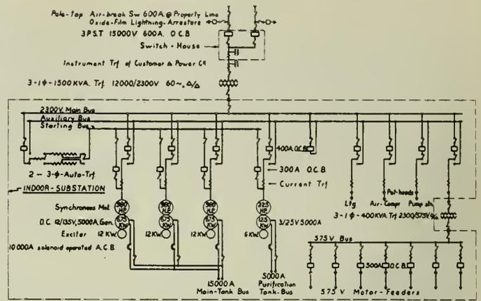
Fig. 6—Diagram of Switching and Circuit Arrangement.
