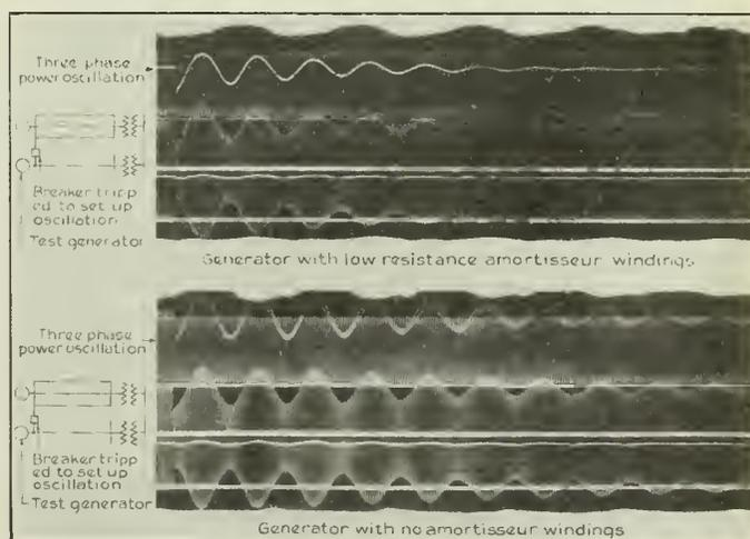
Fig. 26—Effect of Low-Resistance Amortisseur Windings in Damping out Three-Phase Oscillation.
