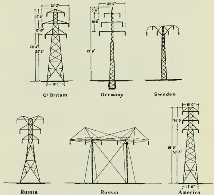
Fig. 4—Double-Circuit Towers.
