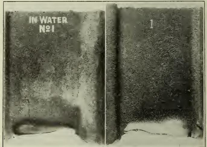
Fig. 8—Pile submerged at Nearly All Times. (a) Before Cleaning. (b) After Cleaning.
