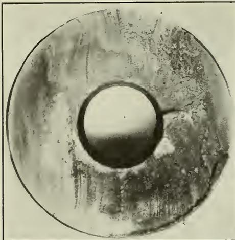
Fig. 6—Service Failure of Nickel Steel Crank Pin.
