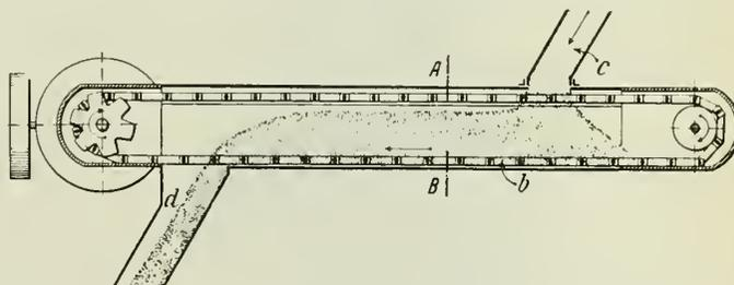
Fig. 9—Diagrammatic Section of Standard Redler Conveyor.
