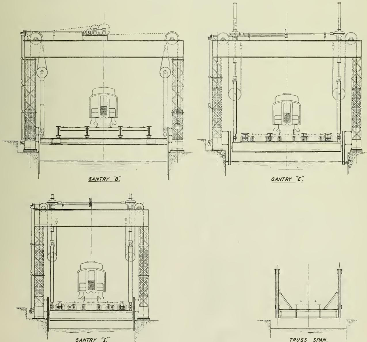
Fig. 6—Transverse Sections of Ferry Landing.
