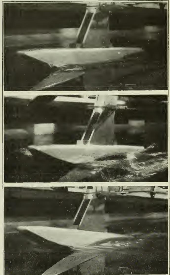
Fig. 8A—Test of Seaplane Float—Speed Three Feet per Second.
