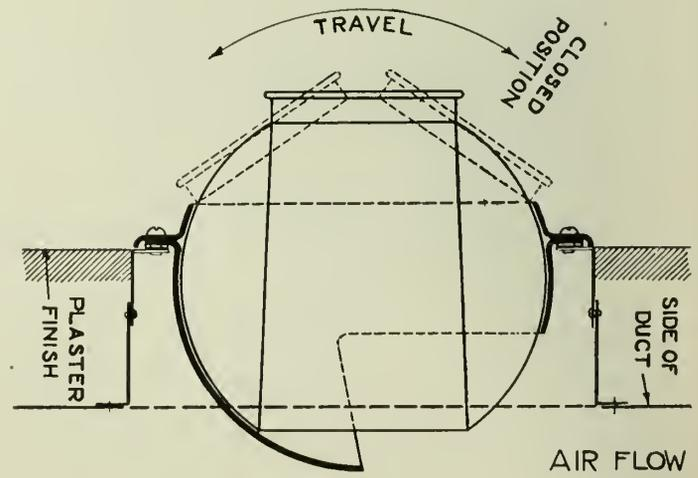
Fig. 6—“Punkah Louvre” type of Air Supply Unit.
