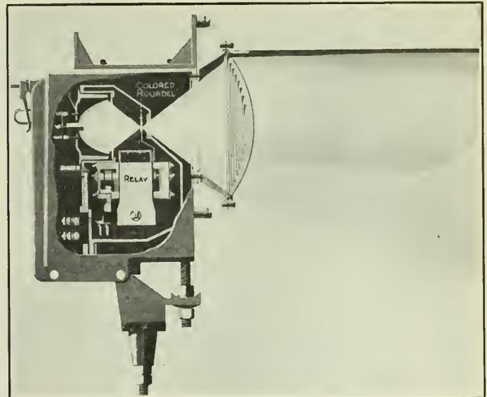
Fig. 5.—Searchlight Type of Colour Light Signal.
