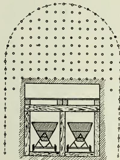
Fig. 5—Layout of Drill Holes in Heading.
