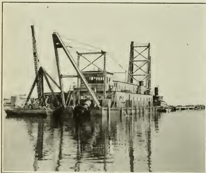
Fig. 7—Diesel Electric Suction Dredge "General Brock."
