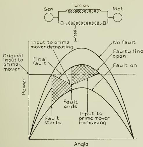
Fig. 15—Effect of Reducing Input to Prime Mover.
