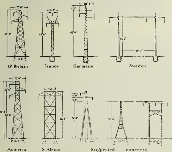
Fig. 3—Single-Circuit Towers.
