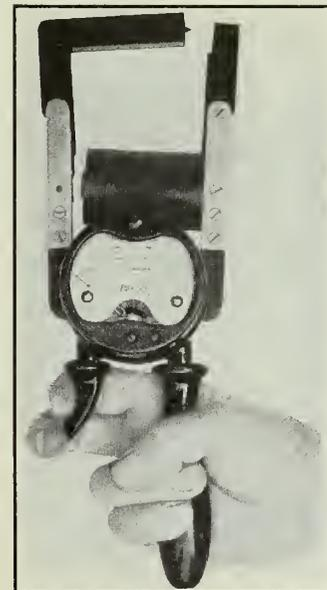
Fig. 6—Ferranti Clip-On-Ammeter.
