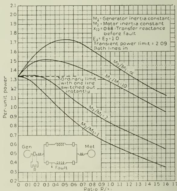
Fig. 28—Per-Unit Power that can be carried through the first Swing with instantaneous Switching using a Series Braking Resistor.
