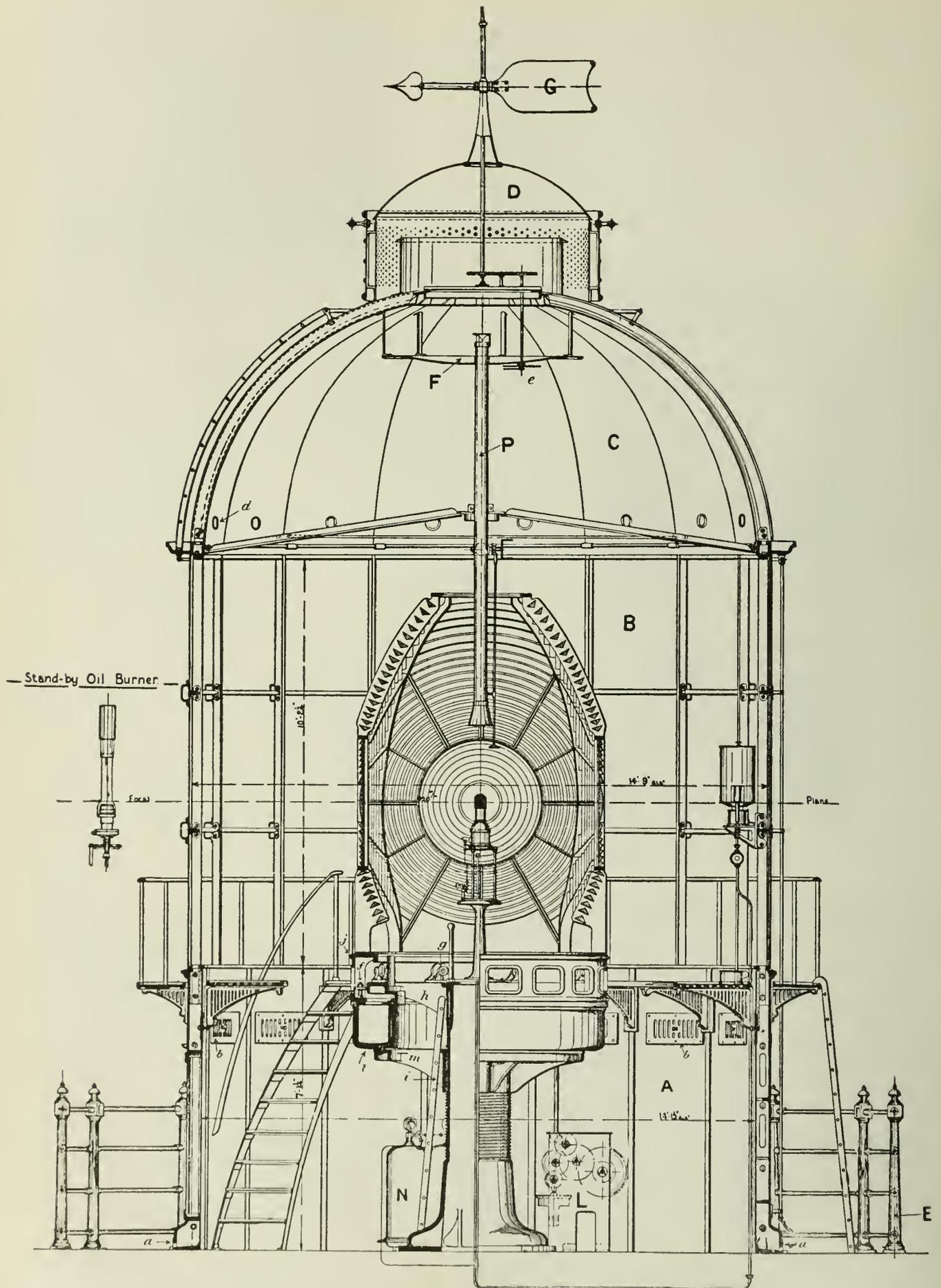
Fig. 10—General Arrangement of Lighthouse Lantern.
