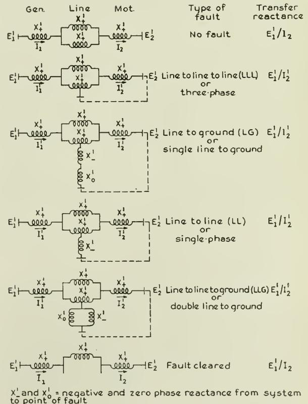
Fig. 12—Transfer Reactance Diagram.
