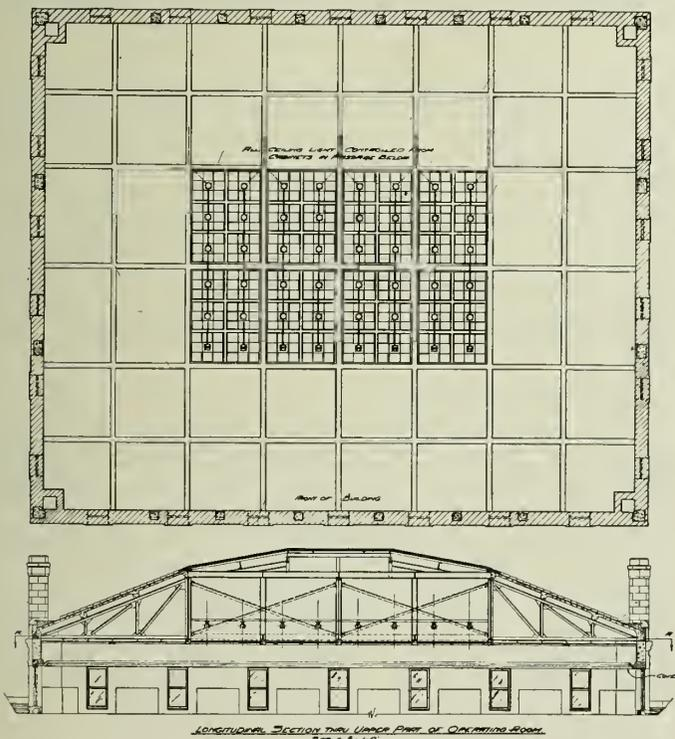
Fig. 5—Cove and Skylight Lighting System Operating Room.
