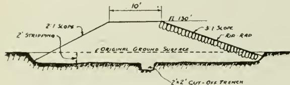
Fig. 11—Typical Section Through Earth Fill Dam.
