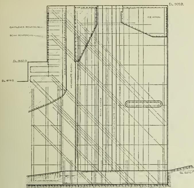
Fig. 5—Section Through Intake Showing Reinforcement.
