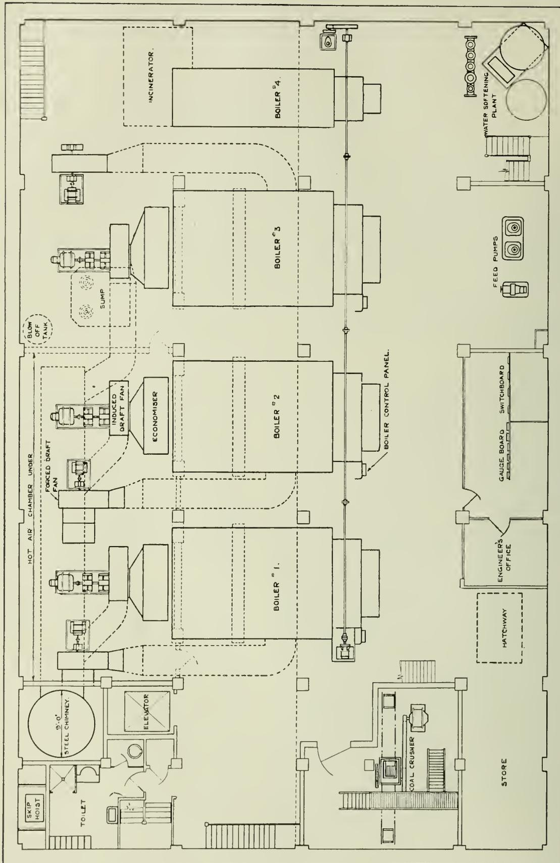
Fig. 1—Plan of Steam Station.
