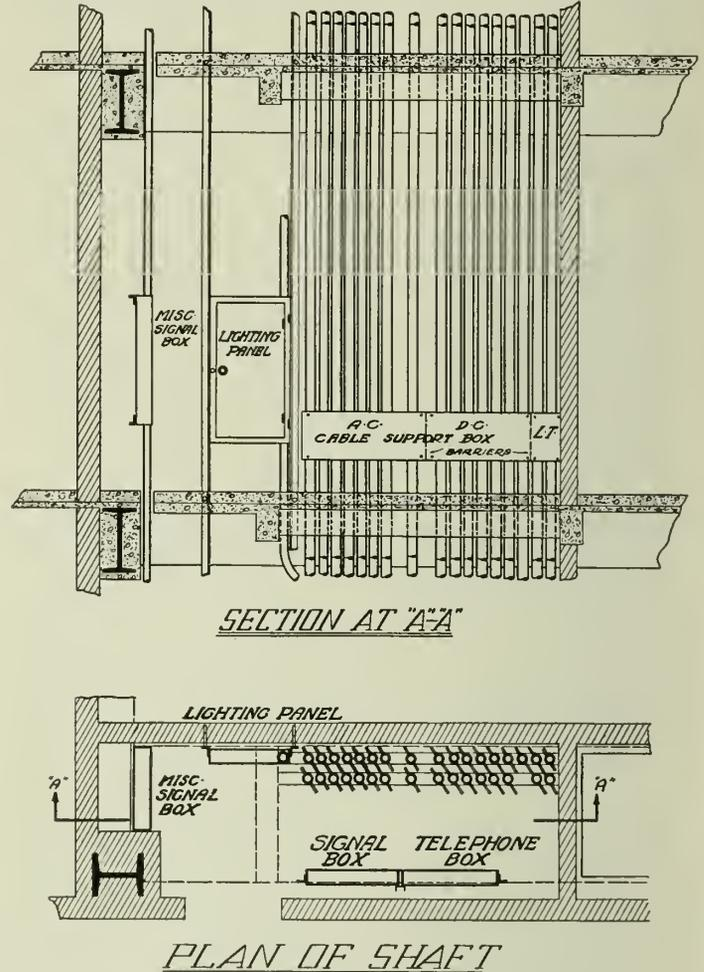
Fig. 7—Details of Typical Electric Riser Shaft.
