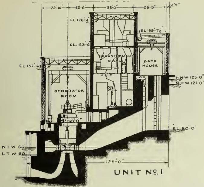
Fig. 8—Cross Section of Power House.
