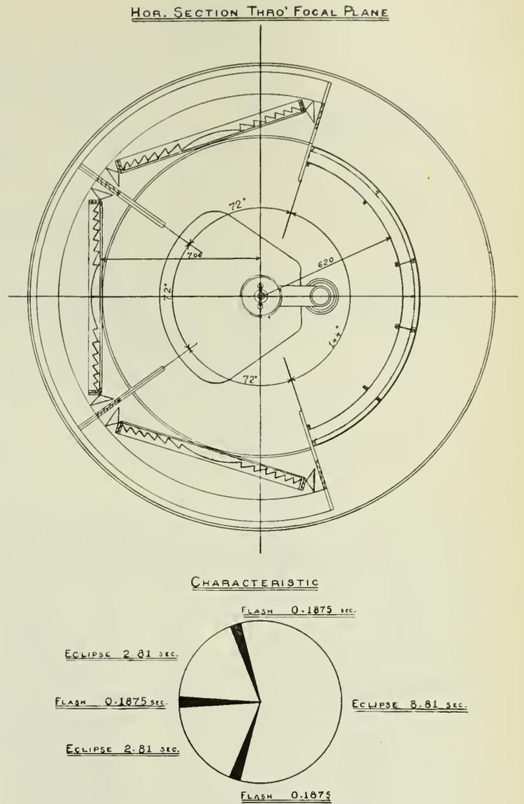
Fig. 8—Section of Second Order Flashing Light.
