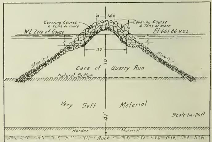
Fig. 4—Typical Section—Rubble Mound Breakwater.
