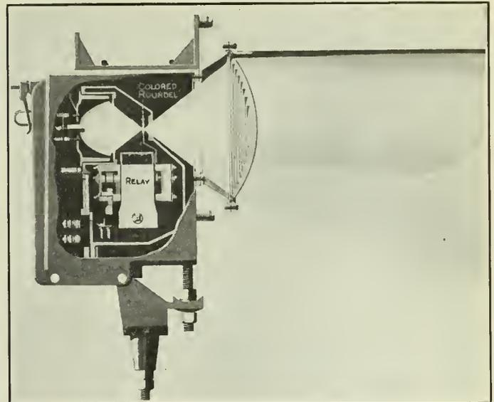
Fig. 5.—Searchlight Type of Colour Light Signal.
