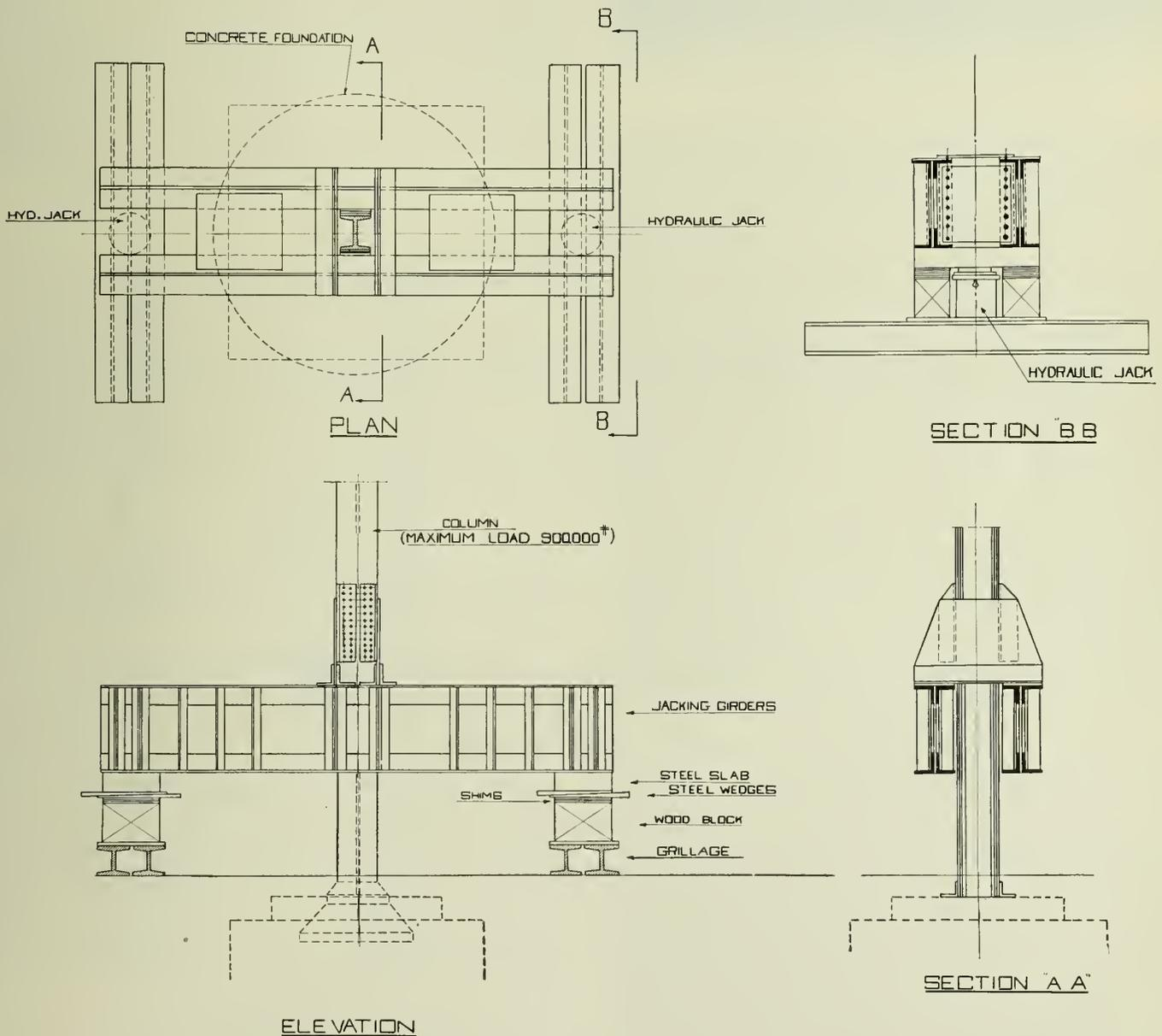
Fig. 13—Arrangement of Girders for lifting Existing Columns.
