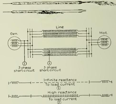
Fig. 11—Transfer Reactance During Three-Phase Faults.
