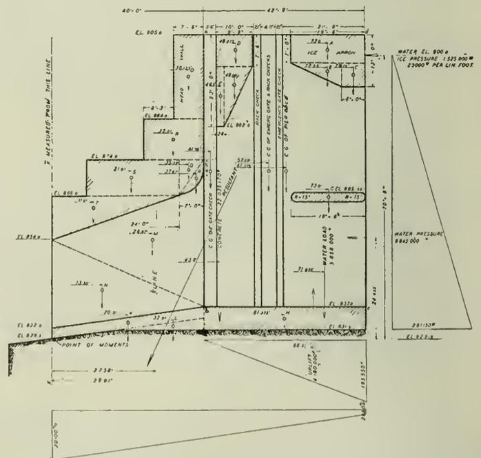
Fig. 4—Power House Stability Diagram.
