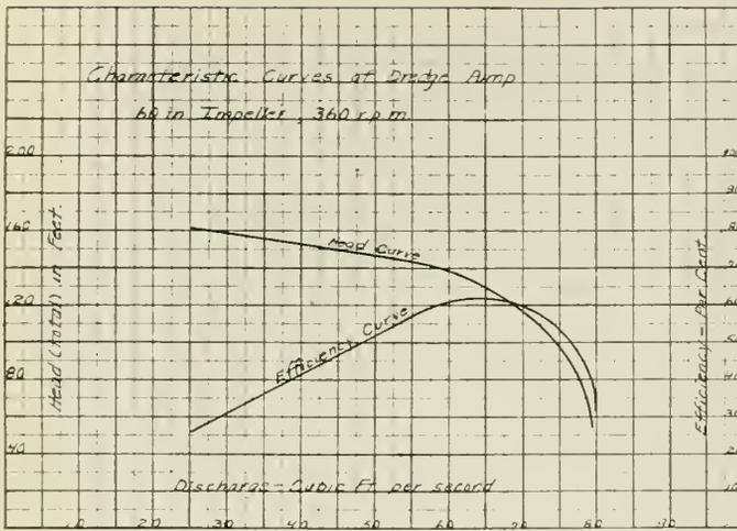
Fig. 1—Characteristic Curves of Dredge Pump.
