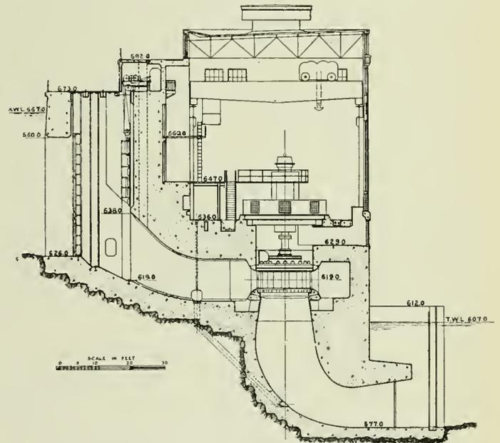
Fig. 10—Section through Power House.
