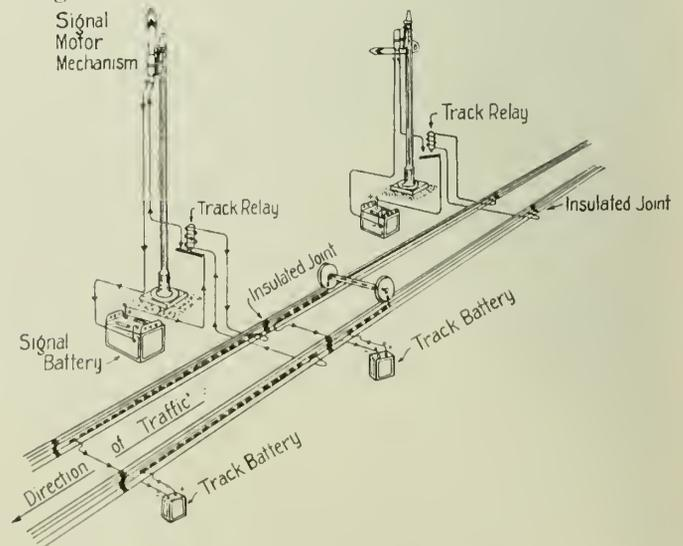
Fig. 2.—Track Circuit Signalling.
