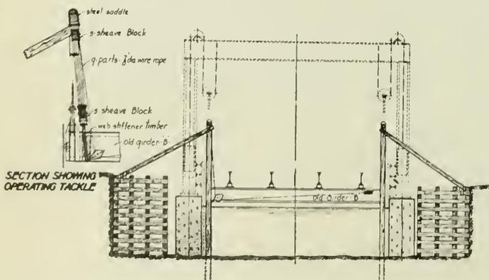
Fig. 18—Temporary Arrangement for Operating Apron at Gantry B.
