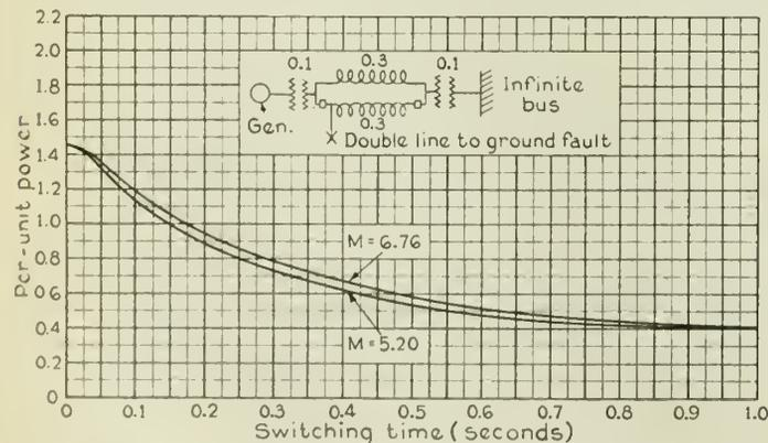
Fig. 18—Effect of Changing Generator  $WR^2$  30 per cent.
