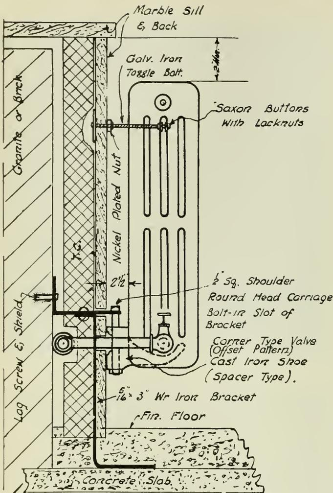
Fig. 1—Typical Detail of Radiator Supports, etc. Lower Zone.
