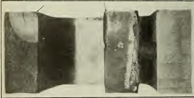
Fig. 9—Failure Caused by Weld.
