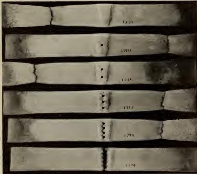
Fig. 4—Transverse Tension Test Specimens.
