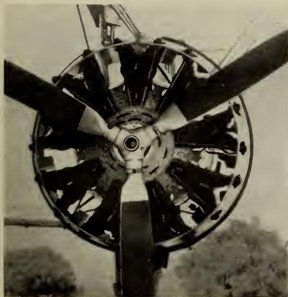
Fig. 2—Parkins' Pusher Engine Ring Cowling and Rocker Box Deflectors.
