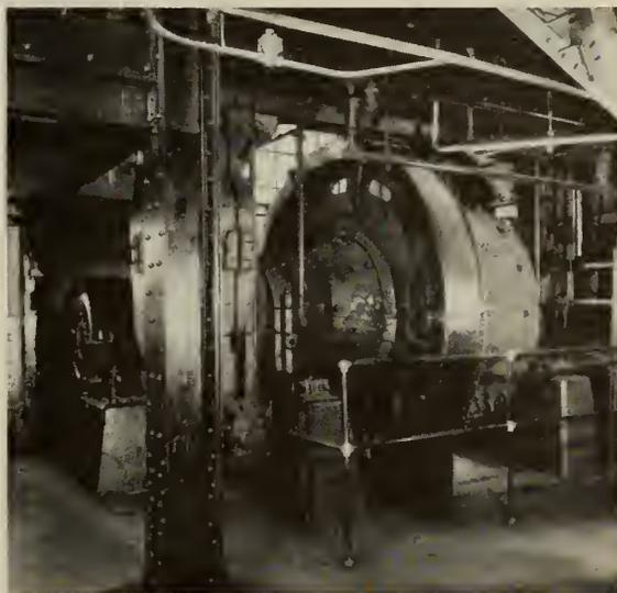
Fig. 2—Hardinge Ball Mill.
