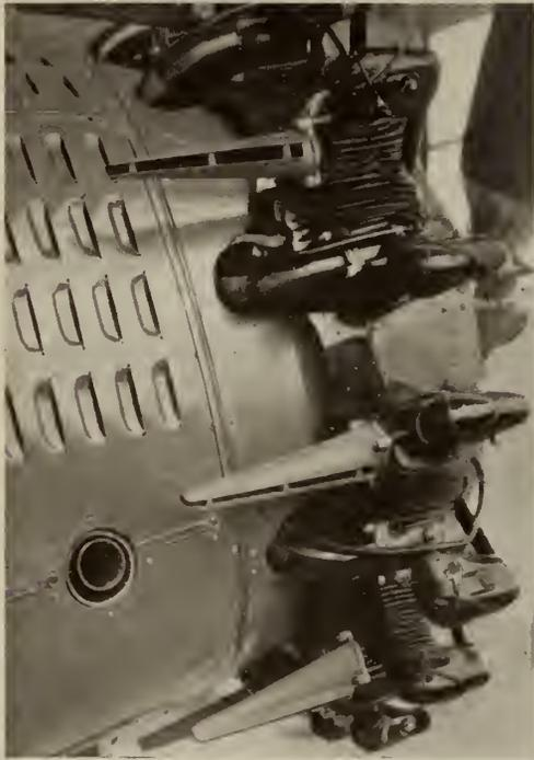
Fig. 4—Inter-Cylinder Deflectors to Improve Cooling on Supercharged Engine.
