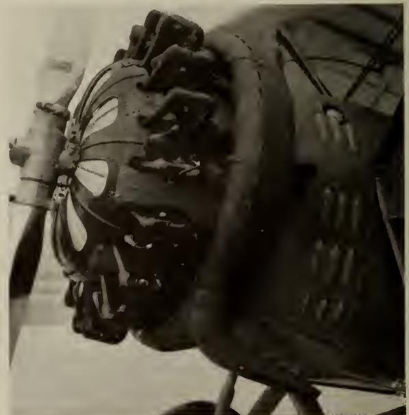
Fig. 1—Wasp Jr. Standard Engine Cowl and Exhaust Collector.
