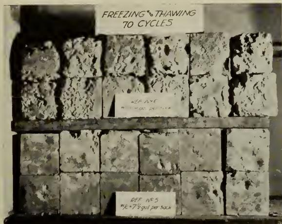
Fig. 4—Effect of Water-Cement Ratio on Resistance of Concrete to Freezing and Thawing.
