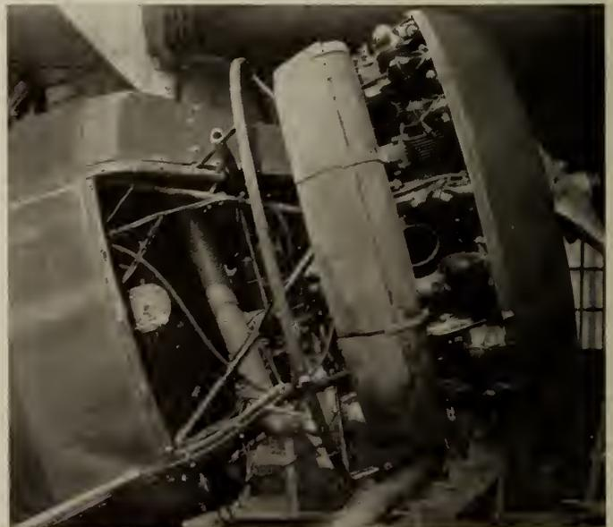
Fig. 5—Use of Streamline Shape Intercylinder Deflectors under N.A.C.A. Cowling. Wasp Jr. Engine in Stearman Mail Plane.
