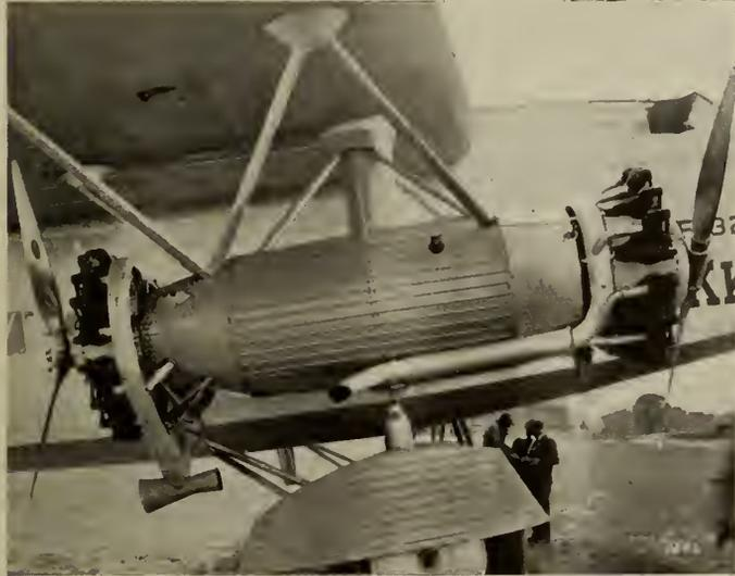
Fig. 6—Tandem Installation—Note Clean Cowling Lines Around Front Engine.
