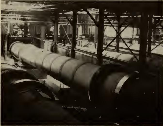
Fig. 2—General View of Rotary Lime Kilns taken from Intake End.
