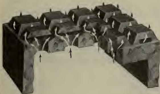
Fig. 6—Detail of Pyramid Grate.
