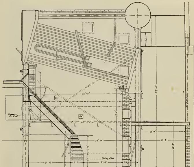
Fig. 5—Boiler Setting for Burning Wood or Coal.
