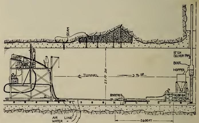
Fig. 8—Grouting Operations.
