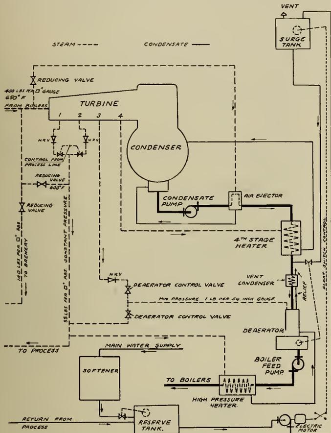
Fig. 7—Bled Steam and Feed Heating System—Monterrey Plant.
