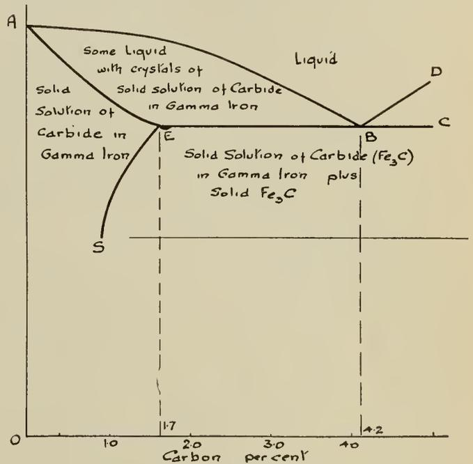
Fig. 10—Upper Portion of Simplified Iron-Iron Carbide Diagram.
