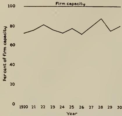
Fig. 6—Yearly Substation Load.
