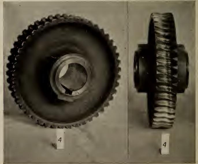
Fig. 14—Worm Gear after Test to Destruction, .4 inch c.p., 30-degree p.a. to Mate Single Thread Worm.
