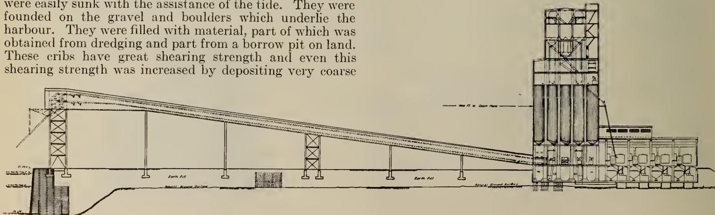
Fig. 12—Wharf, Conveyor Gallery, Workhouse and Track Shed.
