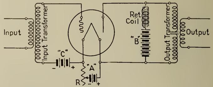
Fig. 3—Simple Amplifying Circuit.
