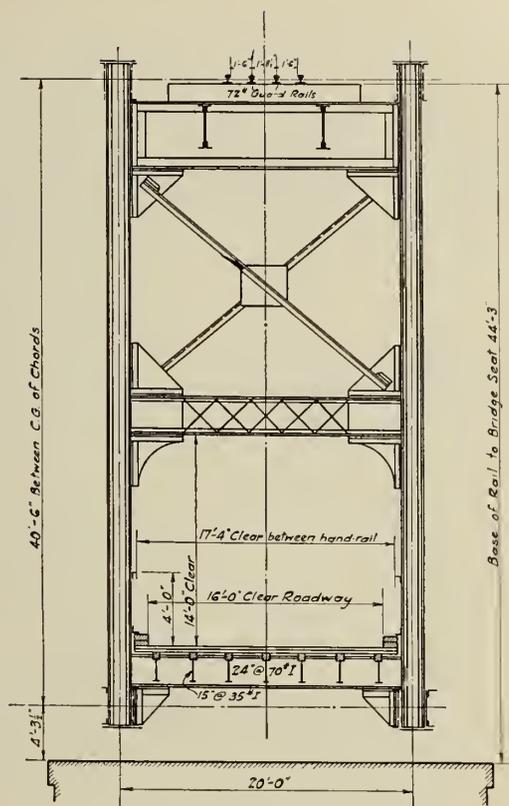
Fig. 7—Typical Section Through Deck Truss.
