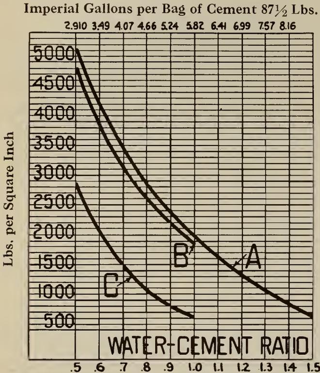
Fig. 7—Relative Compressive Strength of Concrete made with St'd. Portland Cement and Canada XXX H. E. S. Cement. A—Standard Portland Cement at 28 days. B—Canada XXX at 3 days. C—Canada XXX at 1 day.
