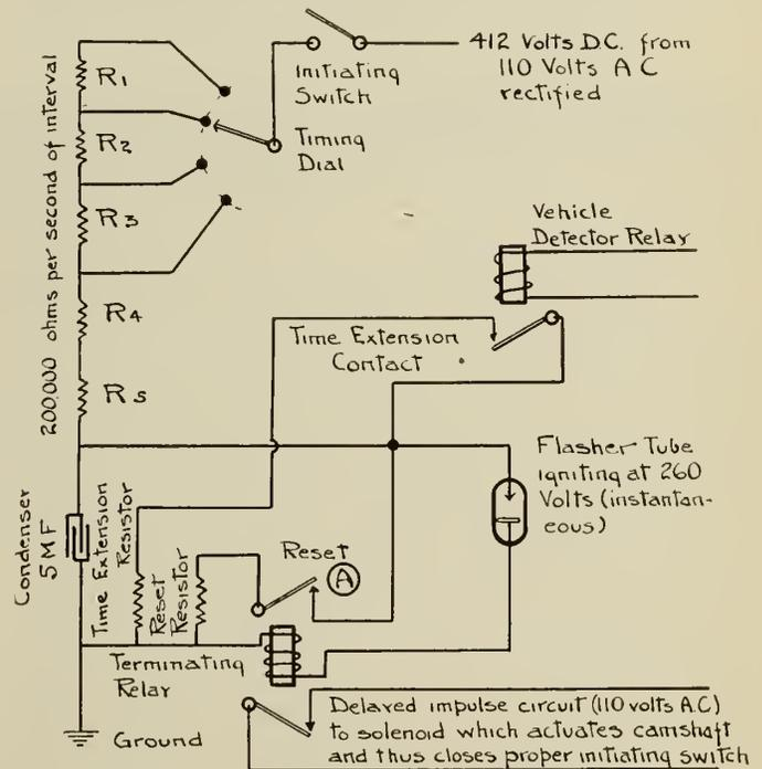
(A) For completing discharge of condenser at the end of each time interval— Really operated mechanically by solenoid—
