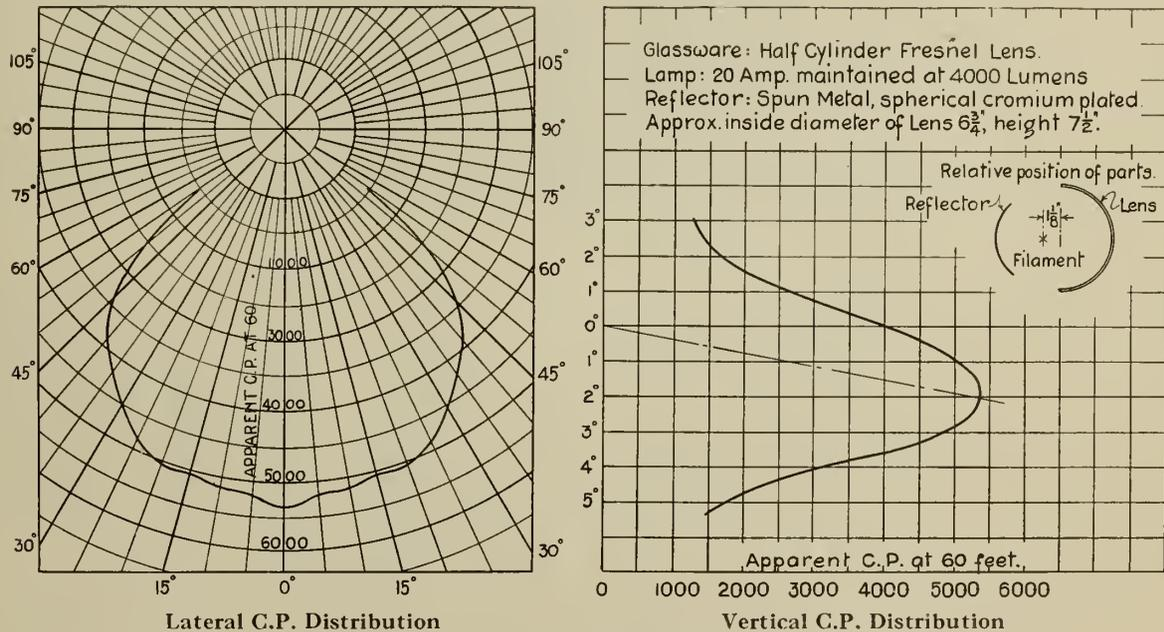
Fig. 14—Distribution Curves of the Prism Lighting Unit.
