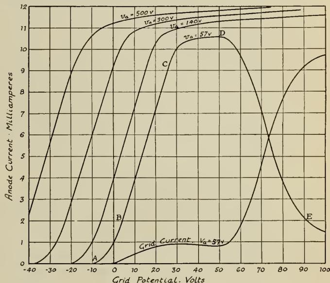
Fig. 9—Characteristic Curves of Typical High-Vacuum Triode.
