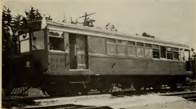
Fig. 1—Sperry Detector Car, Single Unit.
