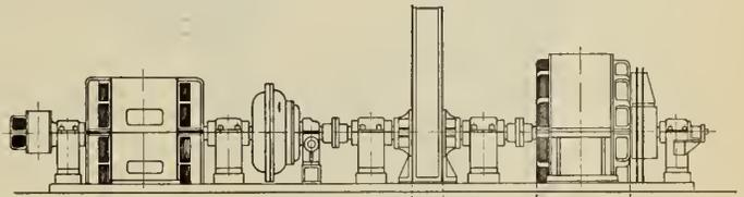
Arrangement of Motor Generator Flywheel Set.
