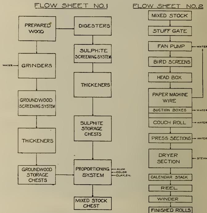
Fig. 1—Stock Flow Diagram for Paper Mill.
