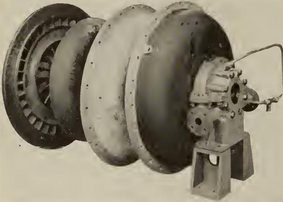
Fig. 5—Hydraulic Coupling, Expanded View.
