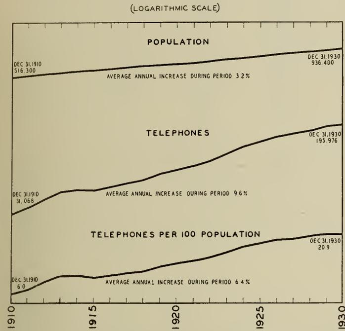
Fig. 8—Population Telephones and Telephone Development in Montreal Exchange Area 1910-1930.
