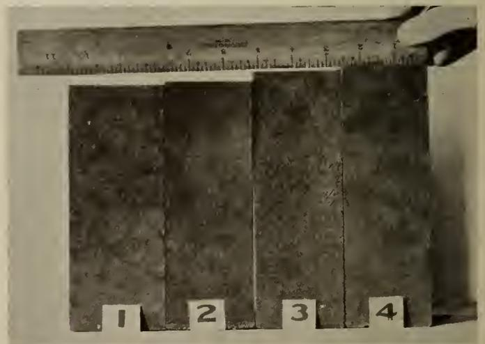
Fig. 4—Brick Showing Decreasing Shrinkage with Increase in Chromite Content from 0 to 30 per cent.
