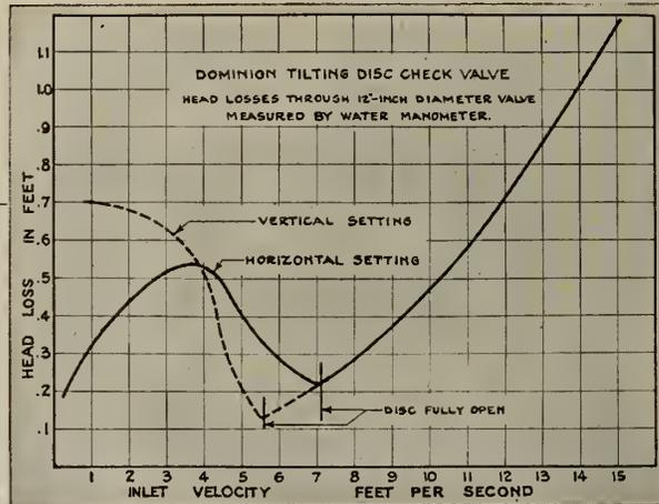
As indicated by the chart, this valve opens fully into line with the flow at moderate velocities, so eliminating disc oscillation and consequent wear at the disc trunnions. The low head loss shown is the result of true stream lining, i.e., no abrupt changes in the velocity or direction of the flow through the valve.
