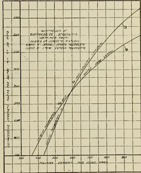
Fig. 14—Strength Curves, Gravel and Stone Concretes.
