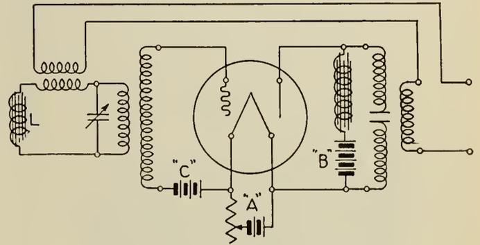
Fig. 6—Simple Vacuum Tube Oscillator.
