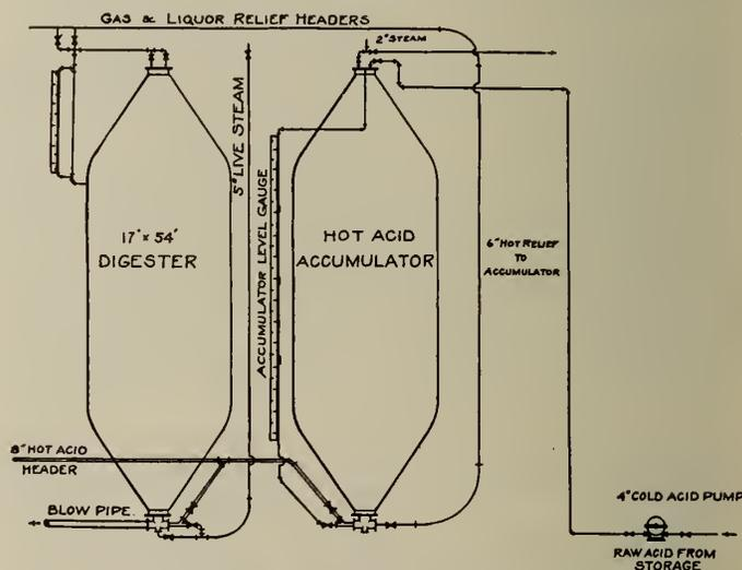
Fig. 3—Chemi-Pulp System for Sulphite Mill.
