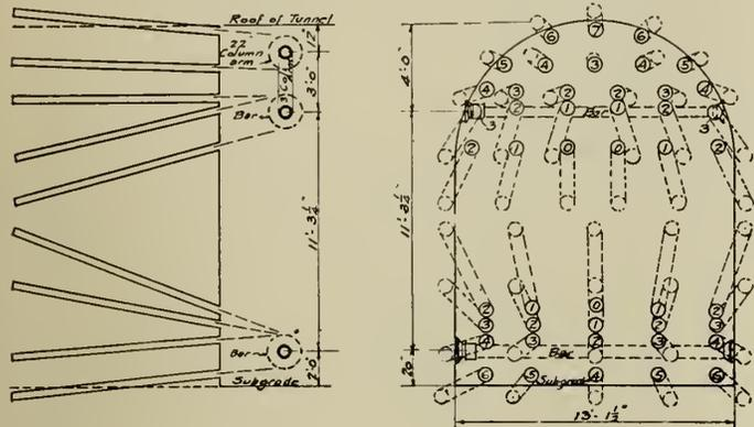
Fig. 7—Typical Full Face Round using Hammer Cut.
