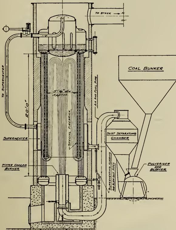
Fig. 1—Sectional View of Bettington Boiler, Waterford Lake Power Plant, 1912.
