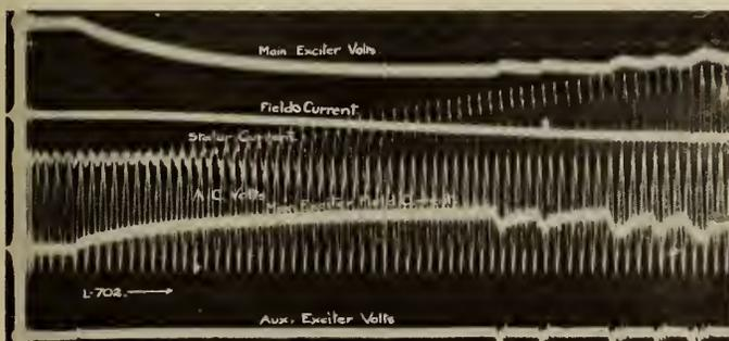
Fig. 4—Record from Test of Excitation Response.
