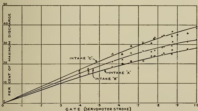
Fig. 9—Distribution of Discharge Between Supply Pipes.
