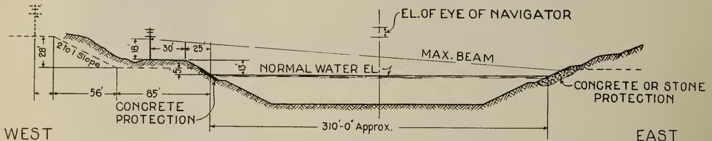
Fig. 13—Typical Cross Sections of Canal Looking North.
