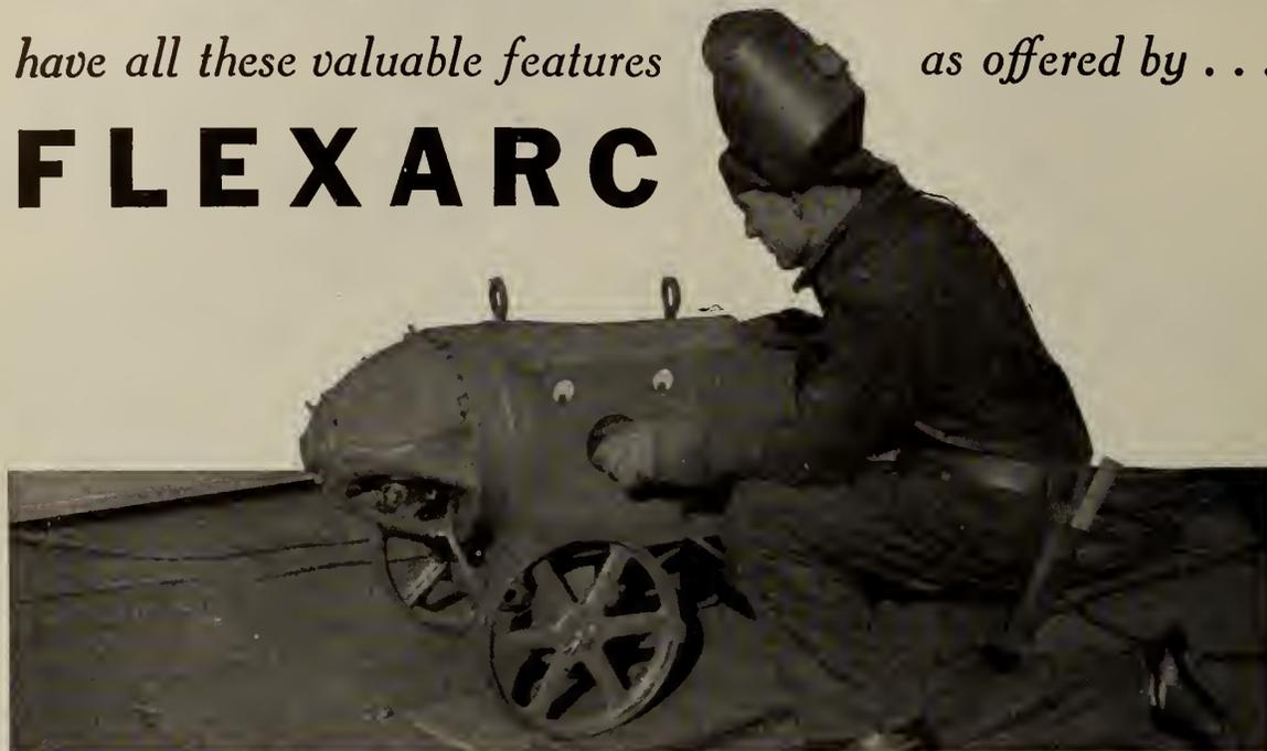
ANY DESIRED WELDING HEAT WITH SINGLE DIAL CONTROL. Changes in electrode sizes, material thicknesses, degree of "blow", class of welding, or degree of penetration, can be speedily matched in current value. No brushes to shift, no knife switches. Just turn one handy knob—a pointer indicates the welding current setting.
