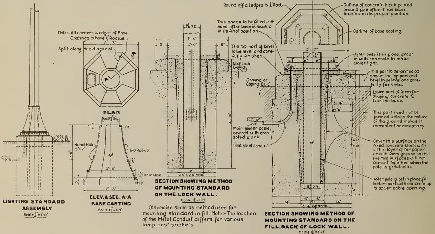
Fig. 7—Concrete Setting for Lighting Standard.
