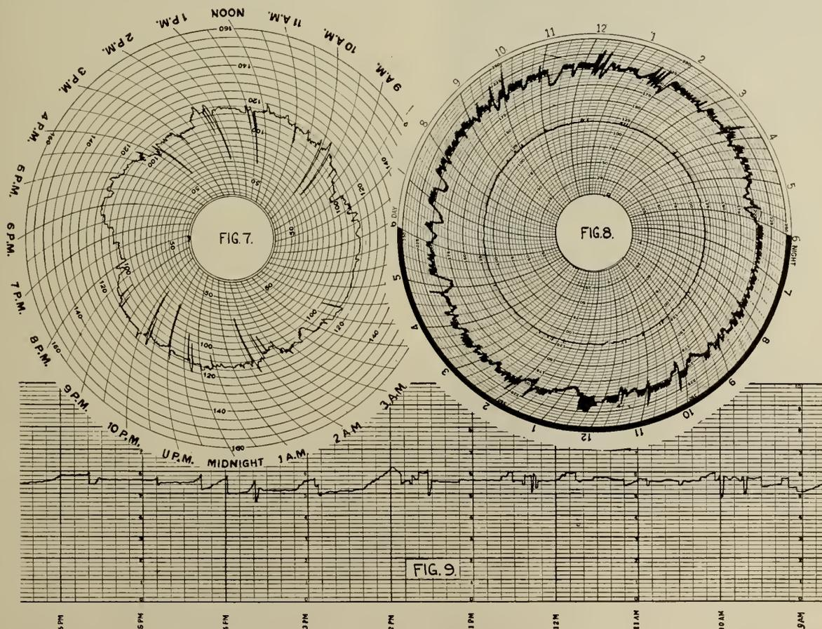
**Figs. 7, 8 and 9—Steam Flow and Corresponding Steam Pressure and Power-Input Charts obtained from Electric Boilers, equipped with Automatic Control.**
