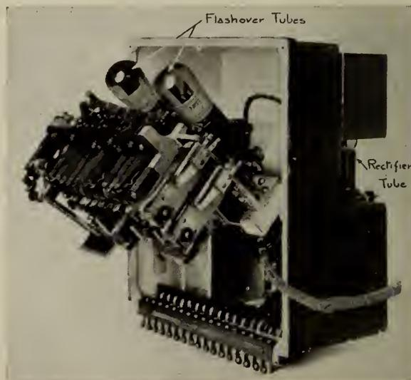
Fig. 5—Control Mechanism Showing Flasher Tubes.
