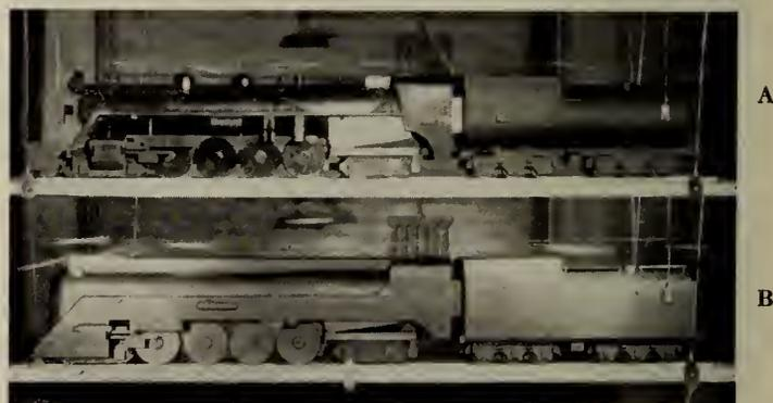
Fig. 11—Model Locomotives Set up in Wind Tunnel Illustrating Turbulent Air Flow.
