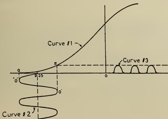
Fig. 5—Action of the Vacuum Tube as a Rectifier.
