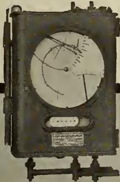
**INDICATE:** Steam Flow, Air Flow and Furnace Draft.
