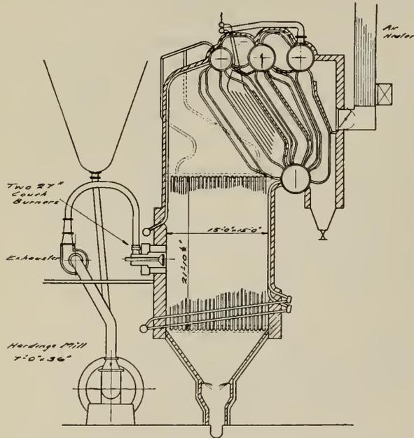
Fig. 3—900-h.p. Stirling Boiler, Seaboard Power Plant.
