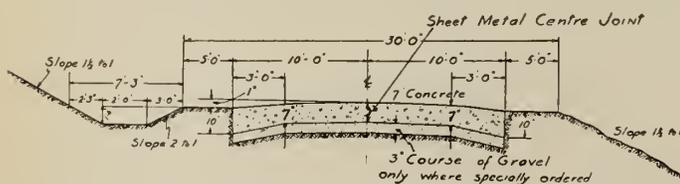
Fig. 3—Cross Section, Concrete Pavement, Ontario Provincial Highway Construction.
