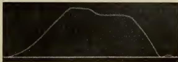
Fig. 9—Record of Timing Valve Stem Motion—with 7-inch injection tube; Injection Pressure, 8,000 pounds per square inch; Initial Injection Tube Pressure, 1,000 pounds per square inch.
