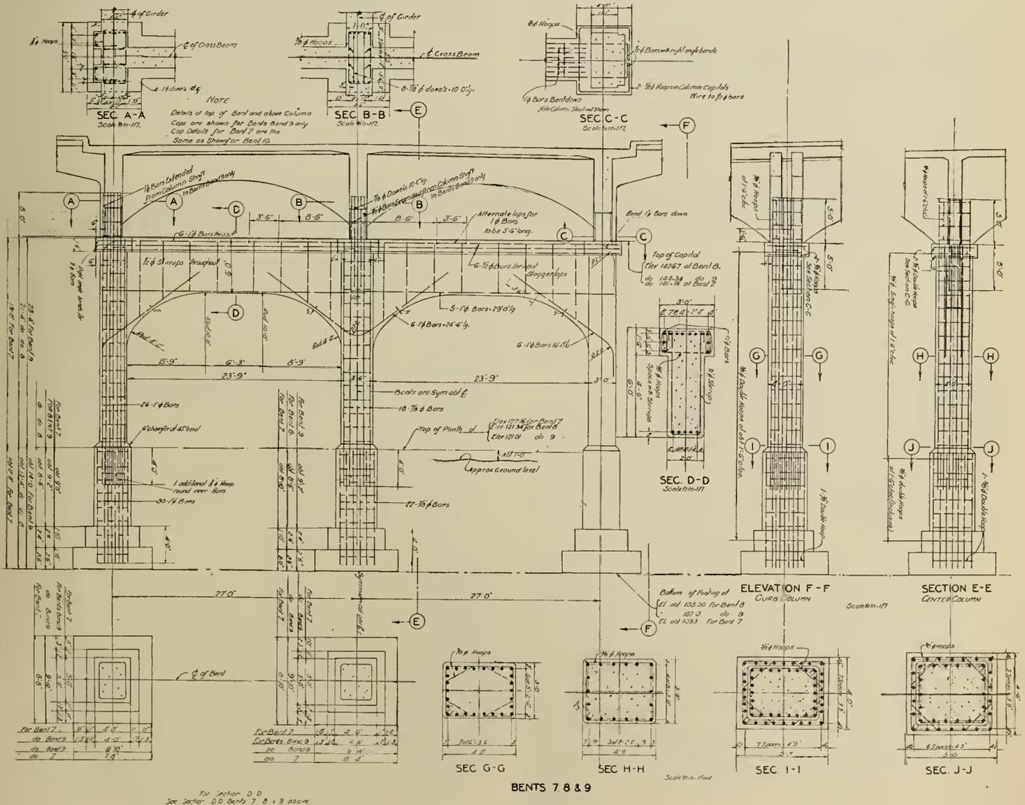
Fig. 6—Concrete Viaducts—Bents 7, 8 and 9.
