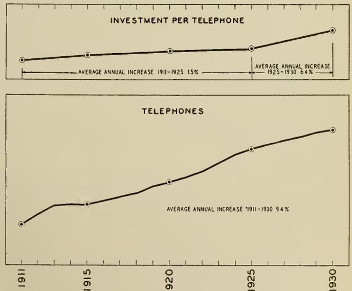
Fig. 9—Relative Rates of Increase in Telephones and Investment per Telephone in Montreal.
