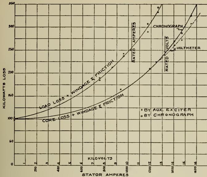
Fig. 2—Generator Losses Determined from Retardation Tests.
