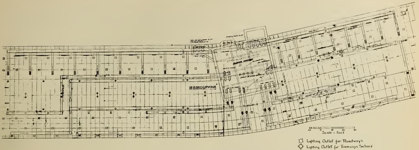
Fig. 6—Ventilation Plan of Portion of South Side.
