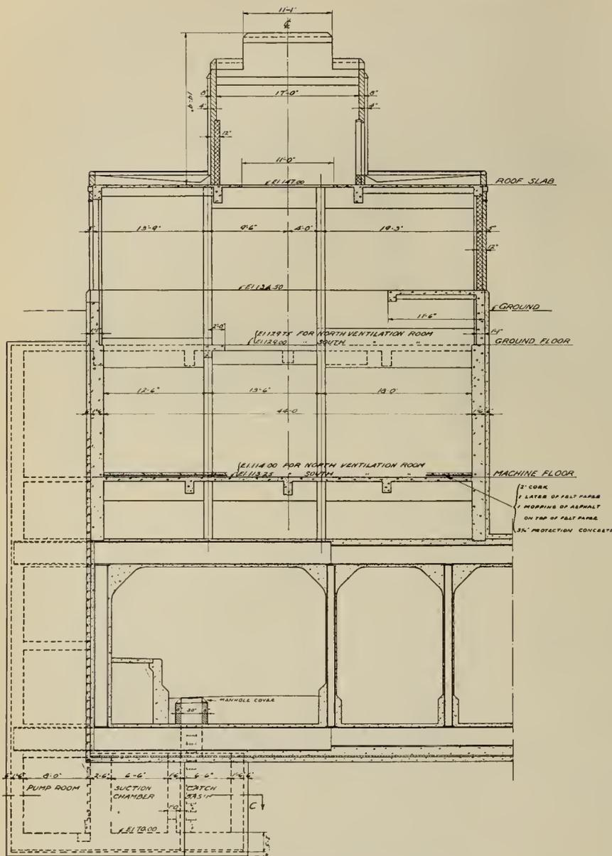
Fig. 5—Cross Section of Ventilation and Pump House.
