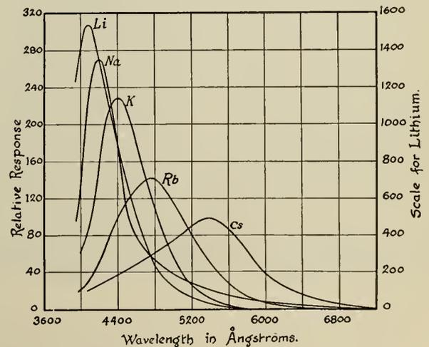
Fig. 2—Colour-Sensitivity Curves for Alkali Metals.
