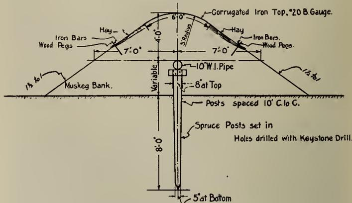
Fig. 13—Water Supply Pipe.
