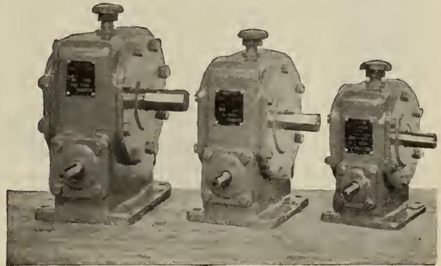
This new series of small worm units is priced so low that there is now no excuse for using inferior imported units. Delivery of the popular ratios is from stock. The low price is due to production economies, for they are of the highest grade. They have ball bearings, glass hard nickel steel worms, phosphor bronze gears and oil seals on both shafts.
