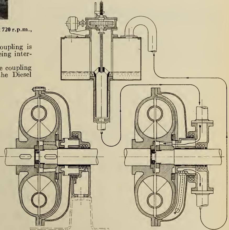
Fig. 4—Scoop Tube Type with Weir-Tank Control.
