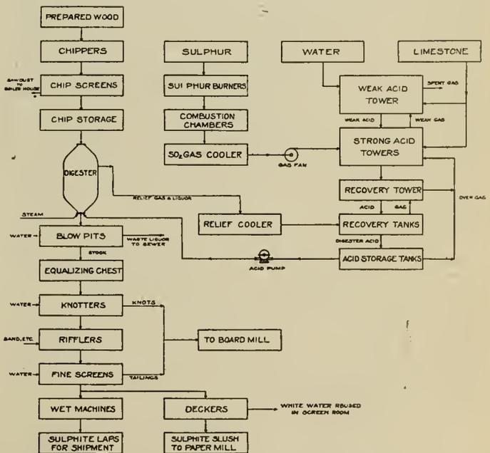
Fig. 2—Stock Flow Diagram for Sulphite Mill.
