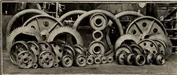
Machine cut Gears manufactured in our Plant.
