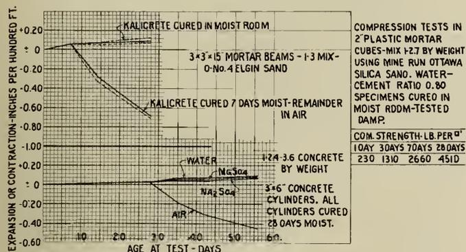
Fig. 11—Comparison of Expansion in Air-Water-MgSO<sub>4</sub> and Na<sub>2</sub>SO<sub>4</sub> Solutions on Sample of Kalicrete\*.
