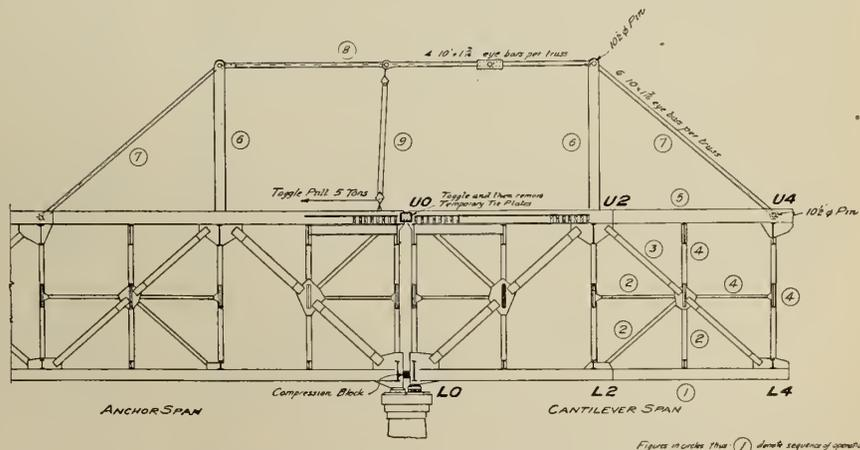
Fig. 8—Temporary Harness for Cantilever Erection.
