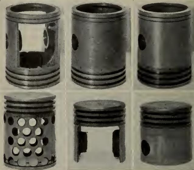
Fig. 2—Various Forms of experimental Pistons.
