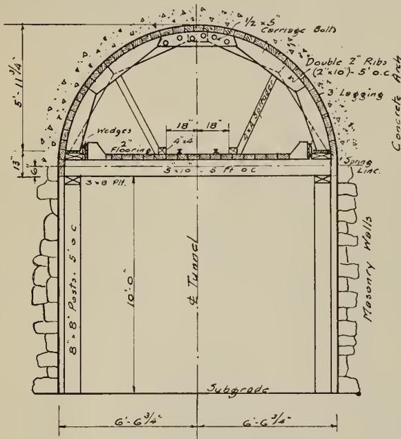
Fig. 9—Tunnel Form used in Pouring Concrete Arch.
