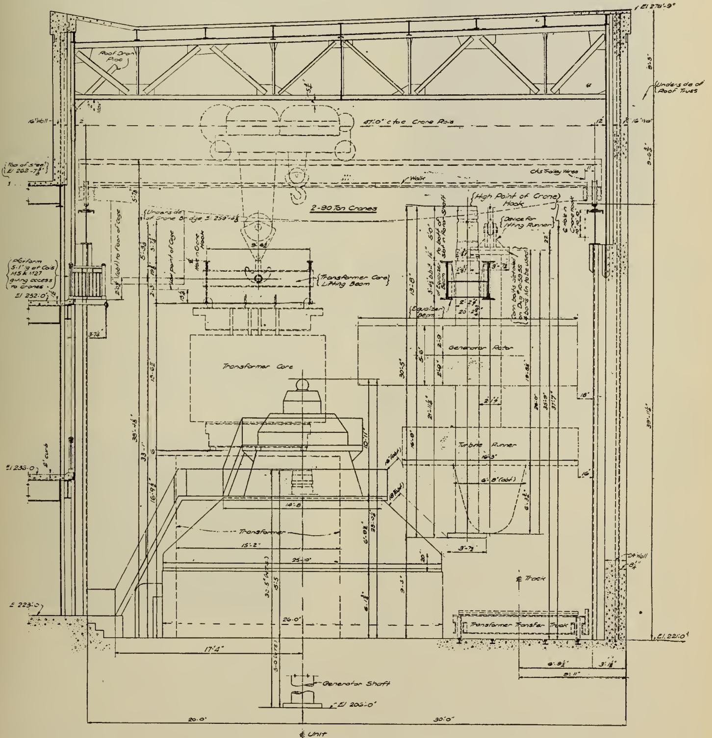
Fig. 5—Power House Assembly Clearances.
