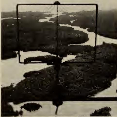
Fig. 4—Navigator's Guide for Use in Flight.
