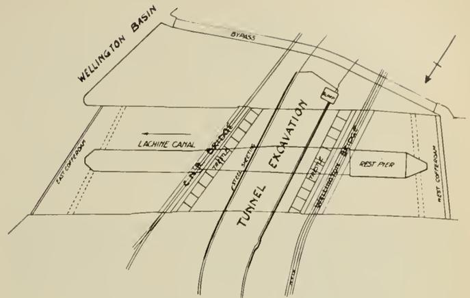
Fig. 9—Location of Cofferdams and By-Pass.
