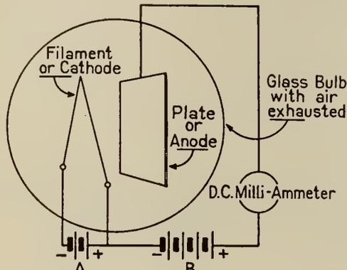
Fig. 1—Two-Electrode Vacuum Tube.
