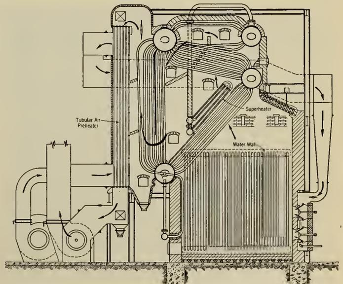
Fig. 8—Steam Generator—Monterrey Plant.
