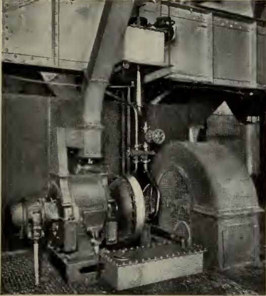
Fig. 3—Vulcan-Sinclair Hydraulic Coupling, 65 h.p. at 720 r.p.m., Driving Forced Draught Fan.
