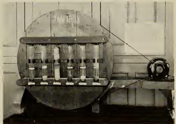
Fig. 4—Merriman Wheel for Sugar Lime Test.
