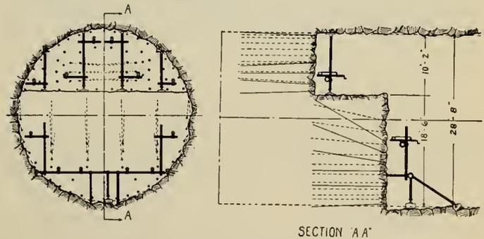
Fig. 3—Top Heading and Bench.
