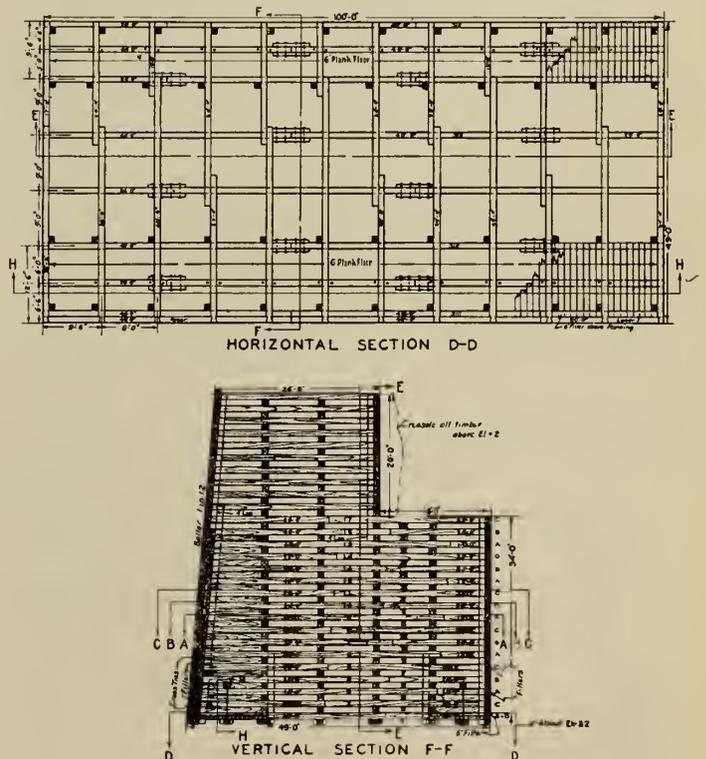
Fig. 11—Deep Water Crib for Permanent Dock, Churchill.
