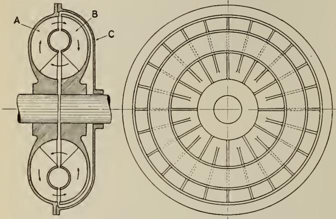
Fig. 1—Elementary Hydraulic Coupling.
