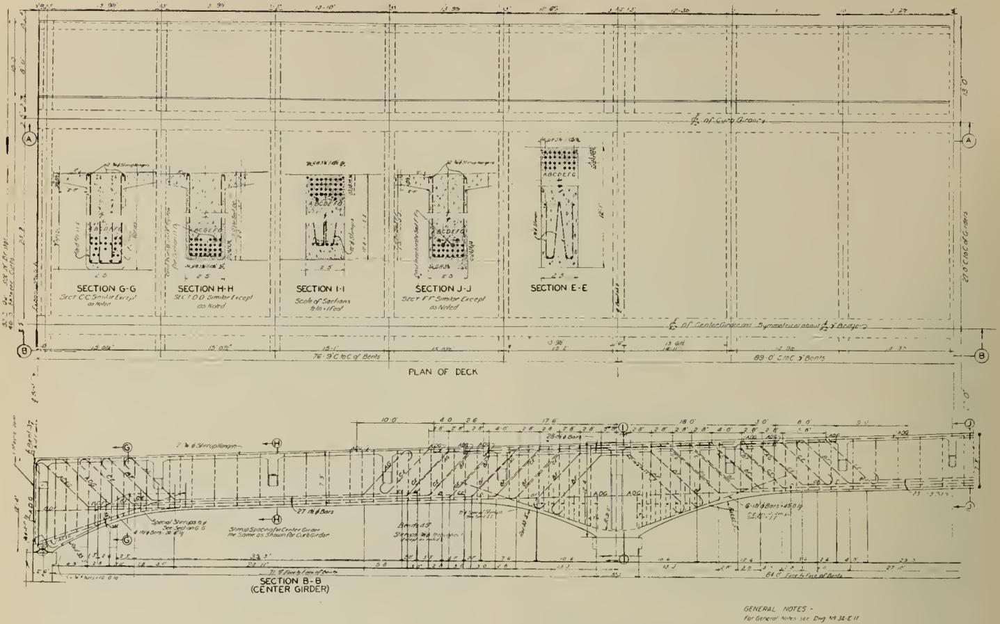
Fig. 5—Concrete Viaduct—Typical Centre Girder and Deck.
