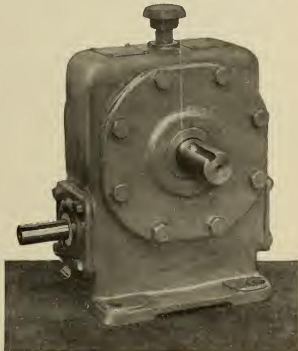
This new series of small worm units is priced so low that there is now no excuse for using inferior imported units. Delivery of the popular ratios is from stock. The low price is due to production economies, for they are of the highest grade. They have ball bearings, glass hard nickel steel worms, phosphor bronze gears and oil seals on both shafts.
