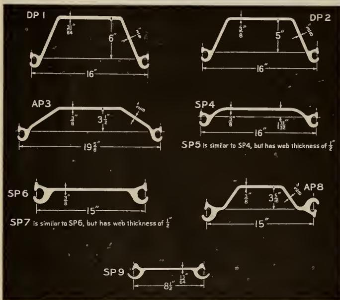
*A Section to cope with any condition*
