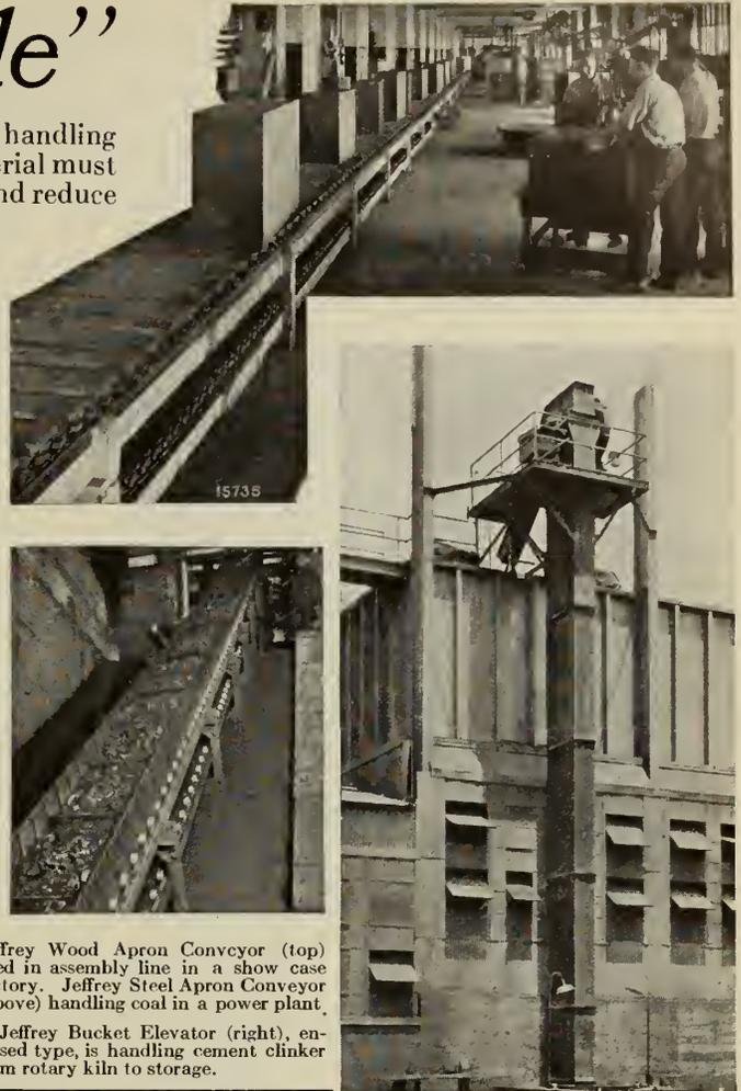
Jeffrey Wood Apron Conveyor (top) used in assembly line in a show case factory. Jeffrey Steel Apron Conveyor (above) handling coal in a power plant.
