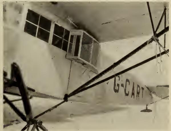
Fig. 3—Navigator's Compartment Replacing Standard Door.
