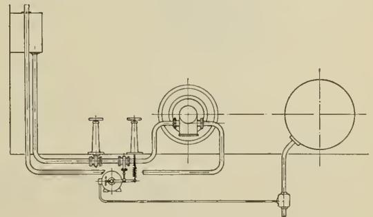
Arrangement of Slip Regulator Gear.
