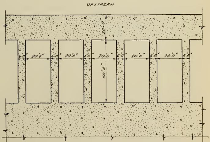
Fig. 3—Foundation Plan of Intake showing Voids.
