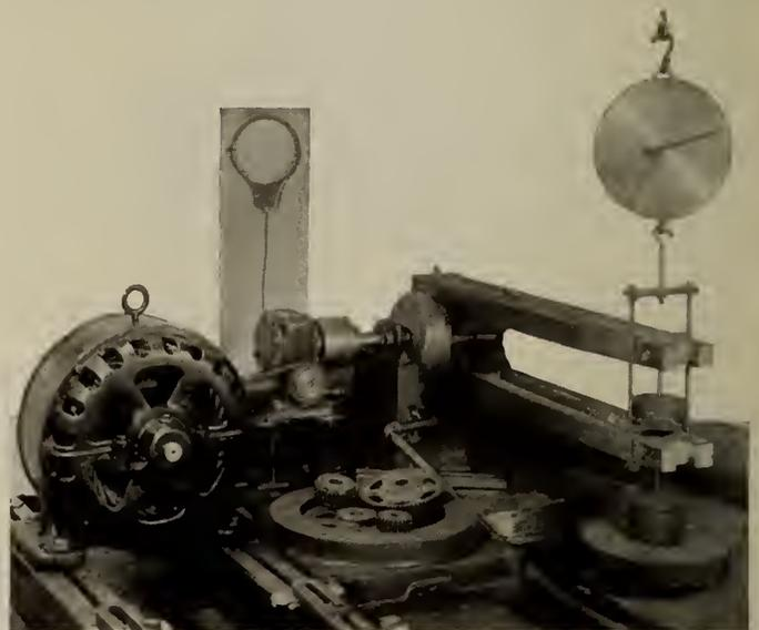
Fig. 2—Set up of Apparatus for Brake Test.
