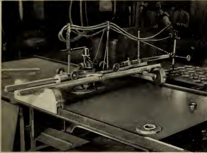
Fig. 4—Stationary Automatic Cutting Machine.
