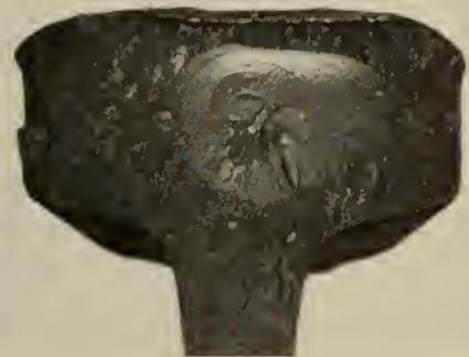
Fig. 3—Transverse Fissure—Area of Fissure approximately 23 Per Cent of Rail head.
