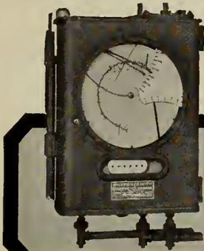
**INDICATE:** Steam Flow, Air Flow and Furnace Draft.
