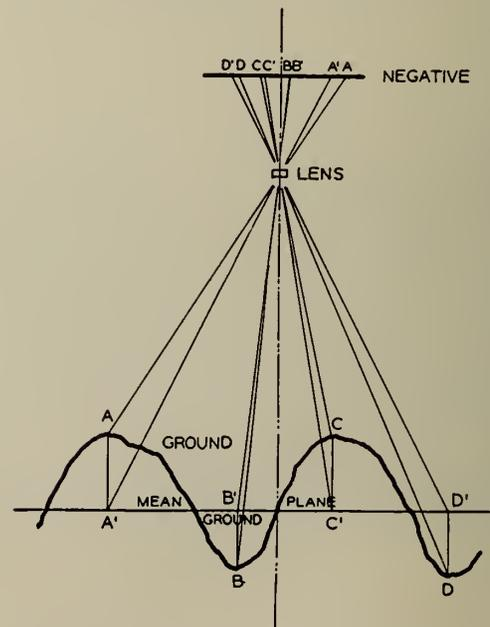
Fig. 5—Displacements Due to Change in Ground Elevation.
