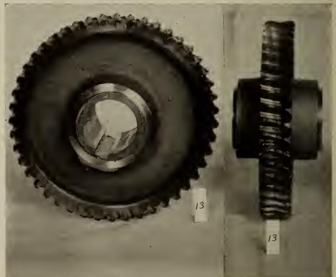
Fig. 13—Worm Gear after Test to Destruction, .4 inch c.p., 30-degree p.a. to Mate Double Thread Worm.
