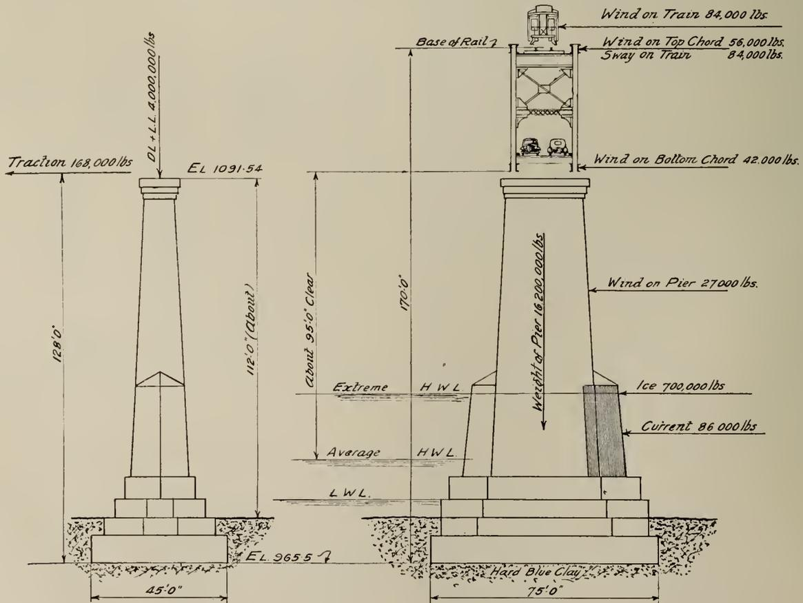
Fig. 4—External Forces Acting on High Piers.
