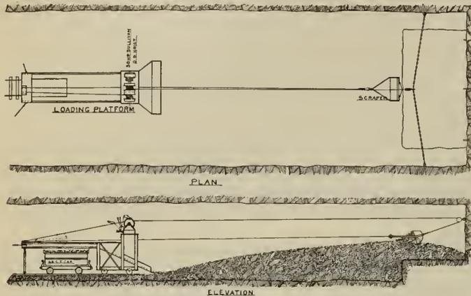
Fig. 4—Mucking Machine in Operation.
