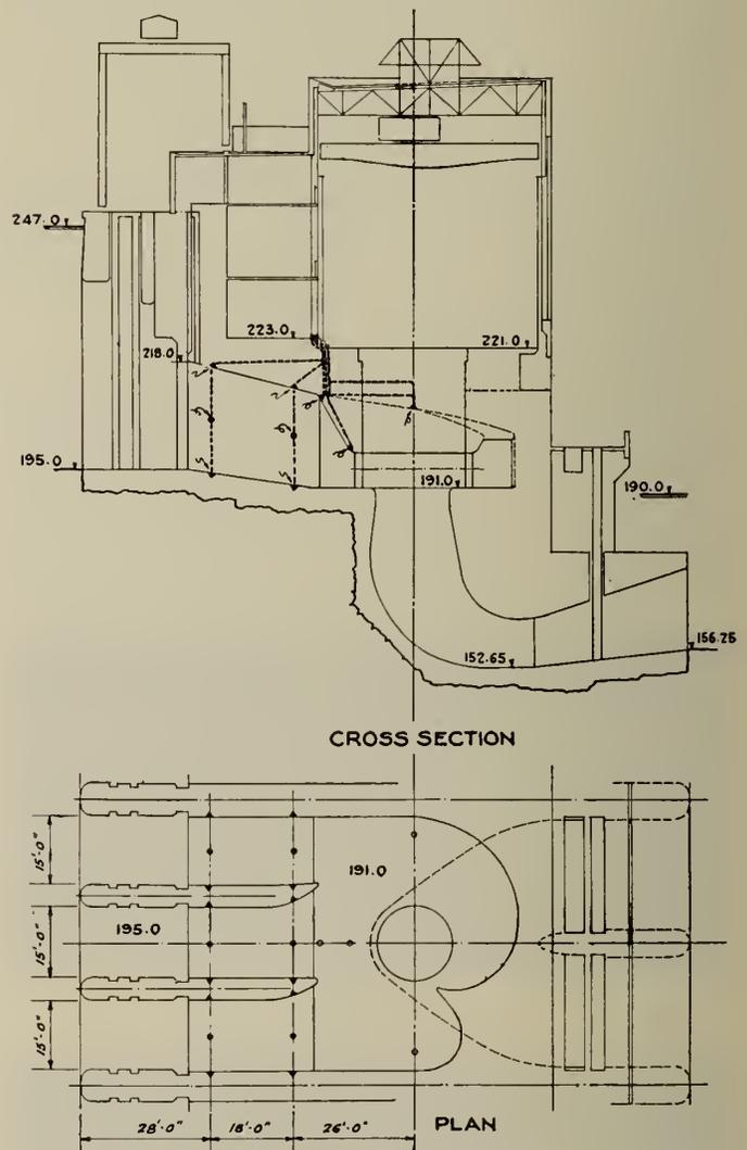
Fig. 7—Piezometer Opening and Piping for Gibson Tests.
