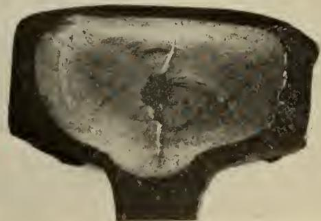
Fig. 4—Transverse Fissure—Area of Fissure approximately 80 Per Cent of Rail head.
