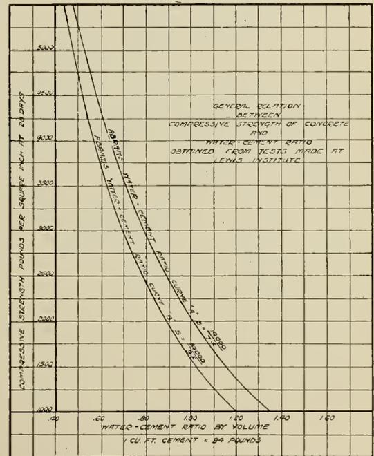
Fig. 11—Portland Cement Association Strength-Water-Cement Ratio Relation.
