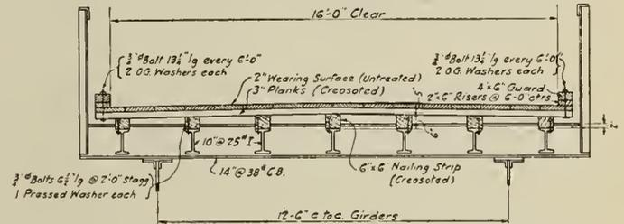
Fig. 11—Typical Section Through Roadway Approaches.
