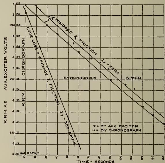
Fig. 1—Typical Retardation Curves.
