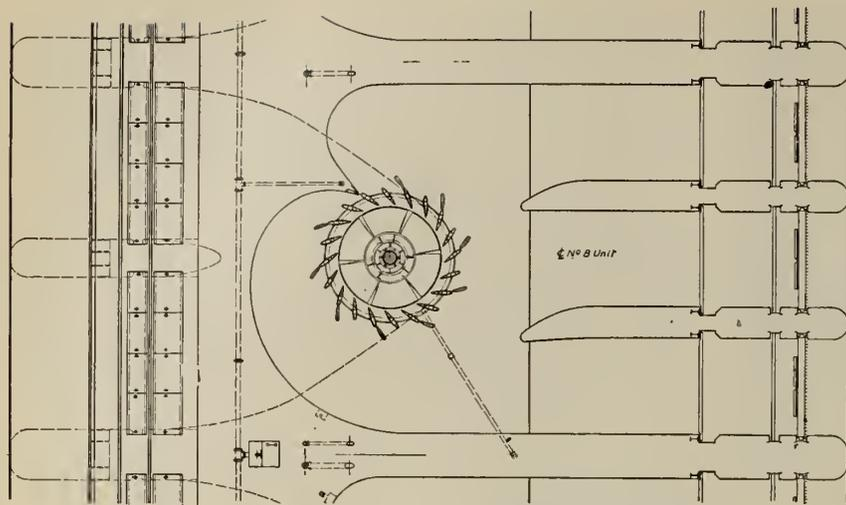
Fig. 8—Sectional Plan of Unit through Water Passages.
