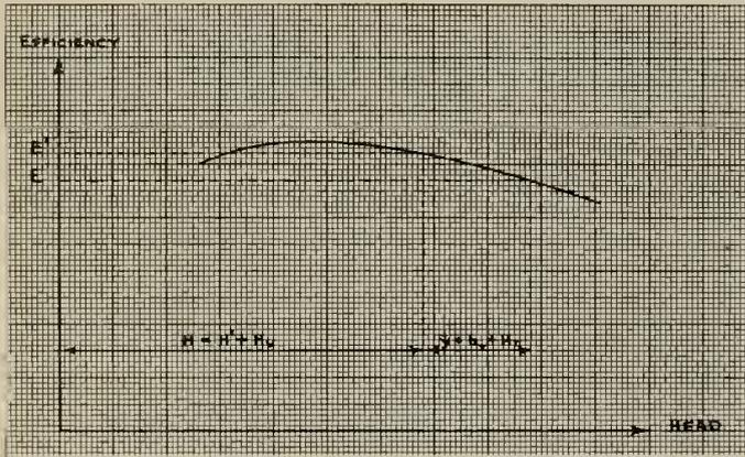
Fig. 4—Efficiency-Head Curve at Constant Power.
