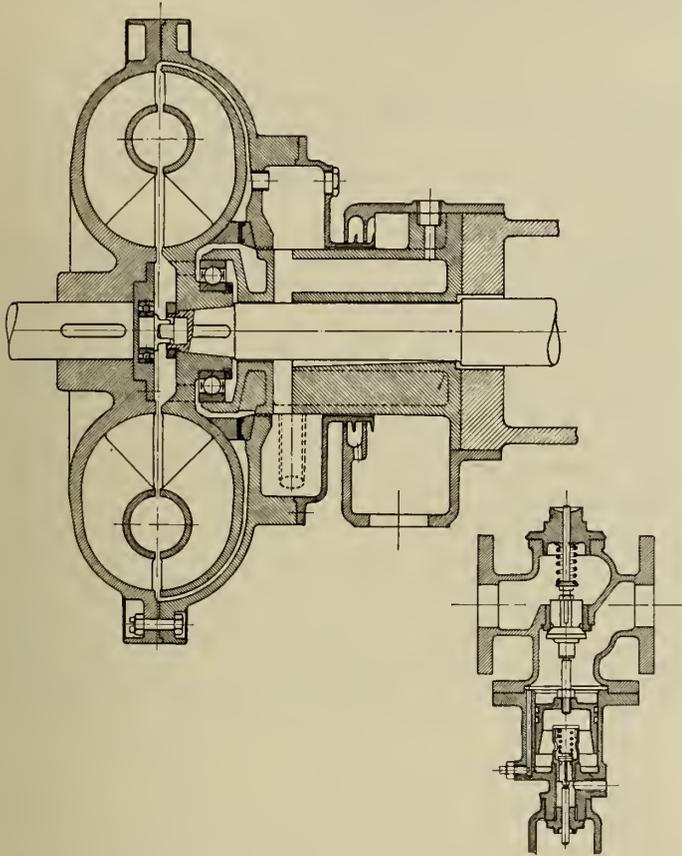
Fig. 8—Scoop Tube Type—Pump Drive, Pressure Valve Control.
