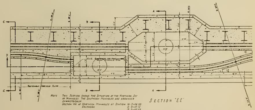
Fig. 7—Sidewalk and Electrical Duct Layout.
