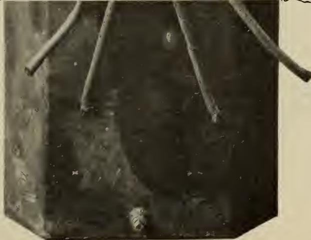
This transformer fell 20 feet without damaging its insulation; it passed all electrical tests satisfactorily.
