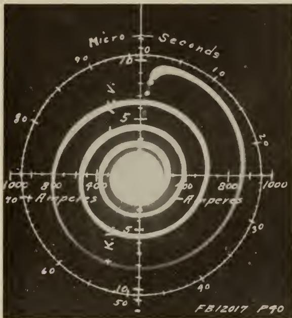
Fig. 7—Oscillogram with Rotating Film.
