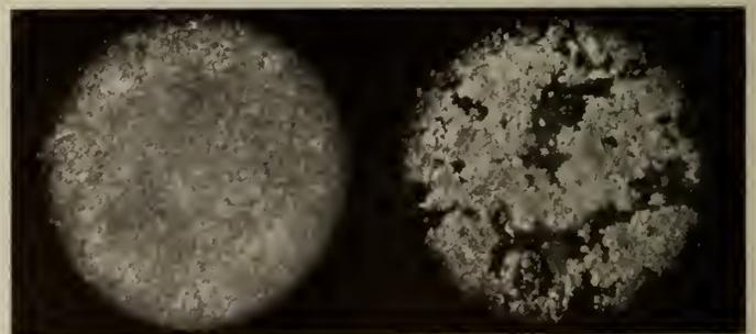
Fig. 8—Samples of Good and Inferior Aluminum Paint.
