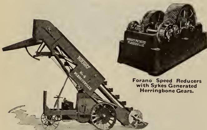
Forano Speed Reducers with Sykes Generated Herringbone Gears.
