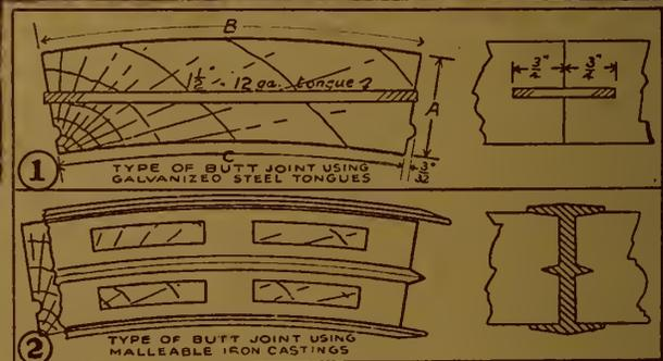
The centre illustration shows a Continuous Stave Wood Pipe line under construction, using this new type butt joint. At the top, Continuous Stave Wood Pipe on cement cradles. Below, (1) a cross section of the original type butt joint using galvanized steel tongue and (2) the new type butt joint using malleable iron castings.
