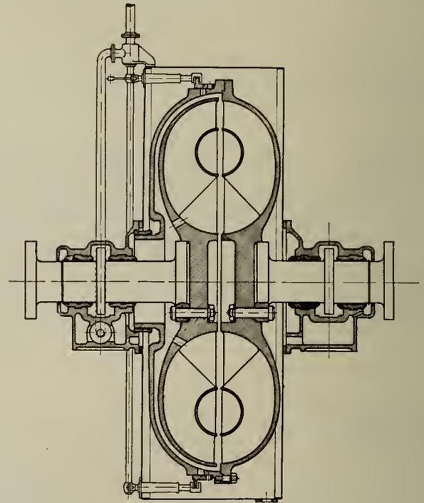
Fig. 2—Hydraulic Coupling—Marine Type.
