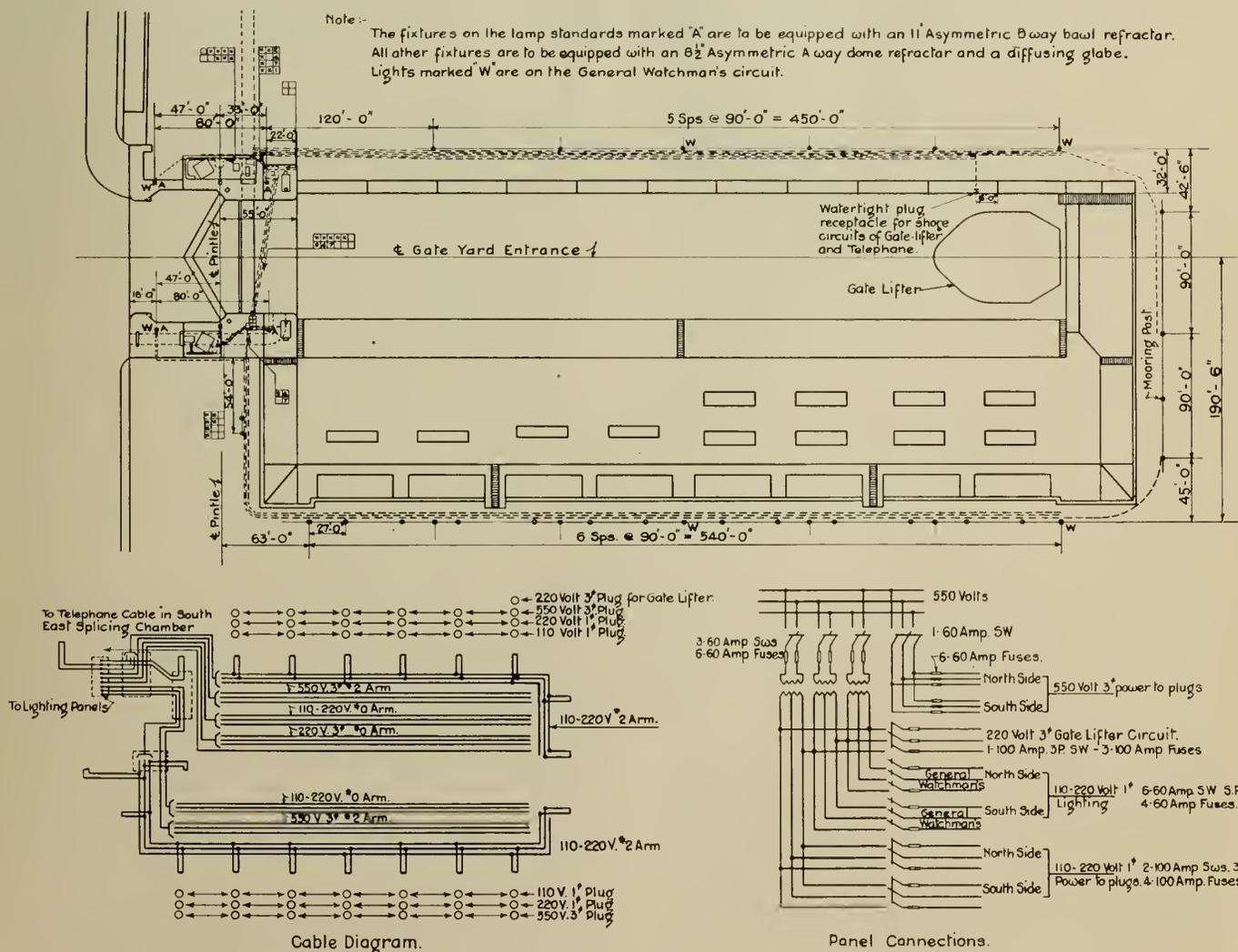
Fig. 11—General Arrangement of Lighting and Circuits for Gate Yard.
