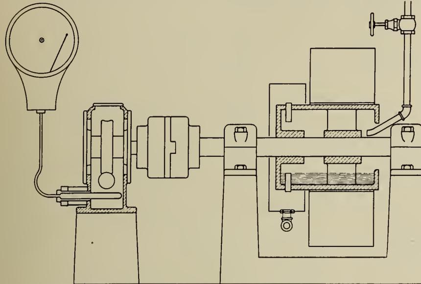
Fig. 3—Details of Arrangement of Brake and Thermometer.
