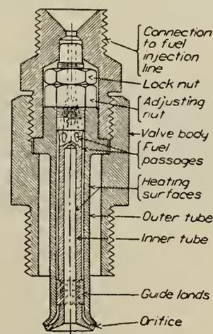
Fig. 5—Section Through Annular Orifice Automatic Injection Valve.
