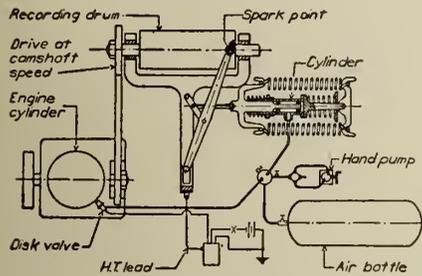
Fig. 3—Electrical Balanced Pressure Disc Type Indicator.
