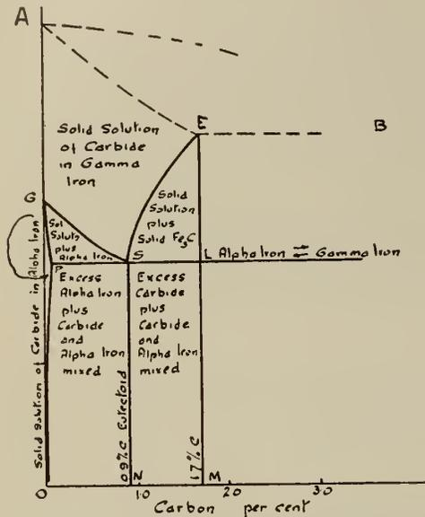
Fig. 11—Lower Portion of Iron-Iron Carbide Diagram.
