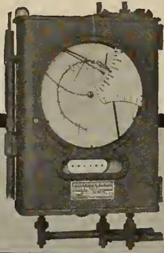
**INDICATE:** Steam Flow, Air Flow and Furnace Draft.
