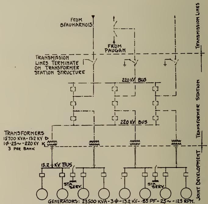
Fig. 1—Electrical Diagram for Generating and Transformer Stations.
