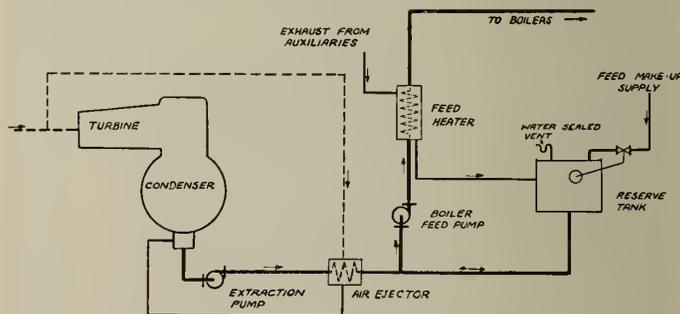
Fig. 4—Diagram of Feedwater Circuit.
