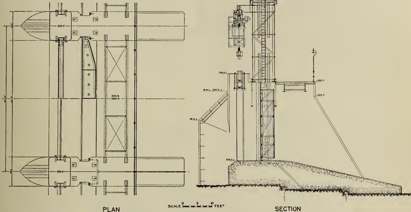
Fig. 3—Plan and Section of one 40-foot sluice gate showing Operating Mechanism and Monorail Hoist.
