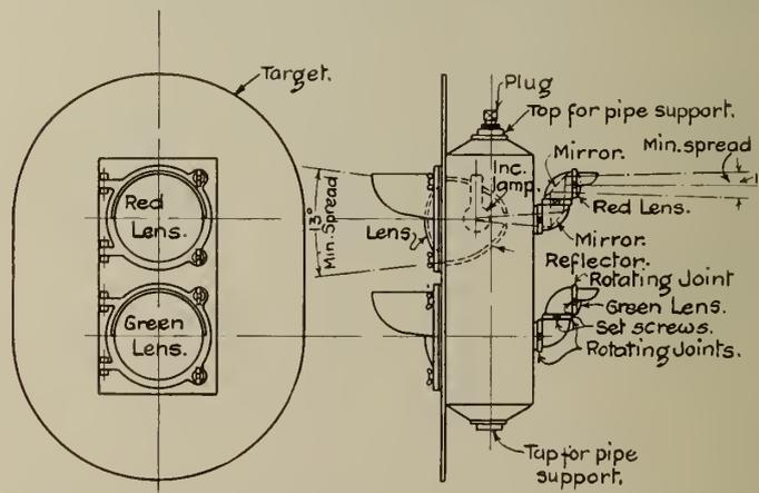
Fig. 17—Colour Light Signals for Locks with Adjustable Rear Sights.
