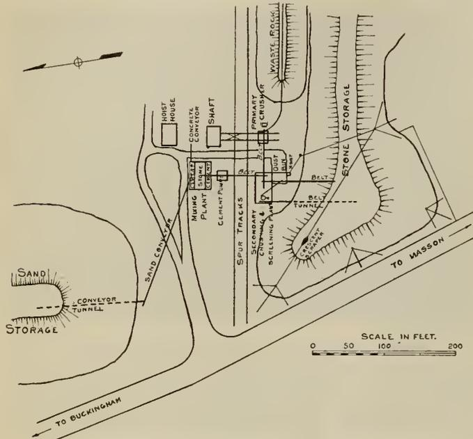
Fig. 10—Layout of Crushing and Mixing Plants.
