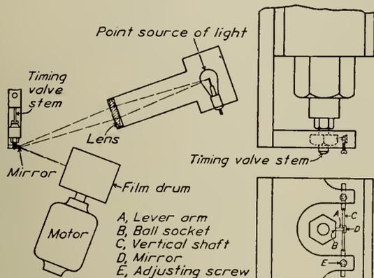
Fig. 8—Apparatus for Recording Motion of Timing Valve Stem. At Right—Enlarged Views of End of Timing Valve.
