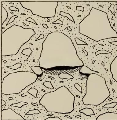
Fig. 7—Diagrammatic Representation of Particle Interference.
