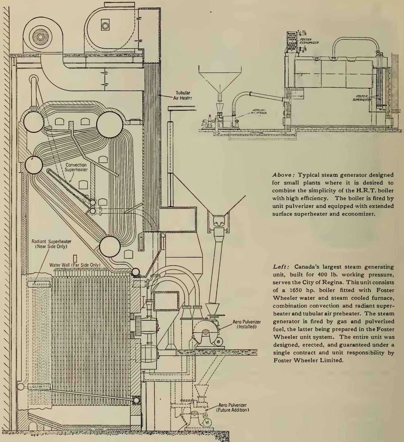
Above: Typical steam generator designed for small plants where it is desired to combine the simplicity of the H.R.T. boiler with high efficiency. The boiler is fired by unit pulverizer and equipped with extended surface superheater and economizer.
