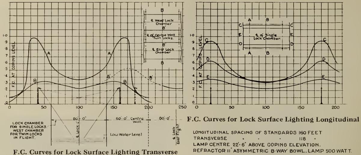
Fig. 6—Curves for Lock Surface Lighting.
