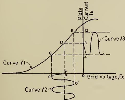
Fig. 4—Action of the Vacuum Tube as an Amplifier.
