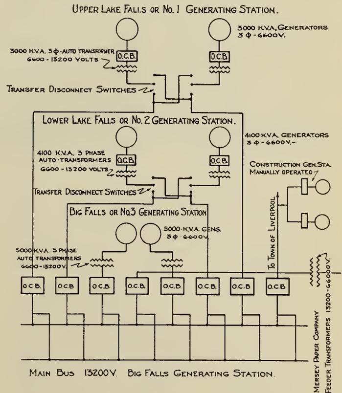
Fig. 4—Diagram of Electrical Arrangement of Mersey System.
