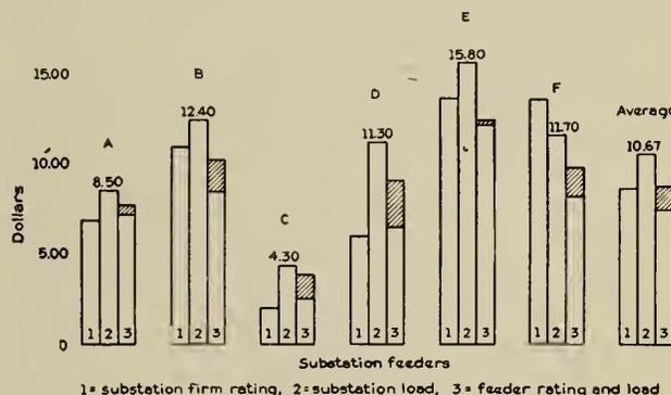
Fig. 10—Feeder Costs Per Kv.-a.
