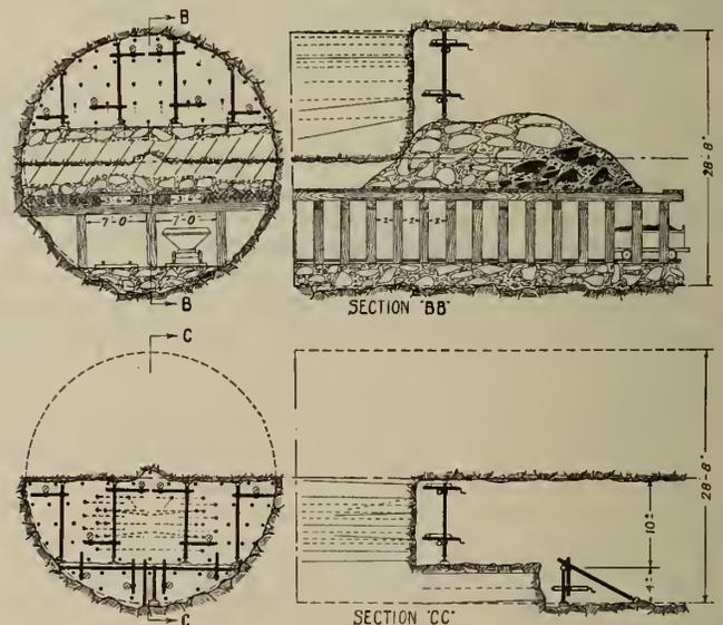
Fig. 5—Breakdown and Bottom Heading and Bench.
