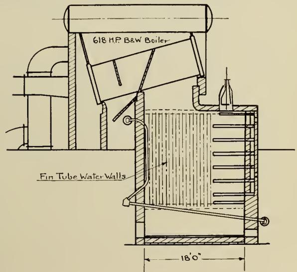
Fig. 2—Installation with Slag Screen and Furnace Walls Partially Water Cooled.
