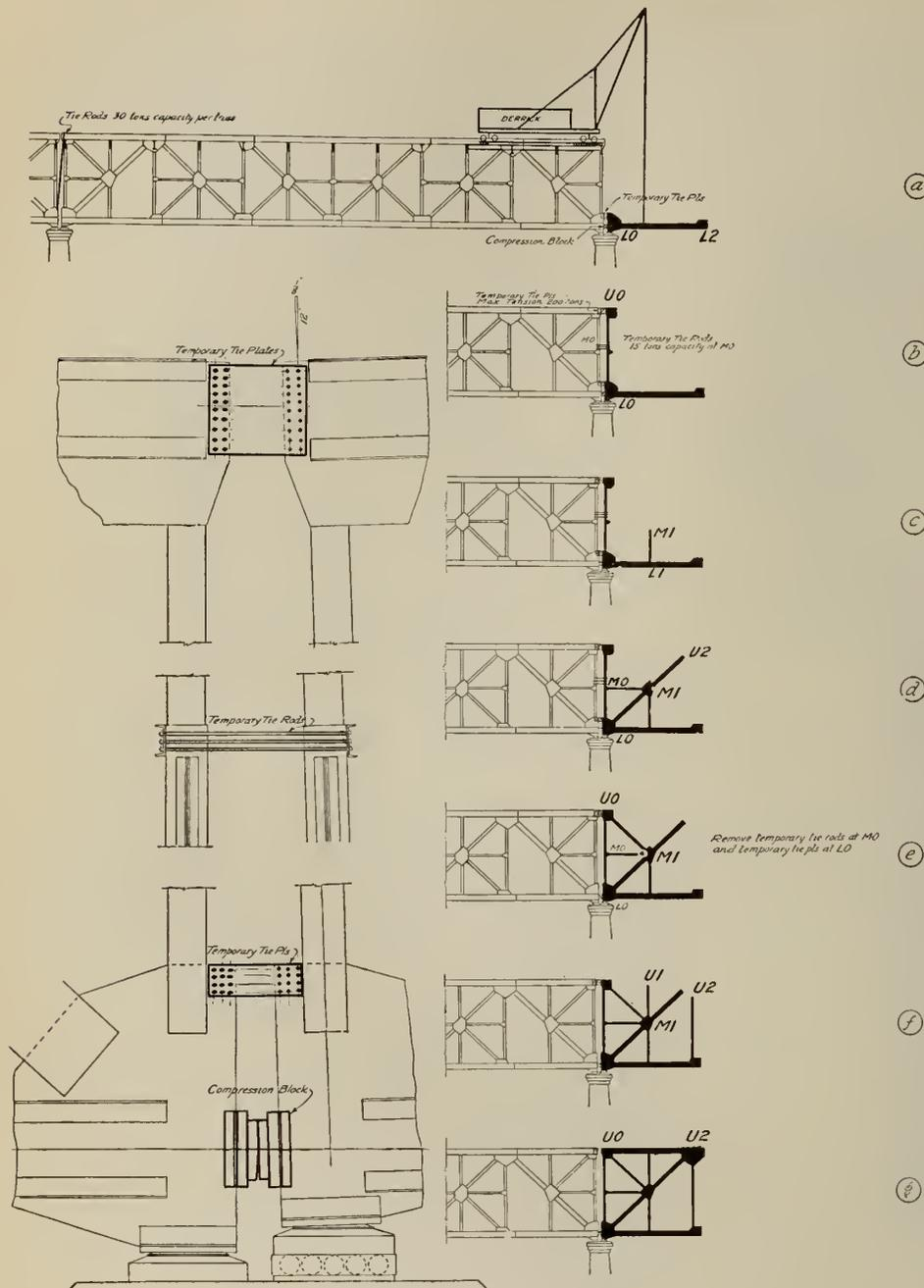
Fig. 9—Cantilever Erection.
