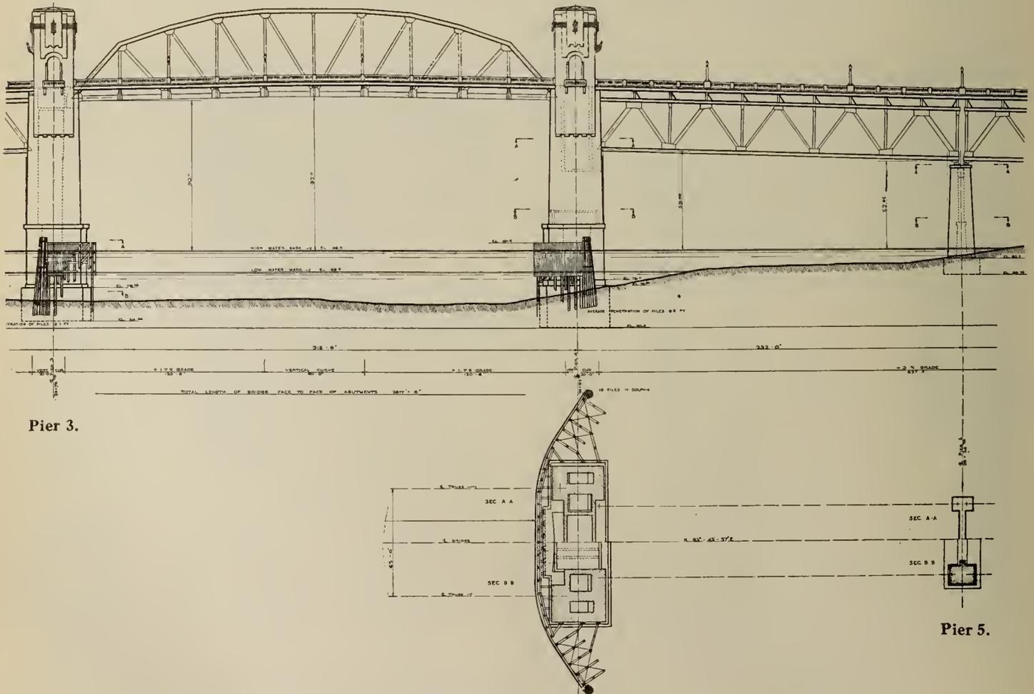
Fig. 7—Main Piers 3, 4 and 5 and Steelwork.
