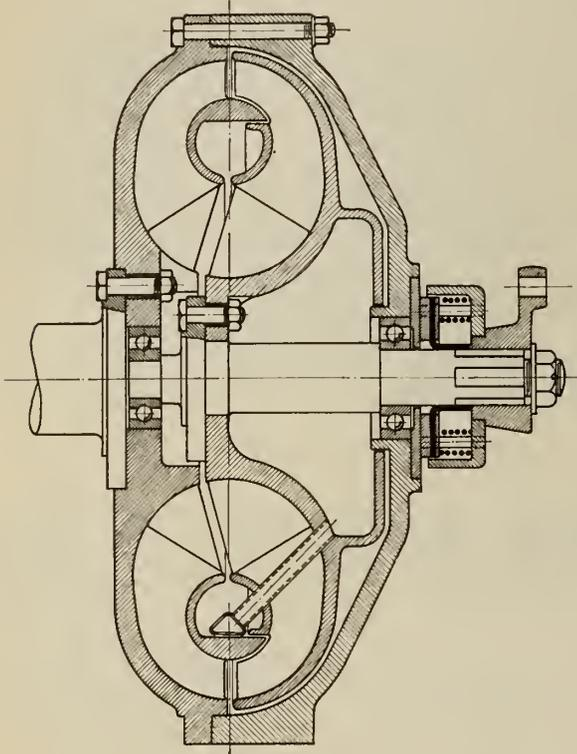
Fig. 11—Hydraulic Coupling—Traction Type.
