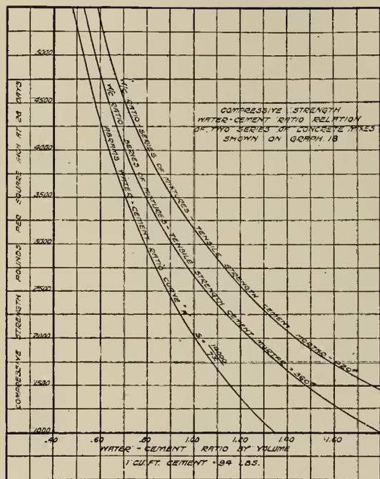
Fig. 19.—Strength-Water-Cement Ratio Relation for Mixtures of Fig. 18.
