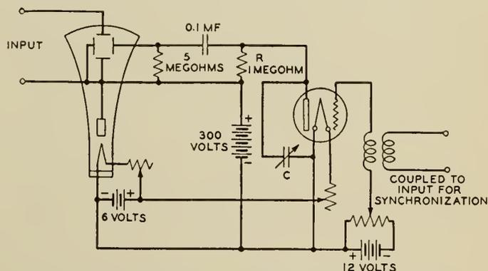
Fig. 10—Circuit Diagram for Linear Time Axis for a Cathode-Ray Oscillograph.
