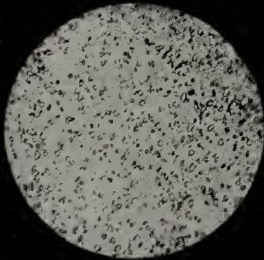
*The structure of **SKF** Through-Hardened Chrome Steel.*
