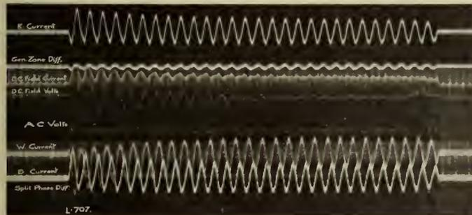
Fig 3—Record from Sudden Short Circuit Test at Rated Voltage.
