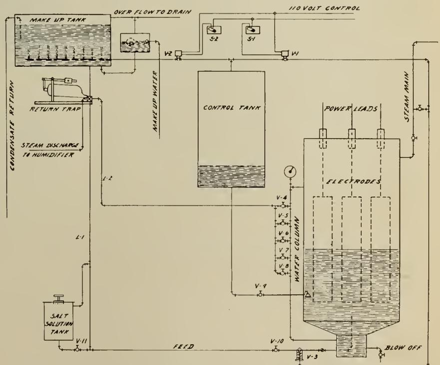
Fig. 12—Diagram showing Scheme of Automatic Water Level Control for 500 kw. Kaelin Electric Boiler.
