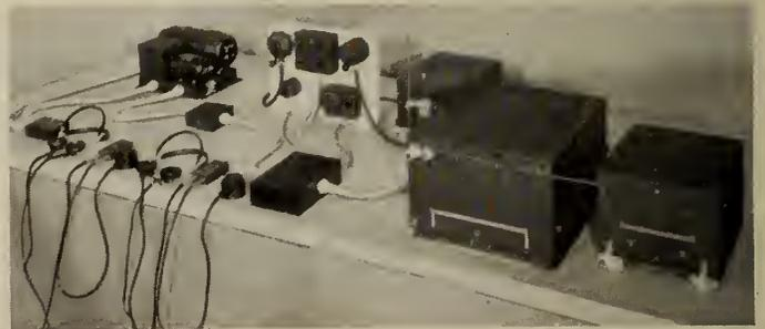
Fig. 7—Equipment for Two-Way Communication from an Aeroplane.
