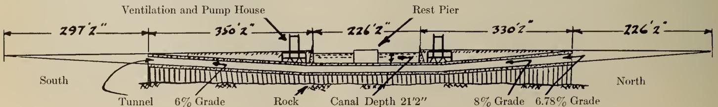
Fig. 2—Longitudinal Section of Subway.
