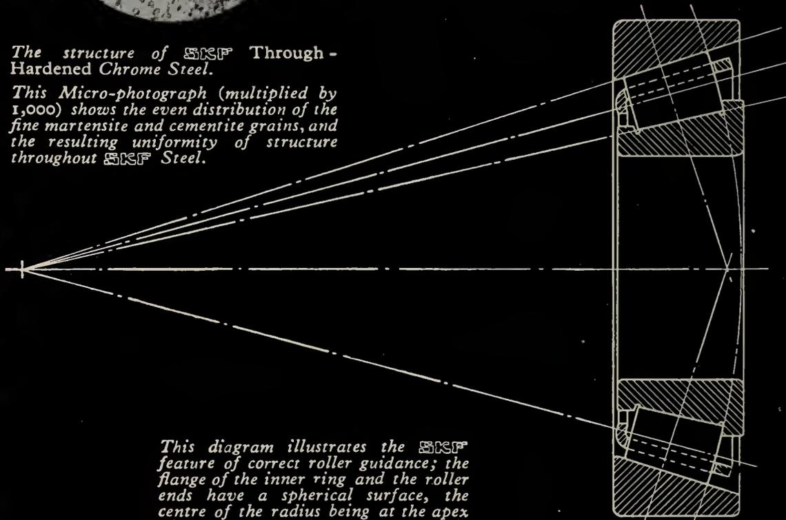
*This diagram illustrates the **SKF** feature of correct roller guidance; the flange of the inner ring and the roller ends have a spherical surface, the centre of the radius being at the apex of the cone that intersects the main axis of the bearing.*
