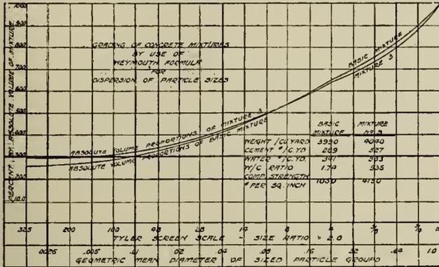
Fig. 17—Gradings of Mixtures by Weymouth Formula.
