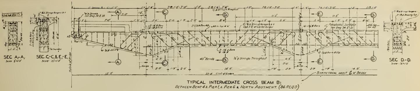
Fig. 3—Concrete Viaduct—Typical Cross Beam.
