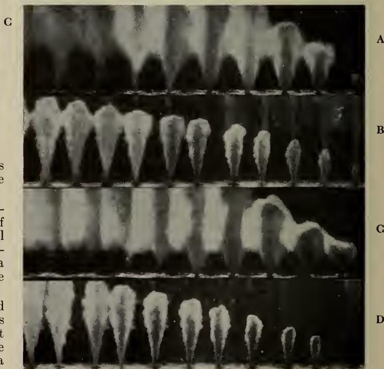
**Fig. 7—A and B—Oil Spray with Secondary Discharge.**
