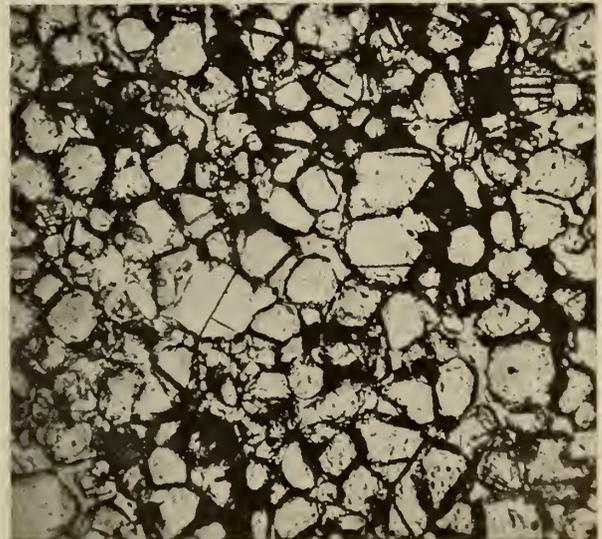
Fig. 2—Thin Section of Open Hearth Furnace Bottom. Magnification approximately 50.
