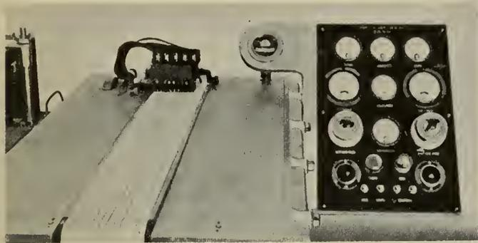
Fig. 7—Recording Table, Record Tape, Pen Units and Control Panel.
