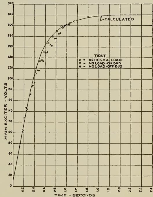
Fig. 5—Voltage Response of Main Exciter.
