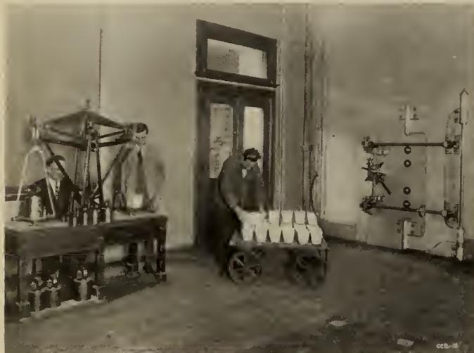
Fig. 2—Weighing Ingot Silver.
