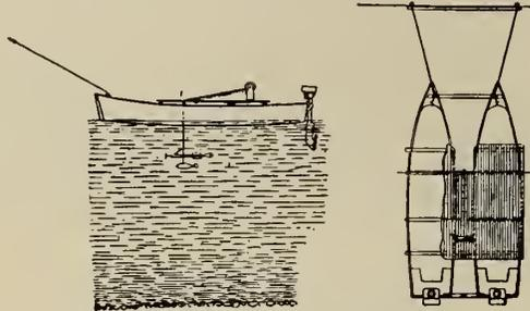
Fig. 2—Equipment Used in Stream Flow Metering.
