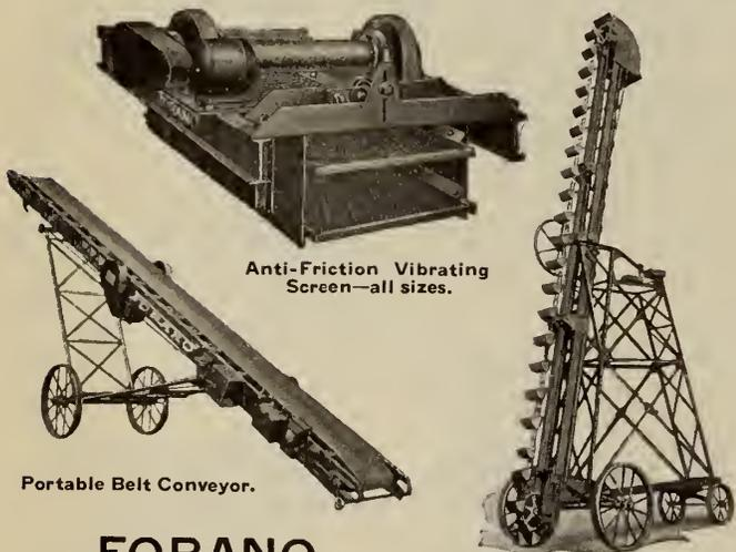
Anti-Friction Vibrating Screen—all sizes.
