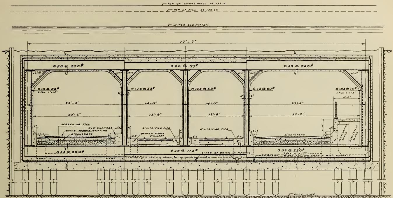
Fig. 3—Cross Section of Subway.
