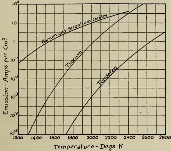
Fig. 1—Comparison of Thermionic Emission from Different Materials.
