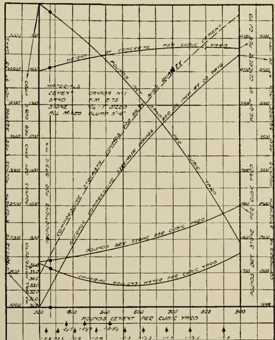
Fig. 18—Mix Proportions and Characteristics.
