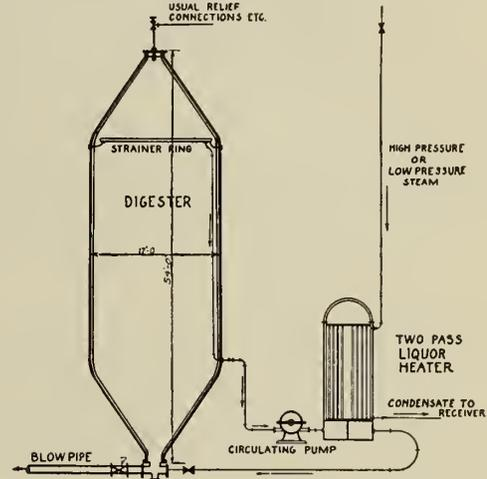
Fig. 4—Digester Circulating and Indirect Heating System.
