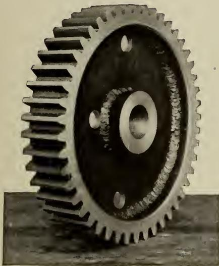
The new "Roldweld" Steel Gear is electric welded, with a forging-quality .45% carbon rim, heat treated. It is long wearing and practically unbreakable. The cost is less than a steel casting, the strength greater, and delivery can be made in a quarter of the time.
