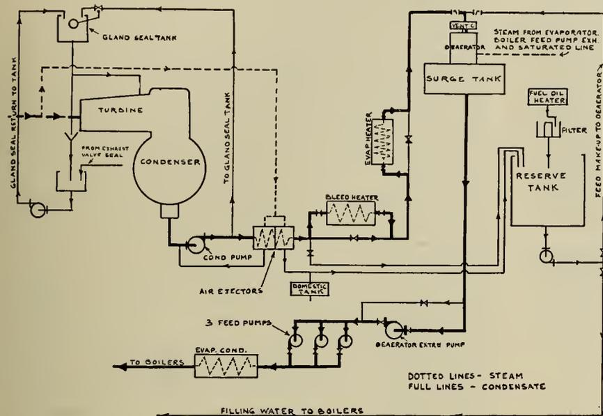
Fig. 3—Diagram of Condensate Circuit.
