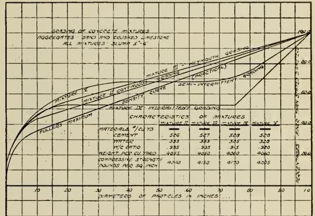
Fig. 6—Mixture Gradings.
