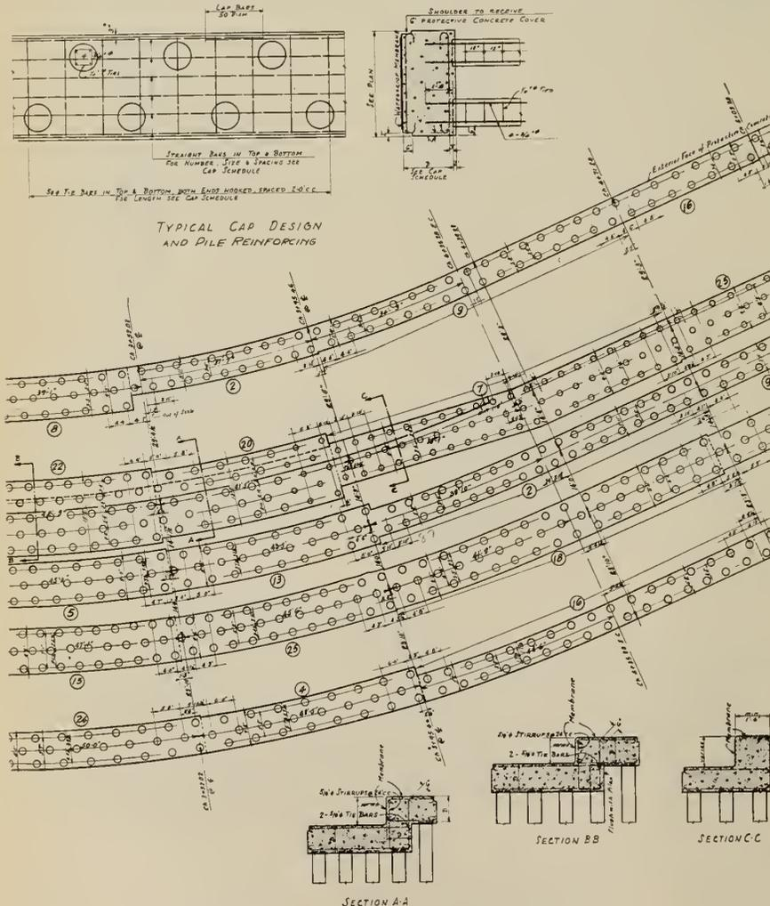
Fig. 8—Typical Concrete Pile Layout.
