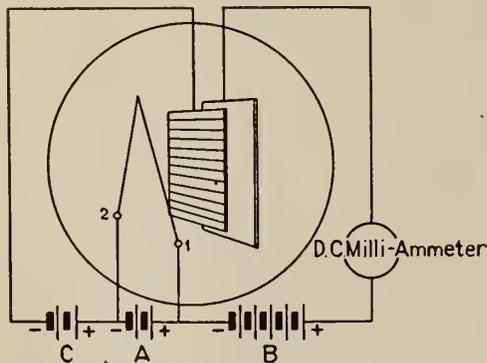
Fig. 2—Three-Electrode Vacuum Tube.
