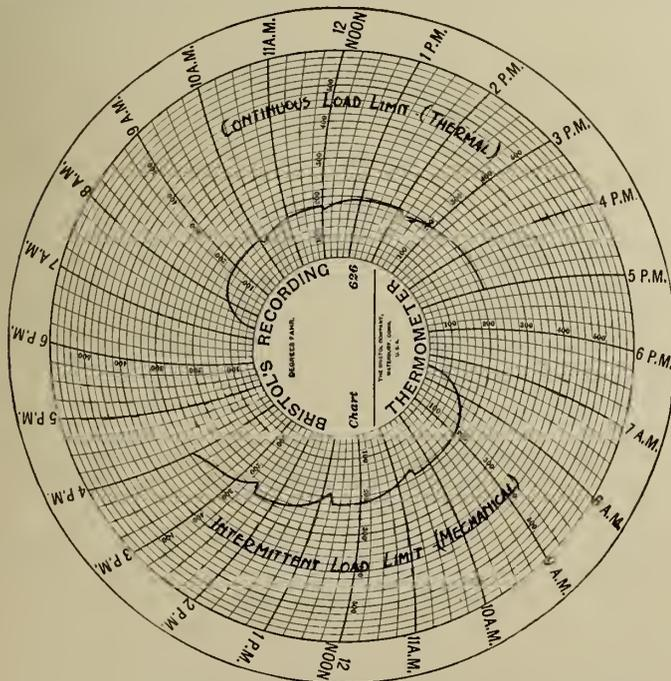
Fig. 4—Oil Temperature Record from Typical Brake Tests.
