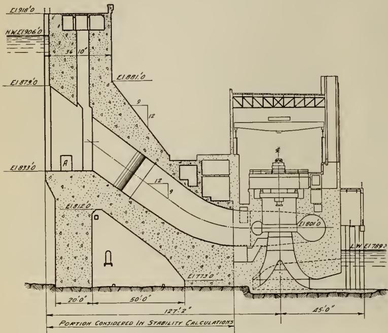
Fig. 1—Section through Intake and Power House.
