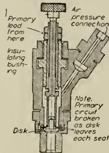
Fig. 4—Electrical Balanced Pressure Disc Valve.
