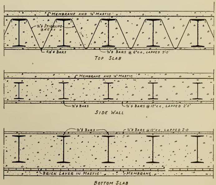
Fig. 4—Typical Slab and Wall Reinforcement.
