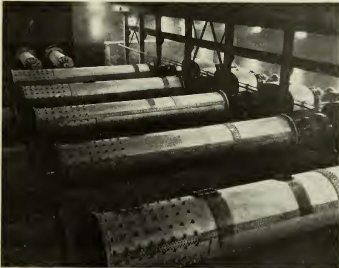
Fig. 2—Unikon Mills in which Limestone is Pulverized Wet.
