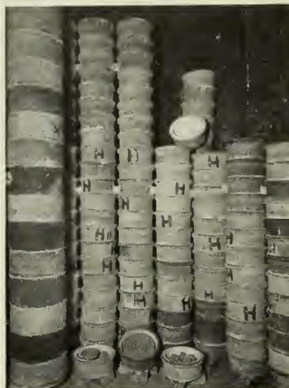
Fig. 11—Interior of Kiln During Loading.
