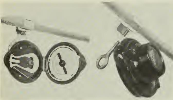
Fig. 16—Servis Vibration Recorder.
