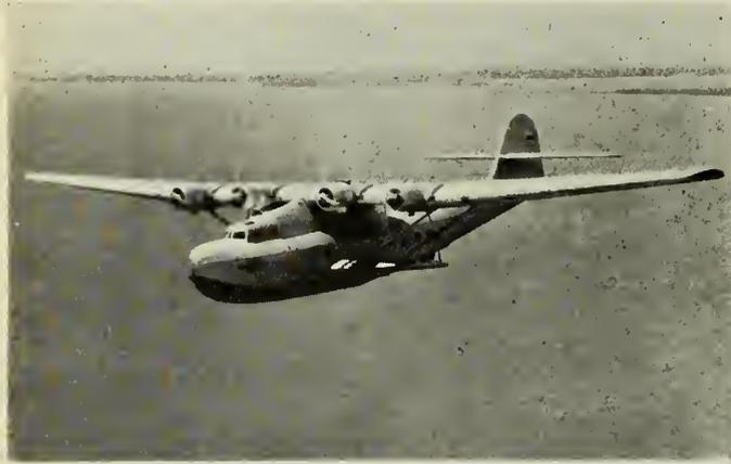
Fig. 8—Glenn Martin Clipper. Four 800-h.p. Motors. All-up Weight 51,000 pounds. Max. Speed 180 m.p.h. with Fuel for 3,200 Miles.
