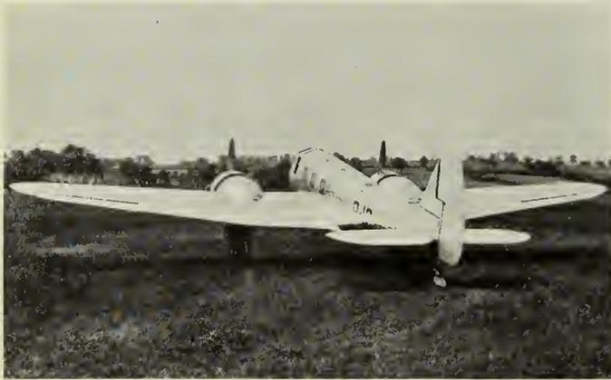
Fig. 6—Bristol Monoplane. Latest British Transport Type. Two 775-h.p. motors. Max. Speed 260 m.p.h.
