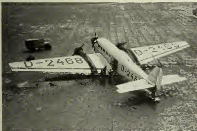
Fig. 4—Junkers 52 Monoplane. Three 700-h.p. motors. All-up Weight 20,900 pounds. Max. Speed 180 m.p.h.
