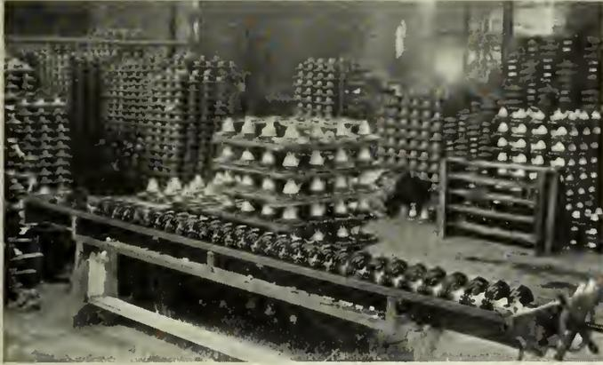
Fig. 14—Routine Tension Test.
