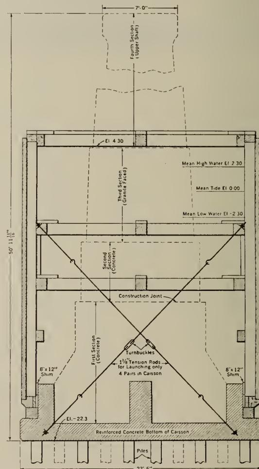
Fig. 6—Section Through Concrete-Bottomed Cofferdam for Piers of Newark Bay Bridge. Jersey Central Railroad.
