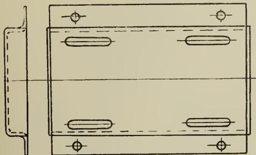
Fig. 1—Bending and Welding Combined to Produce Substantial Bedplate.
