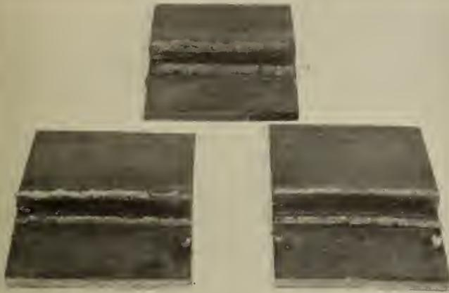
Fig. 5—Welds Produced by Untrained Operators.
