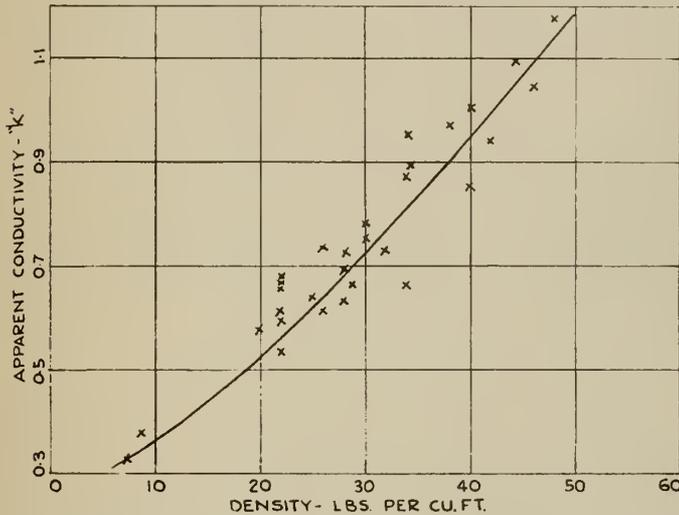
Fig. 7—Test Results on Dry Timber (Mean Temp. 75 degrees F.)
