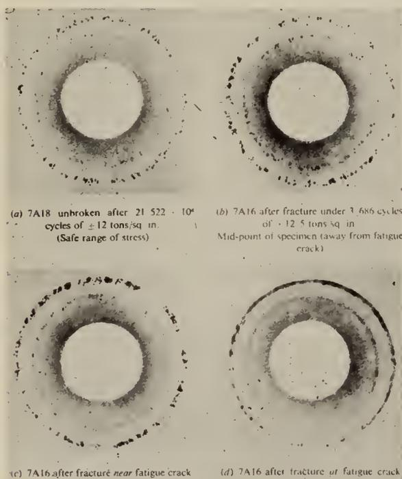
Fig. 1—X-ray patterns showing crystal breakdown.
