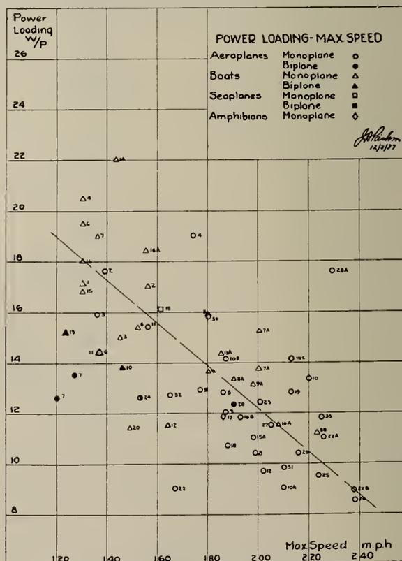
Fig. 23—Power Loading—Maximum Speed.
