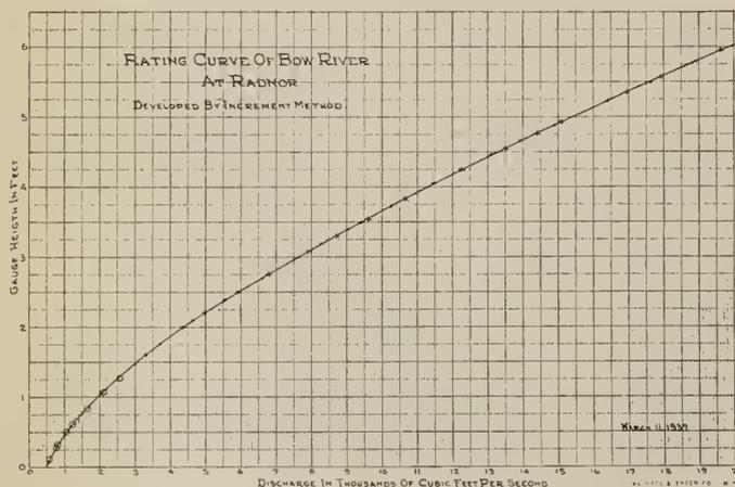
Fig. 1—Rating Curve of Bow River Developed by Increment Method.
