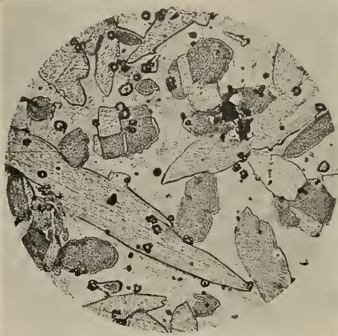
Fig. 3—Manganese Bronze Casting, Magnification 100. Cooled in Sand.
