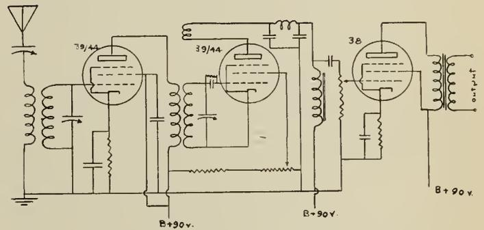
Fig. 6—Diagram of 6.3-volt type receivers installed in 1935.
