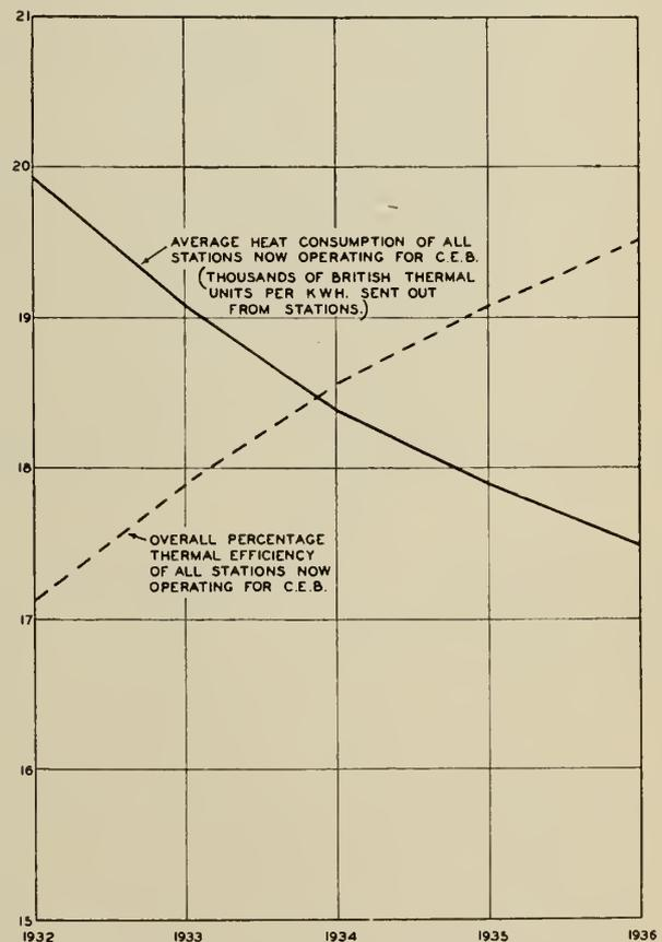
Fig. 15—Fuel Reduction with Grid Operation.
