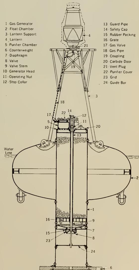
Fig. 11—Diagram of Gas Buoy.
