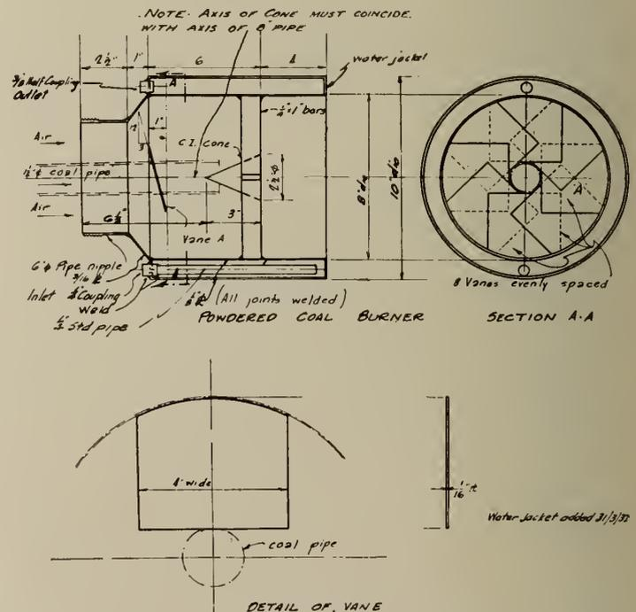
Fig. 1—Detail of Powdered Coal Burner.
