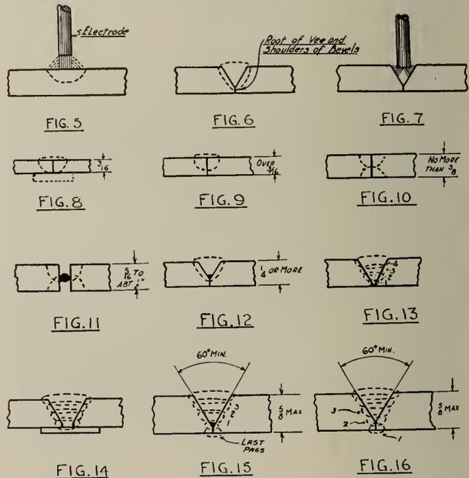
specified. This weld may be made to satisfy such codes if one side is welded and the other side then chipped to solid weld metal and completed.
