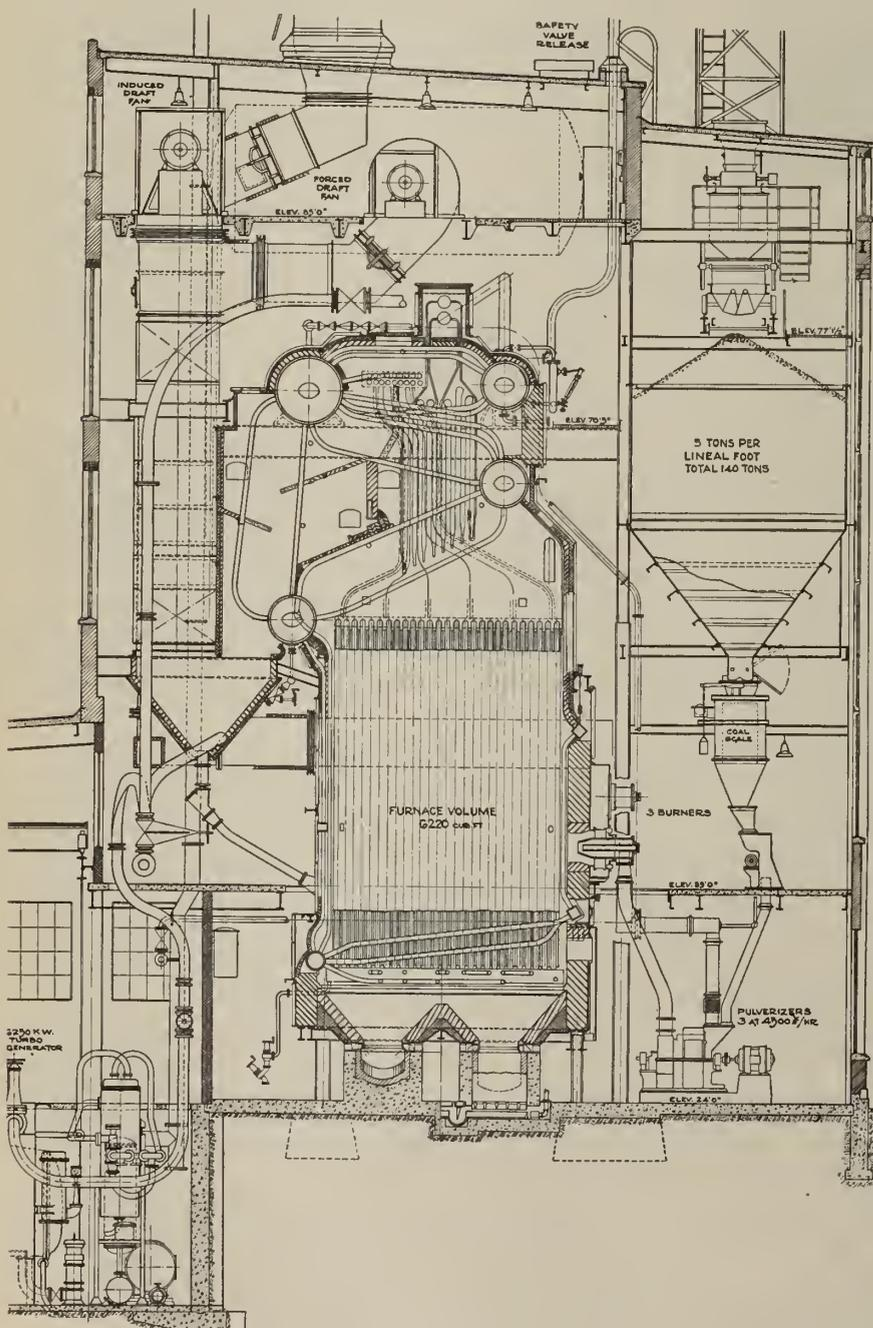
Fig. 3—Cross Section Showing General Arrangement, No. 3 Boiler.
