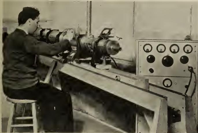
Fig. 8—Transmitting end of Experimental Wave Guide.
