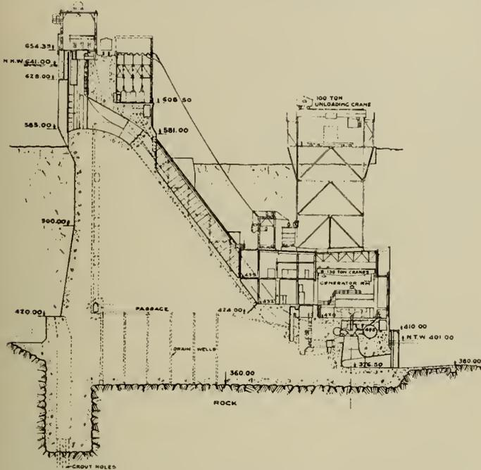
Fig. 6—Abitibi Canyon. Cross Section through Main Dam and Power House.
