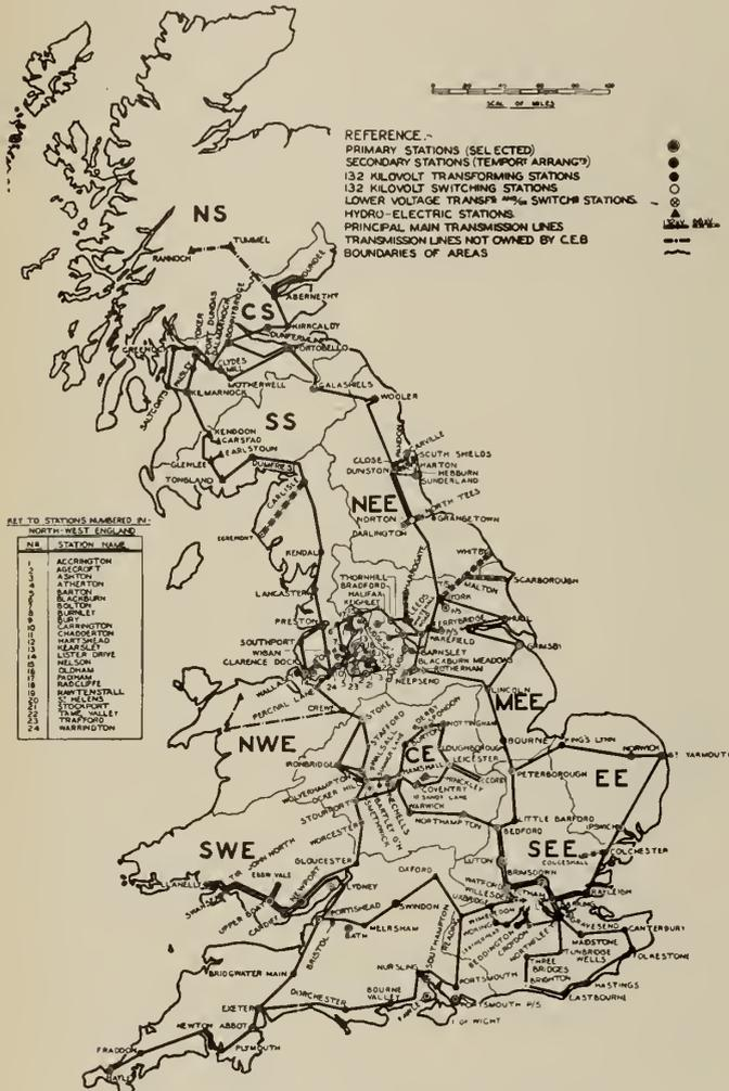
Fig. 1—Main "Grid" Transmission Lines.
