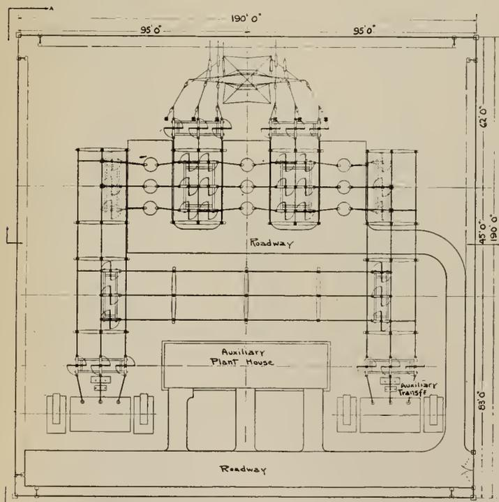
Fig. 5—Typical Mesh-Type Substation.
