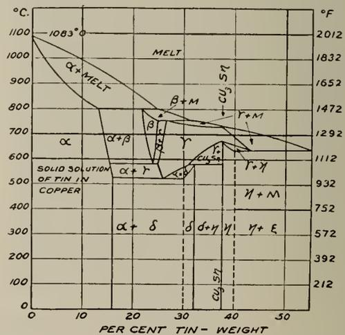
Fig. 11—Copper-rich portion of the Copper-Tin Diagram.
