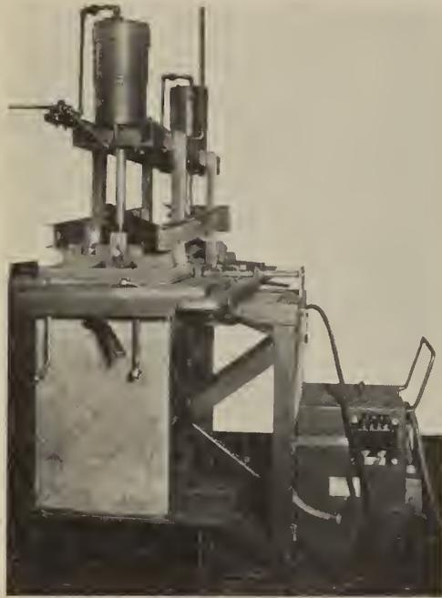
Fig. 7—Welding Fixture and Equipment for Arc Welding Food Compartments. Welding Speeds 22 to 23 inches per minute.
