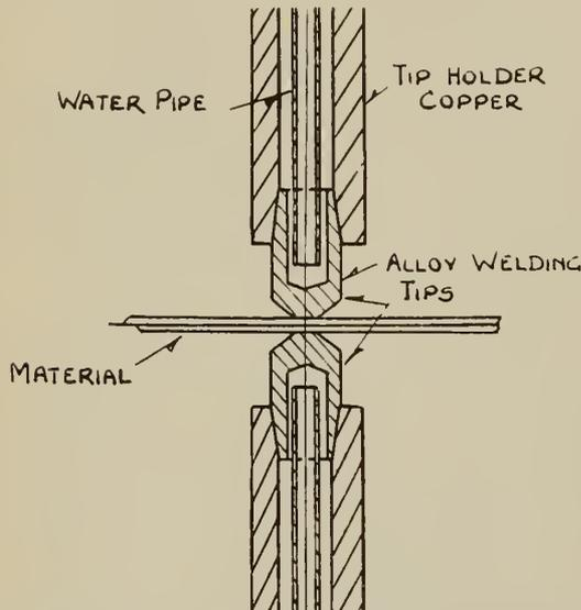
Fig. 10—Cross-Section of Spot Welder Tips, showing Method of Cooling.
