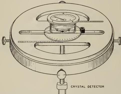
Fig. 5—Apparatus used in Verifying the various Configurations of the Lines of Force shown in Fig. 1.
