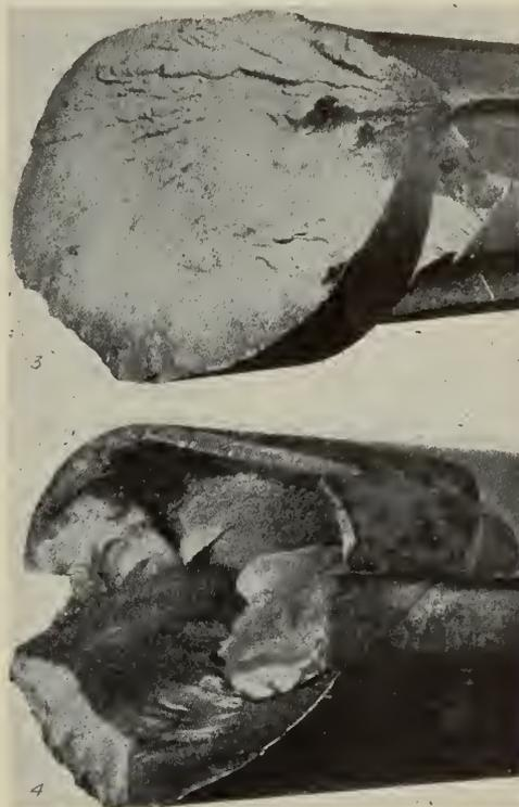
Fig. 4—(above)—A fracture produced by static torsion.
