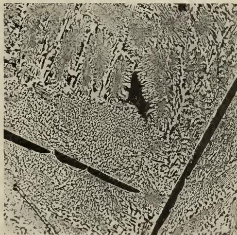
Fig. 20—Copper Antimony Eutectic, Magnification 100. Dark bars are violet  $\text{Cu}_2\text{Sb}$  and dark background is also  $\text{Cu}_2\text{Sb}$ .
