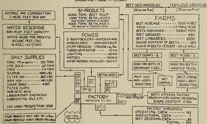
Fig. 3—Materials used in 24 hours in beet sugar factory.
