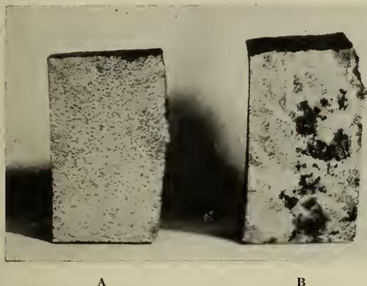
Fig. 17—P.M.G. Bronze. A—properly made, B—coarse crystals.
