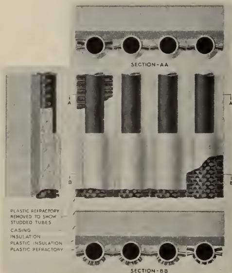
Fig. 20—B-W Bailey Stud-Tube Furnace Wall.
