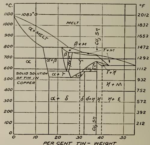
Fig. 11—Copper-rich portion of the Copper-Tin Diagram.
