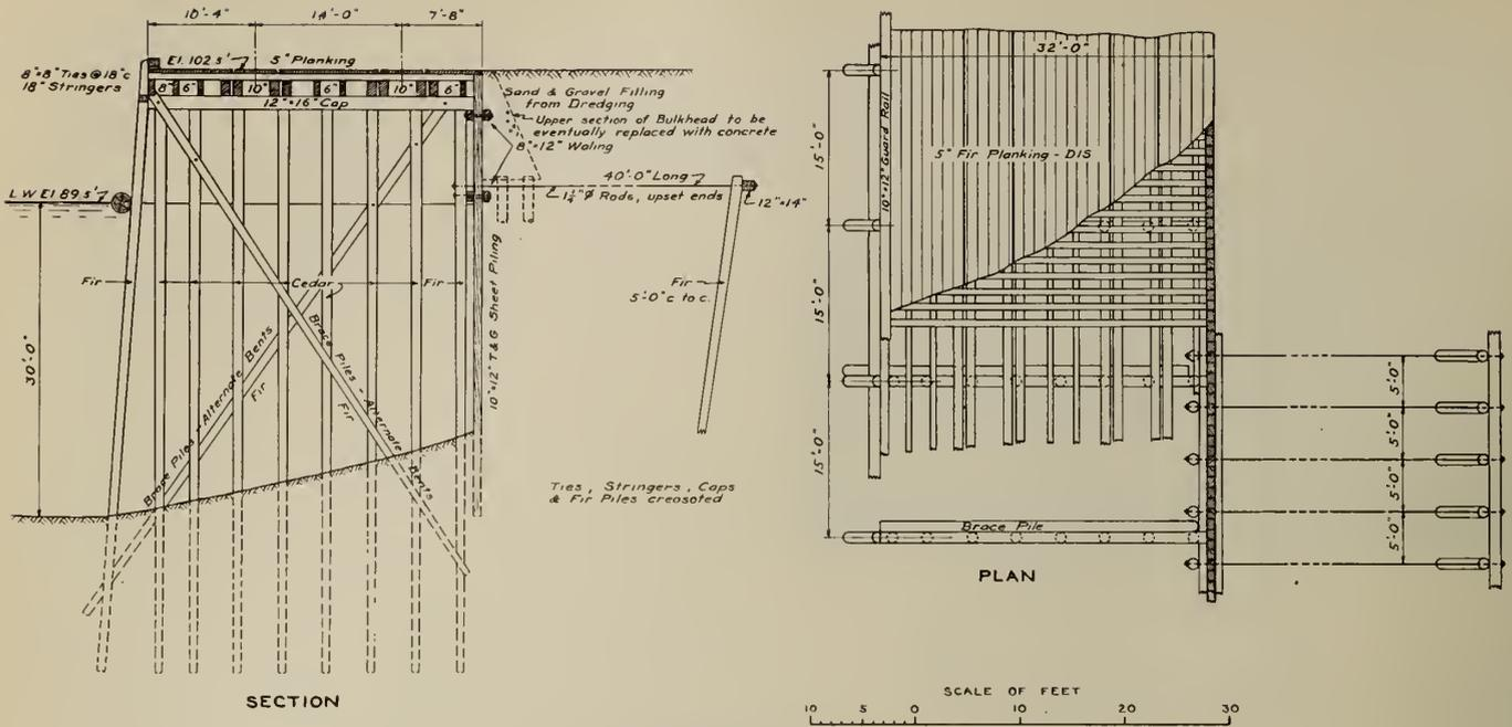
Fig. 16—Typical Wharf and Bulkhead Construction, New Westminster, B.C.
