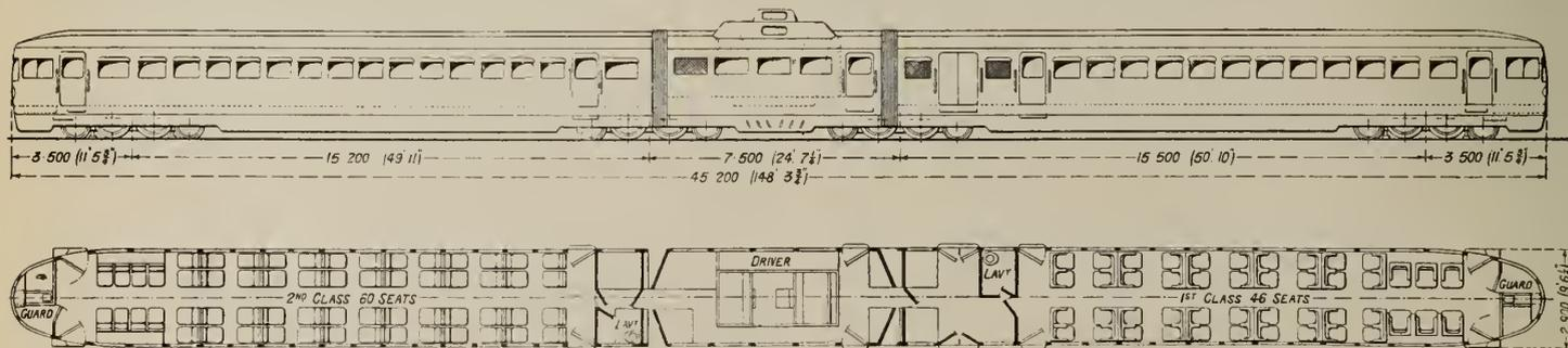
Fig. 15—Longitudinal Section of Michelin-Triple-Car Pneumatically-Tired Train.
