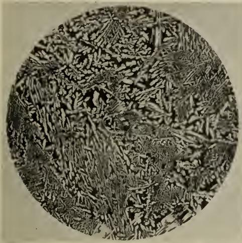
Fig. 6—Manganese Bronze Casting, Magnification 100. Cooled in Sand.
