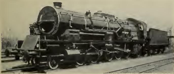
Fig. 6—View of 2-10-2 P.L.M. 4-Cylinder Compound Locomotive with Outside Cylinders.
