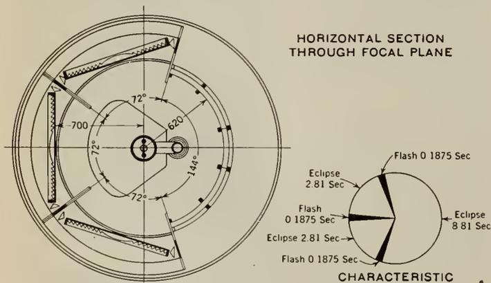
Fig. 7—Section of Second Order Flashing Light.
