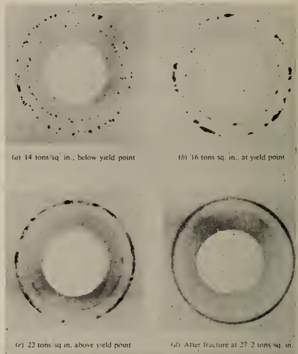
Fig. 2—X-ray patterns showing crystal breakdown.
