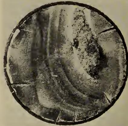
Fig. 1—Low Temperature fracture in a street car axle.
