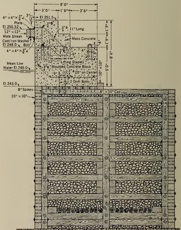
Fig. 11—Section of Harbourhead Wall, Toronto Harbour.
