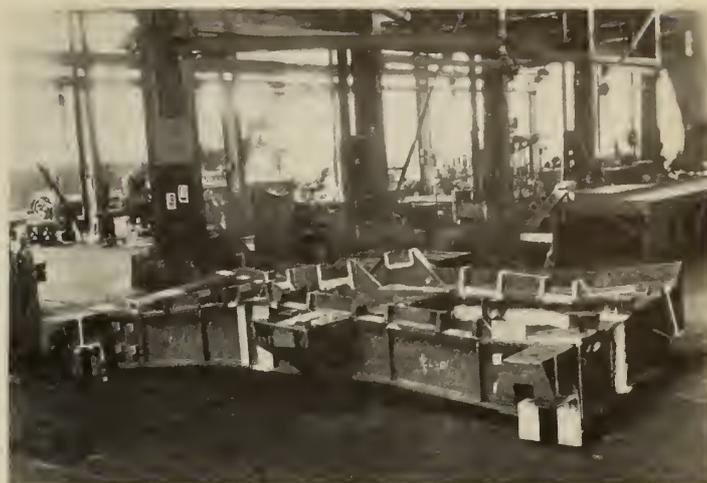
Fig. 3—Arc Welded 60-Ton Crane Trolley Frame.
