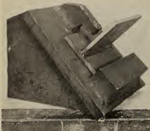
Fig. 3—Fillet Weld Testing Fixture with Weld in position for Breaking.
