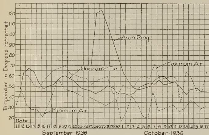
Fig. 14—Temperatures in Main Members during Construction.
