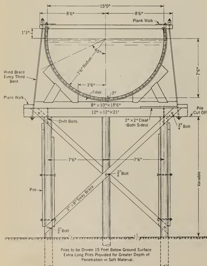
Fig. 12—Section of Lathom Flume.
