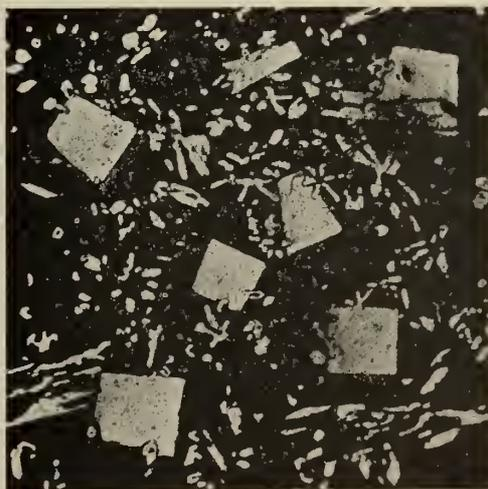
Fig. 21—Babbitt, Magnification 100. Composition. Tin  $83\frac{1}{2}$  per cent; Antimony,  $8\frac{1}{2}$  per cent; Copper,  $8\frac{1}{2}$  per cent; The squares are  $\text{SnSb}$ ; the Stars are Tin-Copper compound.
