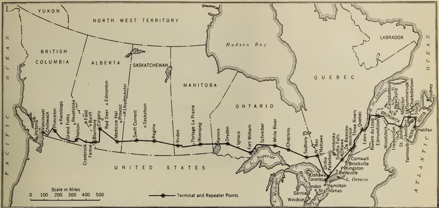
Fig. 9—Route of Trans-Canada Telephone System, showing Terminal and Repeater Points.
