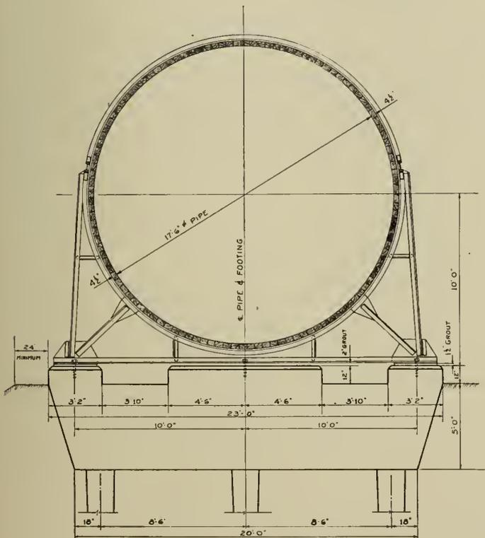
Fig. 4—Typical Section Wood Stave Pipe.
