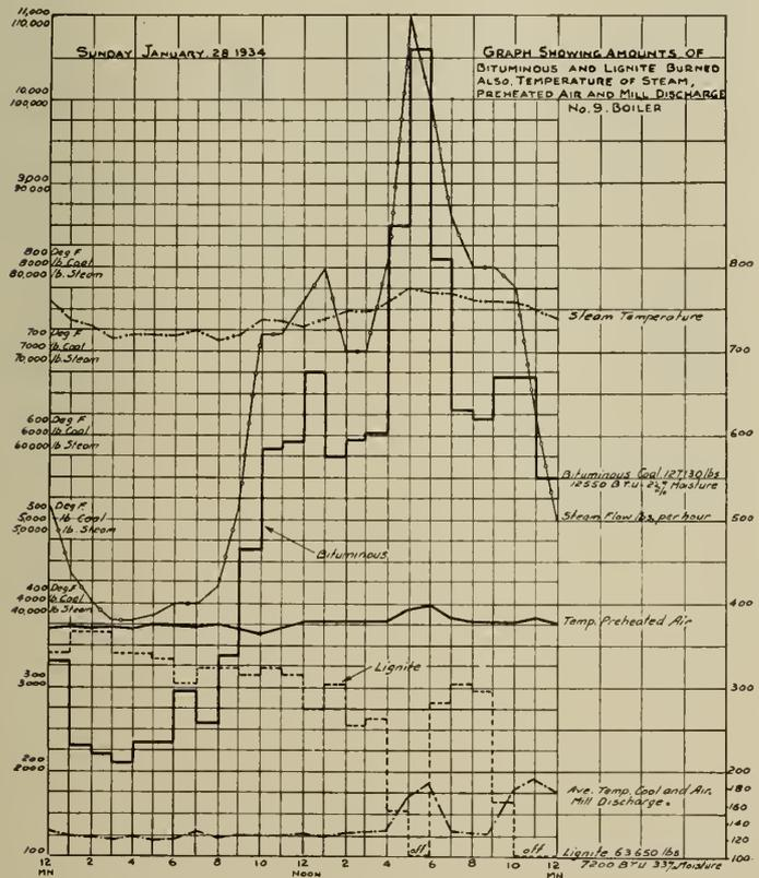
Fig. 5—Coal Burned and Temperatures of Steam, Preheated Air and Mill Discharge on Boiler 9.
