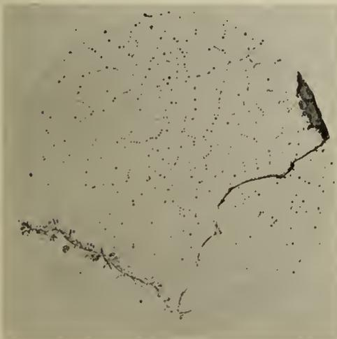
Fig. 7—Manganese Bronze Casting, Magnification 100. Quenched in water from 1,000 degrees F.
