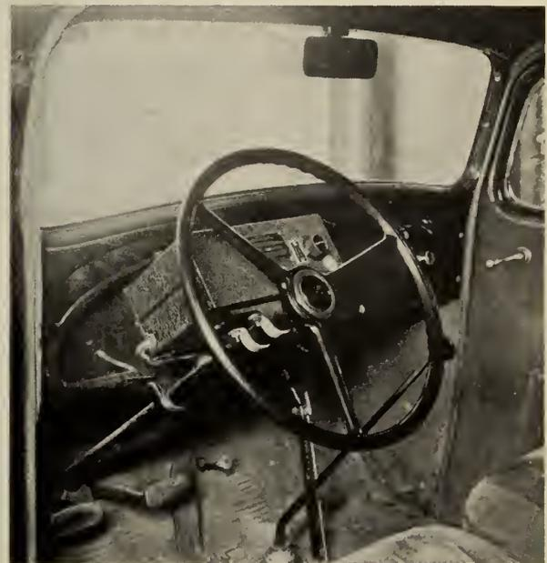
Fig. 14—Police Radio Automobile Receiver.
