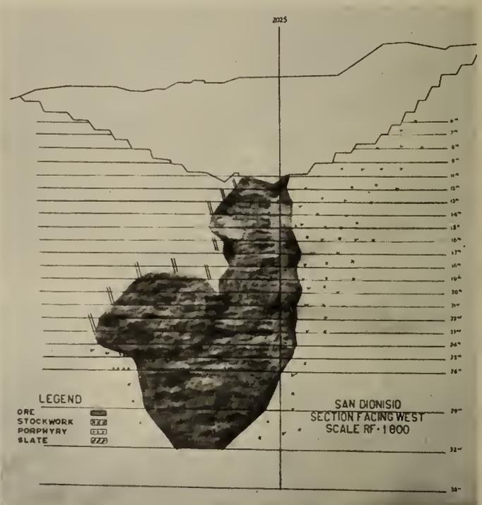
Fig. 4—San Dionisio Orebody. Footwall to Hanging Wall approximately 200 Metres.
