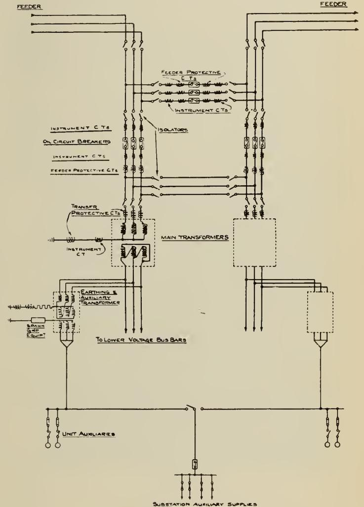
Fig. 4—Typical Three-Switch Substation.
