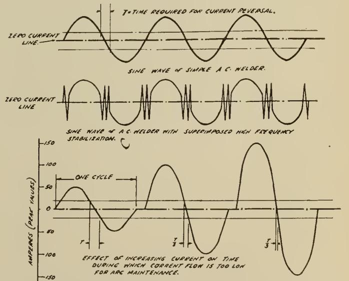
Fig. 6—Sine Waves for Simple and High Frequency Types of a.c. Welders.
