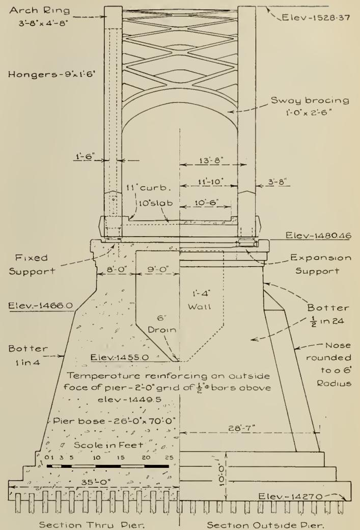
Fig. 4—Side Elevation of Pier with Superstructure.
