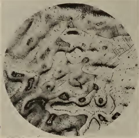
Fig. 13—10 per cent Tin-Bronze, Magnification 100, as Sand Cast. (Note Dendritic structure and tin-copper compound.)
