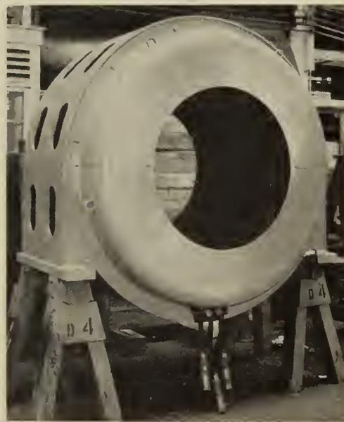
Fig. 2—End Bells for an Electric Motor.
