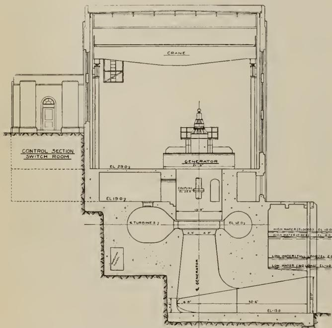
Fig. 5—Cross Section of Power House Showing Arrangement of Main Unit.
