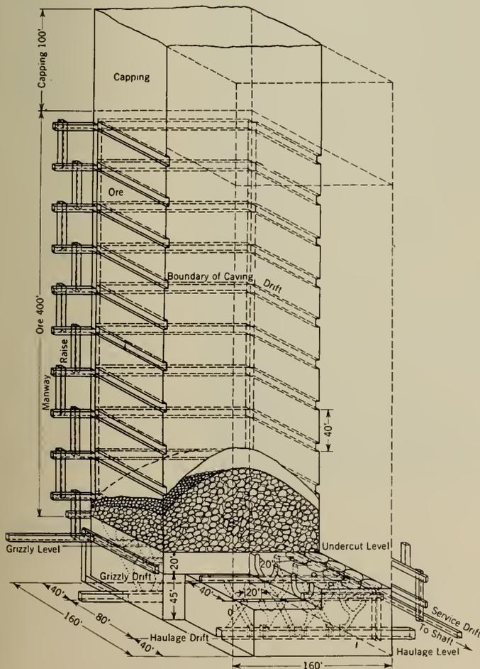
Fig. 2—Isometric Drawing of Stope Block, 160 ft. by 160 ft.
