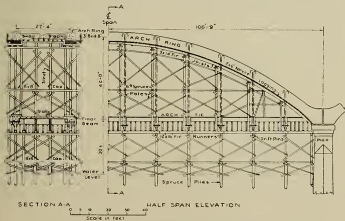
Fig. 18—Falsework for Bowstring Spans.
