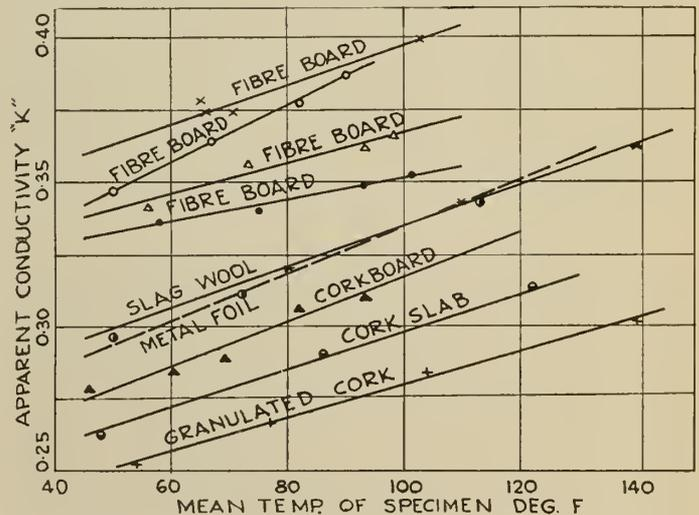
Fig. 6—Effect of Mean Temperature on Test Results.
