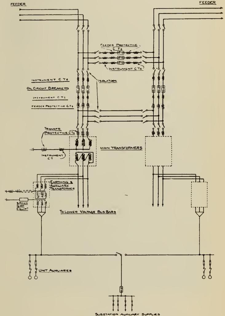
Fig. 4—Typical Three-Switch Substation.
