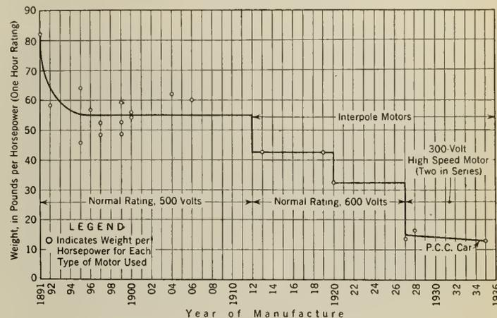
Fig. 3—Curve Showing Trend in Weight of Street Railway Motors.
