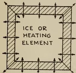
Fig. 1—Simple Hot or Cold Box made entirely of Material to be tested.
