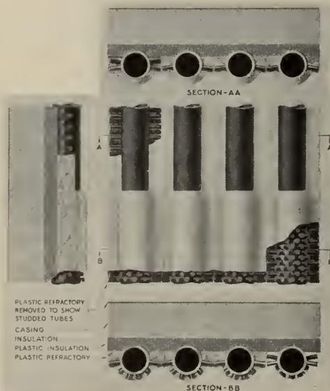
Fig. 20—B-W Bailey Stud-Tube Furnace Wall.
