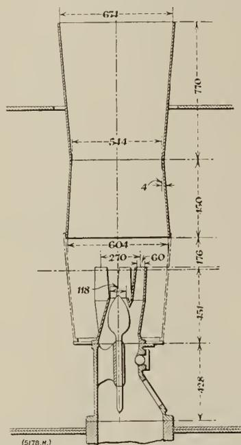
Fig. 8—General Arrangement of Lemaitre Variable Exhaust Nozzle.
