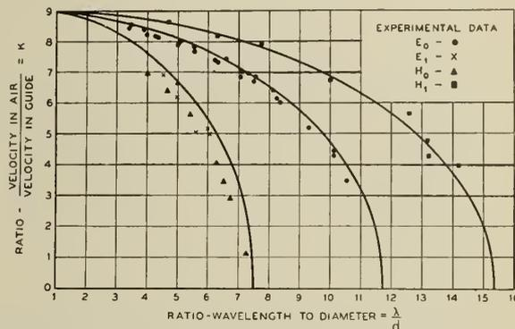
Fig. 4—Comparisons between calculated and measured Velocities of Propagation.
