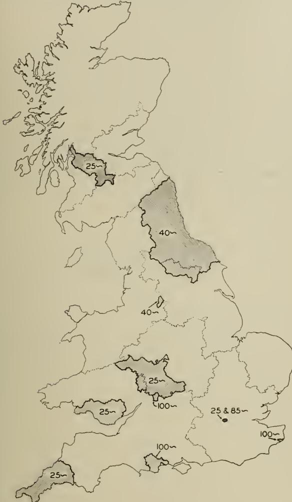
Fig. 11—Areas Changed from Non-Standard a.c. Frequency.
