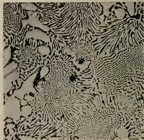
Fig. 5—Eutectic Solder, Magnification 100. Tin 63 per cent. Lead 37 per cent.
