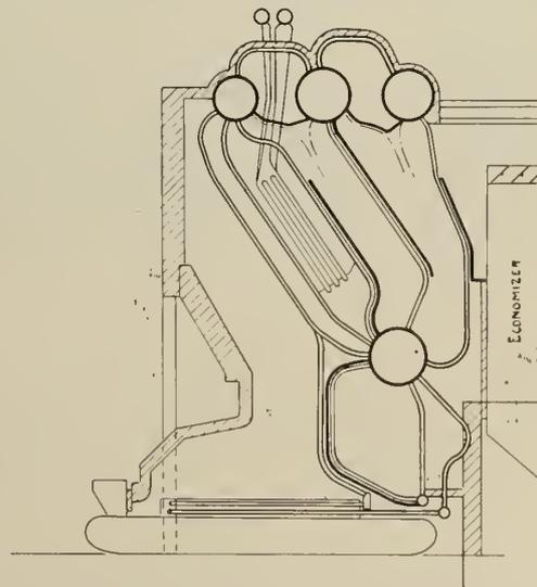
Fig. 16—Stirling Boiler, Water-cooled Rear Arch and Side Walls along Stoker Grate Line. Prince Albert Station.
