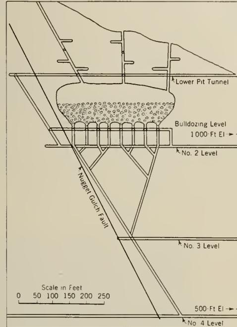
Fig. 3—Longitudinal Section Through Stope at Alaska Juneau Mine.
