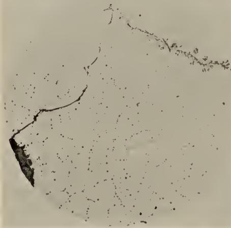
Fig. 4—Manganese Bronze Casting, Magnification 100. Quenched from 1,000 degrees F. in water.
