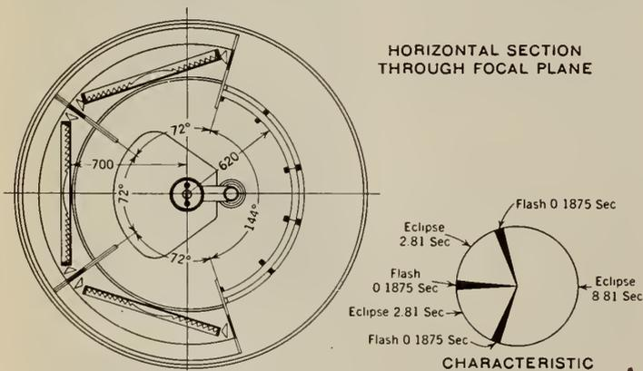
Fig. 7—Section of Second Order Flashing Light.
