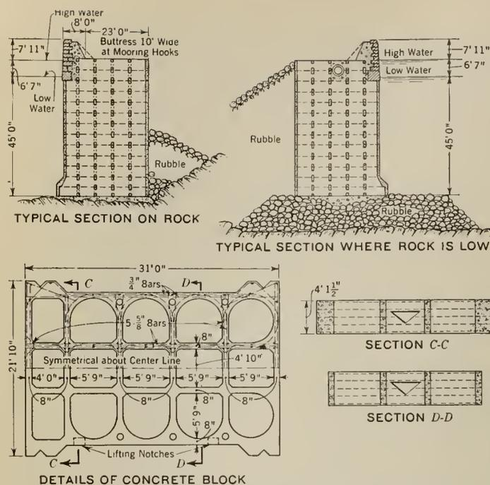
Fig. 1—Detail of Dock Wall Construction, Ocean Terminals, Halifax.
