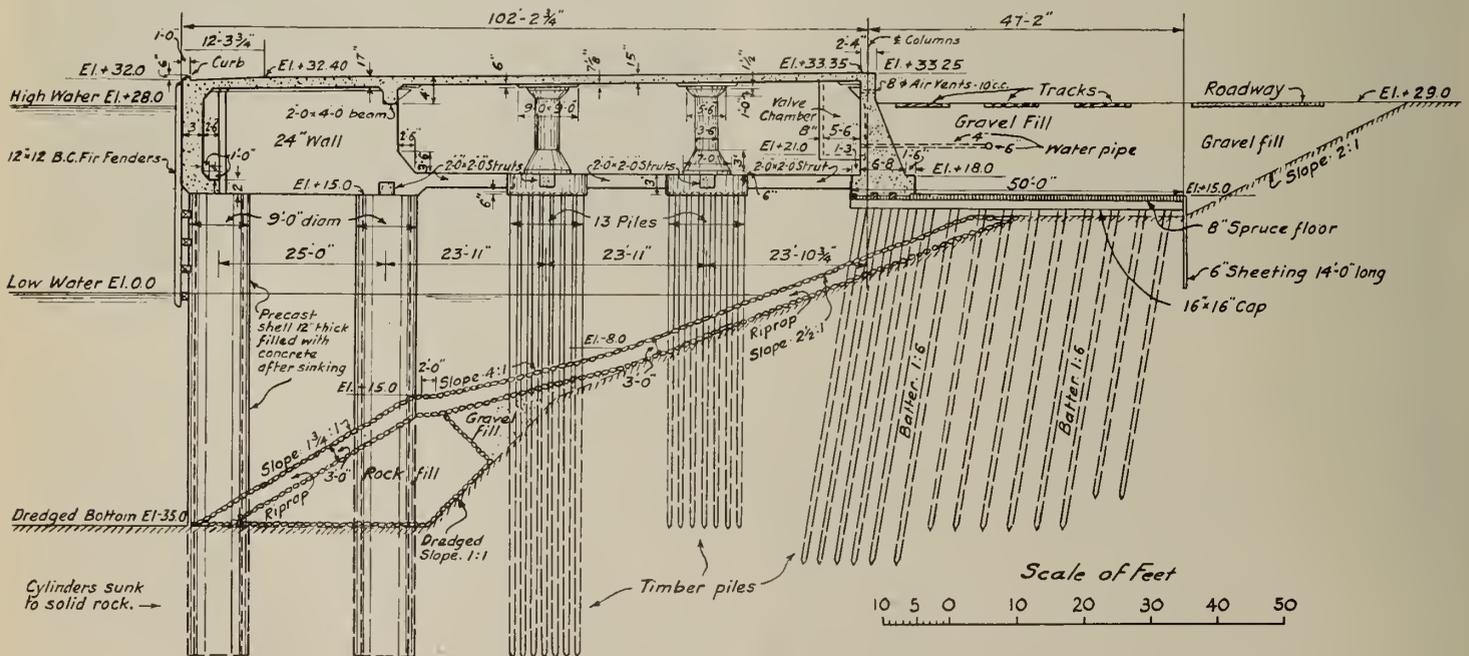
Fig. 5—Section Berths 1, 2, 3 and 4, Saint John, N.B.
