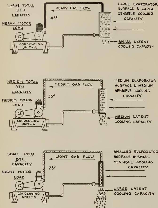
Fig. 2—Selection of Equipment for Central Plant Air Conditioning Systems.
