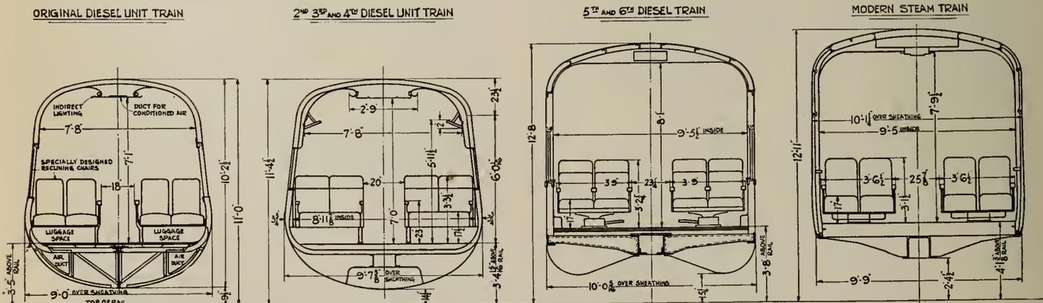
Fig. 5—Comparative Cross Sections of Passenger Cars.
