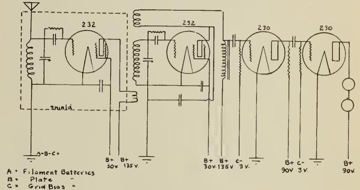
Fig. 5—Diagram of receiver remodelled for 2-volt tubes. The audio stages were changed to resistance coupling, as shown, at the same time.
