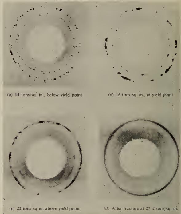
Fig. 2—X-ray patterns showing crystal breakdown.
