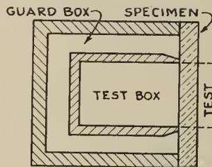
Fig. 2—Guarded Hot Box. The Guard Box and Test Box are kept at the same temperature by Electric Heaters and Fans.
