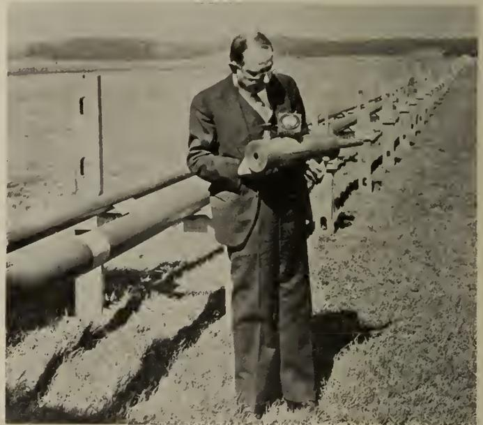
Fig. 7—Experimental Wave Guides shown in testing the Mathematical Theory of Guided Waves.
