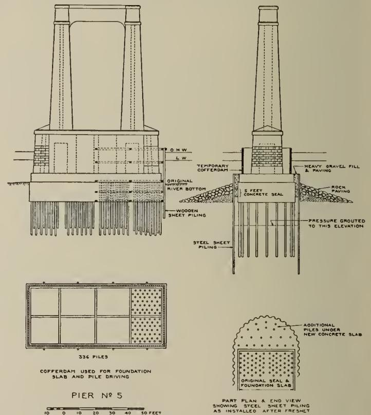
Fig. 12—Pier No. 5, Showing Plan of Restoration.
