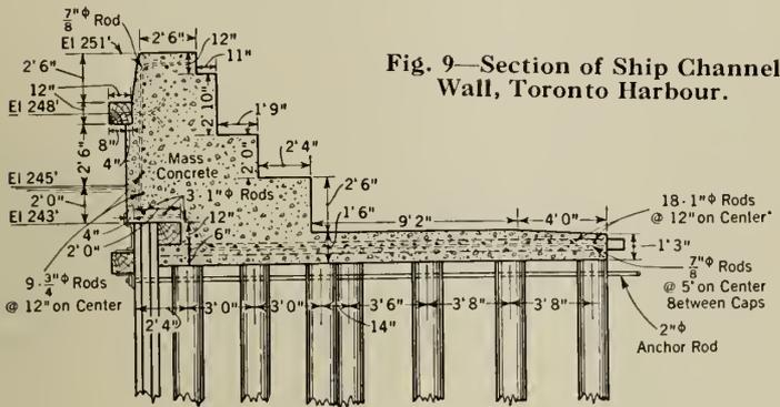
Fig. 9—Section of Ship Channel Wall, Toronto Harbour.
