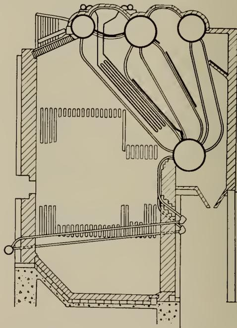
Fig. 18—C-E Bent Tube Boiler, Waterwalls, Type D Burners and Air Preheater. Moose Jaw Station.\*
