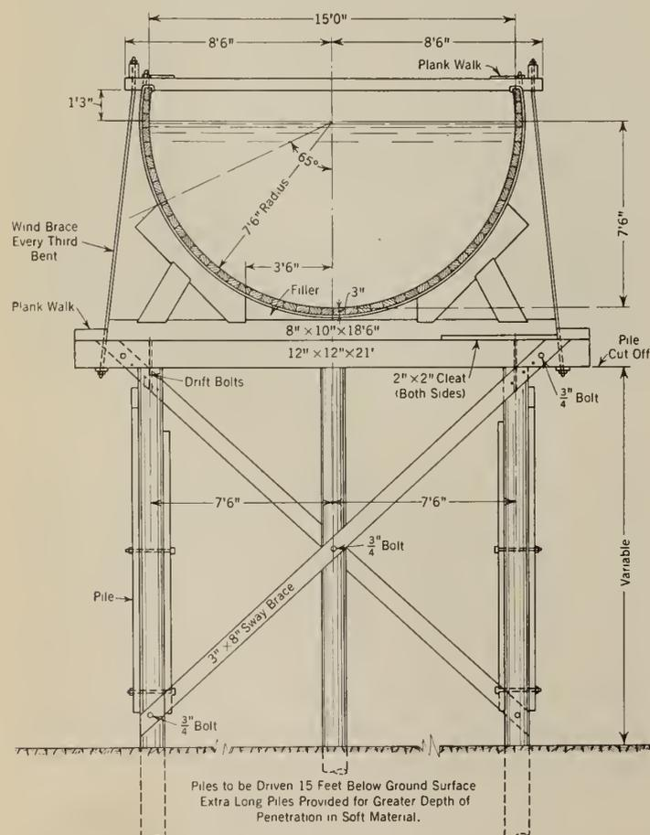
Fig. 12—Section of Lathom Flume.
