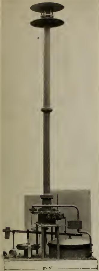
Fig. 10—Automatic Acetylene Fog Signal Gun.
