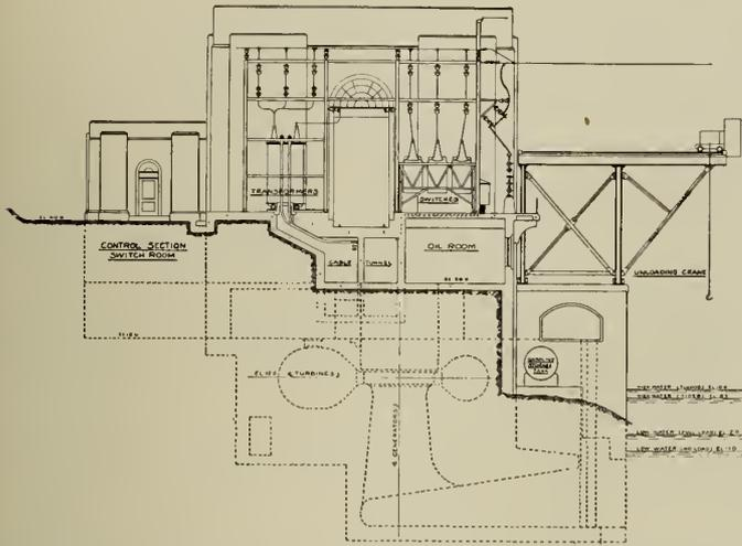
Fig. 6—Sectional Elevation, Transformer and Switching Station.
