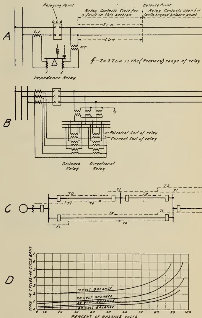
Fig. 2—Essentials of Distance Relaying for Transmission Circuits.
