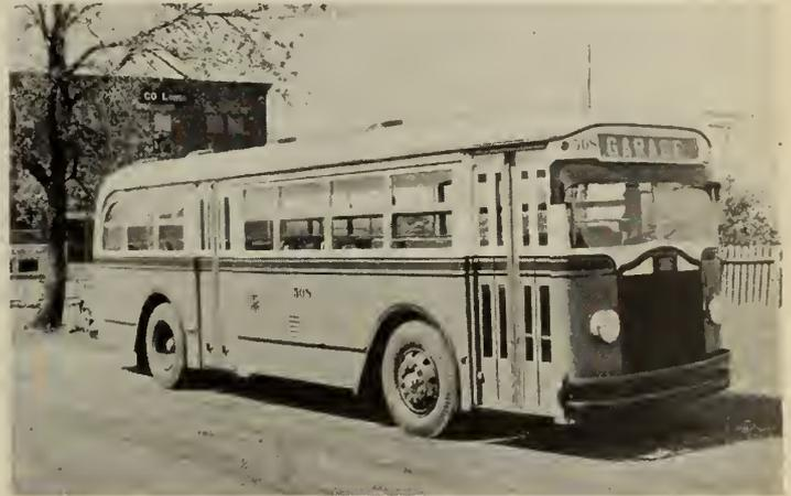
Fig. 14—36-Passenger Gas Bus, Transit Type. Montreal. 1936.
