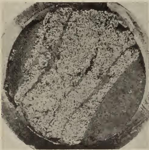
Fig. 5—Fracture produced by reversed axial stress.
