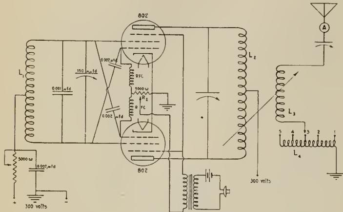
Fig. 7—Circuit diagram of Marconi portable transmitter, type 48030.
