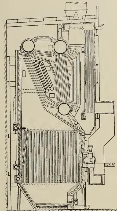
Fig. 4—Sectional View of Boiler 10.
