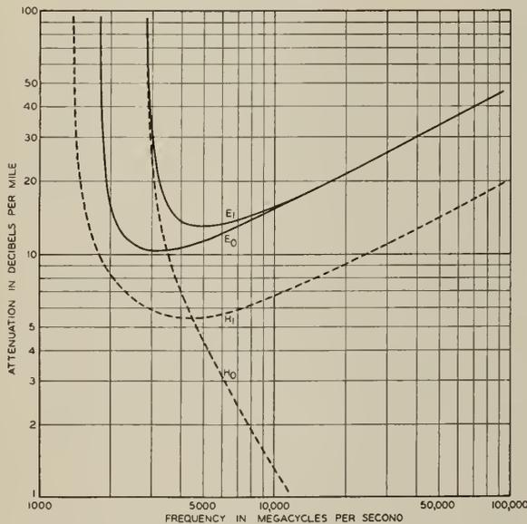
Fig. 6—Calculated Attenuation Characteristics of a 5-inch Hollow Copper Pipe.
