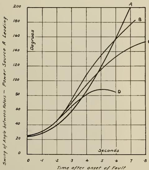
Fig. 5—Effect of Fault Clearance Time on Transient Stability of a System. Fault Location at X.—Phase to Phase to Phase.
