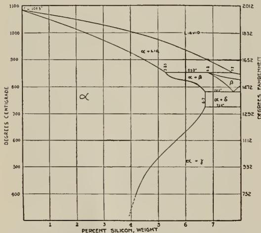
Fig. 10—Copper-Silicon Constitution Diagram. (0-8% Silicon.) (Smith.)
