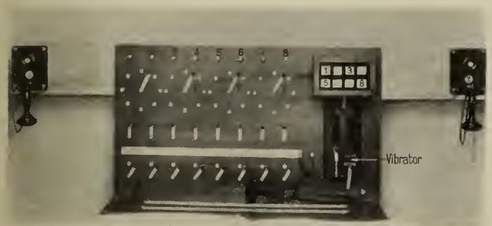
Fig. 6—Typical 8-Line Telephone Switchboard of about 1880.
