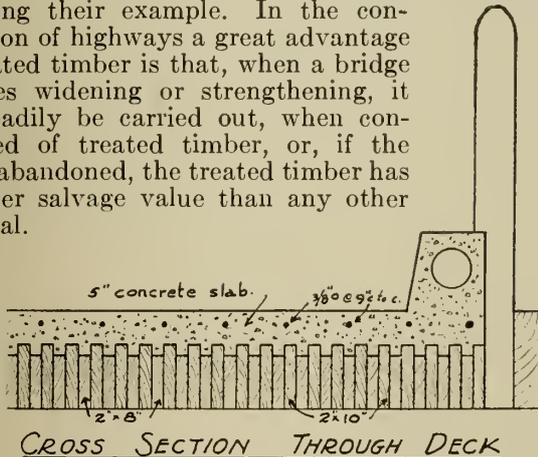
Fig. 7—Construction of roadway for composite bridge illustrated in Fig. 3.
