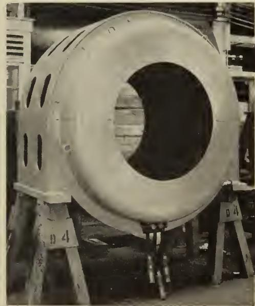
Fig. 2—End Bells for an Electric Motor.
