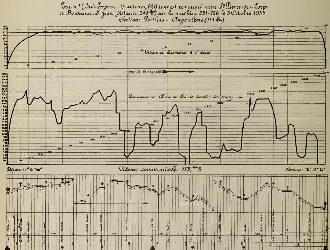
Fig. 4—Chart of Speed, Power and Profile Test with Rebuilt Pacific Locomotive on P.O.-Midi Railway.
