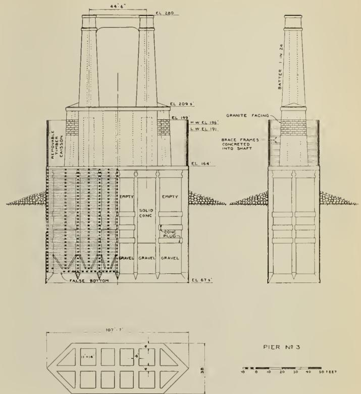
Fig. 5—Pier No. 3, Showing Caisson.
