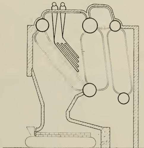
Fig. 15—Stirling Boiler with Economizer Coxe Stoker and Rear Arch Furnace. Lethbridge Station.\*
