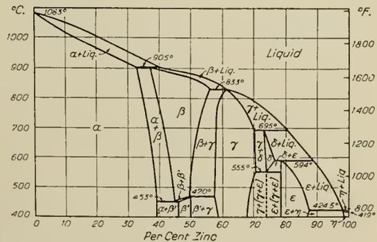
Fig. 8—Constitution of Copper-Zinc Alloys.
