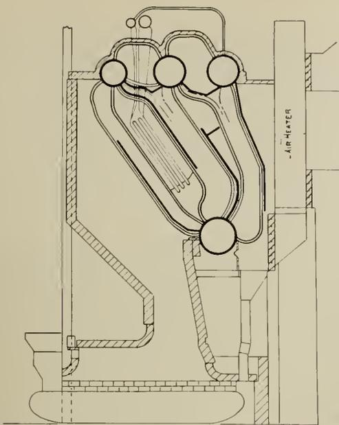
Fig. 13—B-W Steam Generator with Tubular Air Preheater, Harrington Stoker and Air-Cooled Furnace. Edmonton Station.\*
