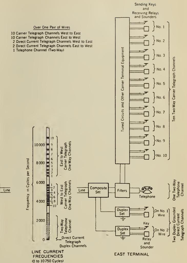
Fig. 4—Diagram Illustrating Open Wire Carrier Telegraph System (Type 50-B-H).
