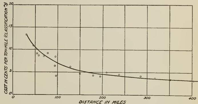
Fig. 2—Cost of Inter-City Truck Freighting out of Montreal.
