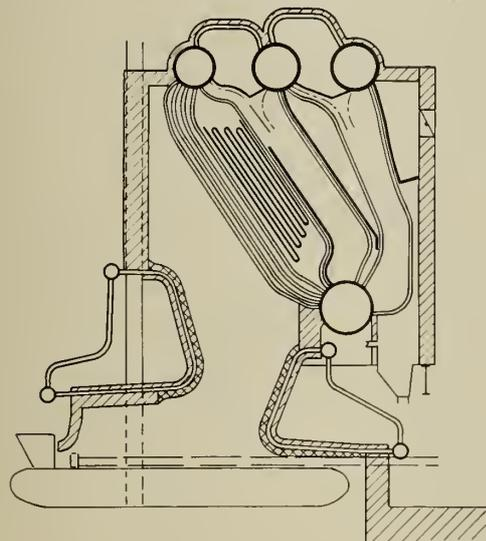
Fig. 14—B-W Steam Generator, Chain Grate Stoker, Water-cooled Front and Rear Arches. Saskatoon Station.\*
