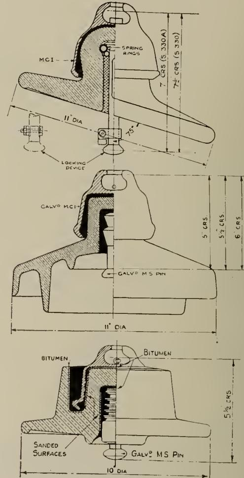
Fig. 3—Anti-Fog Type Insulators.
