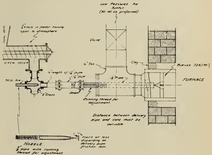
Fig. 2—Arrangement of Powdered Coal Burner.
