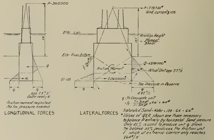
Fig. 3—Study of Pier No. 3, Lateral and Longitudinal Forces.
