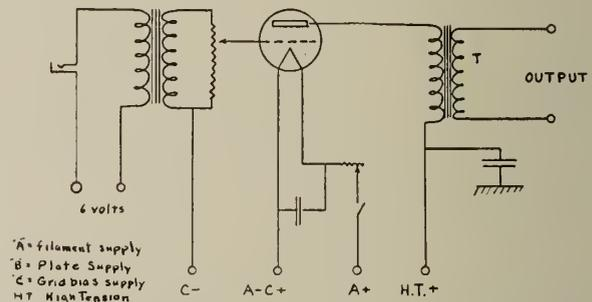
Fig. 3—Diagram of speech amplifier using transformer coupling.
