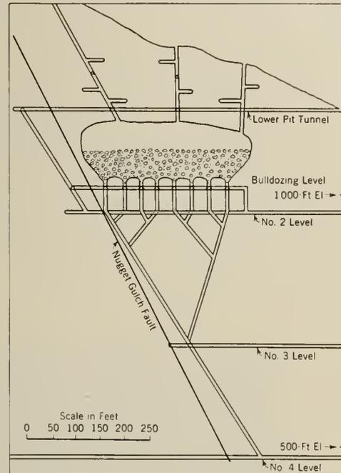
Fig. 3—Longitudinal Section Through Stope at Alaska Juneau Mine.
