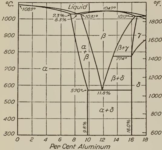
Fig. 9—Copper-Aluminum Constitution Diagram. (Stockdale.)
