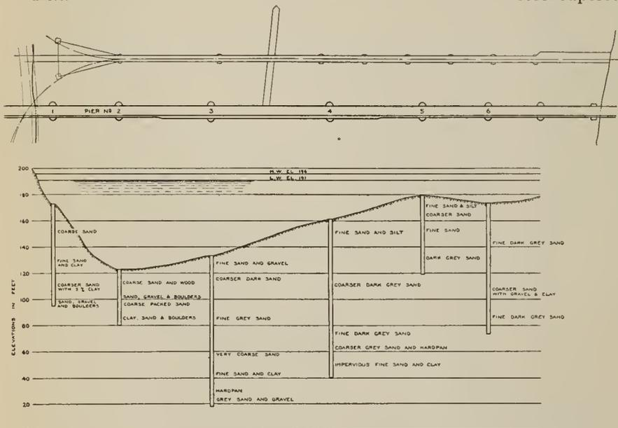
Fig. 2—Plan of Borings.
