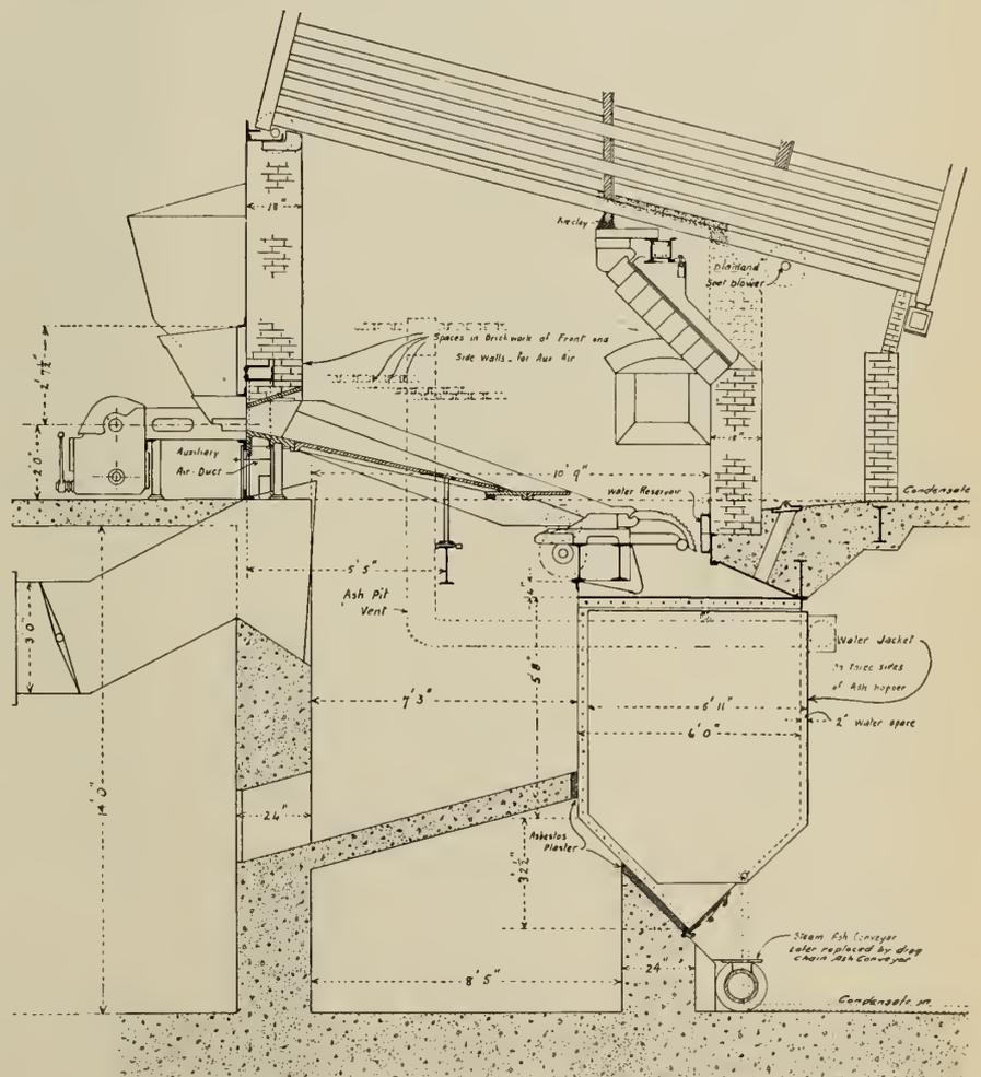
Fig. 2—Stoker Arrangement for Boilers 5 and 6.
