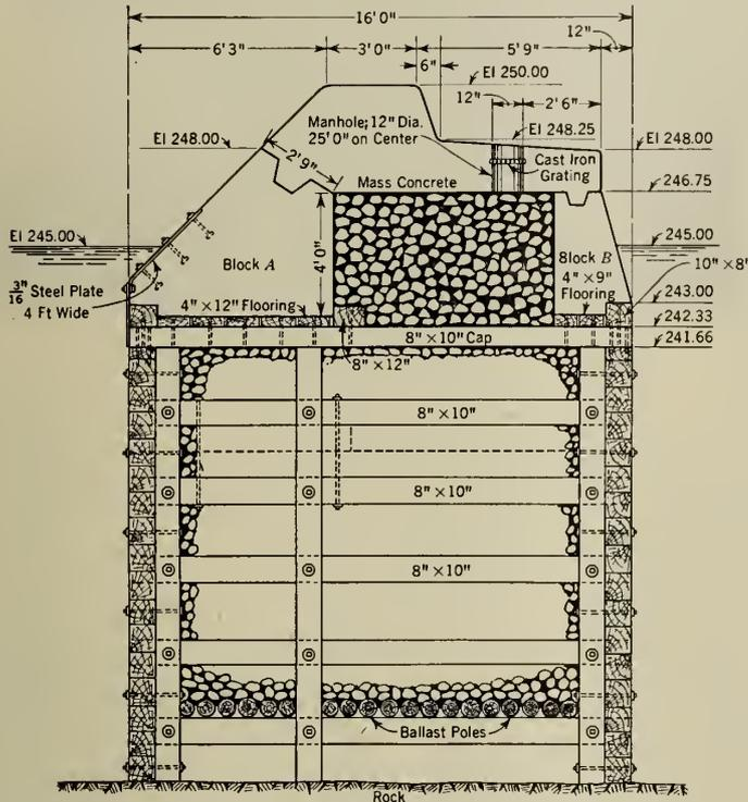
Fig. 12—Section of Western Breakwater, Toronto Harbour.
