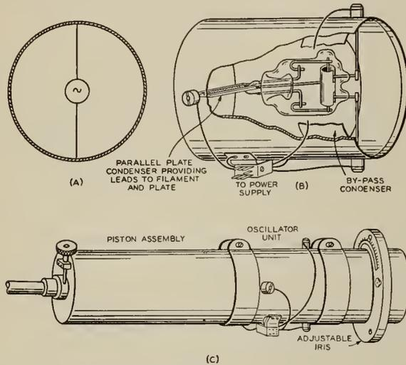
Fig. 10.—Various Component Parts of a Wave Guide Generator. (a) Schematic representation of Connections. (b) The Oscillator Unit. (c) Complete Generator including Oscillator, Iris and Piston.
