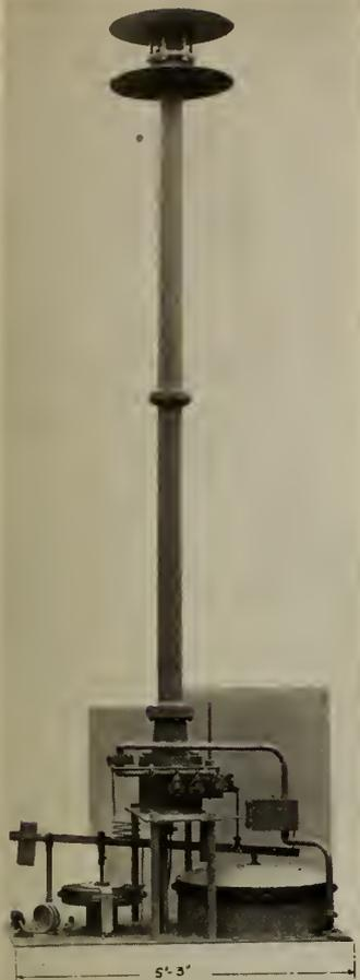
Fig. 10—Automatic Acetylene Fog Signal Gun.
