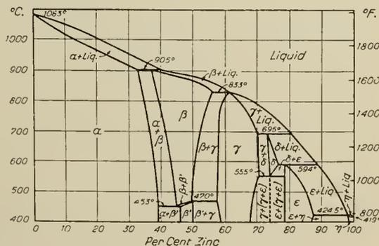
Fig. 8—Constitution of Copper-Zinc Alloys.
