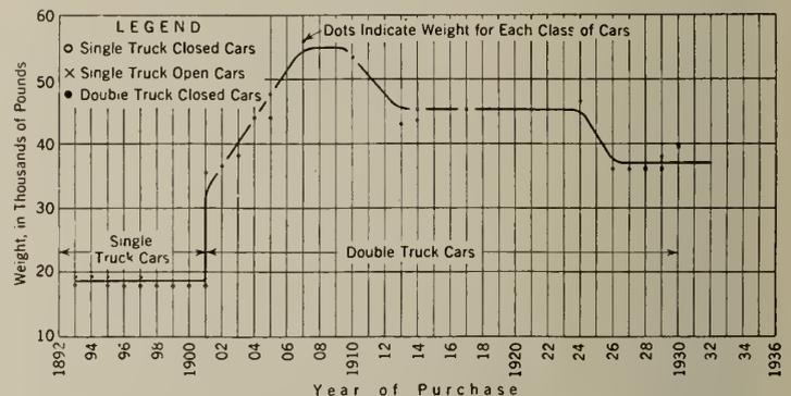
Fig. 6—Curve Showing Trend in Weight of Street Cars.
