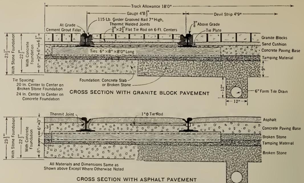
Fig. 21—Standard Track Construction, Montreal. 1932.
