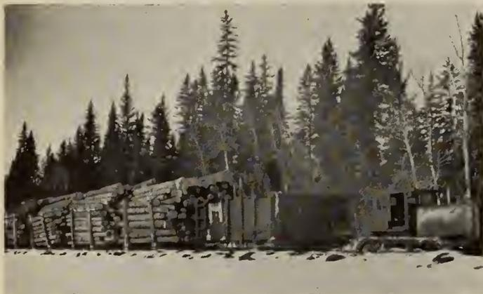
Fig. 3—Tractor-Train consisting of Caterpillar Tractor, Water Tank and 17 Sleighs (only part shown in photograph) of Logs containing 125,000 f.b.m.
