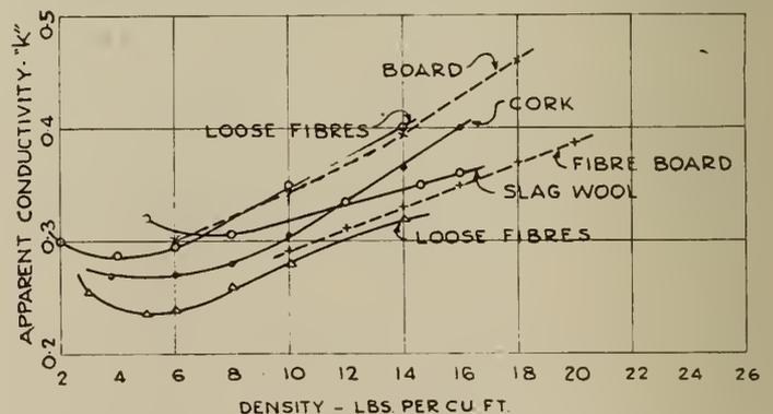
Fig. 8—Effect of Density on Heat Conductance of Insulating Materials.
