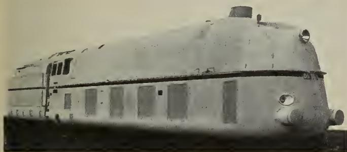
Fig. 10—Streamlined 4-6-4 German Reichsbahn Locomotive Class 05.
