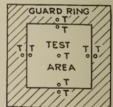
Fig. 4—Guarded Hot Plate. Thermocouples are Indicated by "T."
