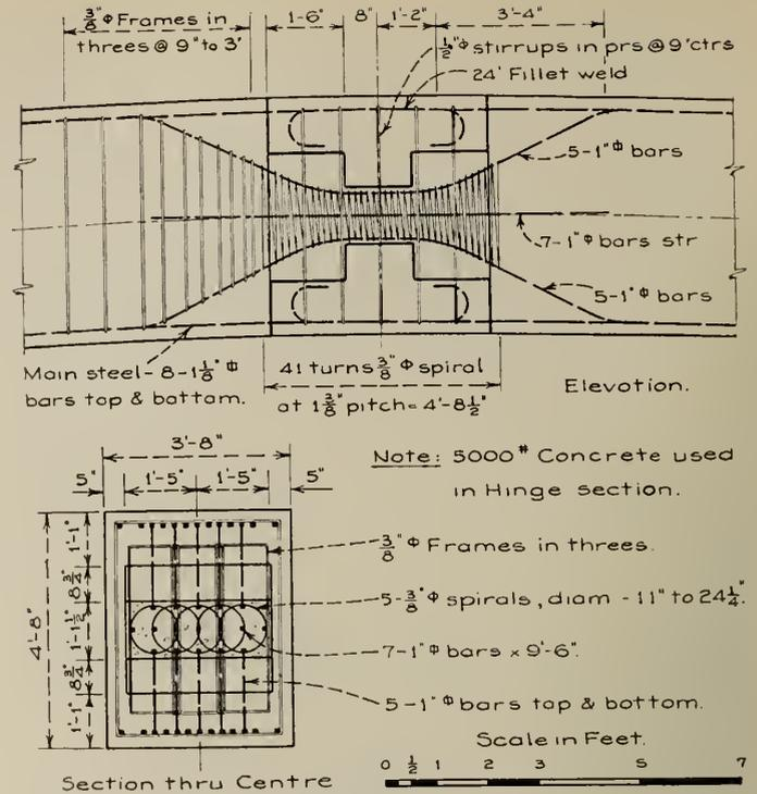
Fig. 9—Details of Crown Hinge.
