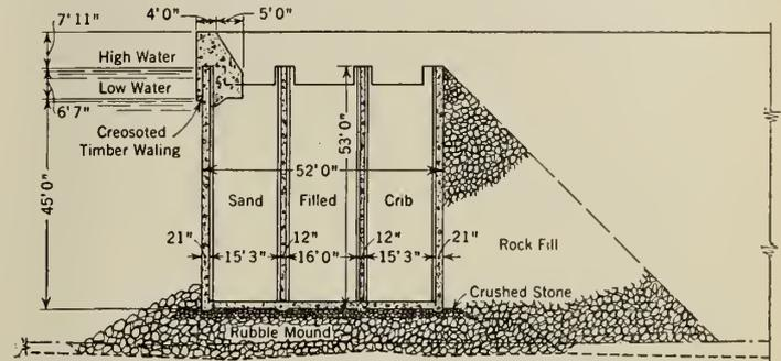
Fig. 3—Section of Dock Wall, Pier B, Halifax.
