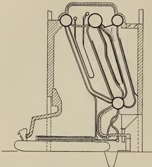
Fig. 17—Stirling Boiler with Dutch Oven, Water-cooled Rear Arch and Side Walls above Stoker Grate Line. Picture Butte Station.
