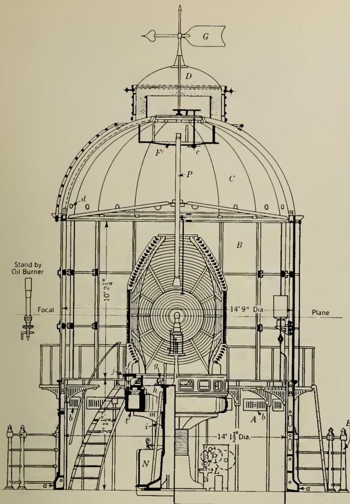
Fig. 5—General Arrangement of Lighthouse Lantern.
