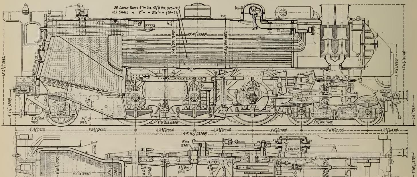
Fig. 1—Longitudinal Section of P.O.-Midi Pacific Locomotive.
