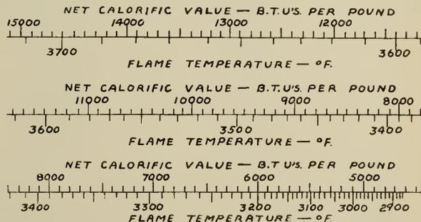
Fig. 6—Net Calorific Value of Coal and Flame Temperature. (Taken from Seylers Fuel Chart.)
