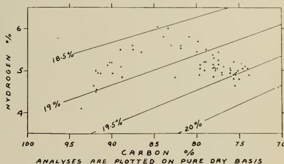
Fig. 5—Canadian Coal Band and Iso-Carbon Dioxide Lines for Dry Flue Gas. (Plotted on Seyler's Classification Basis.)
