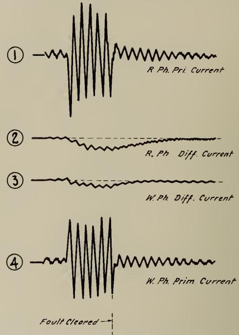
Fig. 4—Transient Differential Relay Occurrence.
