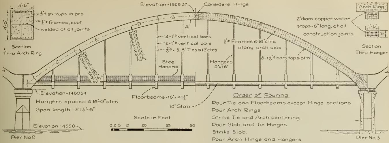
Fig. 6—Elevation of Span 5.
