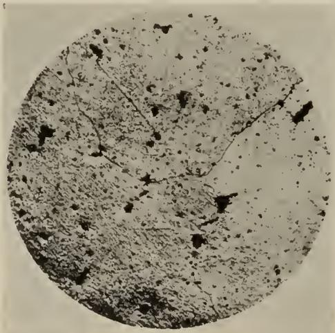
Fig. 14—10 per cent Tin-Bronze, Magnification 100, as Annealed at 1,000 degrees F. (Note that Dendritic structure and tin-copper compound have gone into solid solution.)
