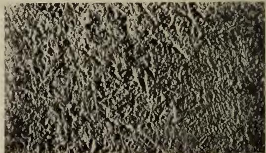
Fig. 15—Three-inch Diameter Bronze Stick Composition. 85 per cent copper—5 tin—5 lead—5 zinc. Unevenly Fed.
