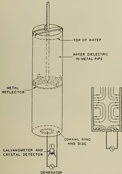
Fig. 2—Apparatus used in Determining Fundamental properties of Wave Guides.
