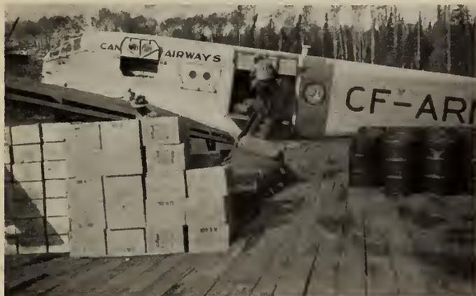
Fig. 10—Junkers 52, Payload on Floats 4,500 lb.
