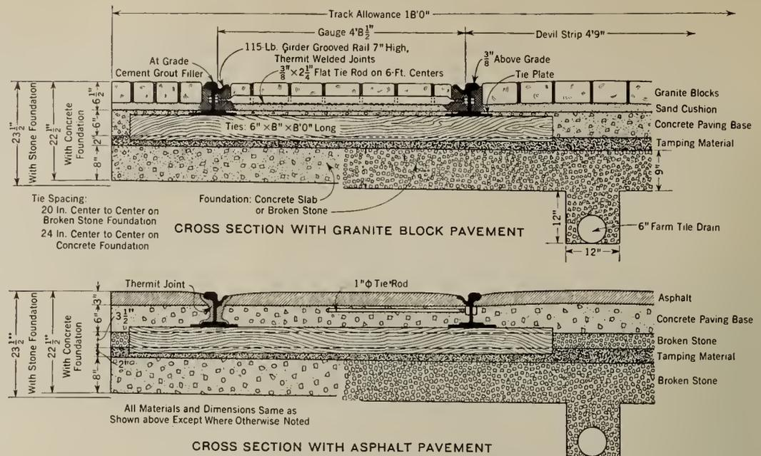
Fig. 21—Standard Track Construction, Montreal. 1932.
