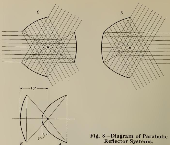
Fig. 8—Diagram of Parabolic Reflector Systems.
