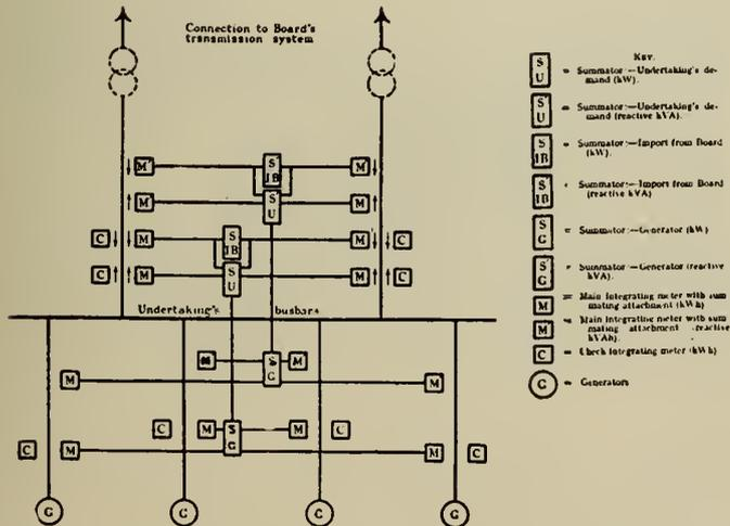
Fig. 7—Metering Scheme for Stations with Generating Plant.
