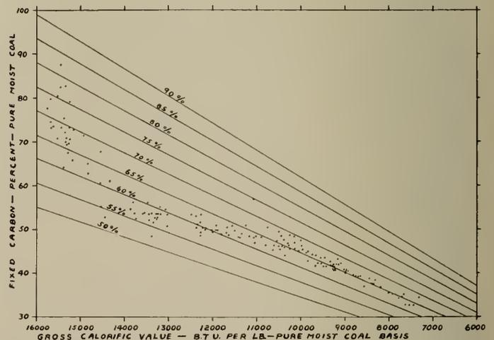
Fig. 3—Canadian Coal Band and Percentage of Heat in Non-Volatiles.
