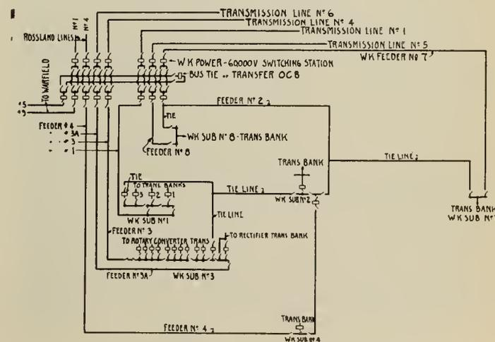
Fig. 3—60,000-Volt Lines, Feeders and Tie Lines, Tadanac.
