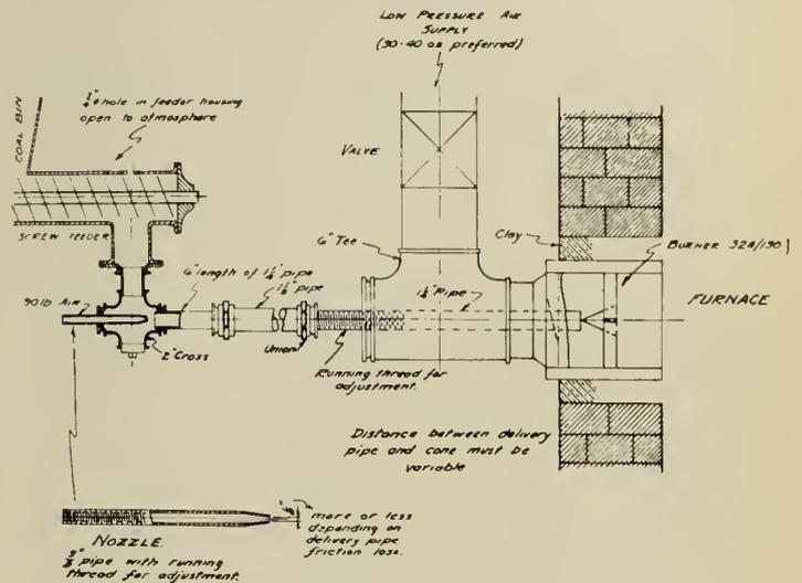
Fig. 2—Arrangement of Powdered Coal Burner.
