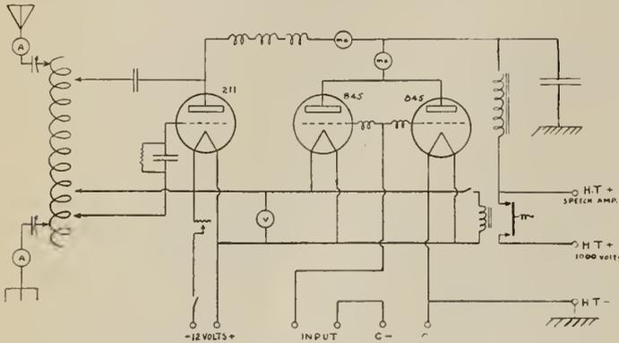
Fig. 2—Original transmitter installed for forestry communication.
