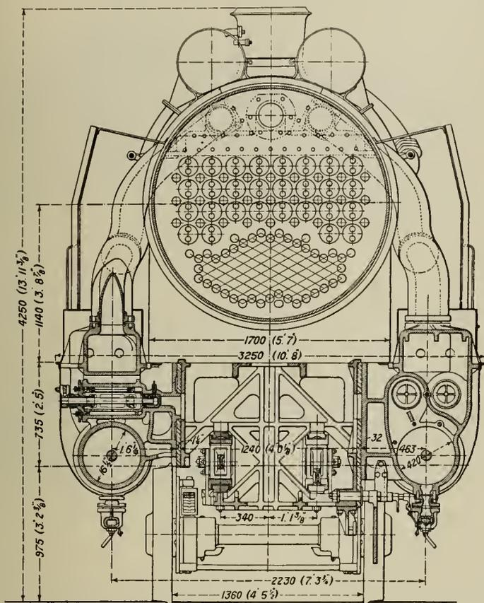
Fig. 2—Cross Section of P.O.-Midi Rebuilt Pacific Locomotive.
