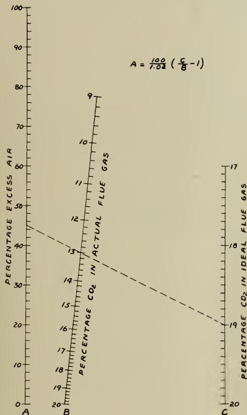
Fig. 4—Excess Air in Combustion of Coal and CO<sub>2</sub> in Flue Gases.
