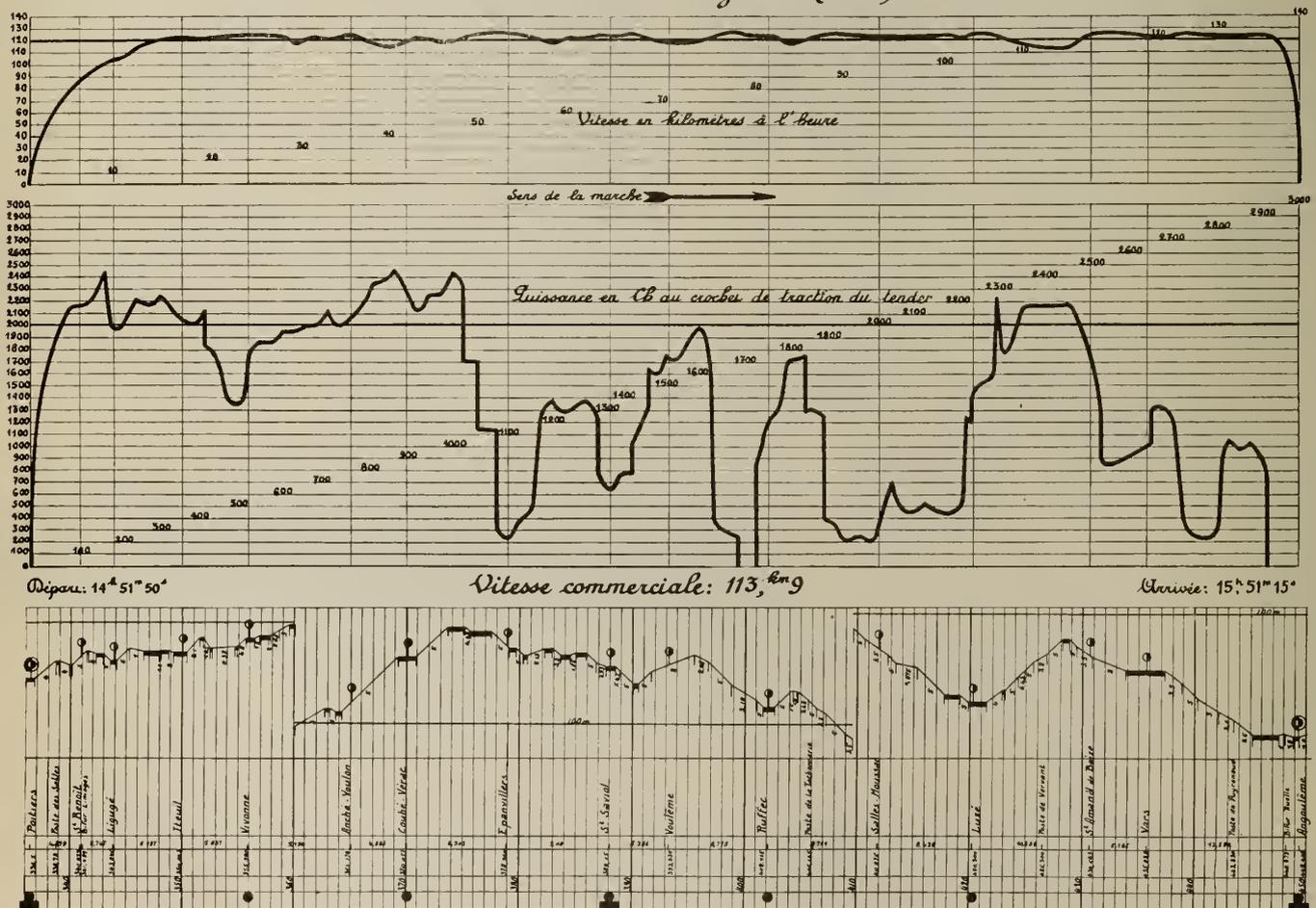
Fig. 4—Chart of Speed, Power and Profile Test with Rebuilt Pacific Locomotive on P.O.-Midi Railway.
