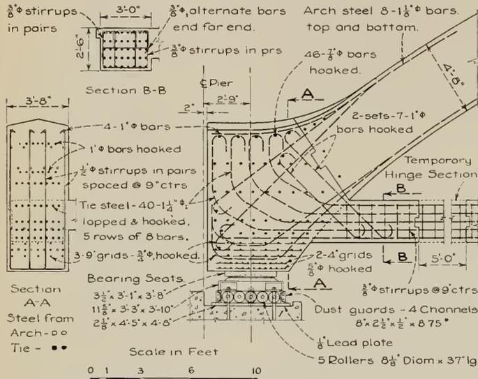
Fig. 7—Detail of Terminal Block.
