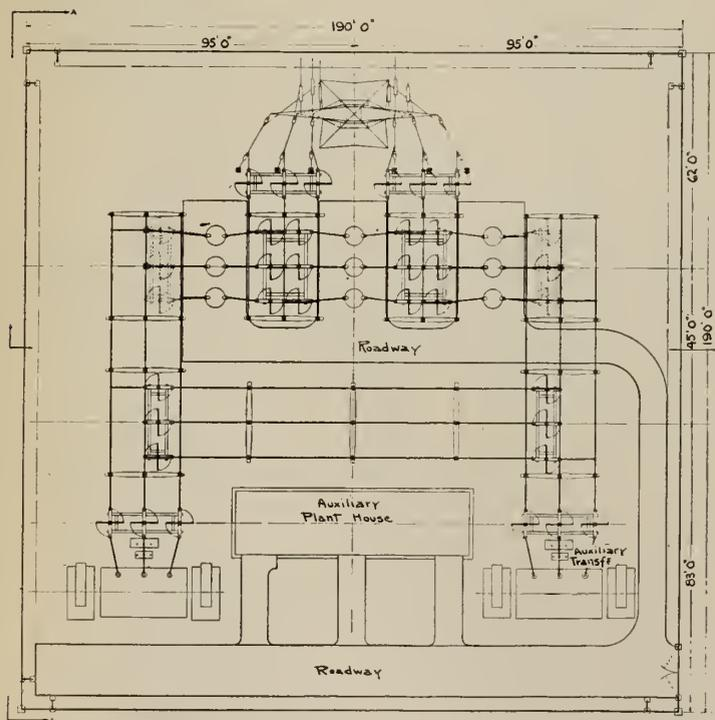
Fig. 5—Typical Mesh-Type Substation.
