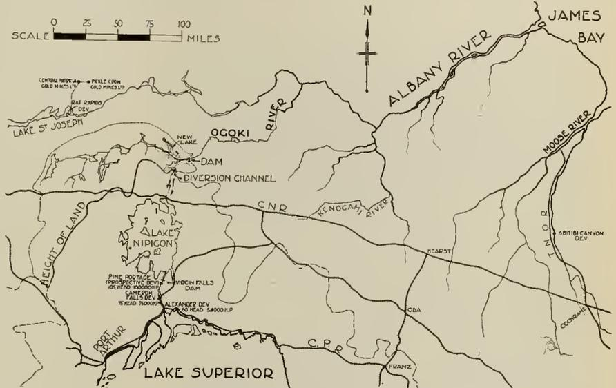
Fig. 4—Map showing proposed Diversion of Portion of Ogoki River into Lake Superior.
