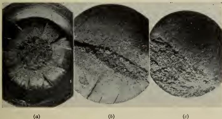
Fig. 3—Fractures produced by reversed bending.
