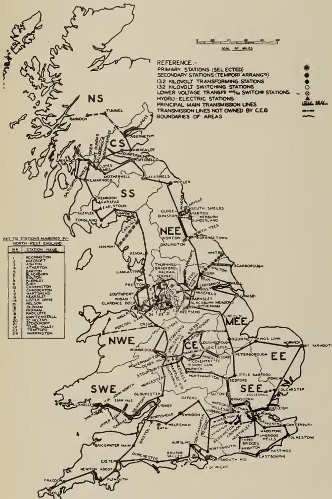
Fig. 1—Main "Grid" Transmission Lines.
