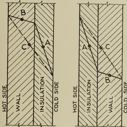
Fig. 5—Full Line—Actual Temperature Gradient.
