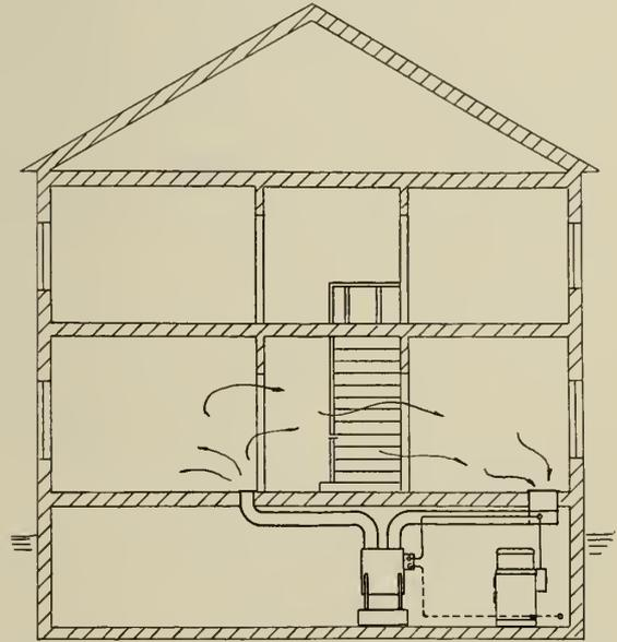
Fig. 1—Typical Installation of Winter Air-Conditioning for House with Radiator Heating, illustrating Heating Connections and Method of Air Distribution.
