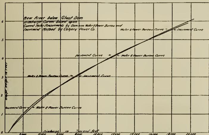
Fig. 2—Current Meter Measurements of Bow River by (a) Dominion Water and Power Bureau and (b) Increment Method.
