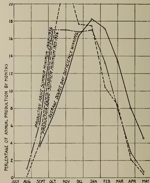
Fig. 3—Relation of Monthly Production of Lignite to Weather Conditions.
