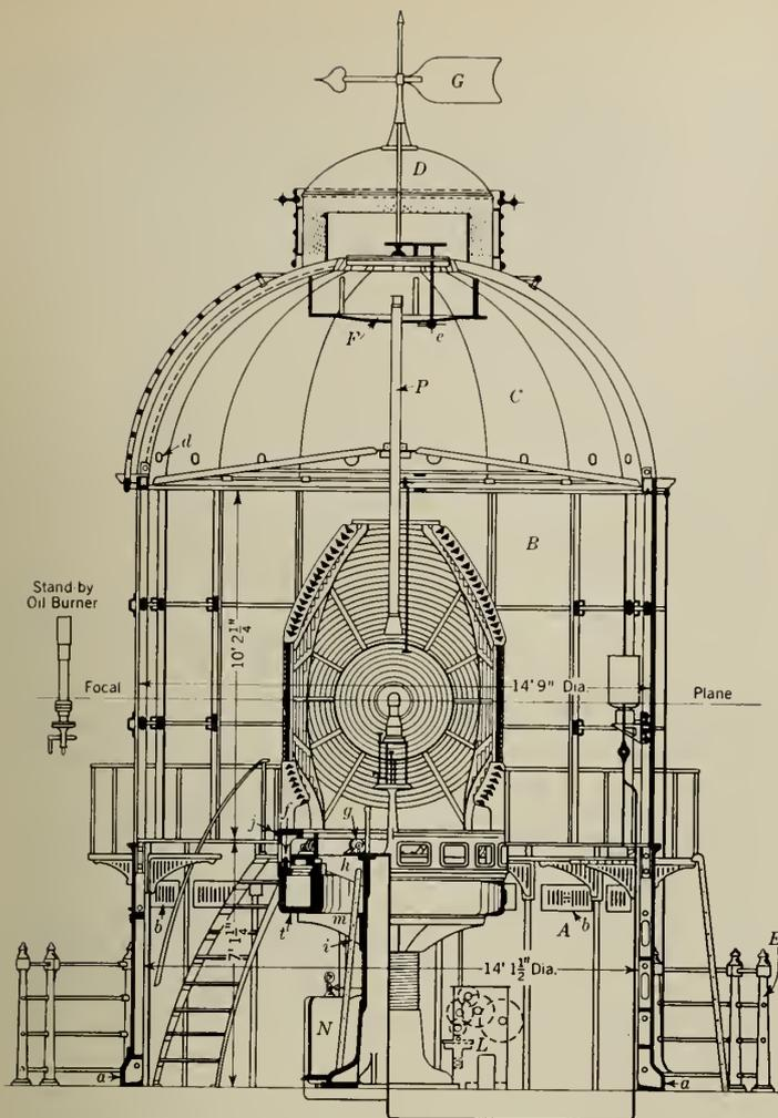
Fig. 5—General Arrangement of Lighthouse Lantern.
