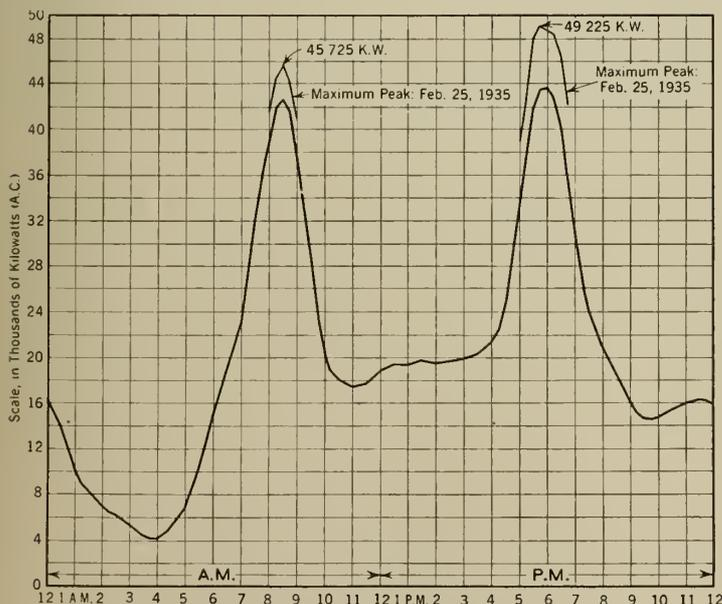
Fig. 20—Typical Load Curve in Winter. Montreal Tramways Company.
