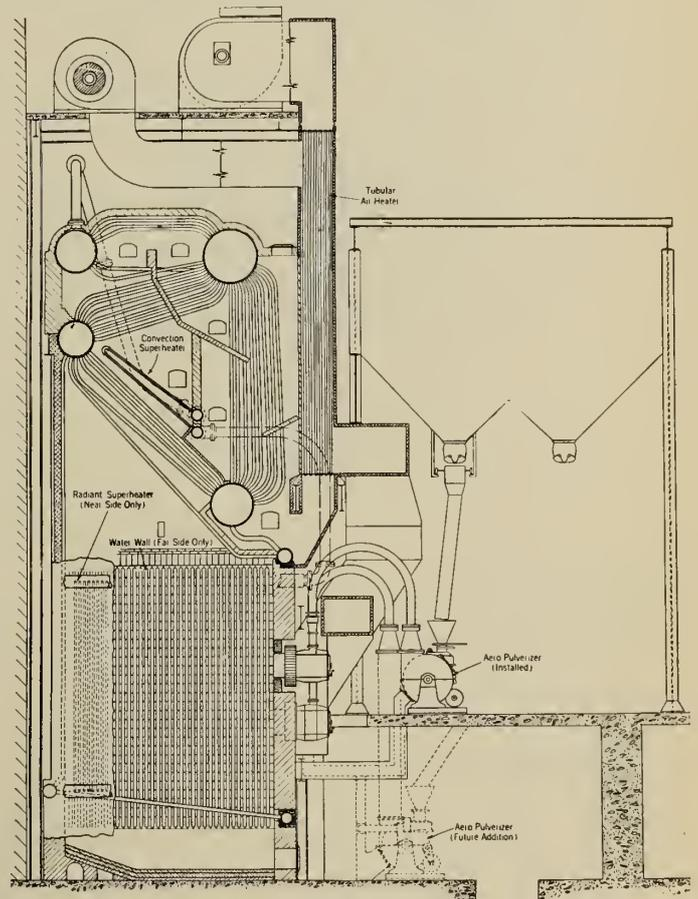
Fig. 3—Sectional View of Boiler 9.
