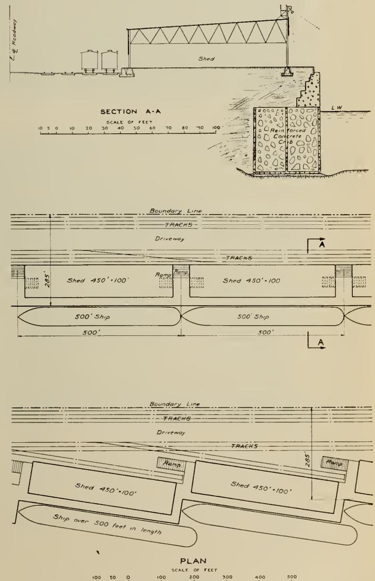
Fig. 8—Two Types of Shore Wharf Construction, Montreal Harbour.
