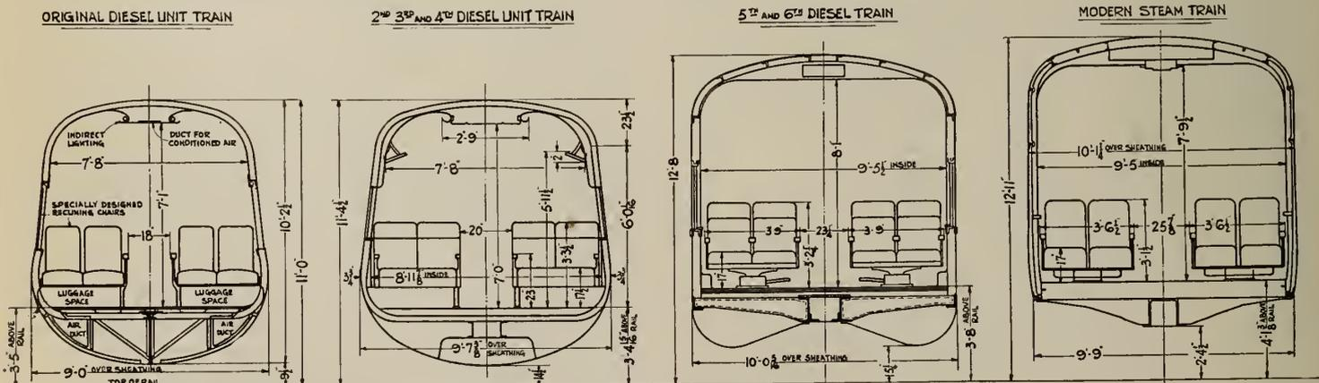
Fig. 5—Comparative Cross Sections of Passenger Cars.
