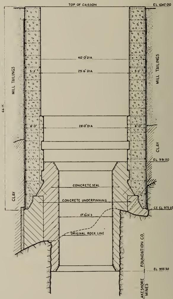
Fig. 3—Pneumatic Caisson for Shaft, Lake Shore Mines.
