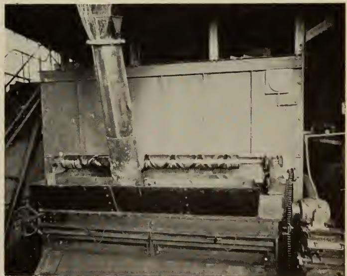
Fig. 19—Traversing Coal Chute.
