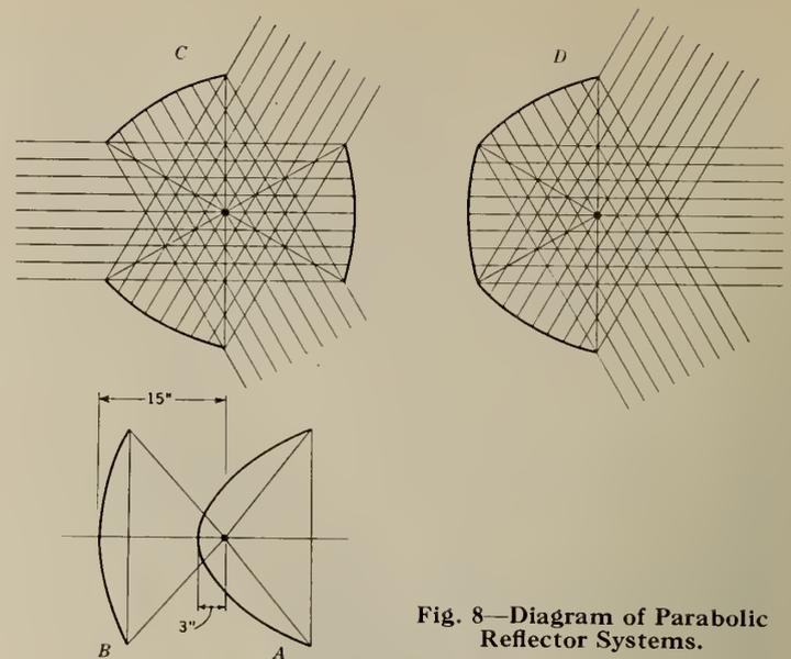
Fig. 8—Diagram of Parabolic Reflector Systems.
