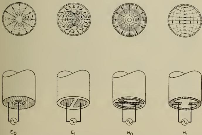
Fig. 3—Methods of launching various types of Waves in a Guide.
