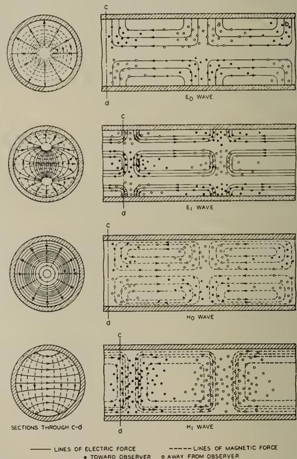
**Fig. 1**—Some of the Possible Configurations of Lines of Electric and Magnetic Force that may be transmitted through a Wave Guide. Propagation is assumed to be directed to the right and away from the Observer.
