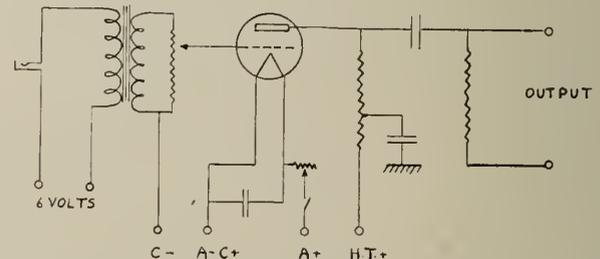
Fig. 4—Diagram of speech amplifier changed to resistance coupling.
