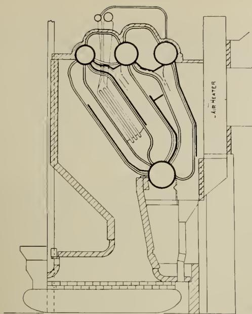
Fig. 13—B-W Steam Generator with Tubular Air Preheater, Harrington Stoker and Air-Cooled Furnace. Edmonton Station.\*
