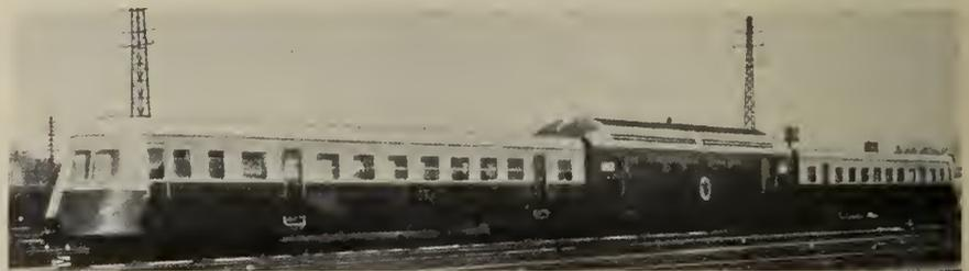
Fig. 12—Renault 1,000 b.h.p. Diesel-Mechanical Train.
