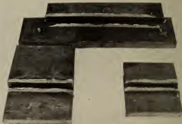
Fig. 4—Samples of Tested First Class Welds.
