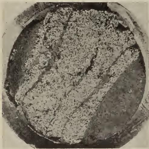
Fig. 5—Fracture produced by reversed axial stress.
