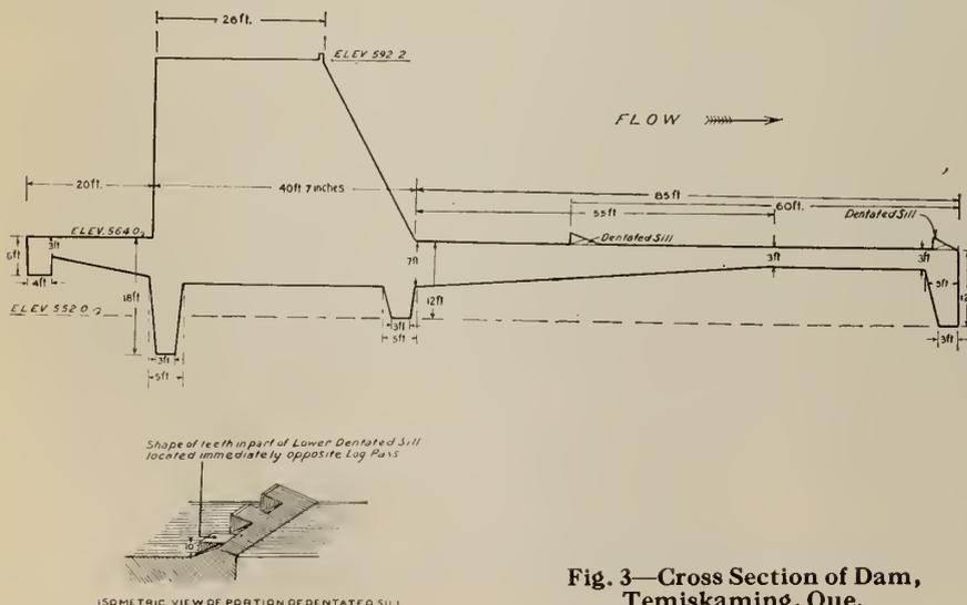
Fig. 3—Cross Section of Dam, Temiskaming, Que.
