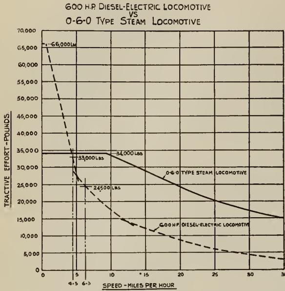
Fig. 4—Speed-Tractive Effort Curves, Switching Locomotives.
