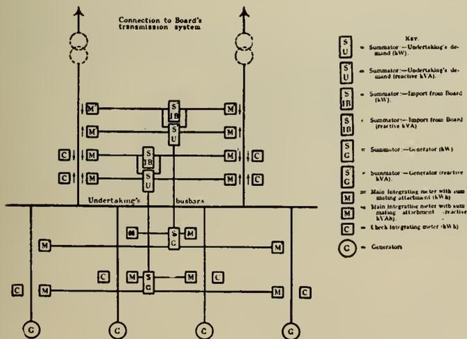
Fig. 7—Metering Scheme for Stations with Generating Plant.
