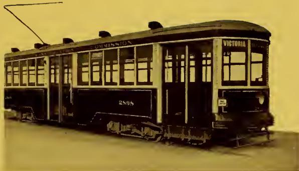
MODERN car operated in Toronto, 47 feet long, and equipped with 4-35 H.P. motors.
