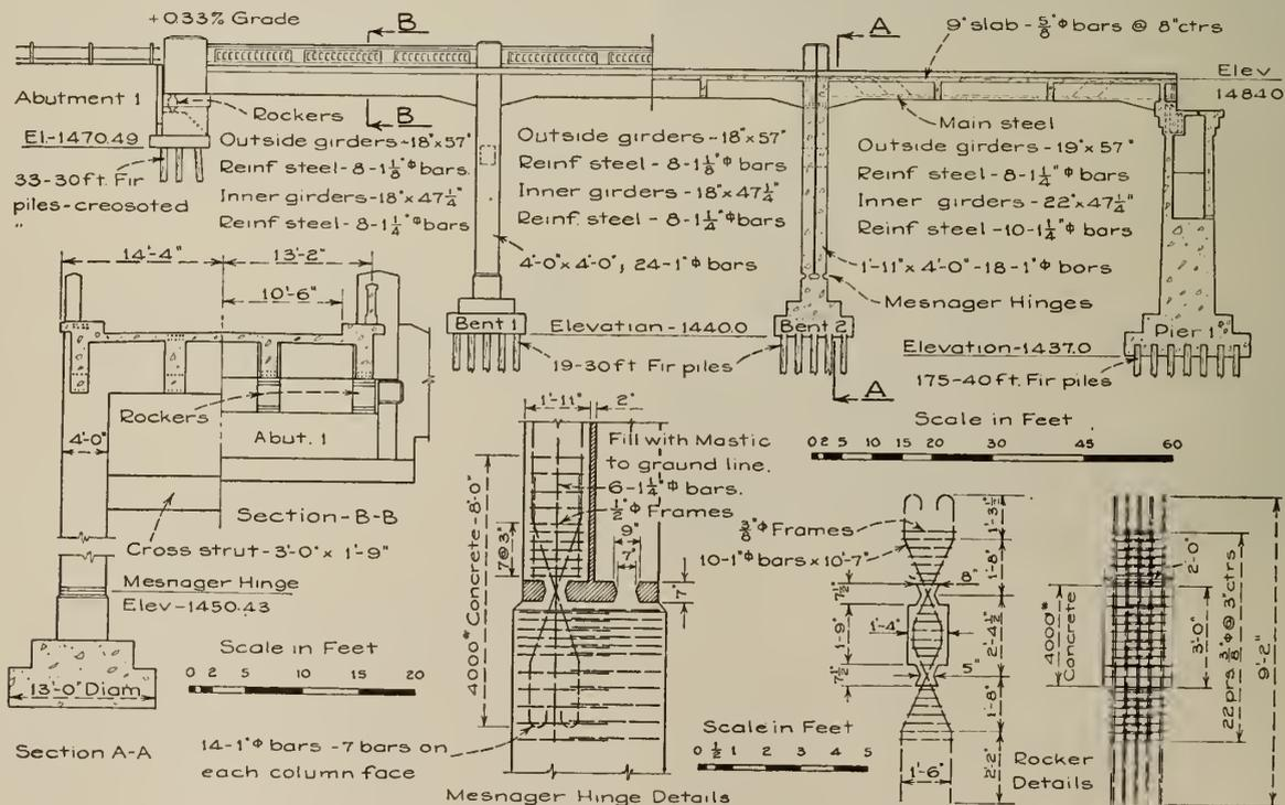
Half Elevation in sections of Girder Spans.
