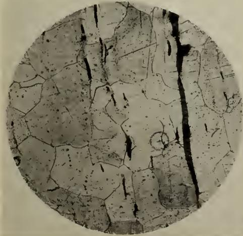
Fig. 1—Wrought Iron, Magnification 100.
