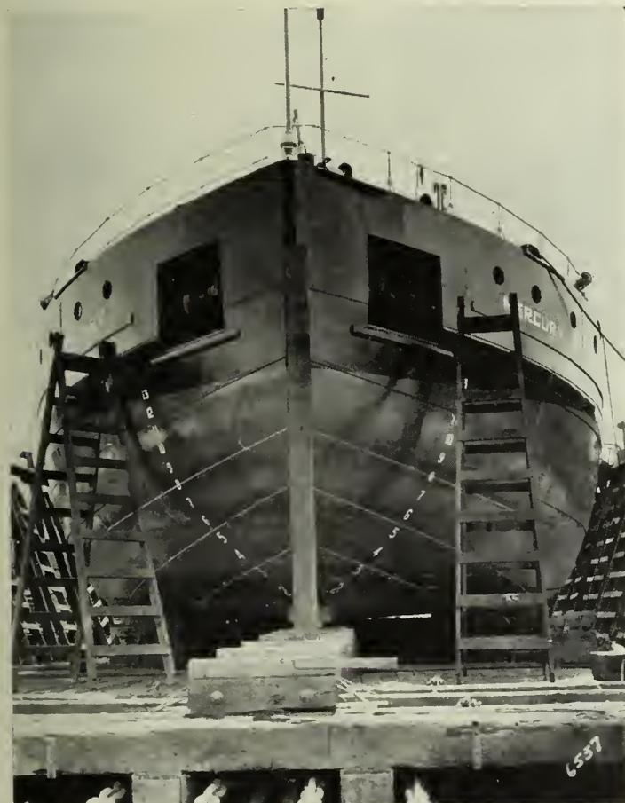
Fig. 3—All Welded Oiltanker, "Mercury," Bow View.
