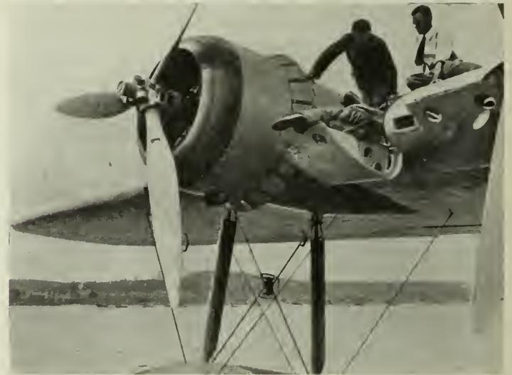
Fig. 3—Nacelle and Servicing Platform of Empire Boat.
