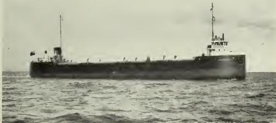
Fig. 1—All Welded Motor Lake Freighter "Franquelin."
