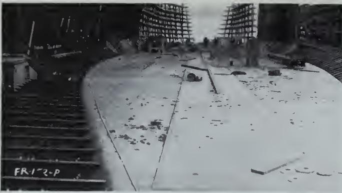
Fig. 5—Tank top showing centre strake, margin and floors.
