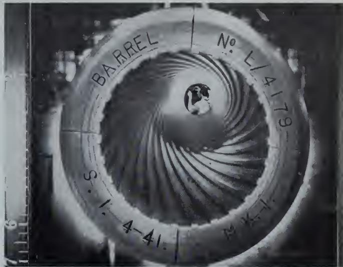
Fig. 6—Muzzle of 25-pounder barrel showing rifling.
