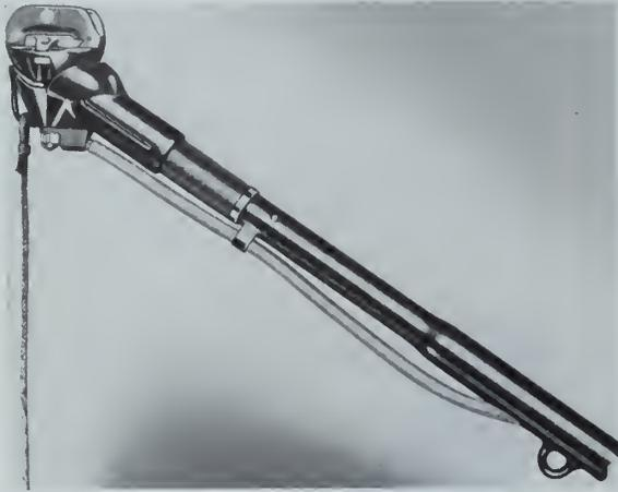
Fig. 3—Shoe collector with carbon insert.
