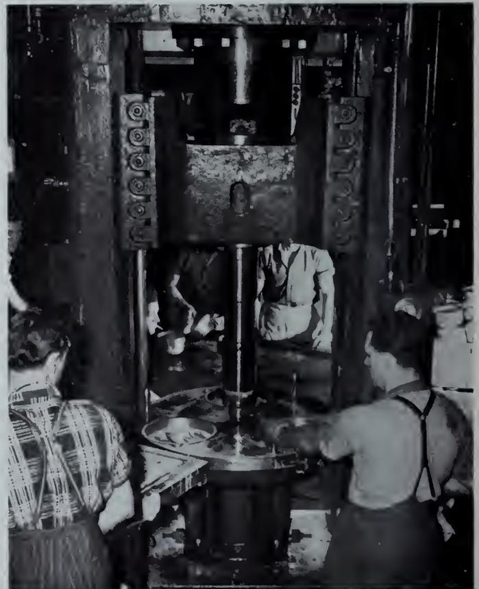
Fig. 7—Cupping 4-inch cartridge case on 300-ton press.
