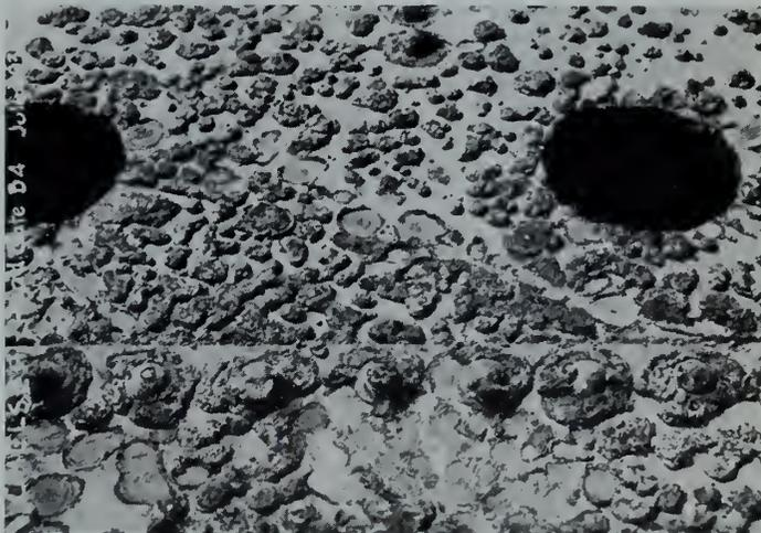
Close up view of rust tubercles. (Some of the tubercles have been scraped off.)
