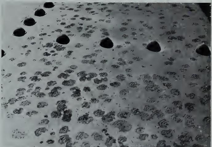
Close up view of cone shaped depressions formed by tubercles. This view shows the steel after grit blasting.
