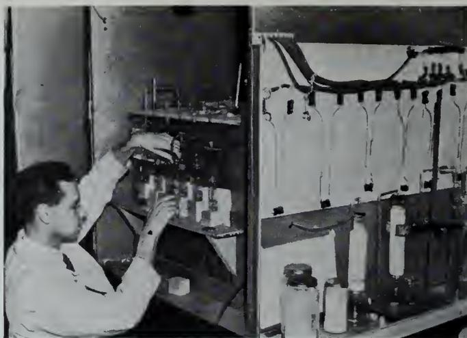
Apparatus for measuring permeability of fabrics by poison gases.
