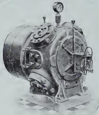
Quadruplex Compressors Single or Double Stage in pressures up to 350 lbs. per sq. in. and 520 cu. ft. per minute.
