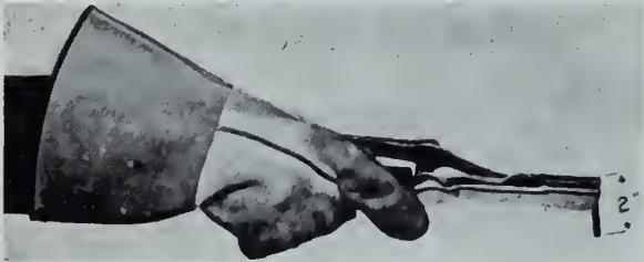
Fig. 1—Standard holder and separate stub.
