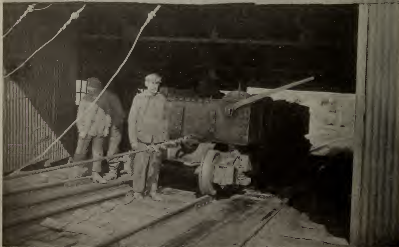
Main Slope Ore-Car. Makes the trip of two miles in five minutes with 20 tons of ore.
