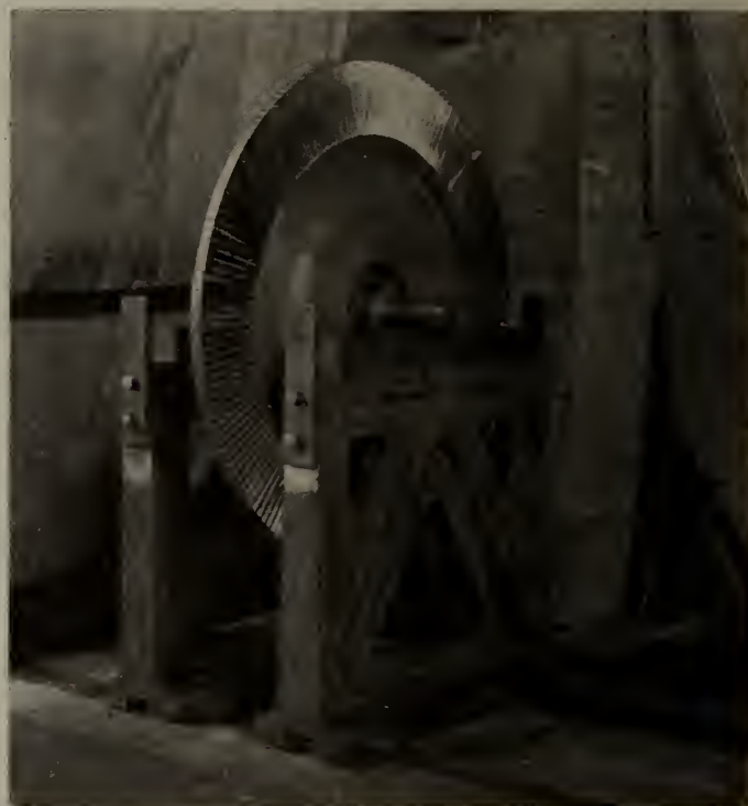
Fig. 4. Low-pressure Wheel of 2,100 h.p. Steam-turbine on static Balancing-wheel.
