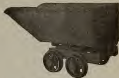
ROTARY SCOOP CARS. Roller Bearings, with dust excluding device. Dumps at either side or either end. Made in any size you want.
