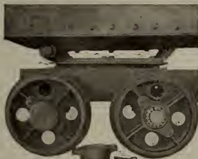
Showing the Roller Bearings supplied in all four wheels of our Mine Cars. Note the dust-excluding cap, with ample capacity for holding grease or oily waste.
