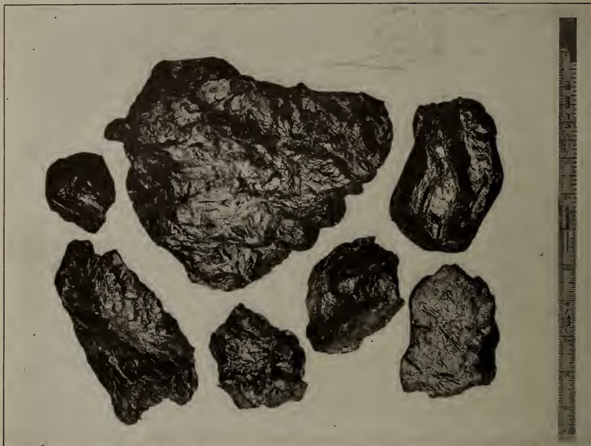
Typical high grade, Canadian flake graphite ore, 15-20 per cent carbon, from the Buckingham district, Que.
