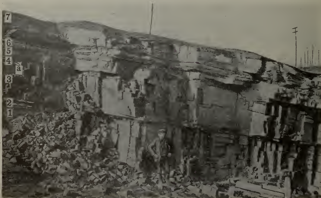
Surface Stripping on the Dominion Ore-bed, showing regular dip of seam, and characteristic cubical fracture of ore.
