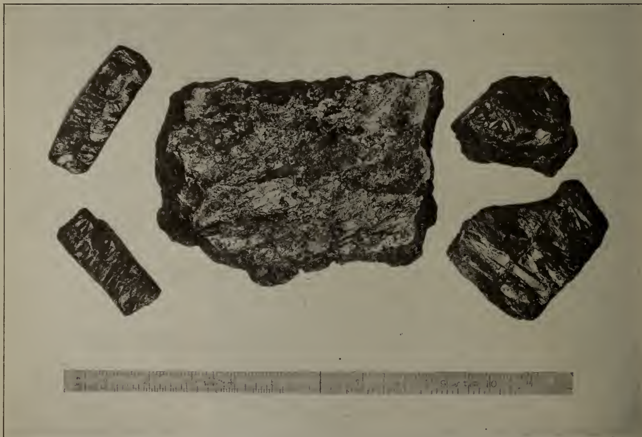
Foliated plumbago, from near Lake harbour, Baffin island. This material is reported to be the equal of Ceylon plumbago for crucible work.
