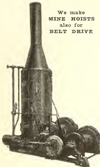
DOUBLE DRUM STEAM HOIST With Two Steam Cylinders and Govern- ment Inspected and Approved Boiler Built for 125 Pounds Working Pressure. The general purpose Hoist, for Der- rick and other work. Made in 7 sizes, from 10 to 50 H.P., and with one, two, or more drums.
