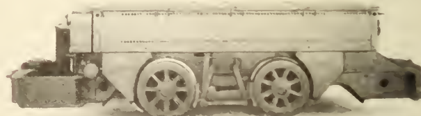
Fig. 6.—Gear-driven, storage-battery loco of large battery capacity. Both axles connected through worm-gears to single motor, and four wheels drive simultaneously.
