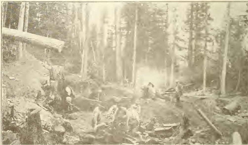
Placer Mining, on left bank of Discovery draw, Cedar Creek area, Cariboo, B. C. — The pay gravels are shown in the open cut beneath the fallen stump.
